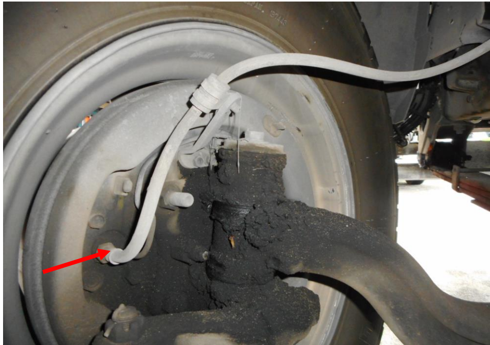
Photo 24 shows the brake hose/pipe (arrowed) at the front left wheel of the Motor Lorry. My static tests of the Motor Bus's braking system, along with my visual examination of the various mechanical components in the braking system had indicated that there was no internal leakage of pressure/vacuum. Hence the braking system of the Motor Bus was likely to be in serviceable condition at the material time of accident.
