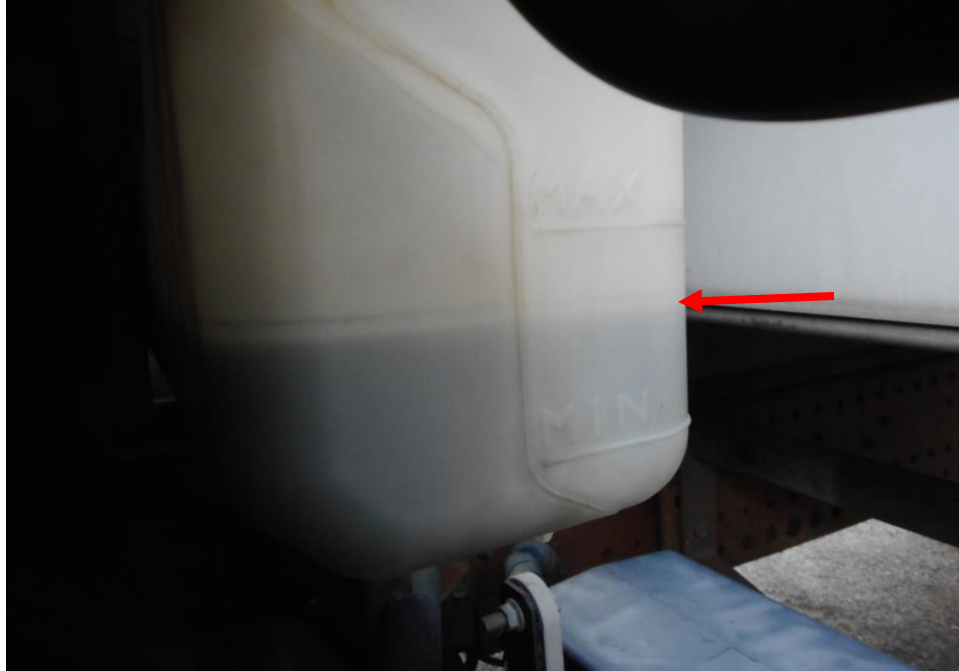
Photo 15 shows the engine coolant reservoir of the Motor Lorry at the time of my inspection. The engine coolant was observed to be of sufficient level (arrowed) and without any visible contamination.
