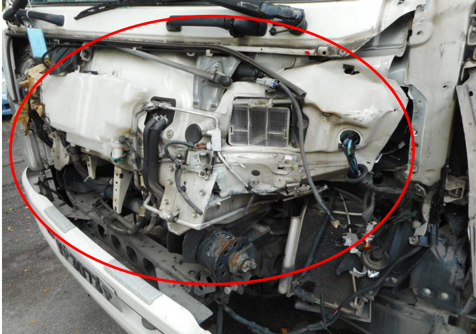
Photo 4 shows a close up view of the Motor Lorry's front portion at the time of my inspection. It appeared to have sustained damage at its front portion. Its front cabin panel (circled) were damage at the time of my inspection.
