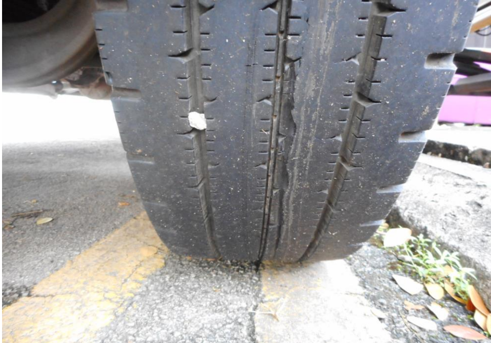
Photo 12 shows the condition of the rear right tyres of the Motor Lorry, which were observed to be in serviceable condition with remaining, tread depth of approximately 4.5mm. There was also no tear, cut or burst mark(s) on the outer and the inner sidewalls as well as across the tread of the 6 tyres that were fitted on the Motor Lorry.
