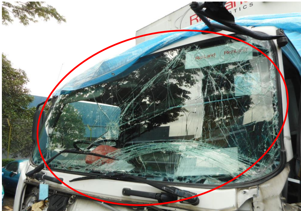
Photo 3 shows a close up view of the Motor Lorry's front portion at the time of my inspection. It appeared to have sustained damage at its front portion. Its front windscreen (circled) was damage at the time of my inspection as a result of the accident.
