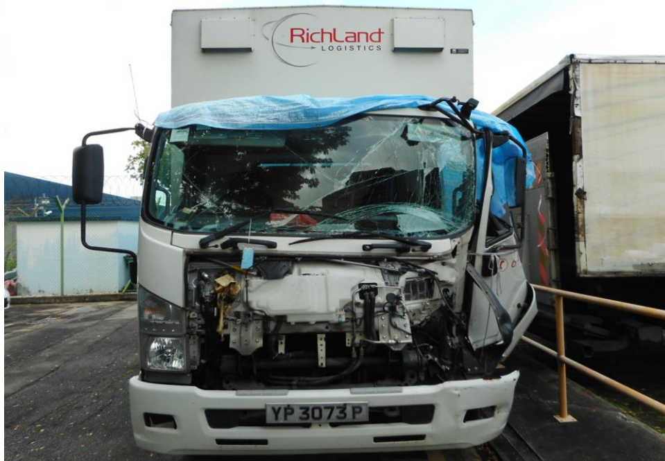
Photo 2 shows a general view of the Motor Lorry's frontal portion at the time of my inspection. The Motor Lorry was observed to have sustained damage at its front portion. Its front windscreen, front cabin panel and front left door were damage at the time of my inspection.
