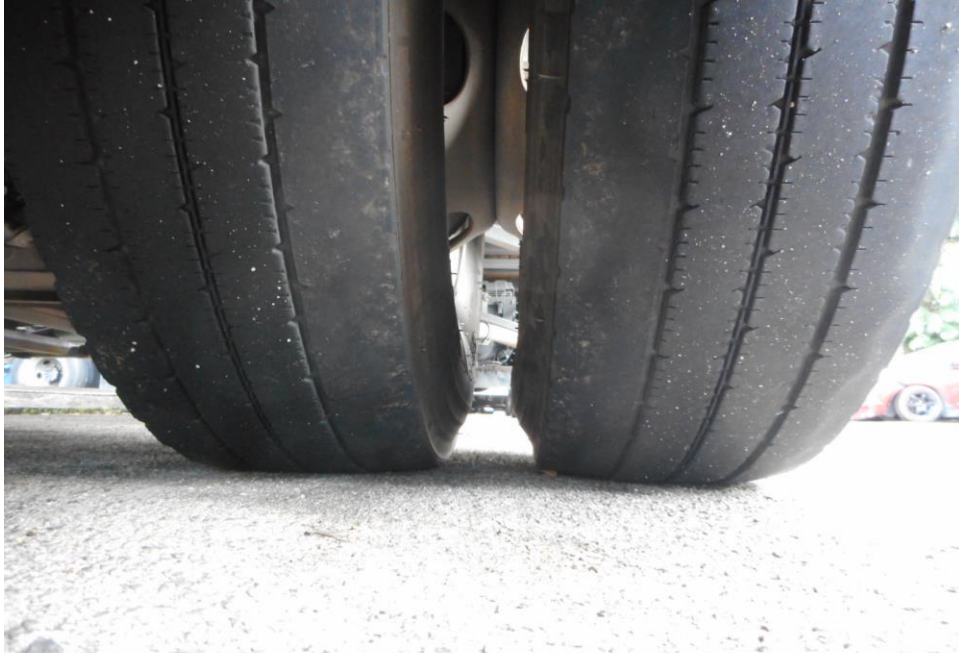
Photo 10 shows the condition of the rear right tyre of the Motor Lorry, which was observed to be in serviceable condition with remaining tread depth of approximately 3.5mm. The tyre, which was wrapped around standard steel wheel rim, it was observed to be sufficiently inflated for vehicular operation.
