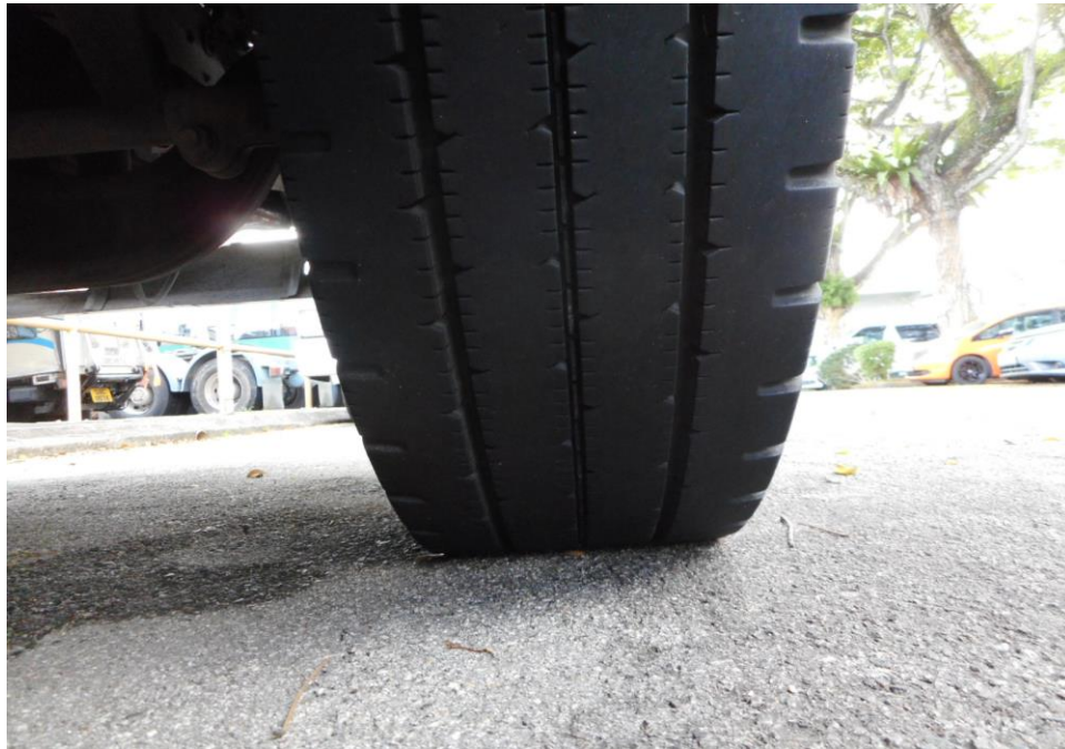
Photo 9 shows the condition of the front right tyre of the Motor Lorry, which was observed to be in serviceable condition with remaining tread depth of approximately 3mm. The tyre, which was wrapped around standard steel wheel rim, was also observed to be sufficiently inflated for vehicular operation. There was no tear, cut or burst mark(s) on the outer and the inner sidewalls as well as across the tread of the 6 tyres that were fitted on the Motor Lorry.
