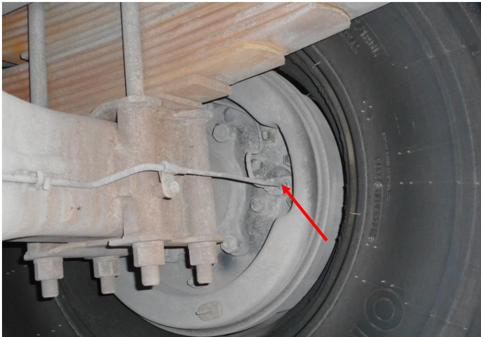
Photo 21 shows the brake pipe (arrowed) at the rear right wheel of the Motor Lorry. I did not observe any leakage of brake fluid at the time of my inspection of the Motor Lorry. My static tests of the Motor Lorry's braking system, along with my visual examination of the various mechanical components in the braking system, had indicated that there was no internal leakage of pressure/vacuum. Hence the braking system of the Motor Lorry was likely to be in serviceable condition at the material time of accident.
