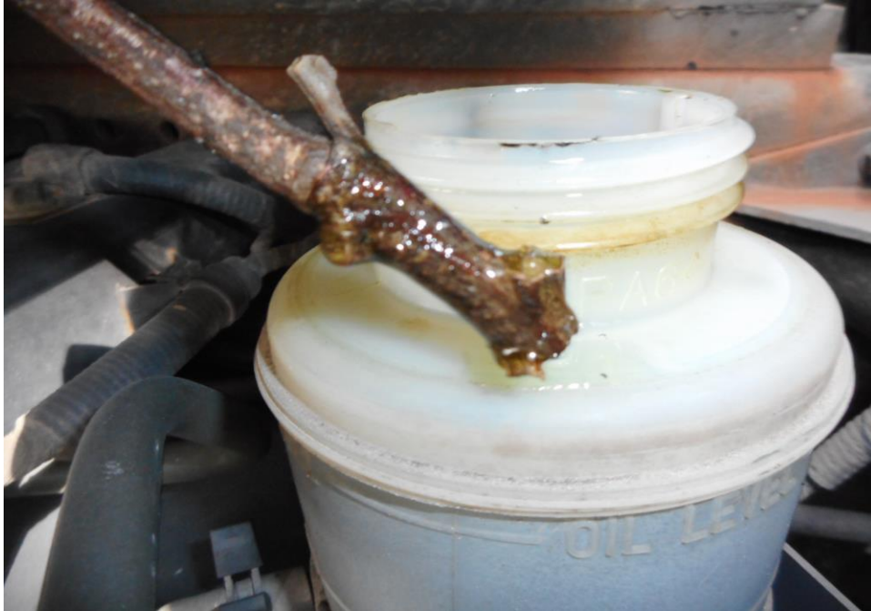
Photo 17 shows the power steering fluid reservoir of the Motor Lorry at the time of my inspection. The power steering fluid was observed to be of sufficient level (arrowed) and without any visible contamination.
