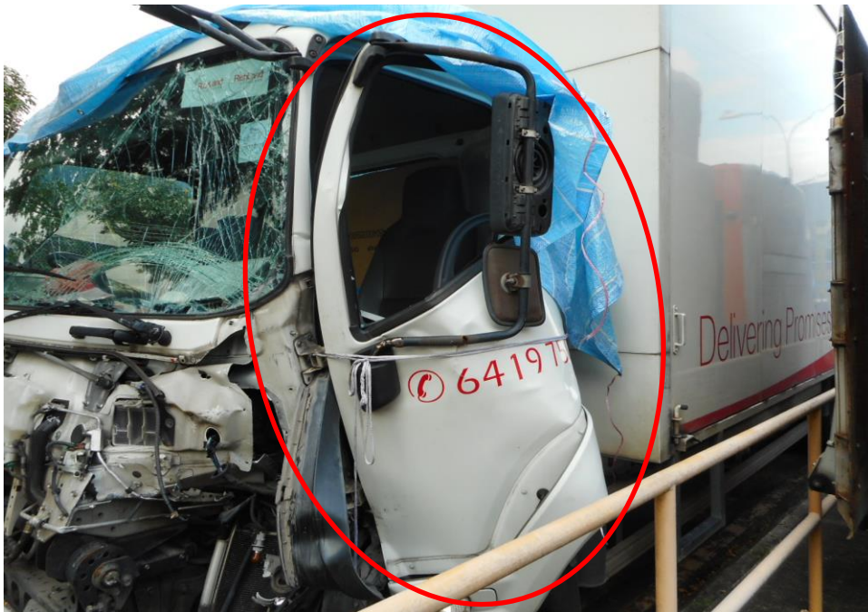
Photo 5 shows a close up view of the Motor Lorry's front portion at the time of my inspection. It appeared to have sustained damage at its front portion. Its front left door (circled) were damage at the time of my inspection.
