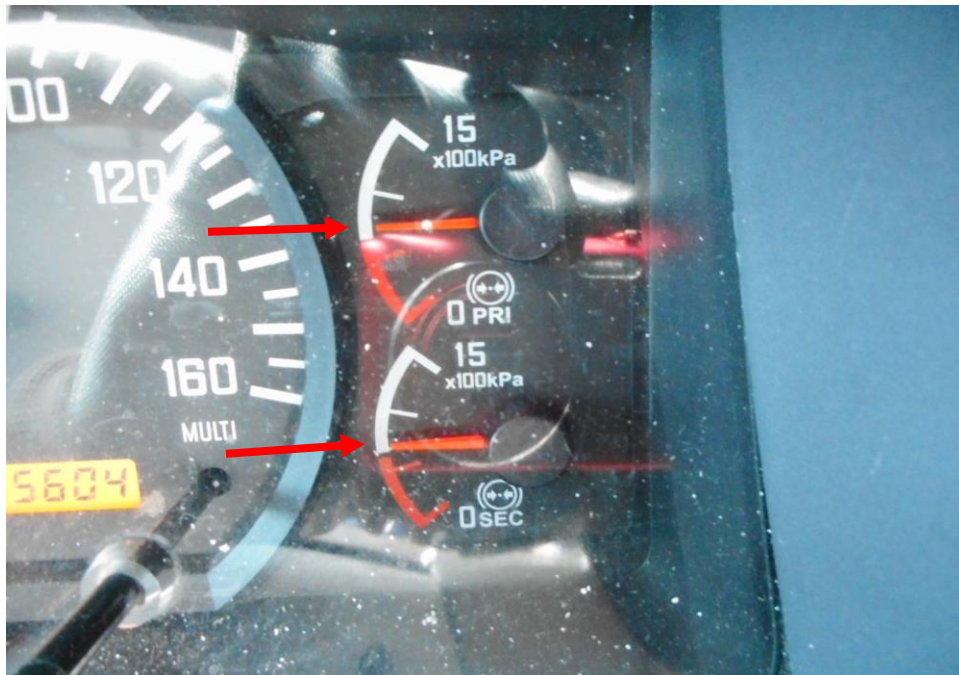
Photo 14 shows the air in the air brake cylinder of the Motor Lorry at the time of my inspection. The air in the cylinder was observed to be of sufficient level & serviceable at the time of the accident.
