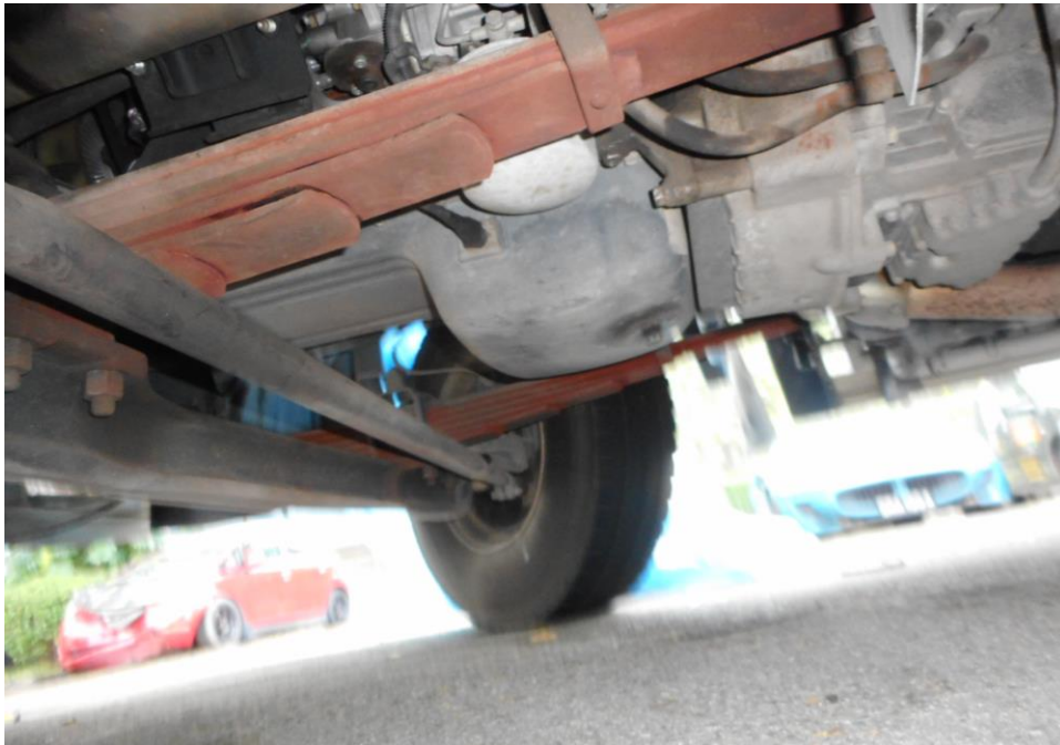
Photo 18 shows the undercarriage of the Motor Lorry, at the area where the engine housing and transmission housing are located. I did not find any sign(s) or indication(s) of fluid leak and/or fluid stain(s) on the underside of the Motor Lorry.
