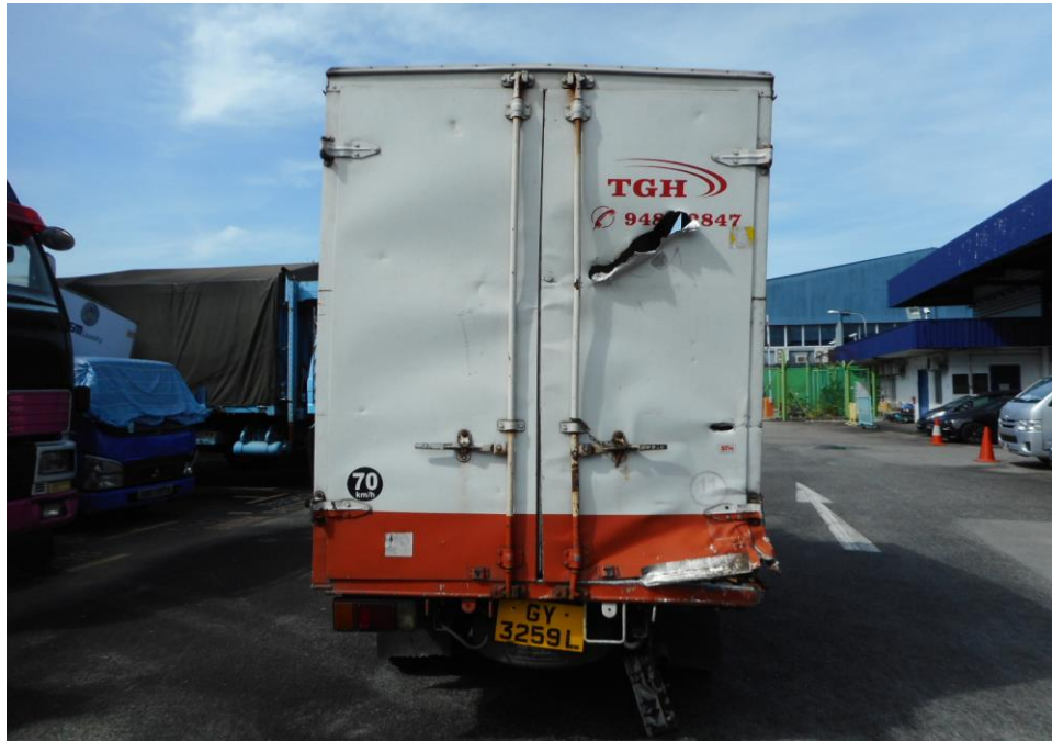
Photo 2 shows a general view of the rear body of the Motor Lorry at the time of my inspection. The Motor Lorry was observed to sustained damage at its front, right and rear portion. Its front windscreen, front body panel, front bumper, front right headlamp, right body panel, rear body panel and brake lamp were damage at the time of my inspection.
