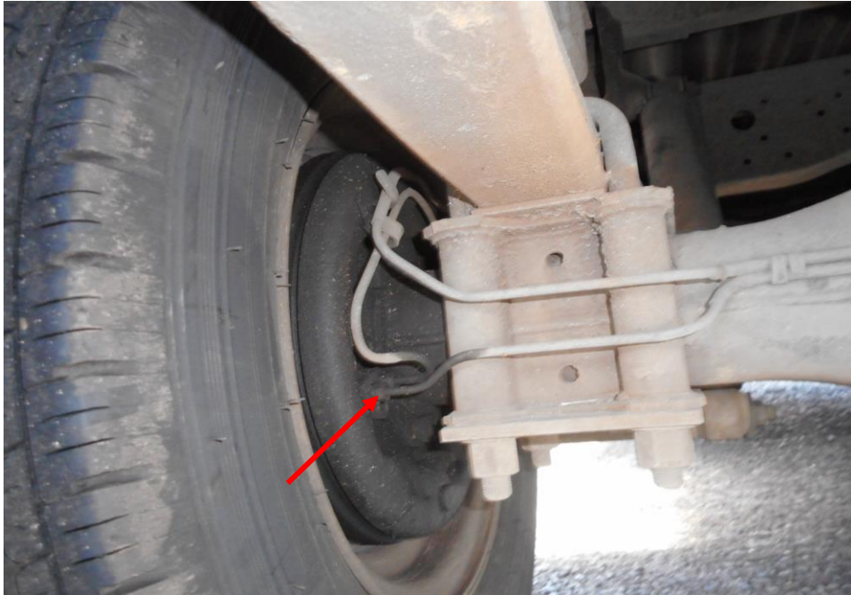
Photo 23 shows the brake pipe (arrowed) at the rear left wheel of the Motor Lorry. I did not observe any leakage of brake fluid at the time of my inspection of the Motor Lorry. My static tests of the Motor Lorry's braking system, along with my visual examination of the various mechanical components in the braking system had indicated that there was no internal leakage of pressure/vacuum. Hence the braking system of the Motor Lorry was likely to be in serviceable condition at the material time of accident.
