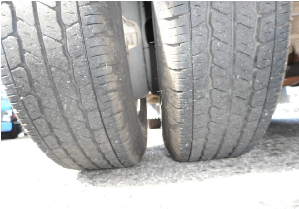
Photo 13 shows the condition of the rear left tyres of the Motor Lorry, which was observed to be in serviceable condition with remaining tread depth of approximately 2.6mm. The tyres, which were wrapped around standard steel wheel rim, were also observed to be sufficiently inflated for vehicular operation. There was also no damage found on all 6 steel wheel rims of the Motor Lorry.
