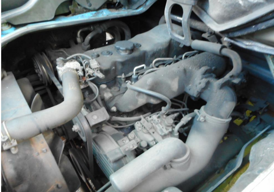
Photo 15 shows a general view of the Motor Lorry's engine compartment, which was accessed by lifting the front cabin of the Motor Lorry. The various parts and components inside the engine compartment were unaffected by the accident. There was also no sign(s) or indication(s) of fresh fluid leakage and/or fluid stain within the engine compartment
