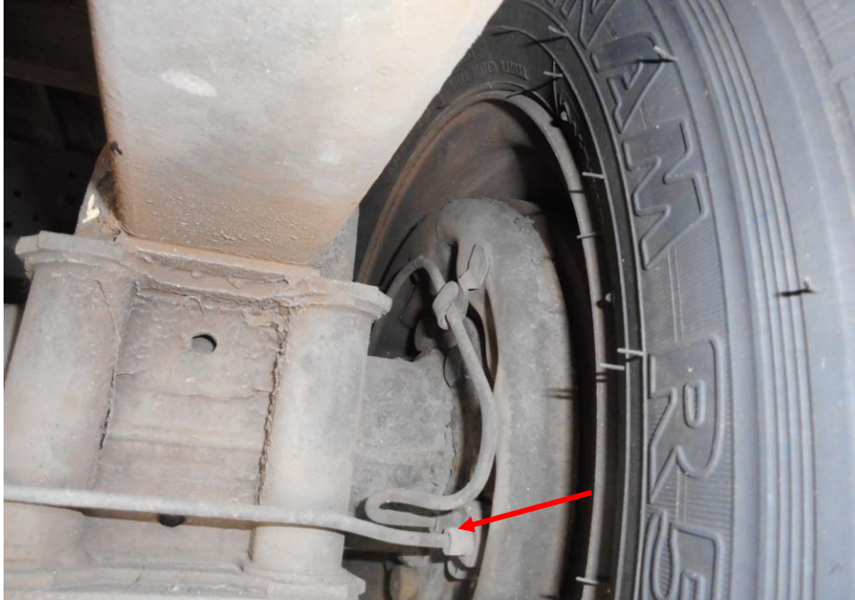
Photo 22 shows the brake pipe (arrowed) at the rear right wheel of the Motor Lorry. I did not observe any leakage of brake fluid at the time of my inspection of the Motor Lorry. My static tests of the Motor Lorry's braking system, along with my visual examination of the various mechanical components in the braking system, had indicated that there was no internal leakage of pressure/vacuum. Hence the braking system of the Motor Lorry was likely to be in serviceable condition at the material time of accident.
