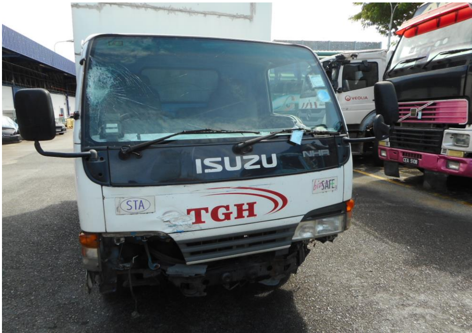
Photo 5 shows a general view of the front body of the Motor Lorry at the time of my inspection. Its front windscreen, front body panel, front bumper and front right headlamp were damage at the time of my inspection.
