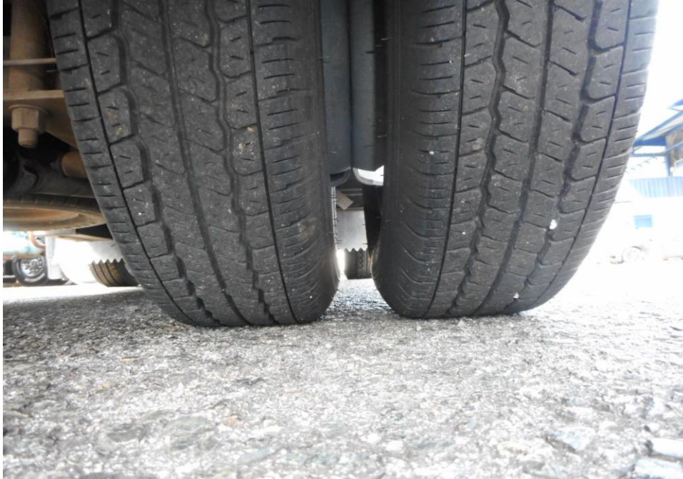
Photo 12 shows the condition of the rear right tyre of the Motor Lorry, which was observed to be in serviceable condition with remaining tread depth of approximately 2.5mm. The tyre, which was wrapped around standard steel wheel rim, it was observed to be sufficiently inflated for vehicular operation.
