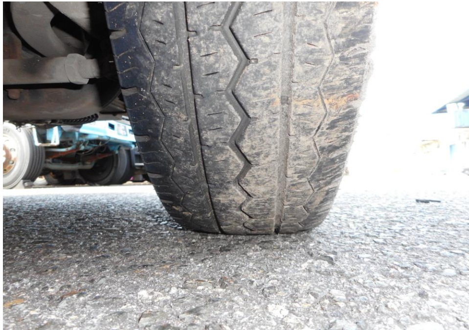
Photo 11 shows the condition of the front right tyre of the Motor Lorry, which was observed to be in serviceable condition with remaining tread depth of approximately 5.7mm. The tyre, which was wrapped around standard steel wheel rim, was also observed to be sufficiently inflated for vehicular operation. There was no tear, cut or burst mark(s) on the outer and the inner sidewalls as well as across the tread of the 6 tyres that were fitted on the Motor Lorry.
