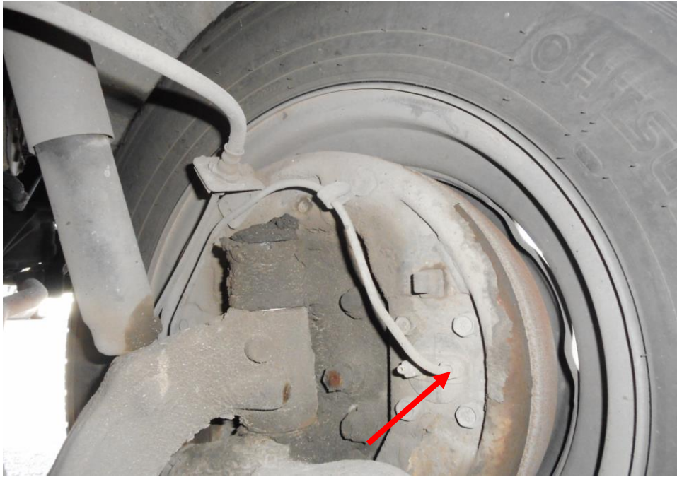
Photo 24 shows the brake hose/pipe (arrowed) at the front right wheel of the Motor Lorry. No leakage of brake fluid was observed. Visual examination of the various components of the braking system like the brake drum, brake booster, brake pedal etc had revealed all to be intact and without visible damage at the time of accident. There was also no sign of fluid stain(s) observed on the various undercarriage components.
