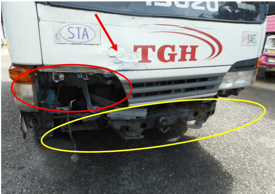
Photo 7 shows a close up view of the Motor Lorry's frontal portion at the time of my inspection. Its front body panel (arrowed) front bumper (yellow circled) and front right headlamp (red circled) were damage at the time of my inspection as the result of the accident.
