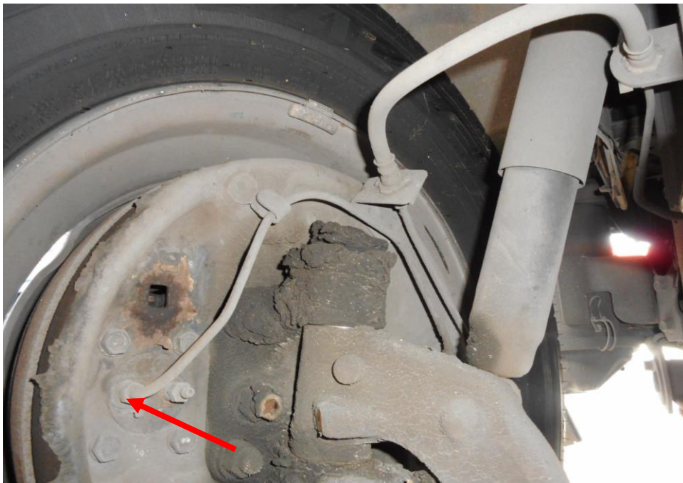
Photo 25 shows the brake hose/pipe (arrowed) at the front left wheel of the Motor Lorry. No leakage of brake fluid was observed. Visual examination of the various components of the braking system like the brake drum, brake booster, brake pedal etc had revealed all to be intact and without visible damage at the time of accident. There was also no sign of fluid stain(s) observed on the various undercarriage components.
