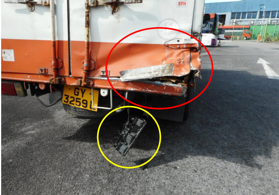
Photo 4 shows a close up view of the rear body of the Motor Lorry at the time of my inspection. Its rear body panel (red circle) and brake lamp (yellow circle) were damage at the time of my inspection.
