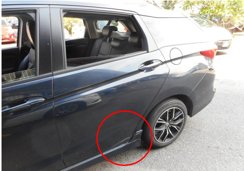
Photo 4 shows the close up view of the Motor Car's left body at the time of my inspection. The Motor Car was observed to have sustained damage at its left rear door (circled) as a result of the accident.
