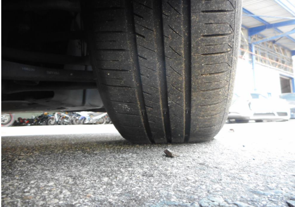
Photo 8 shows the condition of the front right tyre of the Motor Car, which was observed to be in serviceable condition with remaining tread depth of approximately 5.3mm. The tyre was sufficiently inflated for vehicular operation with no tear, cut or burst mark(s) on the outer and the inner sidewalls as well as across the tread. The 4 tyres of the Motor Car were wrapped around standard steel wheel rims without any damage.
