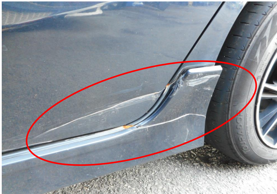
Photo 5 shows the close up view of the Motor Car's left body at the time of my inspection. The Motor Car was observed to have sustained damage at its left rear door (circled) as a result of the accident.
