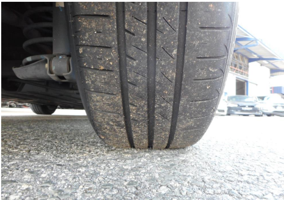
Photo 9 shows the condition of the rear right tyre of the Motor Car, which was observed to be in serviceable condition with remaining tread depth of approximately 4.2mm. The tyre was also observed to be sufficiently inflated for vehicular operation with no tear, cut or burst mark(s).
