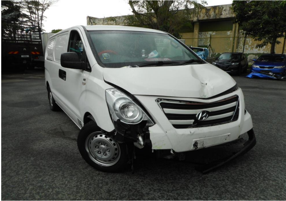
Photo 6 shows a general view of the right body of the Motor Van at the time of my inspection. The Motor Van was observed to be intact and unaffected by the accident.
