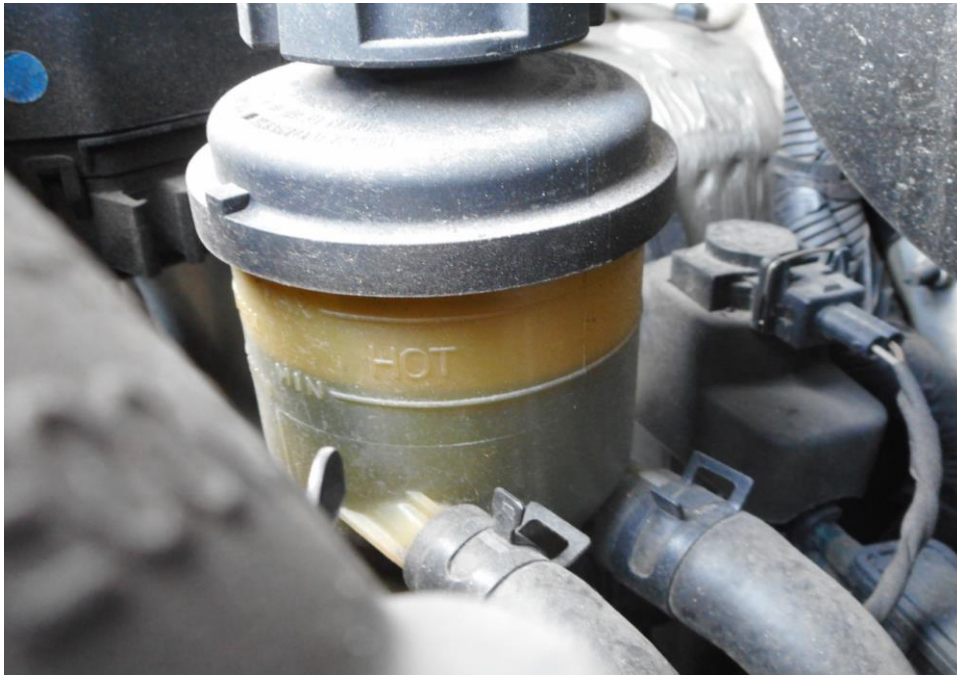
Photo 16 shows the power steering fluid reservoir of the Motor Van at the time of my inspection. The power steering fluid was observed to be of sufficient level (arrowed) and without any visible contamination.
