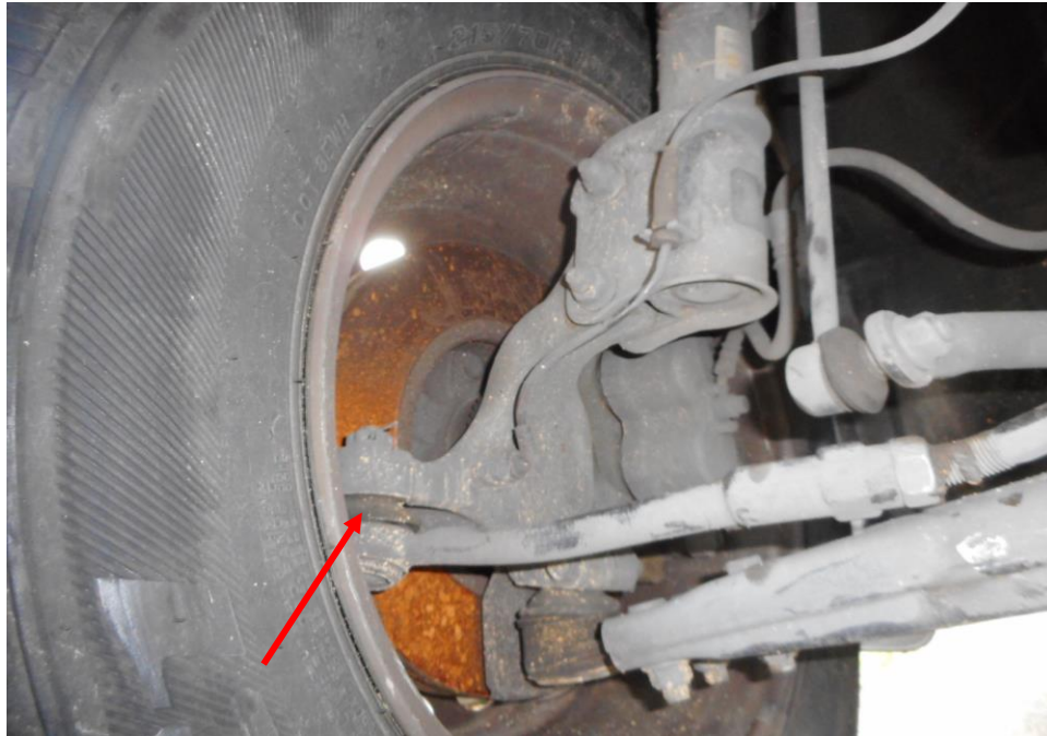
Photo 18 shows the various undercarriage components at the front right wheel of the Motor Van, in particular the steering tie rod end (arrowed). The various steering components were all found to be intact, suggesting that the steering system of the Motor Van was likely to be in serviceable condition at the material time of accident. There was also no sign of fluid stain(s) observed on the various undercarriage components.
