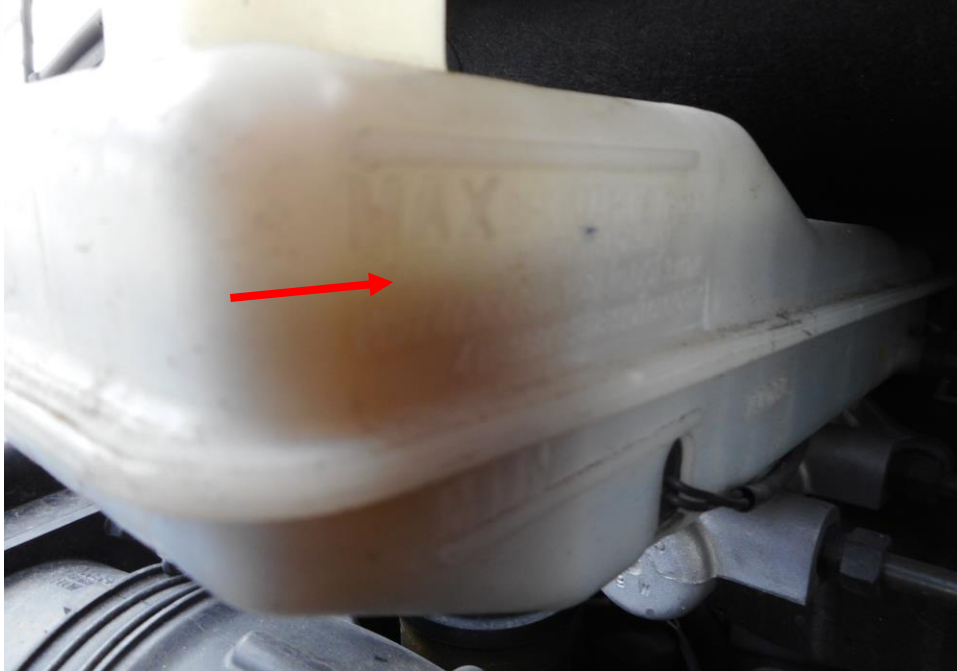
Photo 13 shows the brake fluid reservoir of the Motor Van at the time of my inspection. The brake fluid was observed to be of sufficient level (arrowed) and without any visible contamination.
