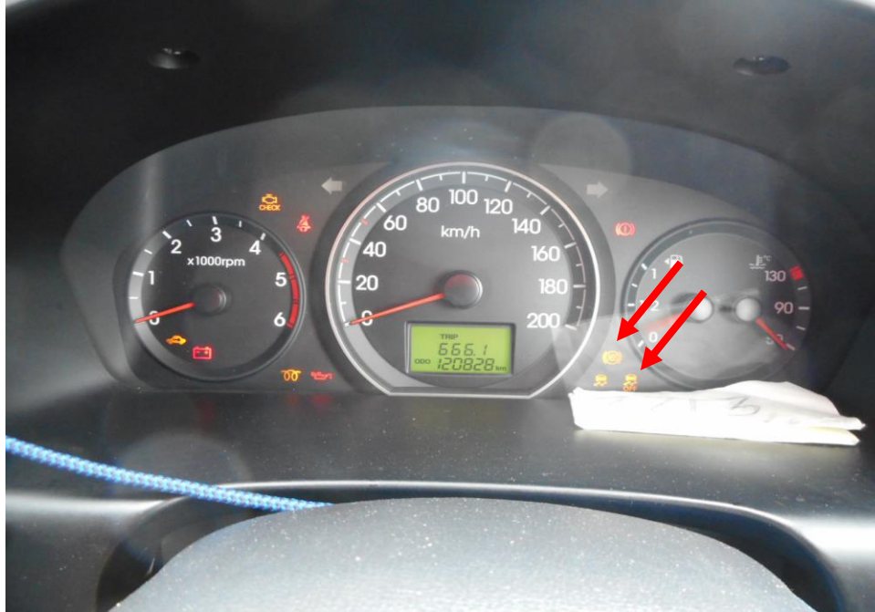
Photo 25 shows the warning light for Anti-Lock Brake System (ABS) and Traction Control System (TCS) (arrowed) appearing on the instrument panel of the Motor Van during the self-test of its various electronic operating systems when its engine was cranked.
