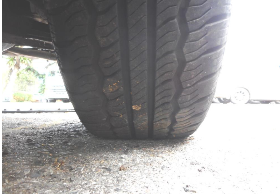
Photo 8 shows the condition of the front right tyre of the Motor Van, which was observed to be in serviceable condition with remaining tread depth of approximately 5.9mm. The tyre, which was wrapped around standard steel wheel rim, was also observed to be sufficiently inflated for vehicular operation. There was no tear, cut or burst mark(s) on the outer and the inner sidewalls as well as across the tread of the 4 tyres that were fitted on the Motor Van.
