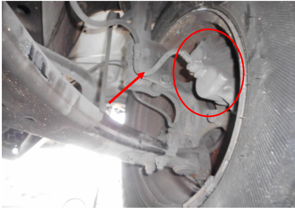
Photo 22 shows the brake hose/pipe (arrowed) at the front right wheel of the Motor Van. No leakage of brake fluid was observed. Visual examination of the various components of the braking system like the brake caliper (circled), brake booster, brake pedal etc had revealed all to be intact and without visible damage at the time of accident. There was also no sign of fluid stain(s) observed on the various undercarriage components.
