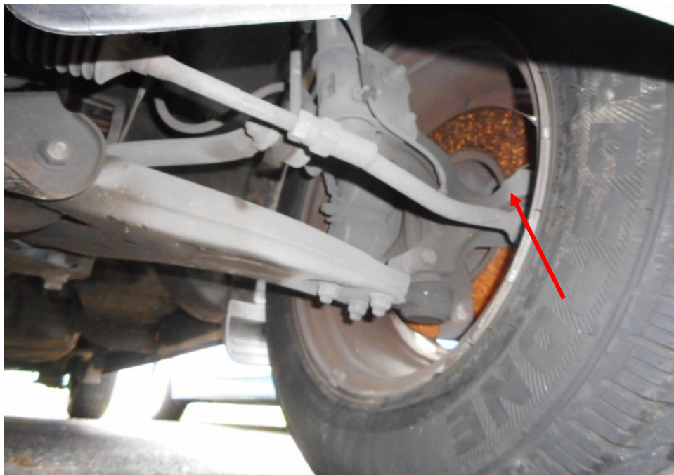
Photo 19 shows the various undercarriage components at the front left wheel of the Motor Van, in particular the steering tie rod end (arrowed). The various undercarriage components of the Motor Van were all found to be intact without any visible damage. There was also no sign of fluid stain(s) observed on the various undercarriage components.
