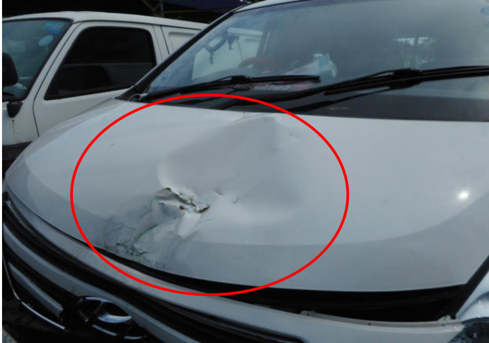
Photo 4 shows a close up view of the Motor Van's front portion at the time of my inspection. Its front bonnet (red circle) was damage at the time of my inspection as a result of the accident.
