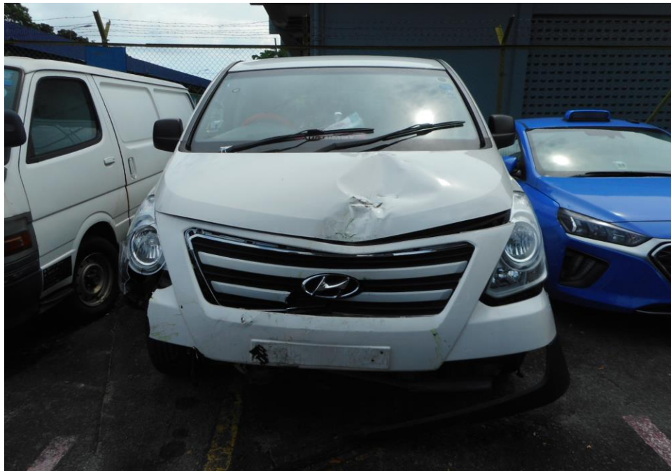
Photo 3 shows a general view of the Motor Van's frontal portion at the time of my inspection. It appeared to have sustained damage at its front portion. Its front bonnet, front right headlamp, front bumper and its various engine components were damage at the time of my inspection.
