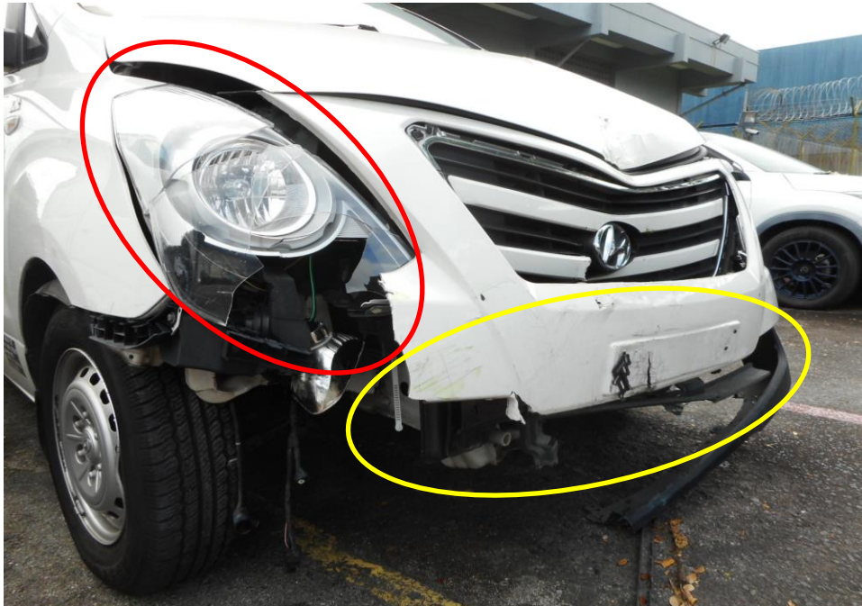
Photo 5 shows a close up view of the Motor Van's front portion at the time of my inspection. Its front right headlamp (red circle) and front bumper (yellow circle) was damage at the time of my inspection as a result of the accident.
