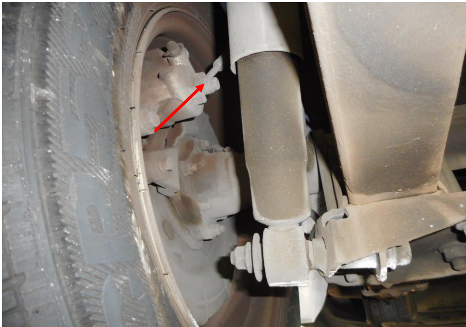
Photo 21 shows the brake pipe (arrowed) at the rear left wheel of the Motor Van. I did not observe any leakage of brake fluid at the time of my inspection of the Motor Van. My static tests of the Motor Van's braking system, along with my visual examination of the various mechanical components in the braking system had indicated that there was no internal leakage of pressure/vacuum. Hence the braking system of the Motor Van was likely to be in serviceable condition at the material time of accident.
