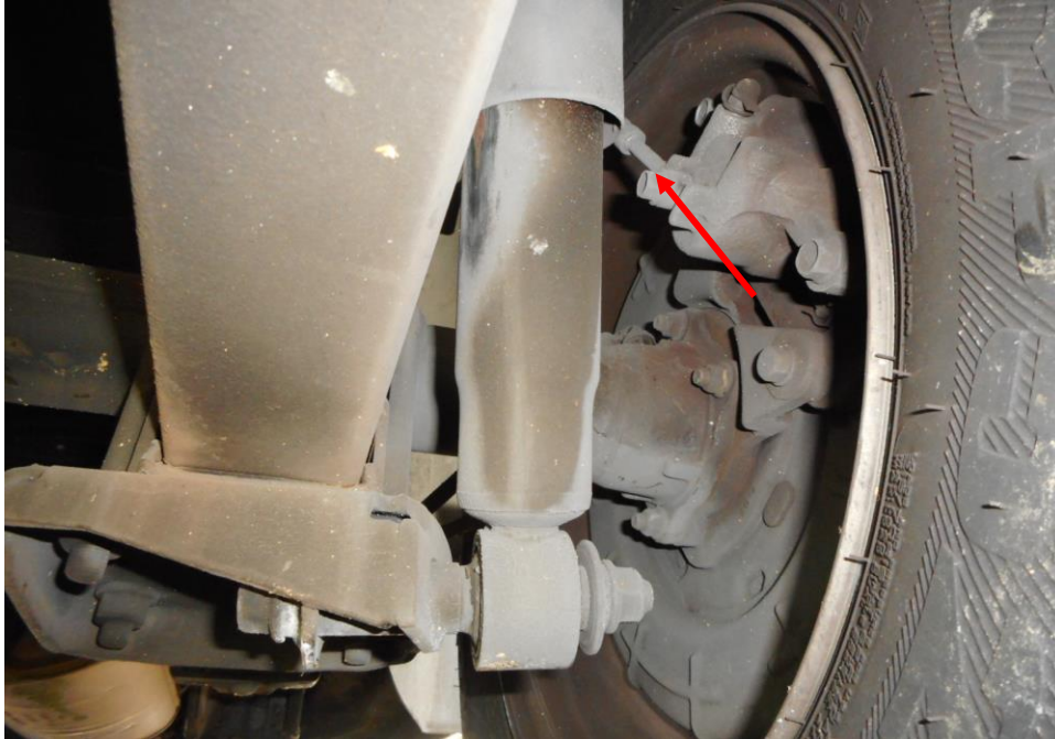
Photo 20 shows the brake pipe (arrowed) at the rear right wheel of the Motor Van. I did not observe any leakage of brake fluid at the time of my inspection of the Motor Van. My static tests of the Motor Van's braking system, along with my visual examination of the various mechanical components in the braking system, had indicated that there was no internal leakage of pressure/vacuum. Hence the braking system of the Motor Van was likely to be in serviceable condition at the material time of accident.
