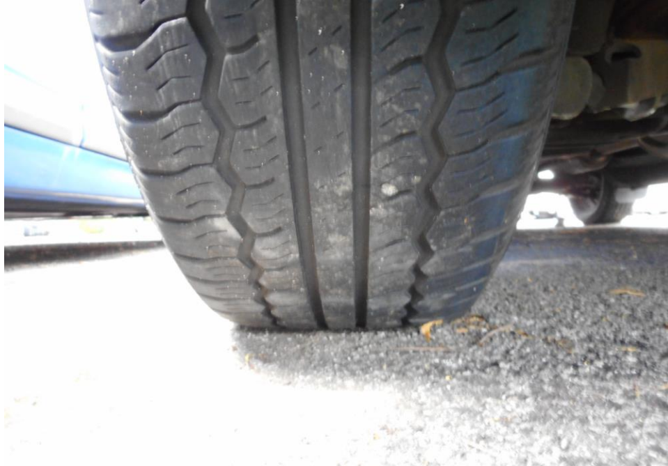
Photo 10 shows the condition of the rear left tyres of the Motor Van, which was observed to be in serviceable condition with remaining tread depth of approximately 4.4mm. The tyres, which were wrapped around standard steel wheel rim, were also observed to be sufficiently inflated for vehicular operation. There was also no damage found on all 4 steel wheel rims of the Motor Van.
