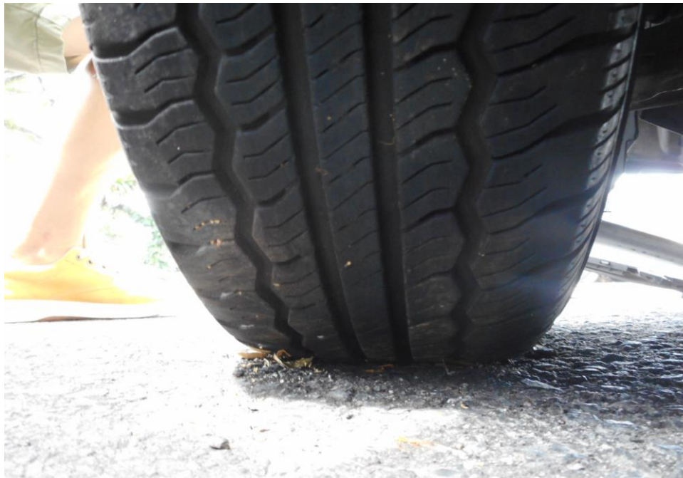
Photo 11 shows the condition of the rear right tyres of the Motor Van, which were observed to be in serviceable condition with remaining tread depth of approximately 6mm. There was also no tear, cut or burst mark(s) on the outer and the inner sidewalls as well as across the tread of the 4 tyres that were fitted on the Motor Van.
