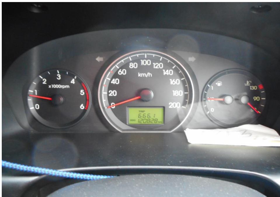
Photo 26 shows no warning lights illuminated on the instrument panel of the Motor Van after the engine was cranked. This would suggest that there was no abnormality to the electronic operating system of the Motor Van, like the ABS, and TCS etc.
