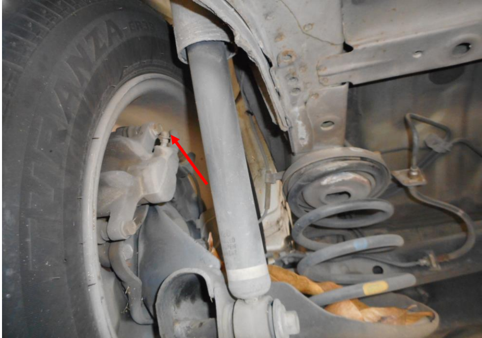
Photo 20 shows the brake pipe (arrowed) at the rear left wheel of the Motor Car. I did not observe any leakage of brake fluid at the time of my inspection of the Motor Car. My static tests of the Motor Car's braking system, along with my visual examination of the various mechanical components in the braking system had indicated that there was no internal leakage of pressure/vacuum. Hence the braking system of the Motor Car was likely to be in serviceable condition at the material time of accident.
