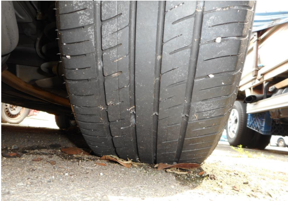
Photo 7 shows the condition of the rear tyre of the Motor Car, which was observed to be in serviceable condition with remaining tread depth of approximately 4.6mm. The tyre, which was wrapped around standard alloy wheel rim, was also observed to be sufficiently inflated for vehicular operation. There was no tear, cut or burst mark(s) on the outer and the inner sidewalls as well as across the tread of the 4 tyres that were fitted on the Motor Car.
