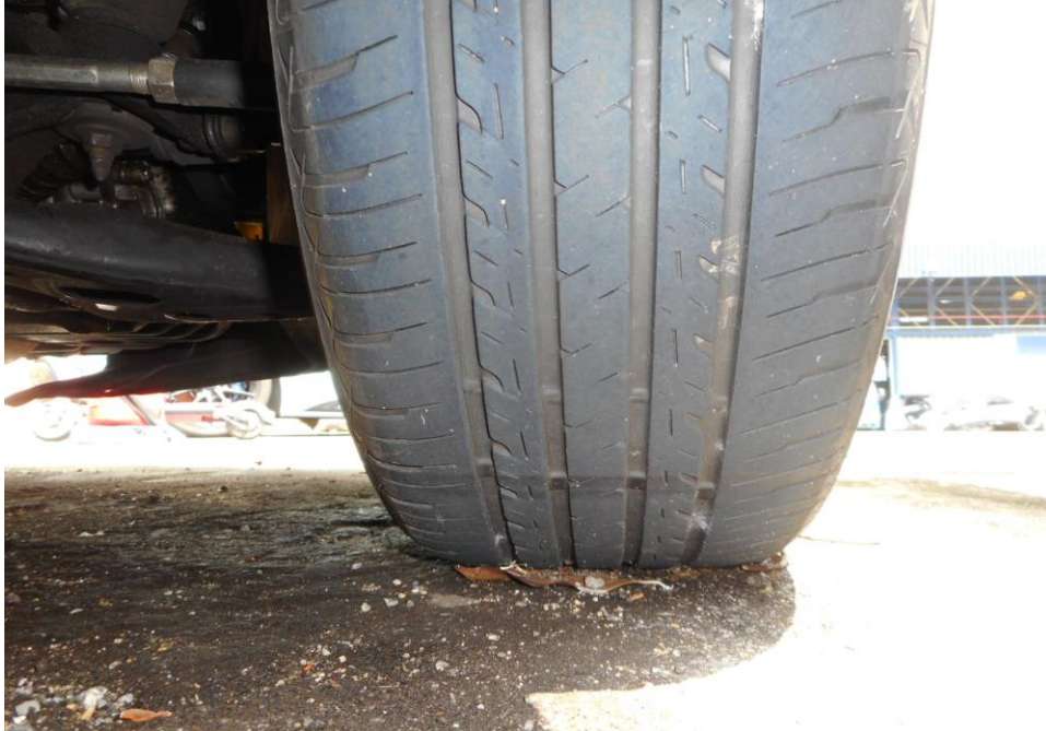
Photo 6 shows the condition of the front right tyre of the Motor Car, which was observed to be in serviceable condition with remaining tread depth of approximately 3.1mm. The tyre, which was wrapped around standard alloy wheel rim, was also observed to be sufficiently inflated for vehicular operation. There was no tear, cut or burst mark(s) on the outer and the inner sidewalls as well as across the tread of the 4 tyres that were fitted on the Motor Car.
