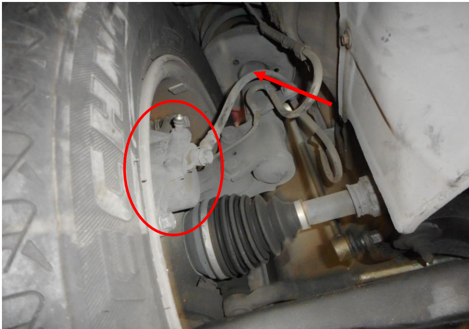
Photo 21 shows the brake hose/pipe (arrowed) at the front right wheel of the Motor Car. No leakage of brake fluid was observed. Visual examination of the various components of the braking system like the brake caliper (circled), brake booster, brake pedal etc had revealed all to be intact and without visible damage at the time of accident. There was also no sign of fluid stain(s) observed on the various undercarriage components.
