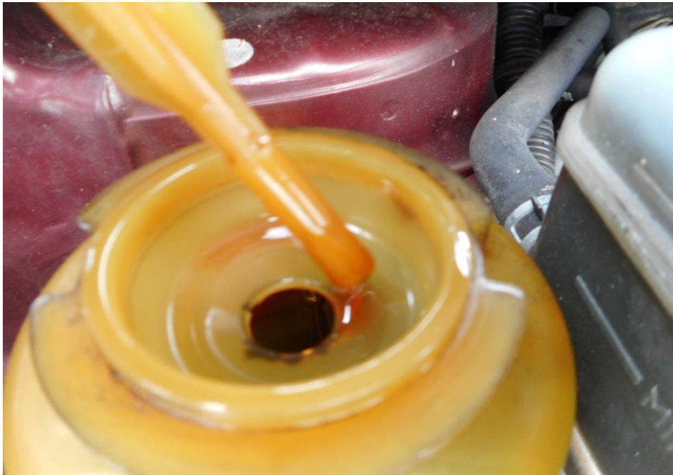
Photo 13 shows the power steering fluid dip stick of the Motor Car at the time of my inspection. The steering fluid was observed to be of sufficient level and without any visible contamination.
