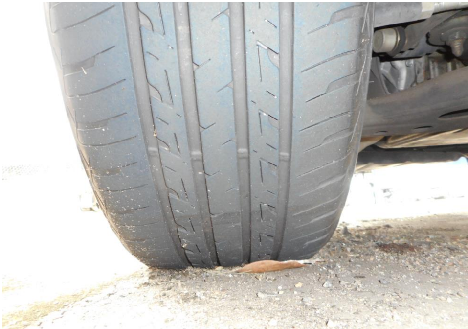
Photo 9 shows the condition of the rear right tyres of the Motor Car, which were observed to be in serviceable condition with remaining, tread depth of approximately 3.7mm. There was also no tear, cut or burst mark(s) on the outer and the inner sidewalls as well as across the tread of the 4 tyres that were fitted on the Motor Car.
