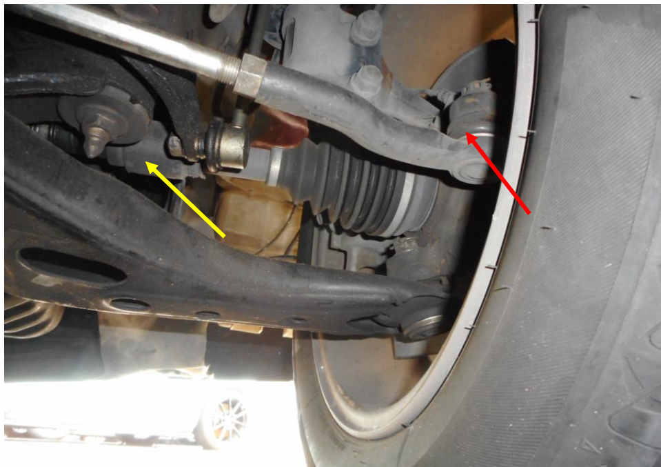
Photo 17 shows the various undercarriage components at the front right wheel of the Motor Car, in particular the steering tie rod end (red arrow) and drive shaft (yellow arrow). The various steering components were all found to be intact, suggesting that the steering system of the Motor Car was likely to be in serviceable condition at the material time of accident. There was also no sign of fluid stain(s) observed on the various undercarriage components.
