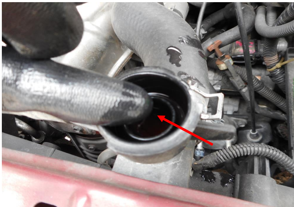
Photo 12 shows the engine coolant reservoir of the Motor Car at the time of my inspection. The engine coolant was observed to be of sufficient level (arrowed) and without any visible contamination.
