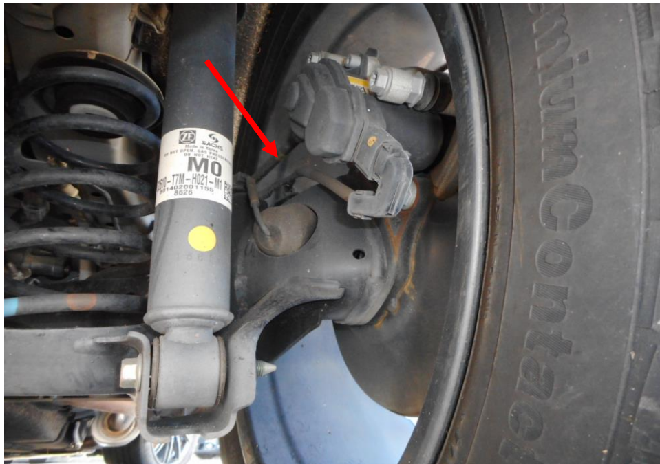
Photo 17 shows the brake hose/pipe (arrowed) at the rear right wheel of the Motor Car. No leakage of brake fluid was observed. Visual examination of the various components of the braking system like the drum brake, brake booster, brake pedal etc. had revealed all to be intact and without visible damage.
