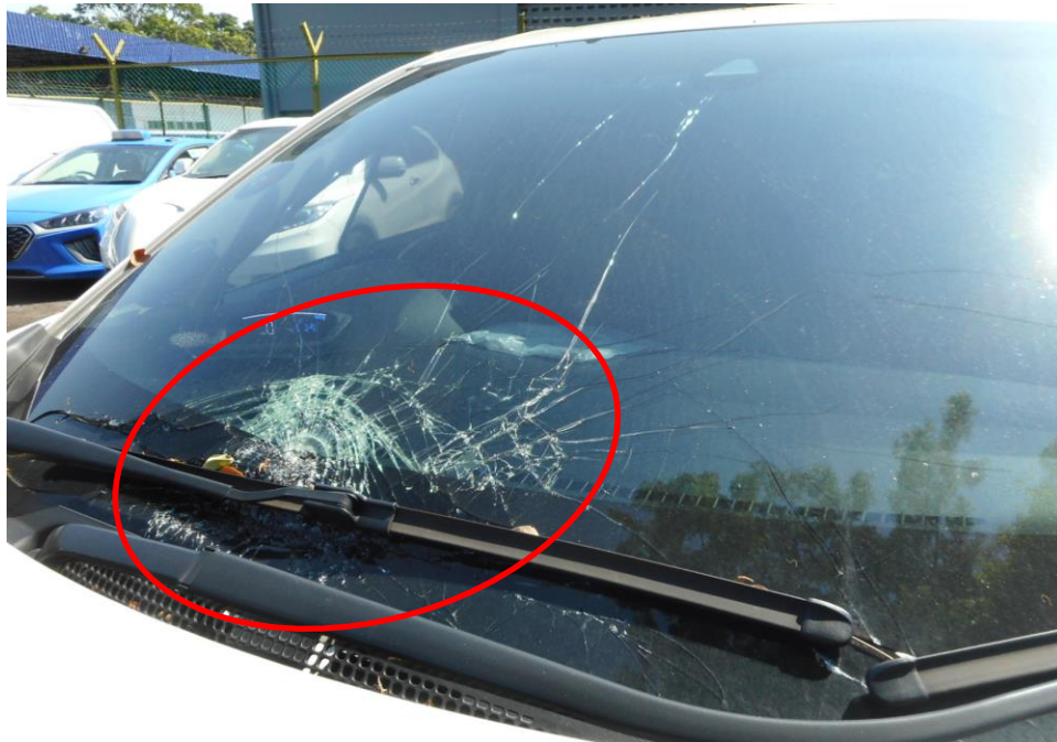
Photo 3 shows the close up view of the Motor Car's front body at the time of my inspection. The Motor Car was observed to have sustained damage at its front windscreen (circled) as a result of the accident.
