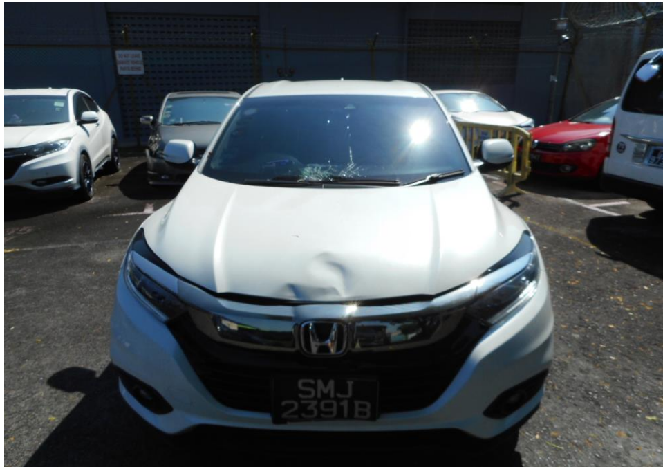
Photo 2 shows a general view of the Motor Car's front body at the time of my inspection. The front portion of the Motor Car was observed to have sustained damage. Its front windscreen and front bonnet was the body parts that were damaged as a result of the accident.
