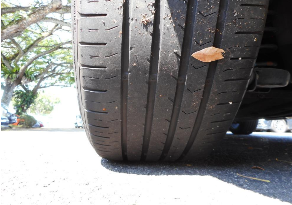
Photo 10 shows the condition of the rear left tyre of the Motor Car, which was observed to be in serviceable condition with remaining tread depth of approximately 3.7mm. The tyre, which was wrapped around steel wheel rim, was also observed to be sufficiently inflated for vehicular operation. The 4 tyres of the Motor Car were wrapped around standard steel wheel rims.
