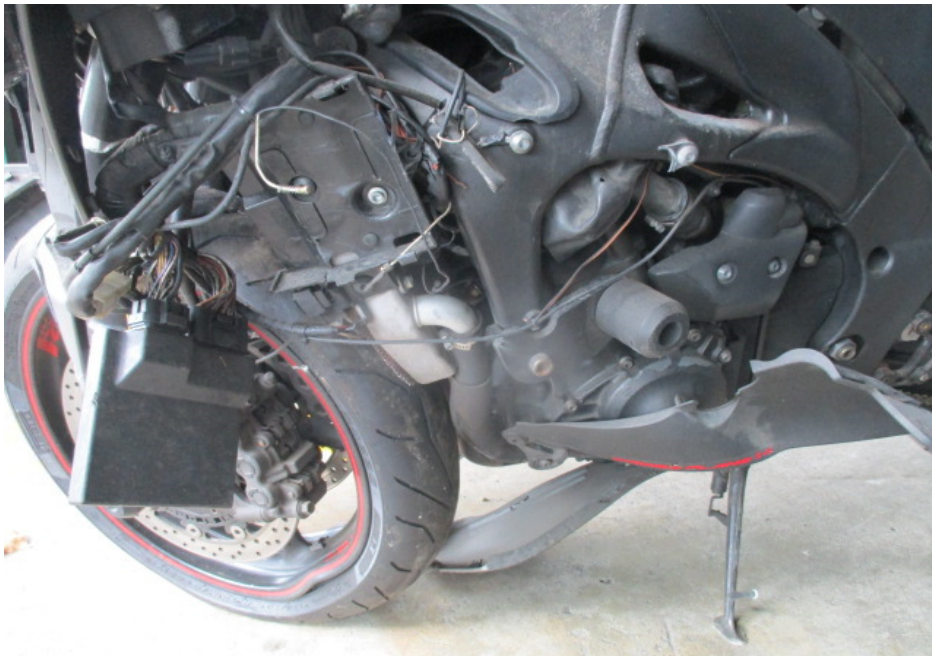
Photo 8 shows a closer view of the missing left cowling of the Motorcycle as a result of the accident.
