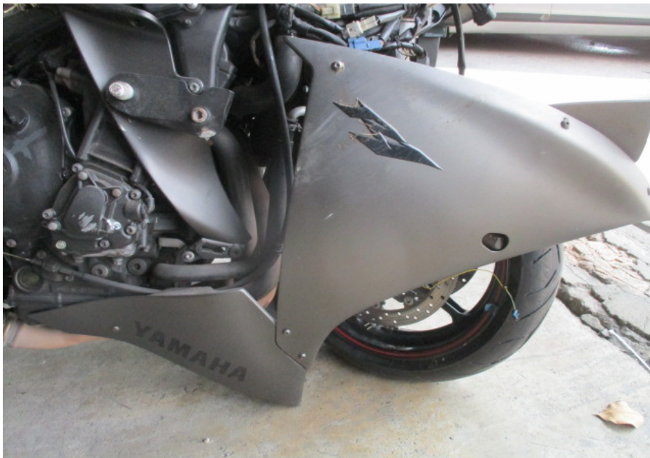
Photo 12 shows a closer view of the broken right cowling of the Motorcycle as a result of the accident.
