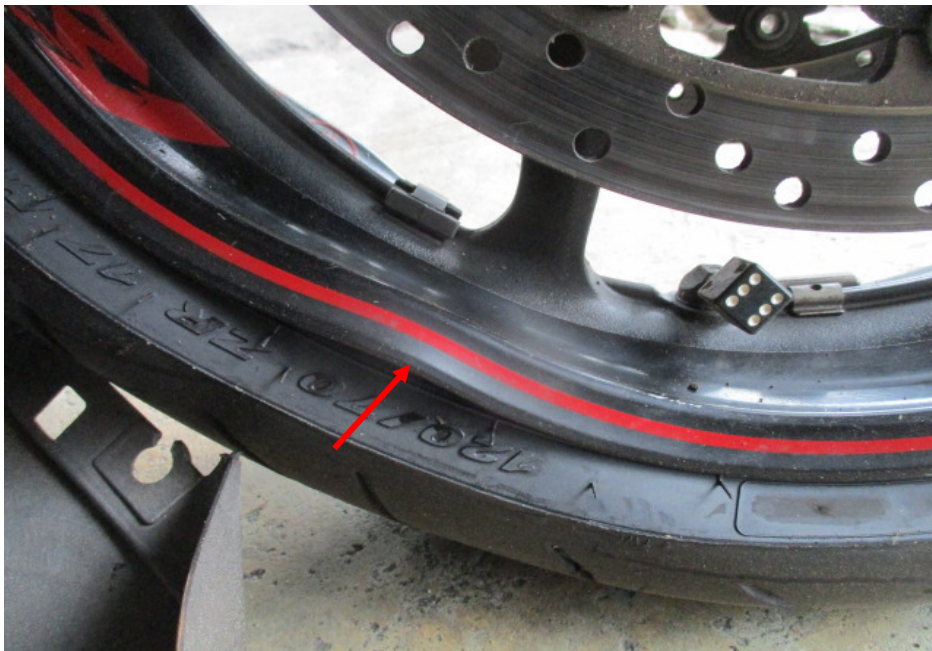
Photo 22 shows a close up view of the bent front wheel rim of the Motorcycle at the time of our inspection (arrowed).
