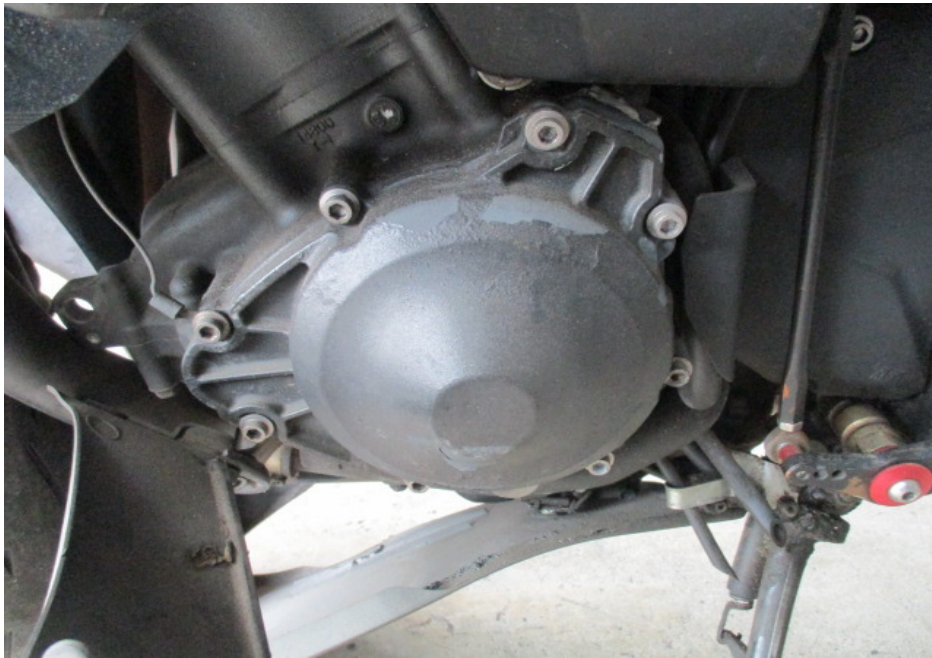
Photo 23 shows the left side of the engine of the Motorcycle at the time of our inspection. The various engine related parts and components were found to be intact with no visible damage. There was also no sign(s) or indication(s) of fluid leak observed around the left engine area of the Motorcycle.
