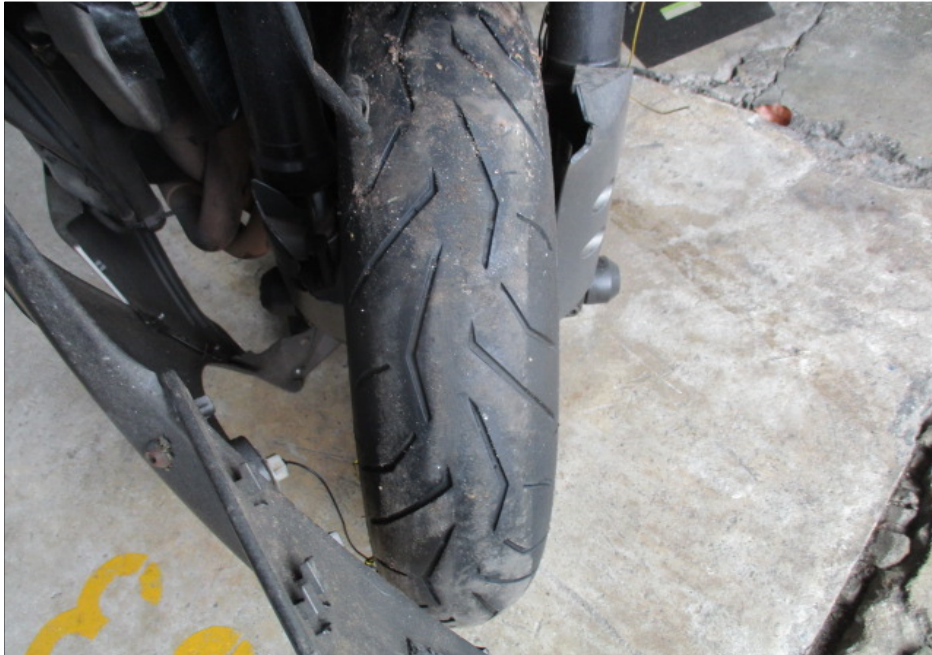
Photo 19 shows the condition of the Motorcycle's front tyre. The front tyre was observed to be in serviceable condition with remaining tread depth of approximately 4mm. We did not observe any tear, burst mark(s) and/or punctured hole(s) on the sidewalls as well as across the tread of the front tyre. However the front tyre was observed to be deflated.
