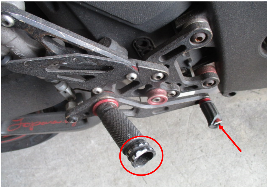
Photo 14 shows a closer view of the right front footrest (circled) and rear brake pedal (arrowed) which were amongst the body parts of the Motorcycle that had sustained damage as a result of the accident.
