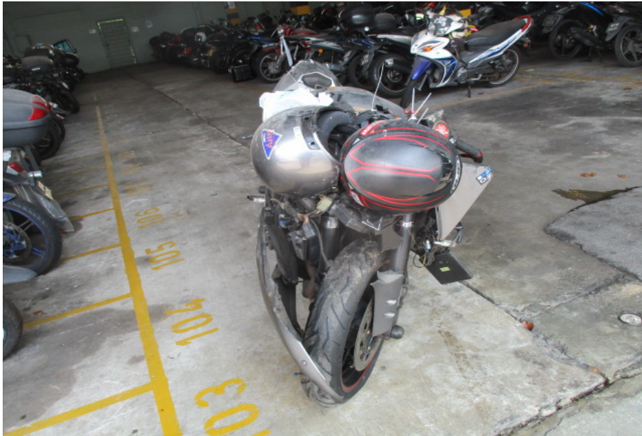
Photo 5 shows a general view of the frontal portion of the Motorcycle at the time of our inspection. The Motorcycle had sustained damages all around. Body parts that were found to have been damaged include its headlight assembly, front mudguard, front fork assembly, front wheel rim, front brake lever, front brake lever guard, clutch lever, clutch lever guard, petrol tank, side cowlings, right rear frame slider, rear brake pedal, right front footrest, right swingarm spool, rear side covers, tail light cover, rear seat cowl, pillion foot peg brackets and pillion foot pegs, amongst others.
