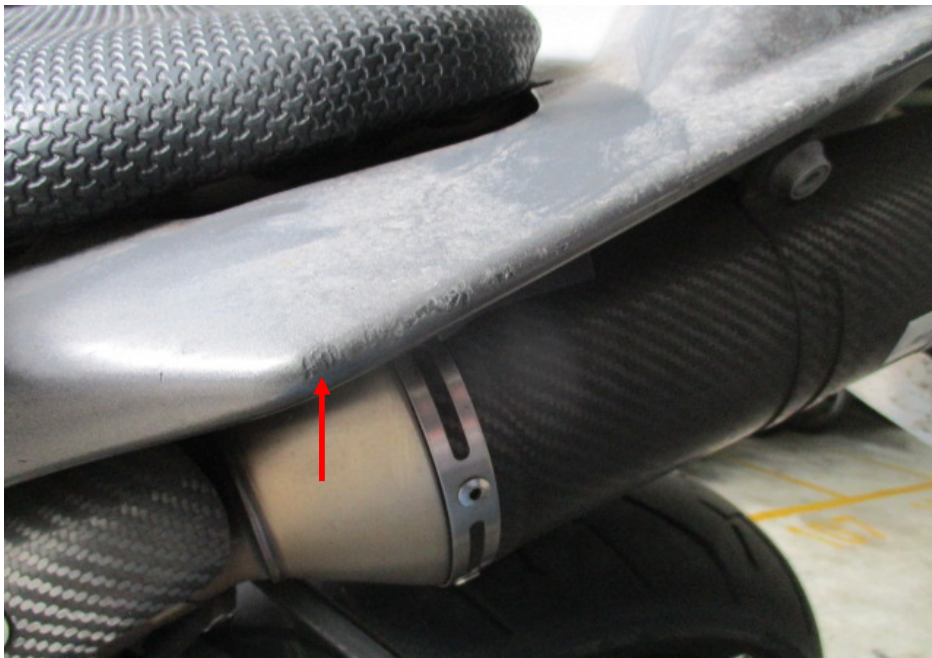
Photo 18 shows the grazed left rear side cover (arrowed) of the Motorcycle as a result of the accident.
