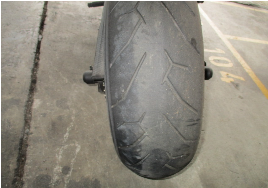
Photo 20 shows the condition of the Motorcycle's rear tyre. The rear tyre was observed to be in serviceable condition with remaining tread depth of approximately 3mm. The tyre was also observed to be sufficiently inflated for vehicular operation. We did not observe any tear, burst mark(s) and/or punctured hole(s) on the sidewalls as well as across the tread of the rear tyre.
