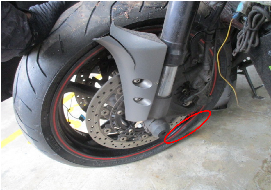
Photo 21 shows the bent front wheel rim of the Motorcycle at the time of our inspection (circled).
