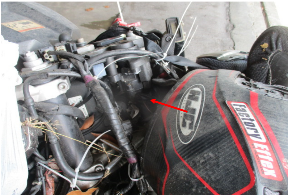
Photo 6 shows a closer view of the missing headlight assembly which was amongst the body parts at the front body of the Motorcycle that had sustained damage as a result of the accident (arrowed).
