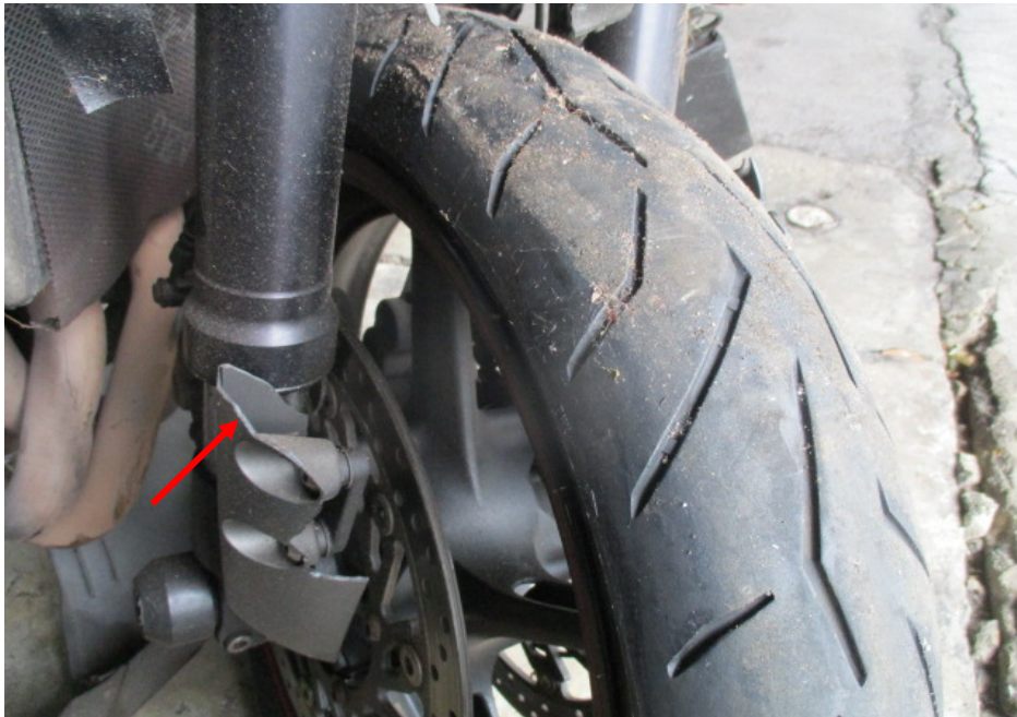
Photo 7 shows a closer view of the cracked front mudguard (arrowed) which was amongst the body parts at the front body of the Motorcycle that had sustained damage as a result of the accident.
