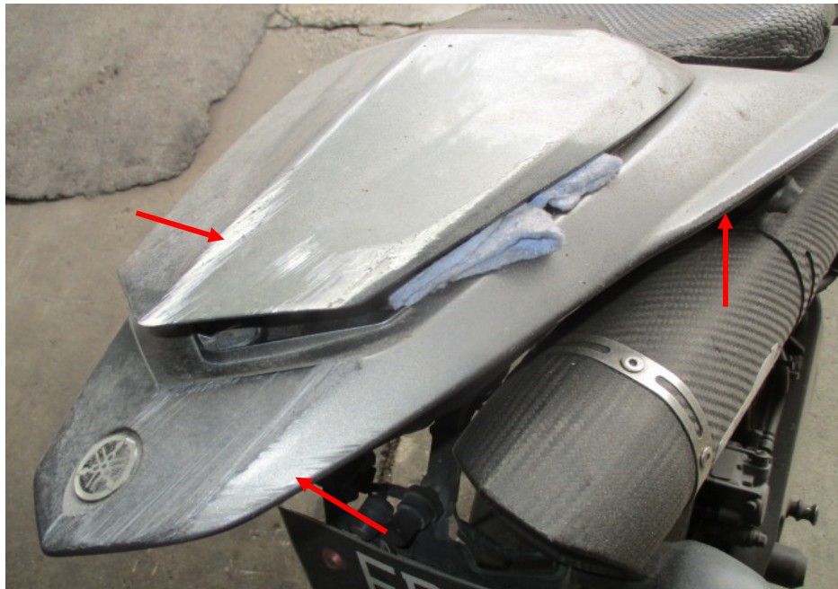
Photo 16 shows the grazed tail light cowl, right rear side cover and rear seat cowl (arrowed) of the Motorcycle as a result of the accident.
