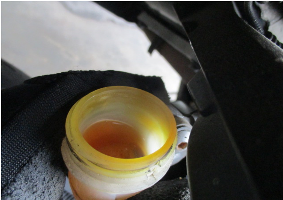
Photo 33 shows the brake fluid reservoir for the rear brake of the Motorcycle. The brake fluid was observed to be of sufficient level and without contamination for operational purposes.
