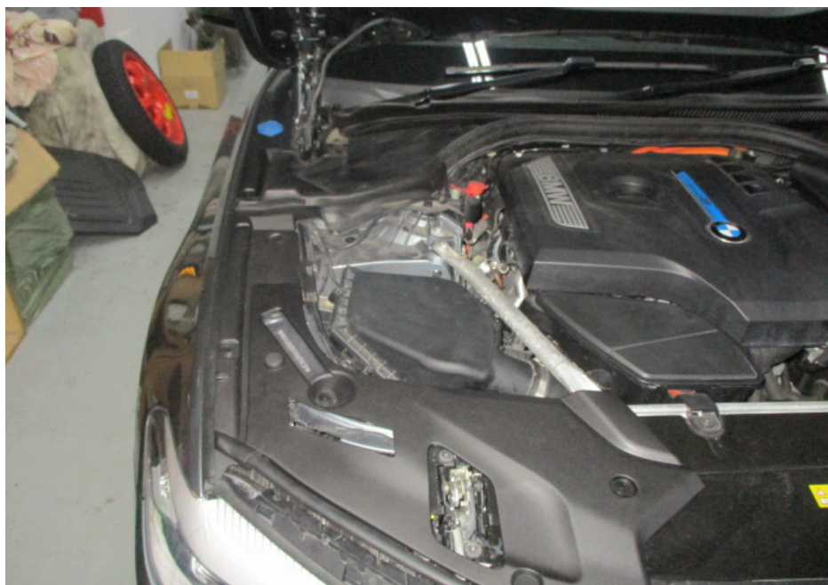
Photo 14 shows a closer view of the right side of the Motor Car's engine compartment. The panel and garnishes at the right side were visually examined and it was observed that the repair/restoration works carried out to the damaged area of the Motor Car (refer to photograph 5 above) were reasonably adequate and in order.
