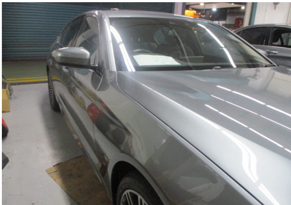
Photo 9 shows a closer view of the front bonnet and front right fender of the Motor Car. The body parts at the front right portion of the Motor Car were visually examined and it was observed that the repair/restoration works carried out to the damaged area of the Motor Car (refer to photograph 1 & 2 above) were reasonably adequate and in order.
