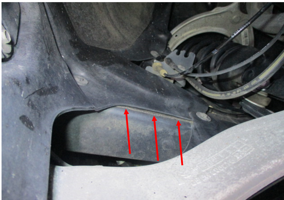
Photo 27 shows the chassis/structural body at the underside front left of the Motor Car. I did not find any weld marks other than original spot weld marks on the chassis/structural body of the Motor Car. The original factory sealant (arrowed) at the joints along the chassis/structural body was also untouched, indicating no work was done on the chassis/structural body of the Motor Car and that the chassis/structural body was originally fitted.
