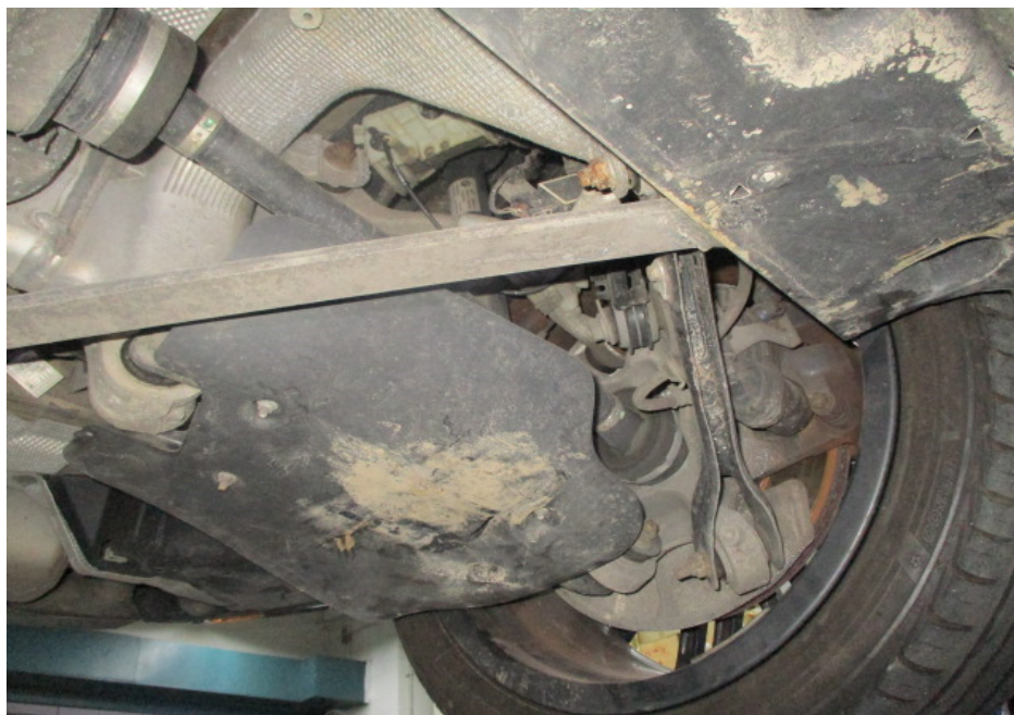
Photo 21 shows a general view of the control arms and linkages at the rear left wheel of the Motor Car. I did not observe any fluid leak and/or fluid stain on the underside of the Motor Car. All of the Motor Car's undercarriage components were observed to be intact and secured in an appropriate manner.
