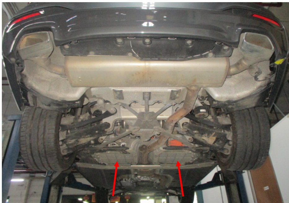
Photo 23 shows a general view of the Motor Car's electric battery (arrowed) that was fitted at the underside centre of the Motor Car. The cable connections were checked and found to be securely fitted into the respective connectors.
