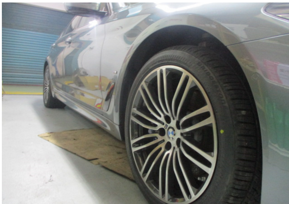
Photo 8 shows a closer view of the front right fender, front right wheel rim, front right tyre and right side rocker panel garnish of the Motor Car. The body parts at the front right portion of the Motor Car were visually examined and it was observed that the repair/restoration works carried out to the damaged area of the Motor Car (refer to photograph 1 & 2 above) were reasonably adequate and in order.
