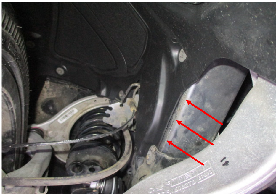
Photo 26 shows the chassis/structural body at the underside front right of the Motor Car. The original factory sealant (arrowed) at the joints along the chassis/structural body was observed to be untouched. In general, I had found no work was carried out on the chassis/structural body of the Motor Car. The chassis/structural body of the Motor Car was originally fitted.
