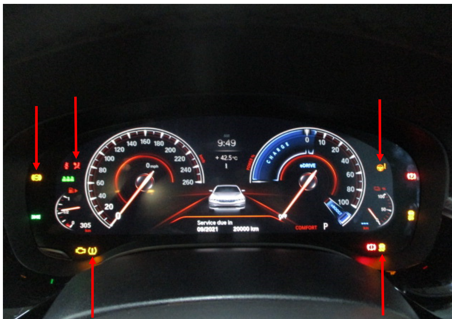
Photo 16 shows the warning lights for the various electronic safety features appearing on the instrument panel of the Motor Car during its self-test when the engine is cranked, in particular the ABS, SRS, IAS, TPM and DSC lights (arrowed).
