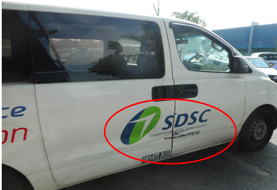
Photo 4 shows a close up view of the Mini Bus's right portion of the Mini Bus at the time of my inspection. It appeared to have sustained damage at its right portion. Its front right door (circled) were damage at the time of my inspection.
