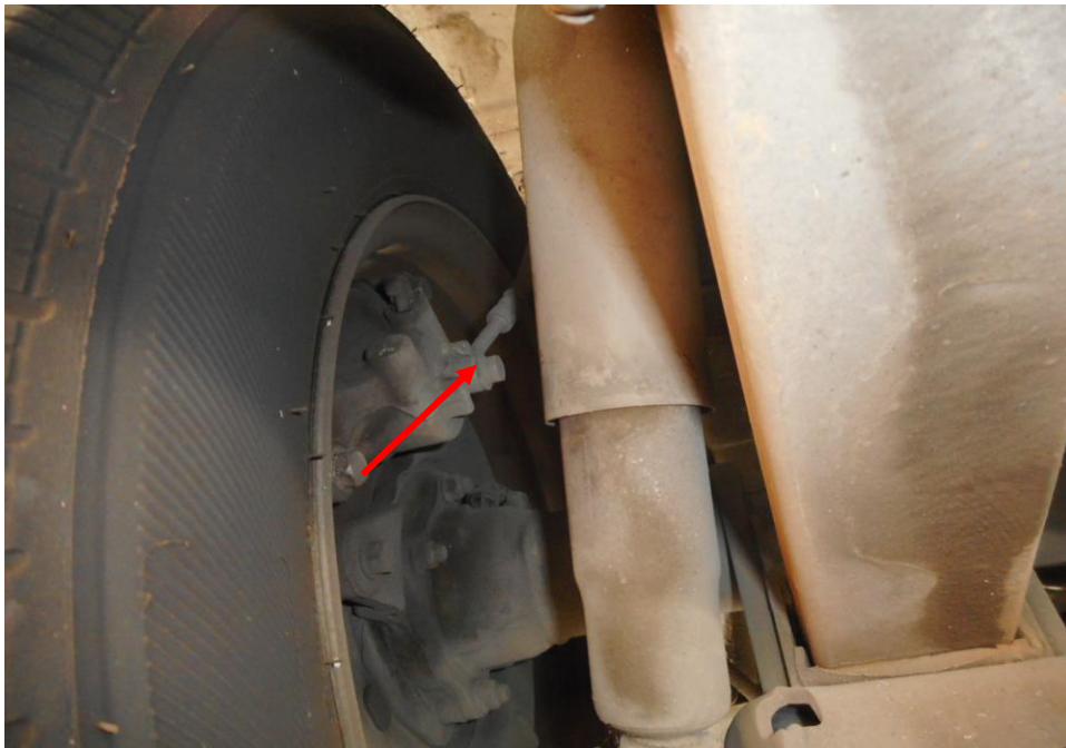
Photo 21 shows the brake pipe (arrowed) at the rear left wheel of the Mini Bus. I did not observe any leakage of brake fluid at the time of my inspection of the Mini Bus. My static tests of the Mini Bus's braking system, along with my visual examination of the various mechanical components in the braking system had indicated that there was no internal leakage of pressure/vacuum. Hence the braking system of the Mini Bus was likely to be in serviceable condition at the material time of accident.
