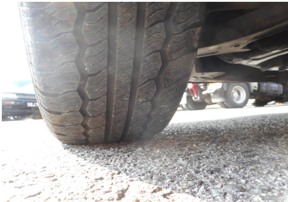
Photo 11 shows the condition of the rear right tyres of the Mini Bus, which were observed to be in serviceable condition with remaining, tread depth of approximately 5.5mm. There was also no tear, cut or burst mark(s) on the outer and the inner sidewalls as well as across the tread of the 4 tyres that were fitted on the Mini Bus.
