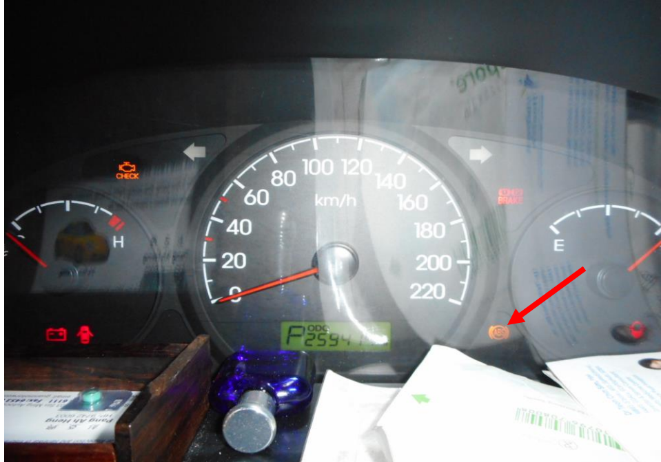
Photo 25 shows the warning light for Anti-Lock Brake System (ABS) (arrowed) appearing on the instrument panel of the Mini Bus during the self-test of its various electronic operating systems when its engine was cranked.
