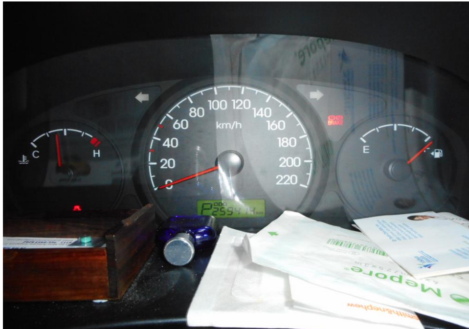
Photo 26 shows no warning lights illuminated on the instrument panel of the Mini Bus after the engine was cranked. This would suggest that there was no abnormality to the electronic operating system of the Mini Bus, like the ABS and etc.
