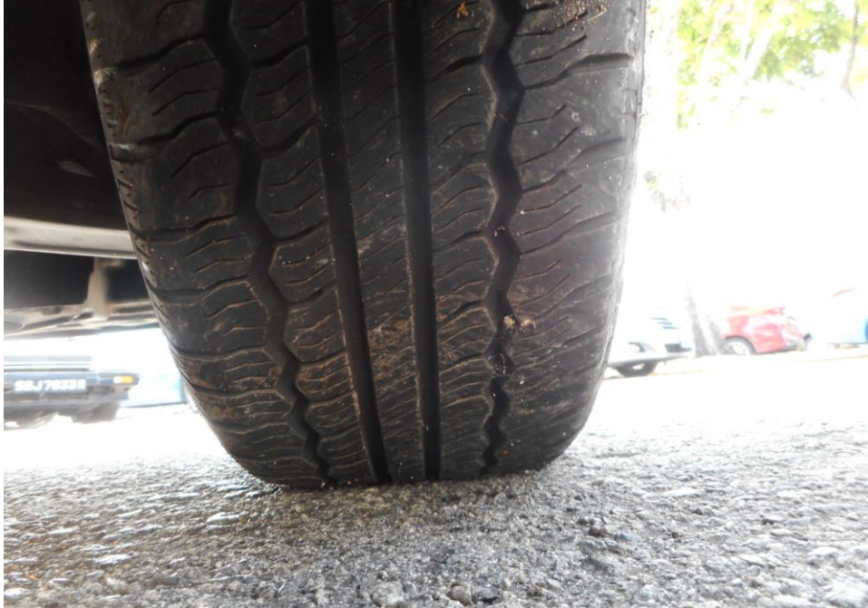
Photo 8 shows the condition of the front right tyre of the Mini Bus, which was observed to be in serviceable condition with remaining tread depth of approximately 6.1mm. The tyre, which was wrapped around standard steel wheel rim, was also observed to be sufficiently inflated for vehicular operation. There was no tear, cut or burst mark(s) on the outer and the inner sidewalls as well as across the tread of the 4 tyres that were fitted on the Mini Bus.
