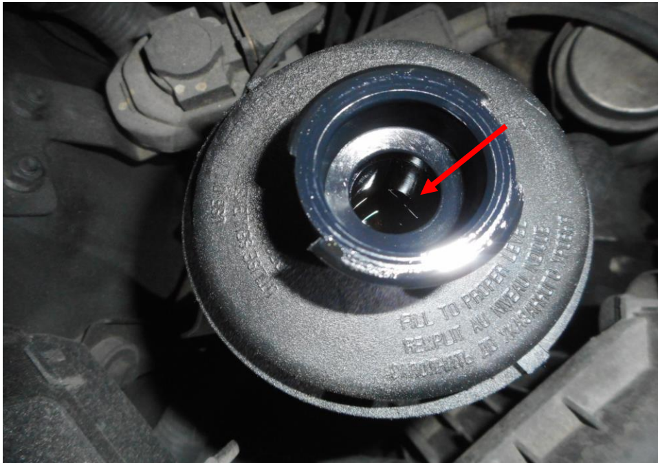
Photo 16 shows the power steering fluid reservoir of the Mini Bus at the time of my inspection. The power steering fluid was observed to be of sufficient level (arrowed) and without any visible contamination.
