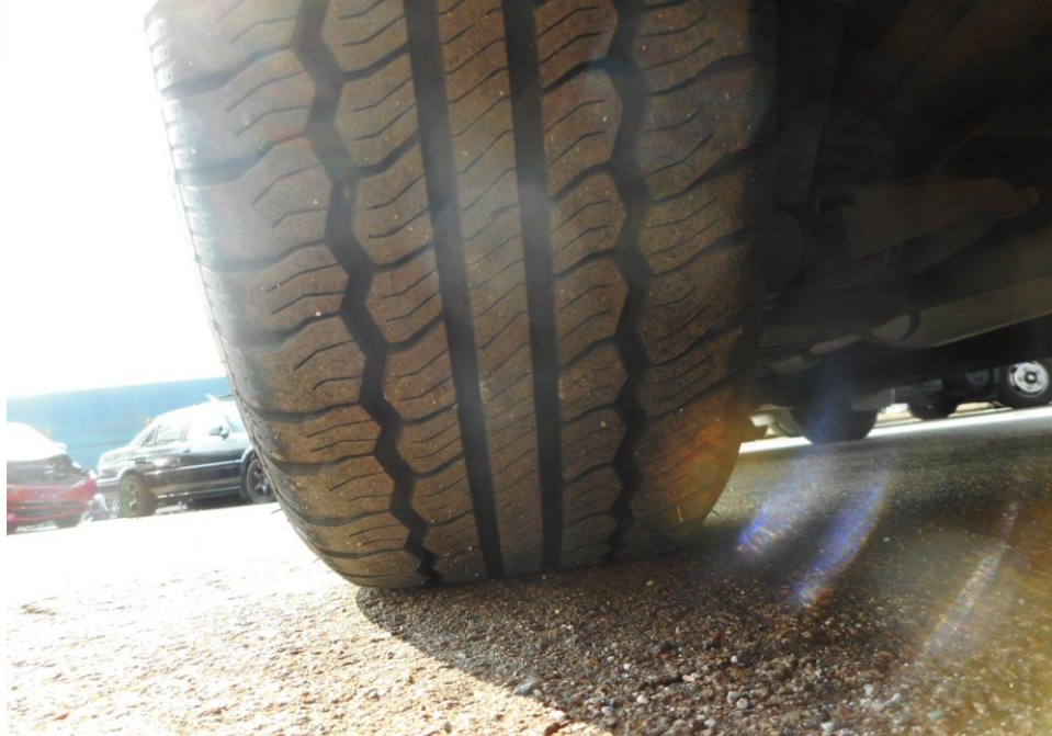
Photo 10 shows the condition of the rear left tyres of the Mini Bus, which was observed to be in serviceable condition with remaining tread depth of approximately 5.9mm. The tyres, which were wrapped around standard steel wheel rim, were also observed to be sufficiently inflated for vehicular operation. There was also no damage found on all 4 steel wheel rims of the Mini Bus.
