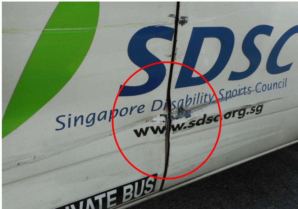
Photo 5 shows a close up view of the Mini Bus's right portion at the time of my inspection. Its right door (circled) was damage at the time of my inspection as a result of the accident.
