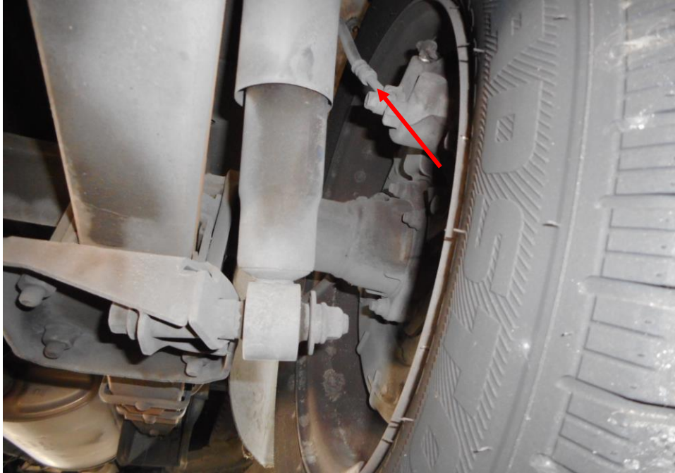
Photo 20 shows the brake pipe (arrowed) at the rear right wheel of the Mini Bus. I did not observe any leakage of brake fluid at the time of my inspection of the Mini Bus. My static tests of the Mini Bus's braking system, along with my visual examination of the various mechanical components in the braking system, had indicated that there was no internal leakage of pressure/vacuum. Hence the braking system of the Mini Bus was likely to be in serviceable condition at the material time of accident.
