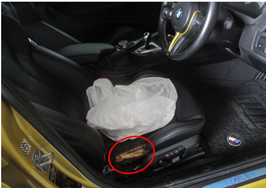
Photo 7 shows the driver seat of the Insured Vehicle at the time of our inspection. The fire damage was confined to its driver side. The driver seat was observed to be partially burnt and/or melted (circled).
