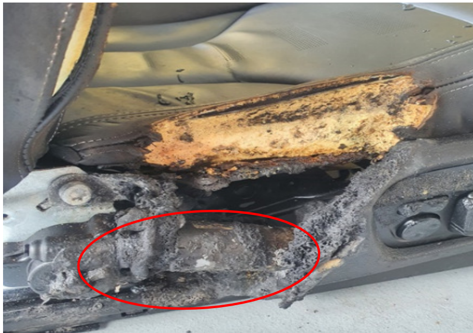
Photo 17 shows upon closer examination, the fire appears to have started from one of the motors located at the right portion of the driver seat (circled).
