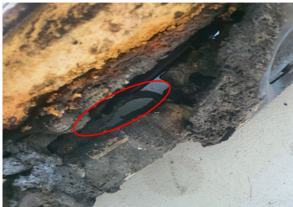
Photo 18 shows a closer look at the wirings leading from the motor located at the right portion of the driver seat of the Insured Vehicle. We found greenish residue on some of the wirings (circled). The presence of such greenish residue suggest occurrence of an electrical short circuit. The greenish residue is normally left behind from oxidation as a result of chemical reaction involving the copper wires.
