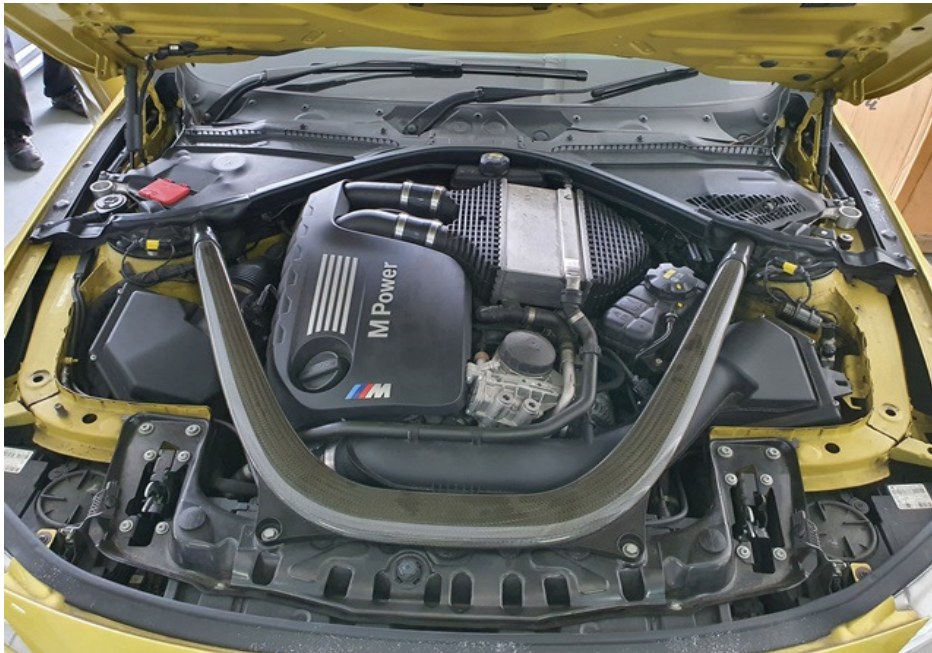
Photo 2 shows the general view of the engine compartment of the Insured Vehicle at the time of our inspection. The fire damage was confined to its interior compartment. The engine compartment of the Insured Vehicle was observed to be relatively unaffected by the fire.
