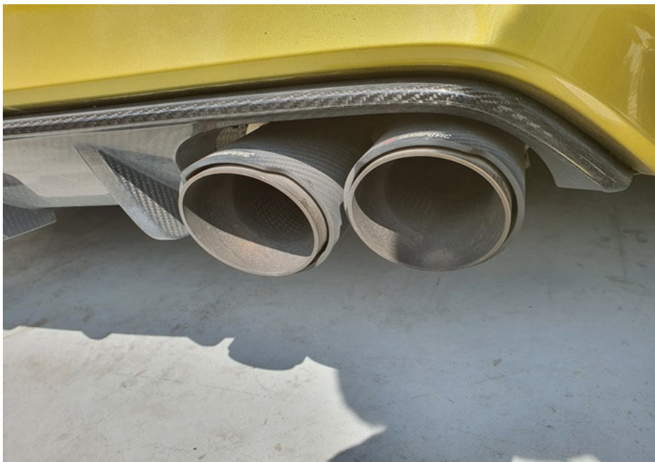
Photo 12 shows a front view of the non-standard rear exhaust mufflers that were found to be fitted on the Insured Vehicle at the time of our inspection.
