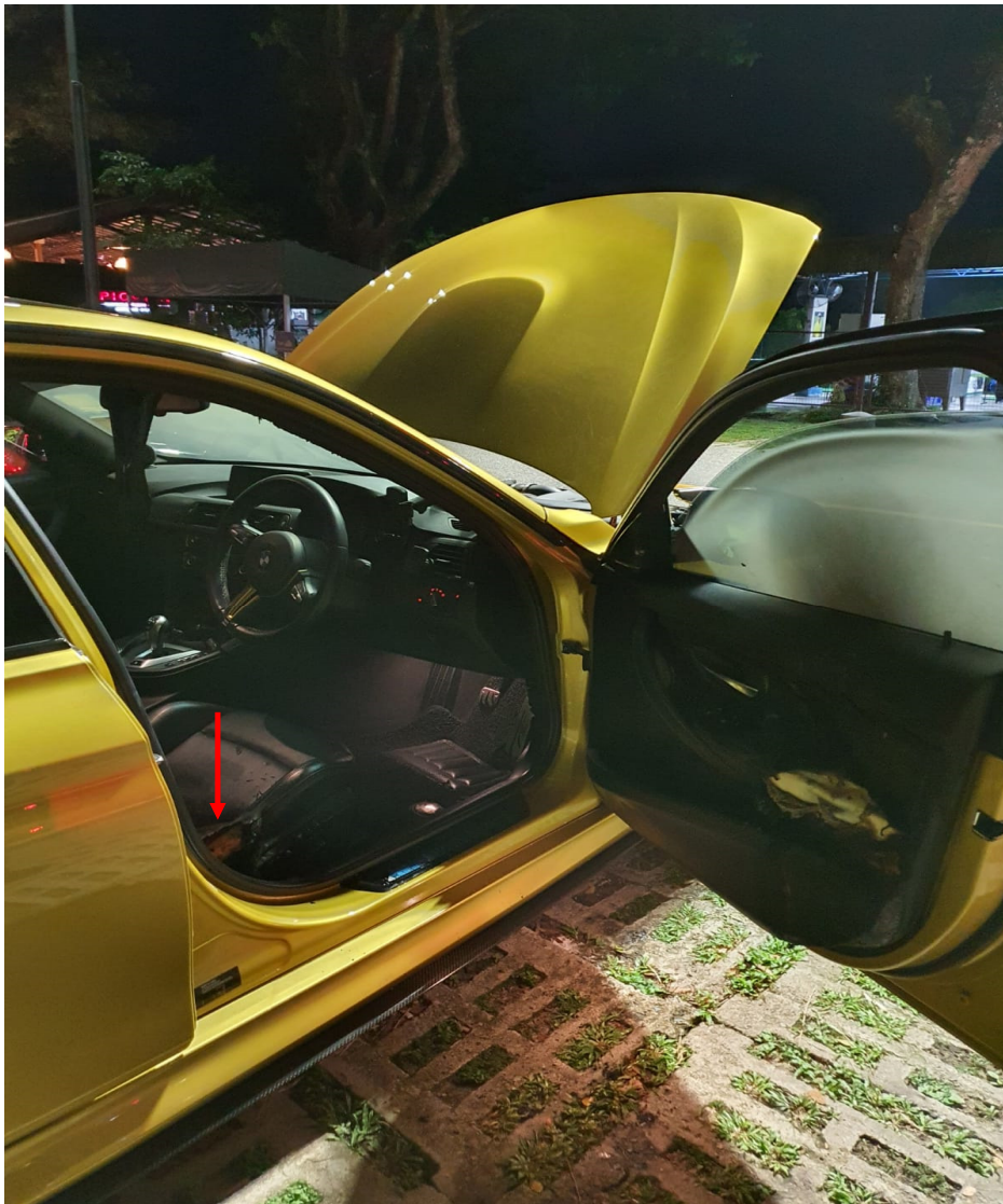
Photo 24 shows the interior compartment of the Insured Vehicle post- incident. In general, the information that could be gathered from this photograph had corresponded to the events that were related to us by Mr Simon, which is the fire had started from the driver seat of the Insured Vehicle (arrowed).
