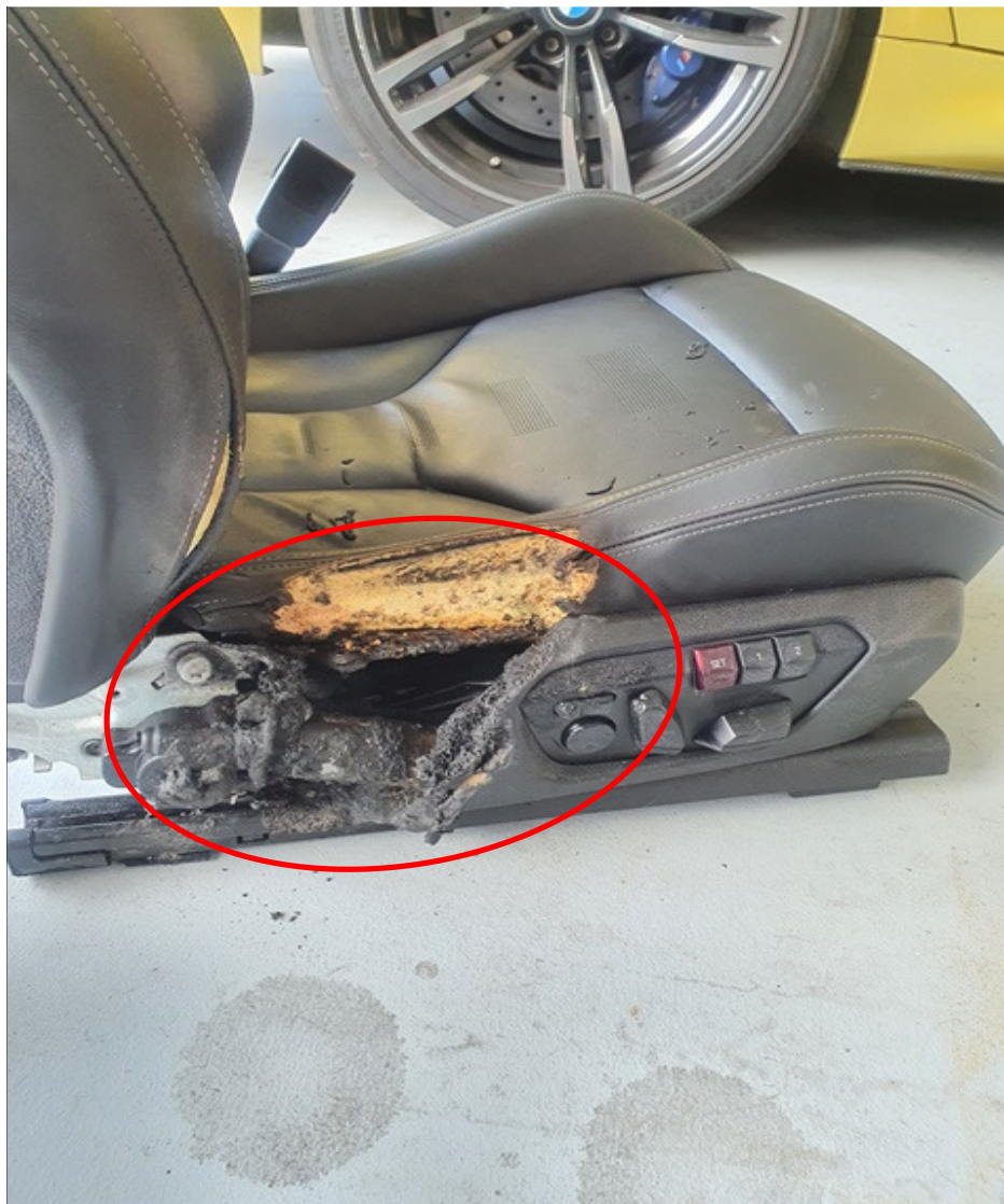
Photo 15 shows the dismantled driver seat of the Insured Vehicle. The fire appears to have originated from the right portion of the driver seat of the Insured Vehicle. This can be observed from the burnt components of the driver seat (circled).
