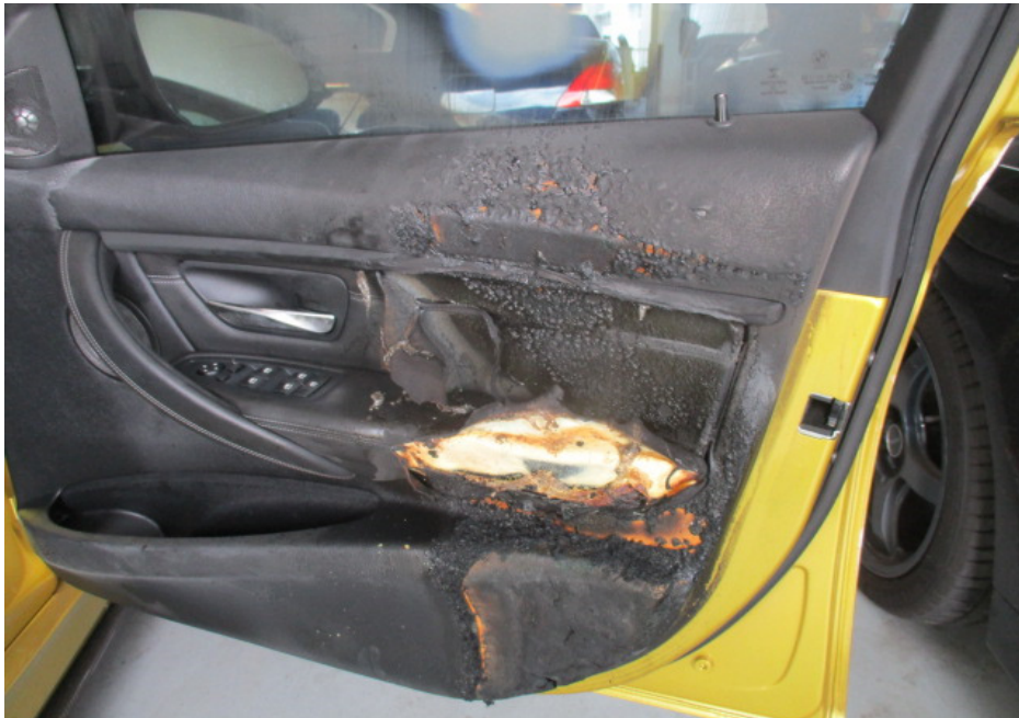
Photo 6 shows the driver door panel of the Insured Vehicle at the time of our inspection. The fire damage was confined to its driver side. The driver door panel was observed to be partially burnt and/or melted.
