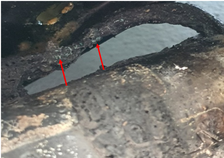
Photo 20 shows a close up view of some of the wirings with greenish residue (arrowed). The presence of such greenish residue suggest occurrence of an electrical short circuit.
