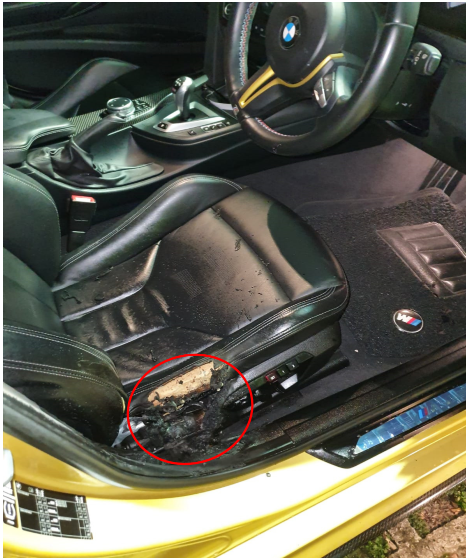
Photo 25 shows a close up view of the driver seat of the Insured Vehicle post-incident. In general, the information that could be gathered from this photograph had corresponded to the events that were related to us by Mr Simon, which is the fire had started from the driver seat of the Insured Vehicle (circled).
