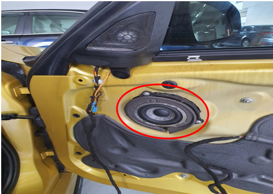
Photo 11 shows the 1st aftermarket speaker fitted at the driver door panel (circled). The brand of the speaker was 'FOCAL'.
