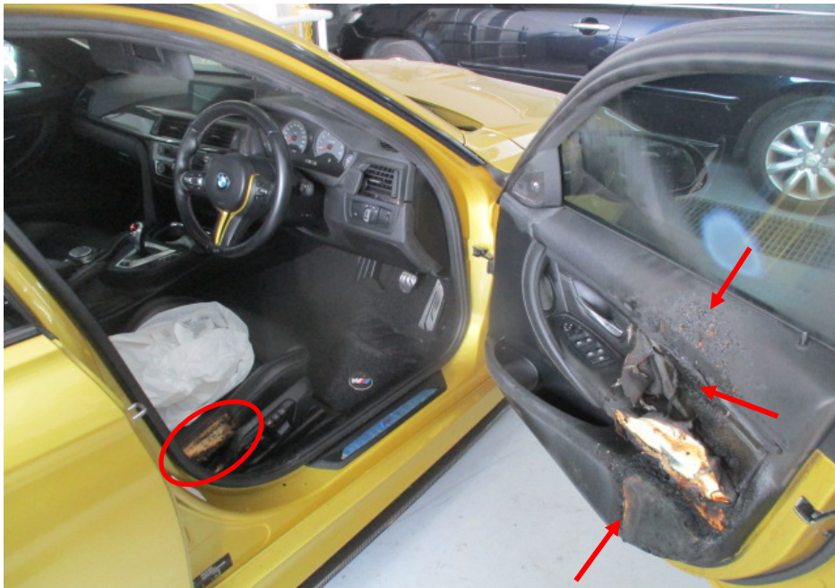
Photo 5 shows the interior compartment of the Insured Vehicle at the time of our inspection. The fire had resulted in several components in the interior compartment to be slightly burnt and/or damaged. This had included its driver seat (circled), floor carpet, insulating material covering the floor panel and driver door panel (red arrows) amongst others.
