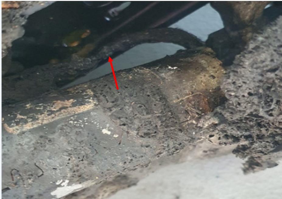
Photo 19 shows a closer view of some of the wirings with greenish residue (arrowed). The presence of such greenish residue suggest occurrence of an electrical short circuit.
