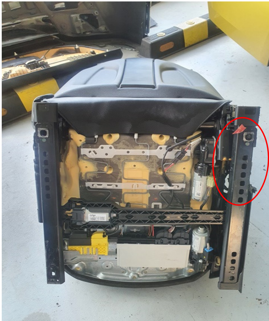
Photo 16 shows the underside of the dismantled driver seat of the Insured Vehicle. The components on the underside of the driver seat were relatively unaffected by the fire. Hence the fire appears to have originated from the right portion of the driver seat of the Insured Vehicle (circled).
