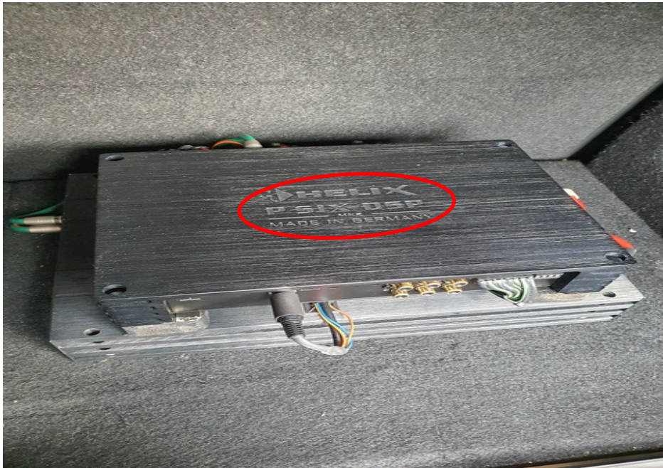
Photo 9 shows the aftermarket amplifier fitted at the boot of the Insured Vehicle upon our inspection. The brand of the amplifier was 'HELIX' (circled).
