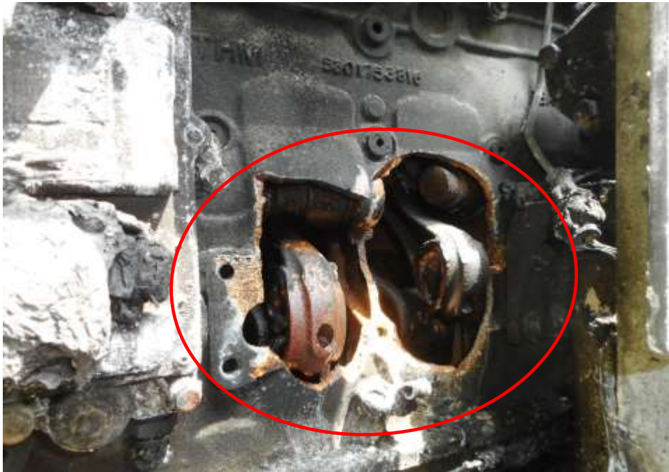
Photo 15 shows the close up view of the engine block on the Insured Vehicle at the time of our inspection. The Insured Vehicle was observed to have sustained damaged to its engine block and piston connecting rod (circled) due to insufficient engine oil for lubrication and heat removal purposes in the engine that resulted in the sudden seizure of the running components in the engine causing them to break.
