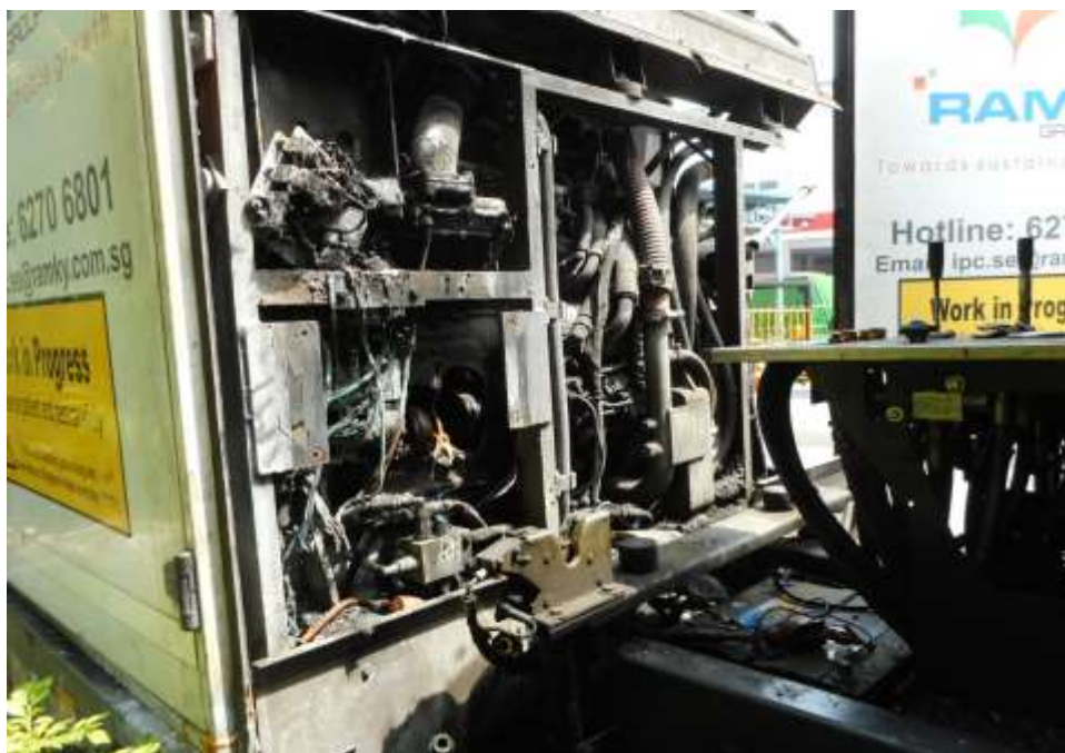
Photo 6 shows the engine compartment in the middle of the Insured Vehicle at the time of our inspection. The engine compartment of the Insured Vehicle was observed to be burnt. The electrical wirings, engine block and components around the engine area was damaged as a result of the fire.
