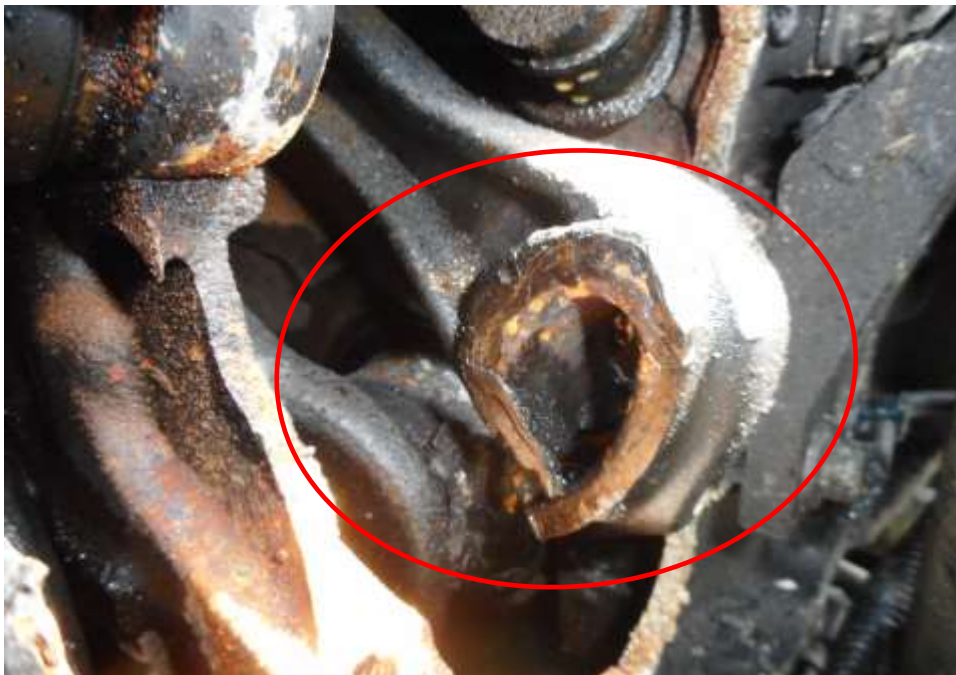
Photo 16 shows the close up view of the engine block n the Insured Vehicle at the time of our inspection. The Insured Vehicle was observed to have sustained damaged to piston connecting rod (red circled) due to insufficient engine oil for lubrication and heat removal purposes in the engine that resulted in the sudden seizure of the running components in the engine causing them to break.
