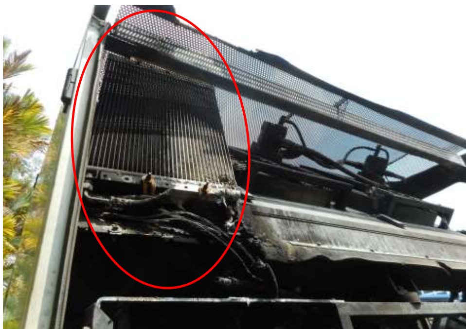
Photo 8 shows the engine compartment of the Insured Vehicle at the time of our inspection. The Insured Vehicle was observed to have sustained fire damage to its engine radiator component (circled) was damaged as a result of the fire.
