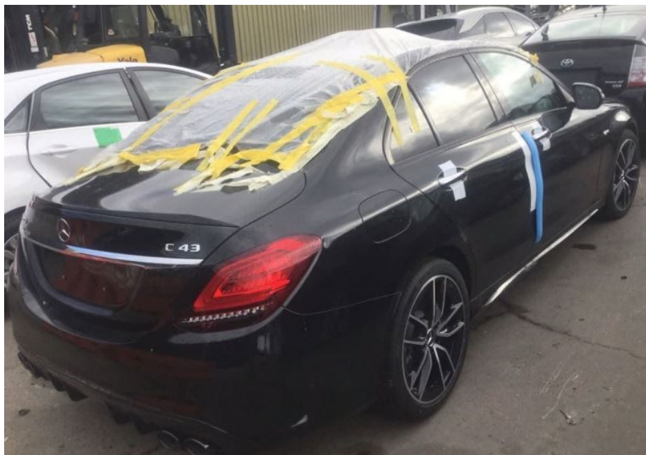
Photo 3 shows the rear right body of the Motor Car prior to any repairs being carried out (photograph provided to me). The Motor Car was observed to have sustained damages of indentation nature to exterior body parts. The roof panel and rear windscreen of the Motor Car were covered with plastic sheets, indicating possible damage to the rear windscreen and panoramic sunroof of the Motor Car.
