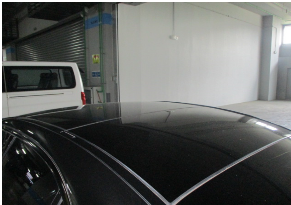
Photo 10 shows the roof panel and panoramic sunroof of the Motor Car at the time of my inspection. In general, I had found that the repair/restoration works carried out to the damaged area of the Motor Car (refer to photograph 3 & 4 above) were reasonably adequate and in order.
