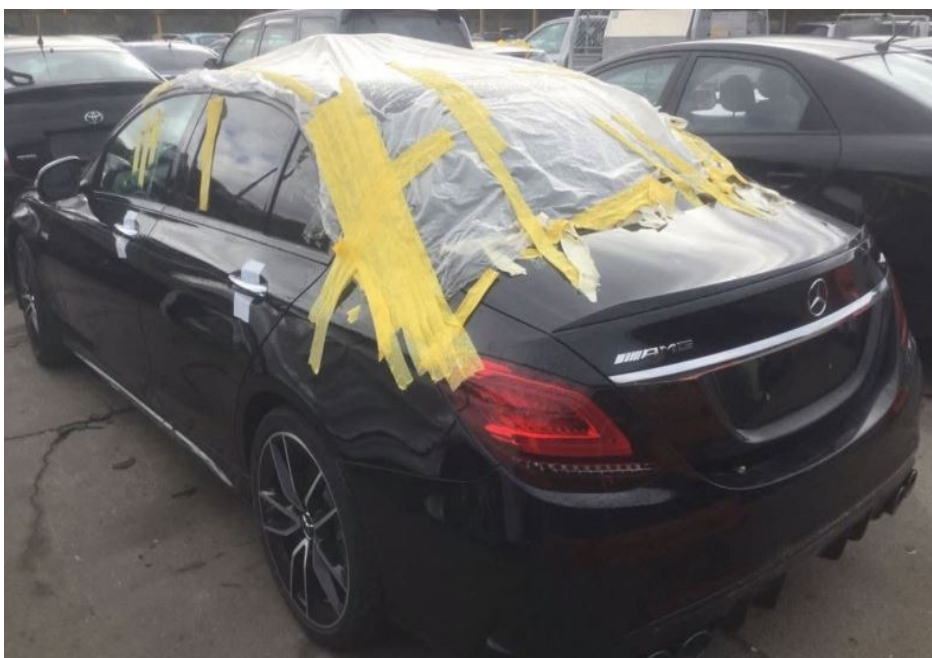
Photo 4 shows the rear left body of the Motor Car prior to any repairs being carried out (photograph provided to me). The Motor Car was observed to have sustained damages of indentation nature to exterior body parts. The roof panel and rear windscreen of the Motor Car were covered with plastic sheets, indicating possible damage to the rear windscreen and panoramic sunroof of the Motor Car.
