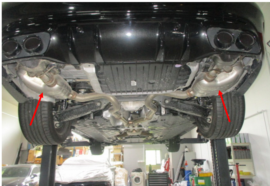
Photo 20 shows a general view of the Motor Car's exhaust system (arrowed). My examination of the Motor Car's exhaust system revealed no sign(s) or indication(s) of any cut or weld marks along its catalytic converters, exhaust pipes and on its rear mufflers (arrowed).
