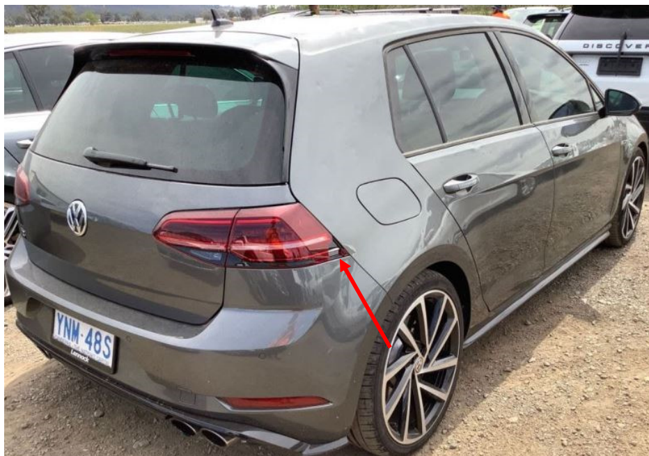
Photo 3 shows the rear right body of the Motor Car prior to any repairs being carried out (photograph provided to me). The Motor Car was observed to have sustained damages of indentation nature to exterior body parts. The rear right taillamp (arrowed) was also observed to be broken.
