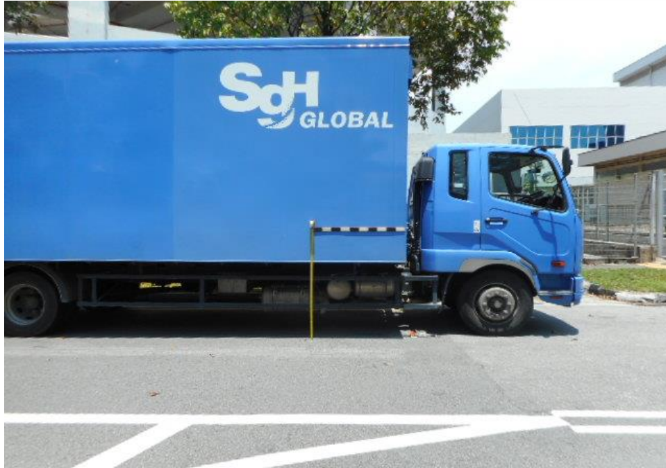
Photo 7 shows the general view of the height measurement being conducted on the right portion of Third Party. The height above ground level of where the damages were found to the right body panel of the Third Party was between 130cm and 135cm.
