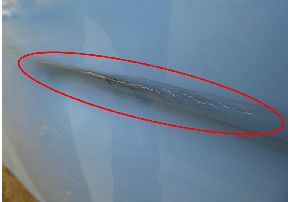
Photo 2 shows the close up view of the rear portion of Third Party at the time of inspection. The right body panel had been damaged. It was also noted that these were paint crack marks, dents and black rubber marks (circled).
