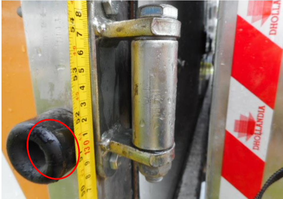
Photo 5 shows a close up view of the Insured rear portion. We observed scratches on the rear left rubber stopper (circled).
