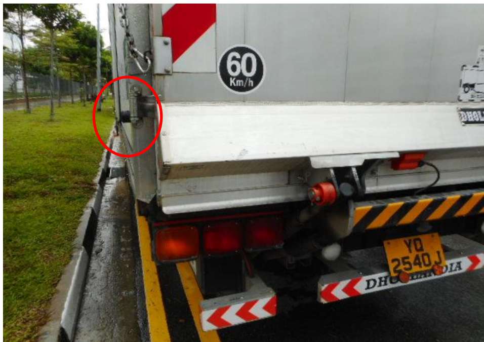
Photo 4 shows a close up view of the Insured rear portion. We observed scratches on the rear left rubber stopper (circled).
