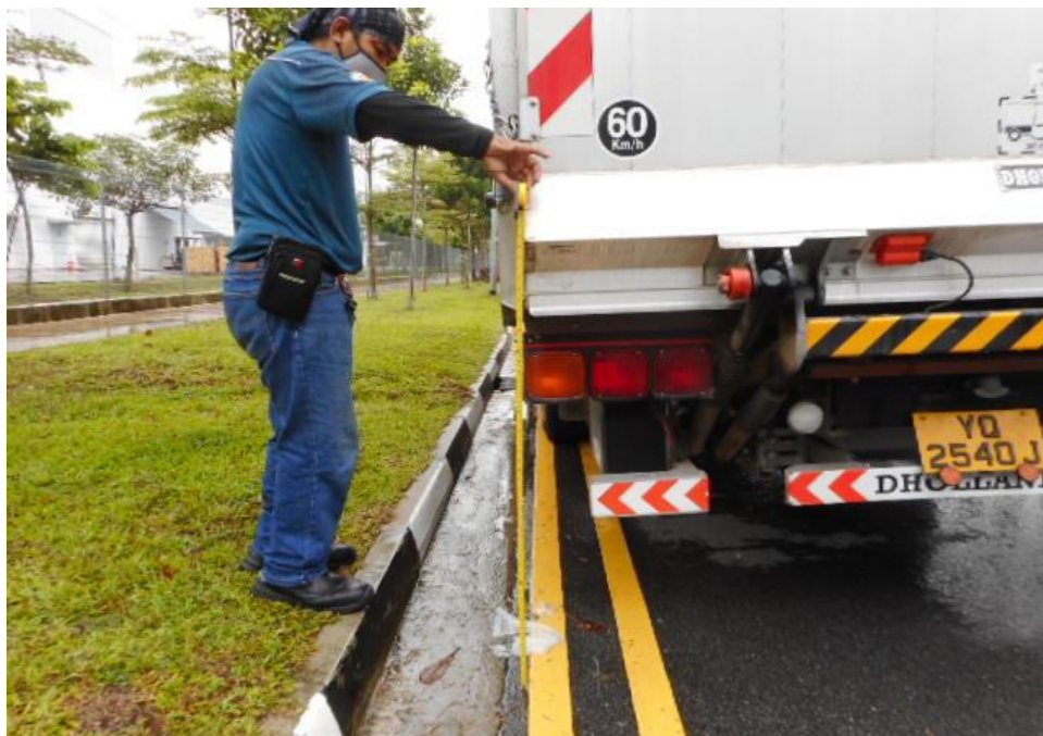
Photo 8 shows a general view of the height measurement being conducted on the rear left portion of Insured. The scratch marks found on the rear left rubber stopper was measured to be between 129cm to 132cm above ground level.
