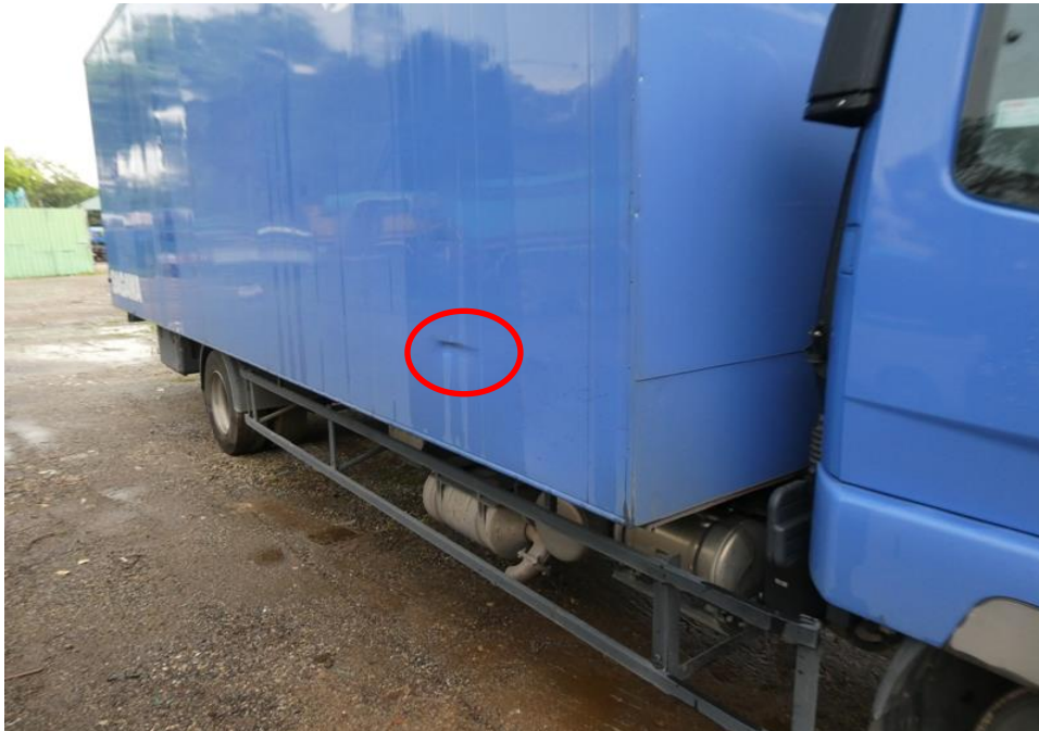
Photo 1 shows the general view of the rear portion of Third Party at the time of inspection. The right body panel had been damaged. It was also noted that these were paint crack marks, dents and black rubber marks (circled).
