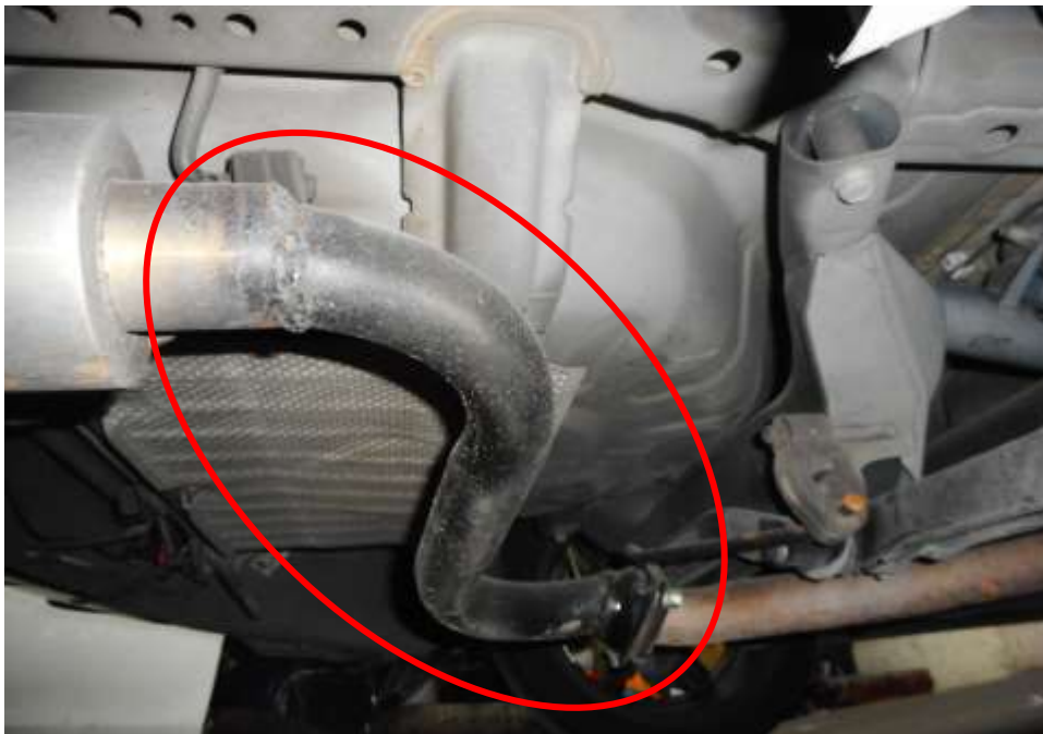
Photo 11 shows the additionally fitted exhaust pipe (arrowed) that was fitted on the insured vehicle at the time of my inspection. This was at the tailpipe section, at the rear of the insured vehicle. It was noted that there was additional piping and welding marks linking the exhaust muffler to the middle pipe of the Insured Vehicle's exhaust system. From my observations, the exhaust system fitted on the insured vehicle is not LTA compliant.
