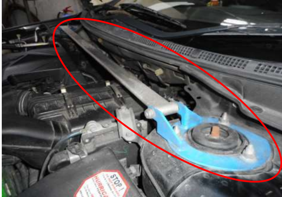
Photo 7 shows a general view of the engine compartment of the insured vehicle. Additional non-standard parts were found fitted. This includes an additionally fitted front anti-roll bar (circled) and electronic component.
