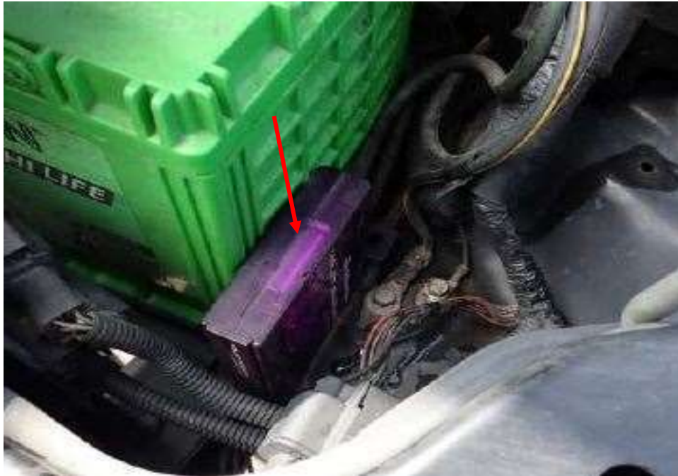
Photo 9 shows a closer view of the additionally fitted electronic component that was found inside the engine compartment of the insured vehicle. From my understanding and from my research this electronic component is collectively advertised to be able to improve acceleration response whilst improving fuel efficiency through stabilization of the electrical system of a motor car.
