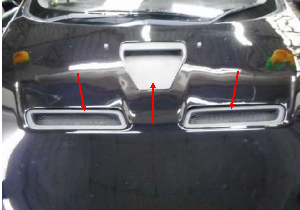
Photo 12 shows a general view of the front bonnet of the insured vehicle. An aftermarket front bonnet with scoops (arrowed) made of carbon fiber material type were found fitted.
