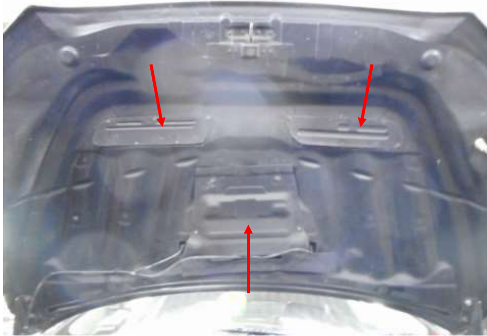
Photo 13 shows a general underside view of the front bonnet of the insured vehicle. An aftermarket front bonnet with scoops (arrowed) made of carbon fiber material type were found fitted.
