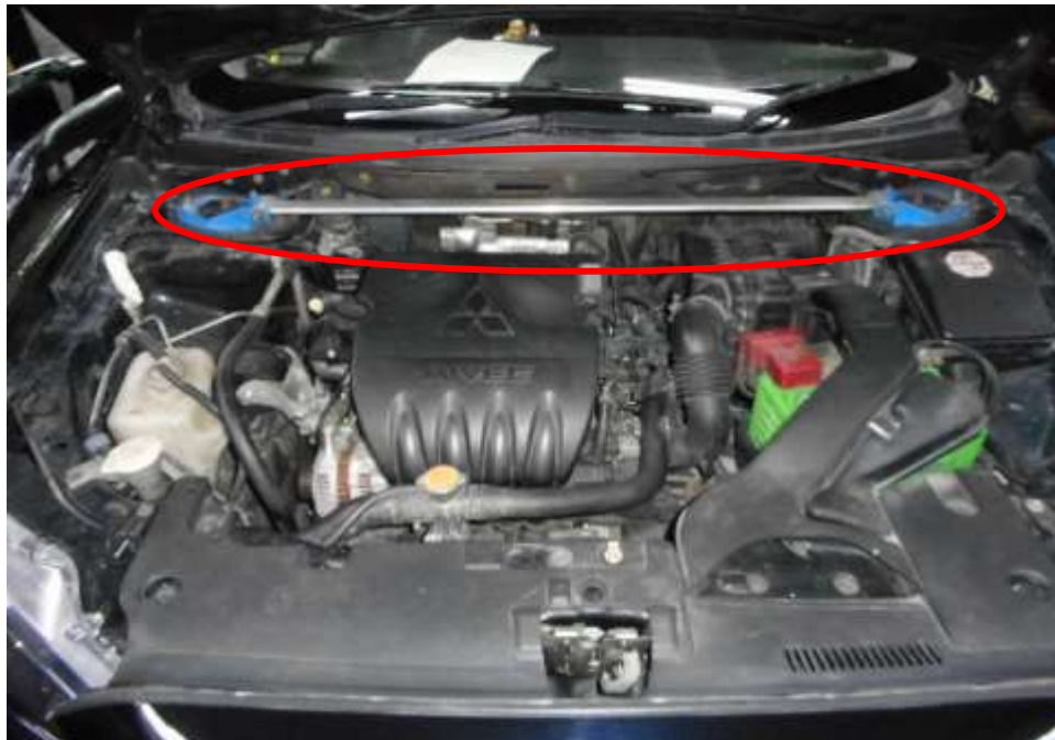
Photo 6 shows a general view of the engine compartment of the insured vehicle. Additional non-standard parts were found fitted. This includes an additionally fitted front anti-roll bar and electronic component.
