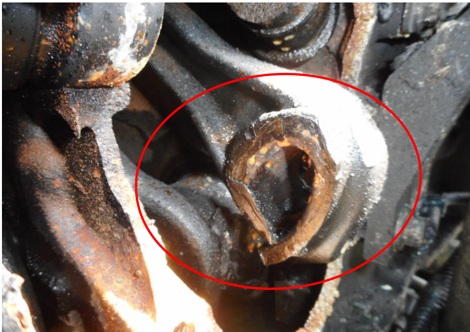
Photo 17 shows the close up view of the engine block n the Insured Vehicle at the time of our inspection. The Insured Vehicle was observed to have sustained damaged to piston connecting rod (red circled) due to insufficient engine oil for lubrication and heat removal purposes in the engine that resulted in the sudden seizure of the running components in the engine causing them to break.
