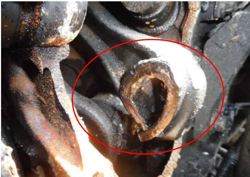
Photo 17 shows the close up view of the engine block on the Insured Vehicle at the time of our inspection. The Insured Vehicle was observed to have sustained damaged to piston connecting rod (red circled) due to insufficient engine oil for lubrication and heat removal purposes in the engine that resulted in the sudden seizure of the running components in the engine causing them to break.
