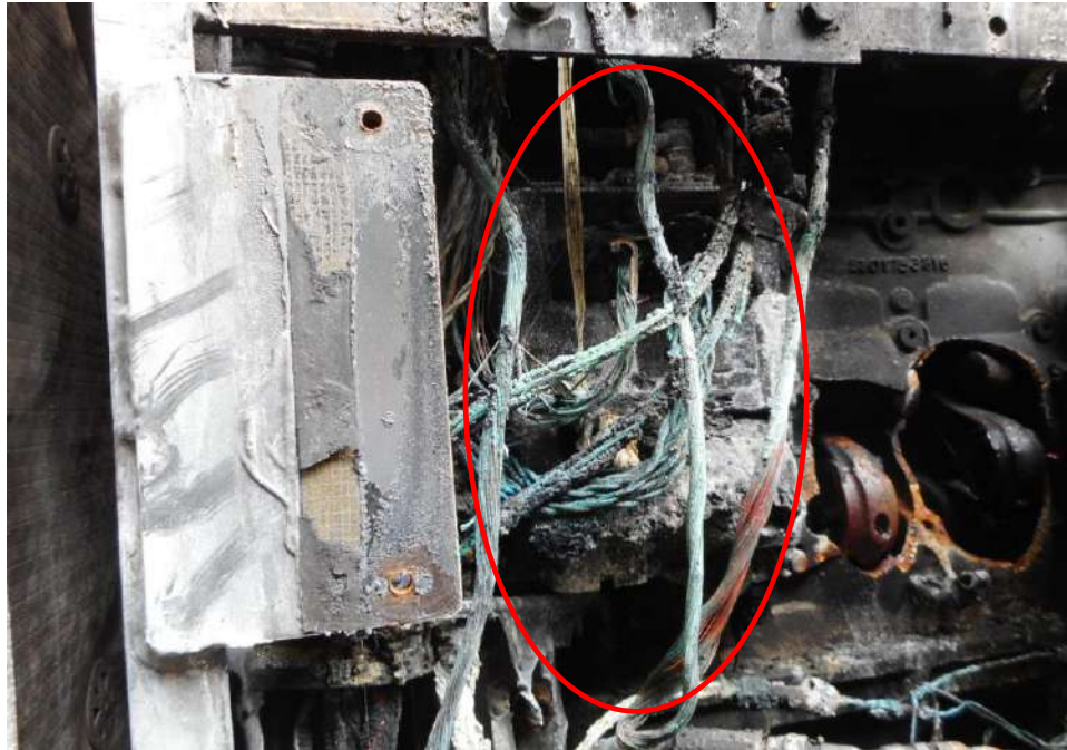
Photo 10 shows the close up view of the engine of the Insured Vehicle at the time of our inspection. The burn pattern of the various components which were observed to be partly melted and burn from the high heat intensity and exposure of bare copper wirings (circled) indicates that the fire had originated from the wirings of the engine portion of the Insured Vehicle.
