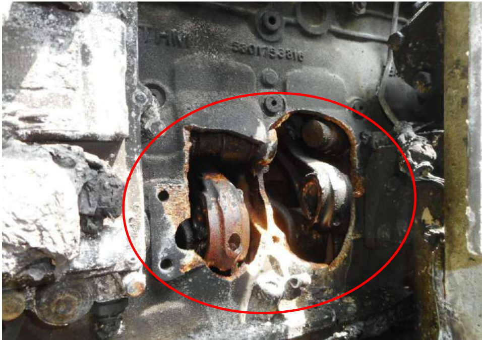
Photo 16 shows the close up view of the engine block on the Insured Vehicle at the time of our inspection. The Insured Vehicle was observed to have sustained damaged to its engine block and piston connecting rod (circled) due to insufficient engine oil for lubrication and heat removal purposes in the engine that resulted in the sudden seizure of the running components in the engine causing them to break.
