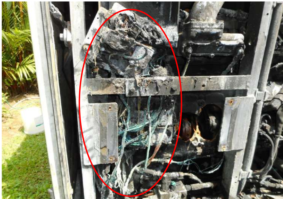
Photo 9 shows the close up view of the engine of the Insured Vehicle at the time of our inspection. The burn pattern of the various components which were observed to be partly melted and burn from the high heat intensity and exposure of bare copper wirings (circled) indicates that the fire had originated from the wirings of the engine portion of the Insured Vehicle.
