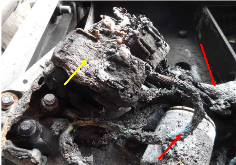
Photo 13 shows close up view of the original wiring harness from the batteries (red arrow) to the electrical components (yellow arrow) was observed with greenish residue on the surface. The presence of greenish residue indicates internal heating of copper wires, a sign of an electrical short circuit occurring. The greenish residue is normally left behind from oxidation as a result of chemical reaction involving the copper wires.
