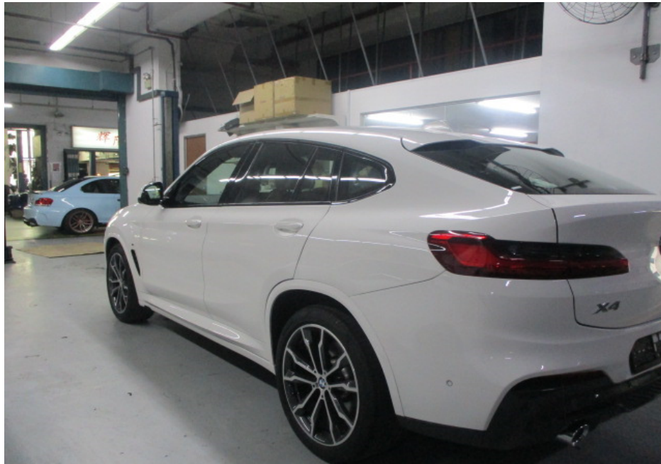
Photo 10 shows a general view of the rear left body of the Motor Car at the time of my inspection. The Motor Car was observed to be in a relatively good general condition with no loose exterior fittings observed. The body parts along the entire left side portion of the Motor Car were visually examined and it was observed that the repair/restoration works carried out to the damaged area of the Motor Car (refer to photograph 1 - 4 above) were reasonably adequate and in order.
