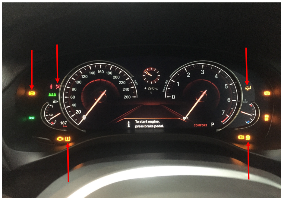
Photo 15 shows the warning lights for the various electronic safety features appearing on the instrument panel of the Motor Car during its self-test when the engine is cranked, in particular the ABS, SRS, IAS, TPM and DSC lights (arrowed).
