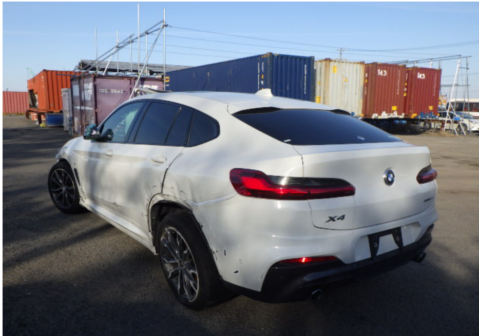
Photo 3 shows the rear left body of the Motor Car (photograph provided to me). The Motor Car was observed to have sustained damages along its entire left side portion. The rear bumper, rear left fender, rear left fender wheel arc garnish, rear left wheel rim and rear left door were amongst the parts that were observed to have been damaged.
