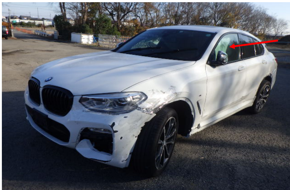
Photo 1 shows the front left body of the Motor Car (photograph provided to me). The Motor Car was observed to have sustained damages along its entire left side portion. The front bumper, front bumper left lower grille, front bumper left day running light, front left headlamp and front left fender were amongst the parts that were observed to have been damaged. The left side curtain airbag (arrowed) was also deployed.
