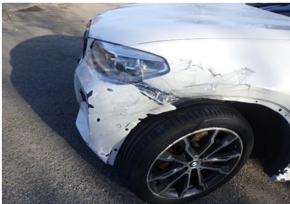
Photo 2 shows a closer view of the damage at the front left portion of the Motor Car (photograph provided to me). The front bumper, front left fender, front left fender wheel arc garnish and front left wheel rim were amongst the parts that were observed to have been damaged. The orientation of the front left wheel and front right wheel (refer to photograph 5 below) indicate damage to the front left undercarriage parts of the Motor Car.
