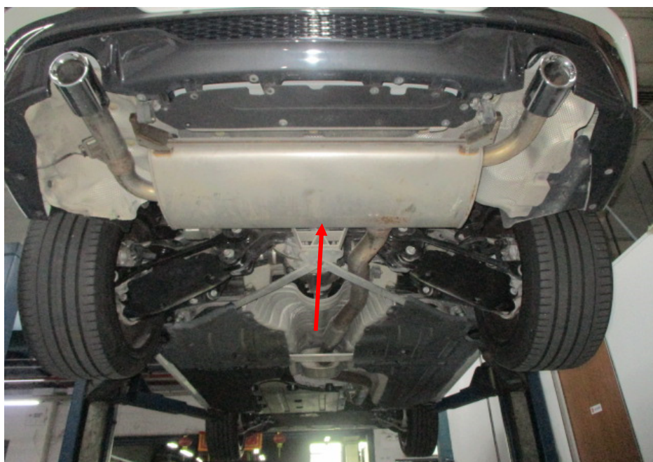
Photo 21 shows the Motor Car's rear muffler (arrowed). My examination of the Motor Car's exhaust system revealed no sign(s) or indication(s) of any cut or weld marks along its exhaust pipes and on its catalytic converter.
