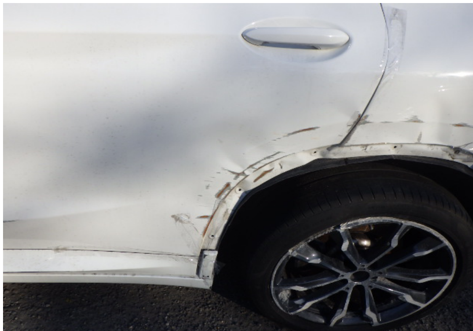
Photo 4 shows a closer view of the damage at the rear left portion of the Motor Car (photograph provided to me). The rear left fender, rear left fender wheel arc garnish, rear left wheel rim, left rear door, left rear door lower moulding and left rocker panel garnish were amongst the parts that were observed to have been damaged.
