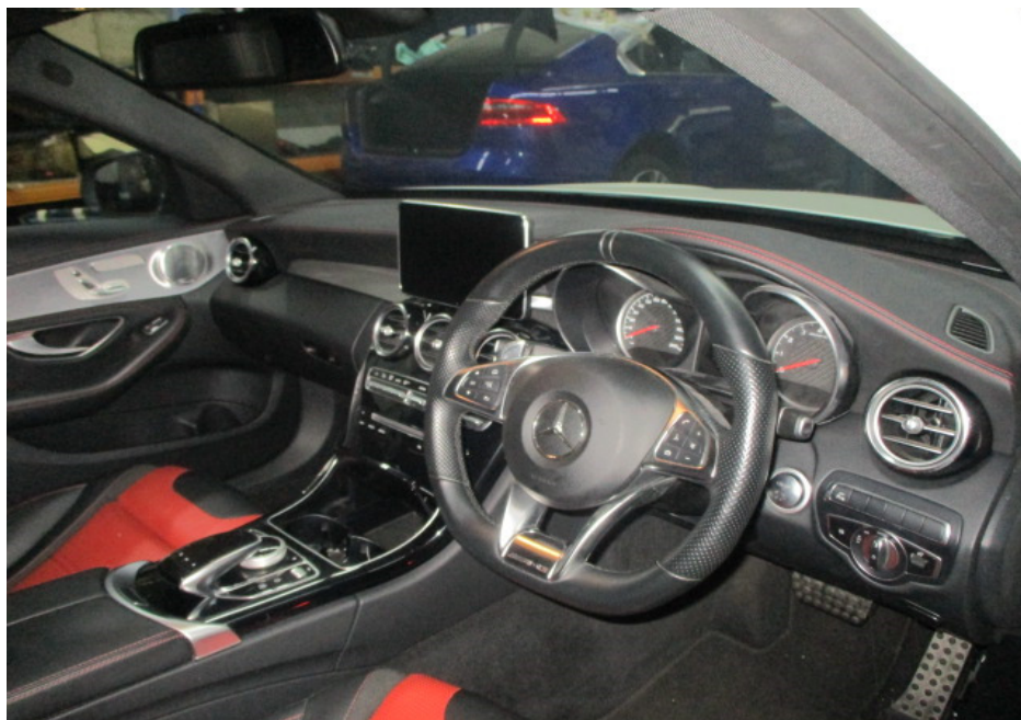
Photo 10 shows a general view of the dashboard panel of the Motor Car. The steering wheel (driver's airbag) and dashboard panel (front left passenger airbag) were checked, and it was observed that the repair/restoration works carried out to parts damaged by the activation of the driver's airbag and front left passenger airbag were reasonably adequate and in order.
