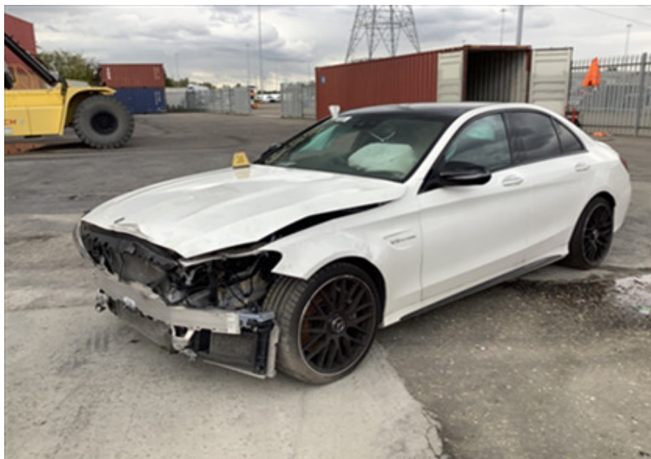
Photo 2 shows the front left body of the Motor Car (photograph provided to me). The Motor Car was observed to have sustained damage at its frontal portion. The front left passenger airbag and left curtain airbag were activated.
