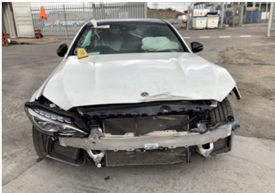
Photo 1 shows the frontal body of the Motor Car (photograph provided to me). The Motor Car was observed to have sustained damage at its frontal portion. The front bumper and all its related attachments and fittings, front bumper reinforcement, radiator grille, front headlamps, front fender inner shields, front bonnet, front bonnet lock, aircon condenser, radiator, radiator air guide, front support panel and front support panel top garnish were amongst the parts that were observed to have been damaged.
