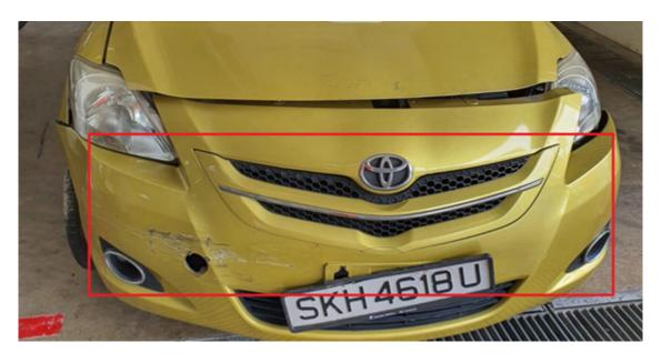
3) SPECIAL NETT No. 21: FT Fender Inner Cowling Clips - Damages to Fender is obvious proof that clips would not ne usable.
