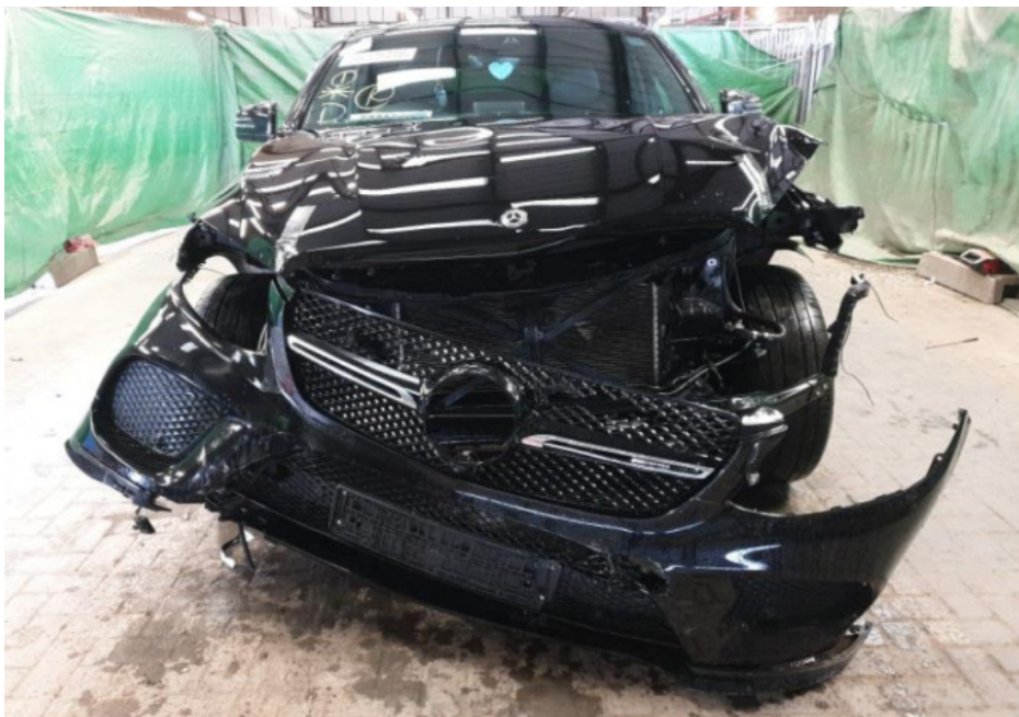
Photo 2 shows the frontal body of the Motor Car (photograph provided to me). The Motor Car was observed to have sustained damage at its frontal portion. The front bumper, front bumper centre lower grille, radiator grille, radiator grille emblem, front headlamps and front bonnet were amongst the parts that were observed to have been damaged.
