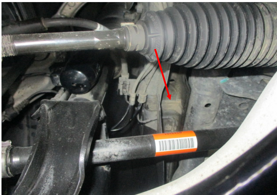
Photo 22 shows the chassis/structural body at the underside front right of the Motor Car. I did not find any weld marks other than original spot weld marks on the chassis/structural body of the Motor Car. The original factory sealant (arrowed) at the joints along the chassis/structural body was also untouched, indicating no work was done on the chassis/structural body of the Motor Car and that the chassis/structural body was originally fitted.
