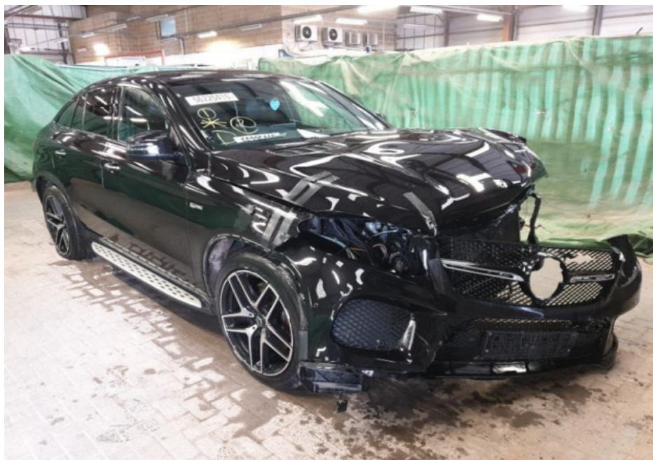
Photo 3 shows the front right body of the Motor Car (photograph provided to me). The Motor Car was observed to have sustained damage at its frontal portion. The front bumper, radiator grille, radiator grille emblem, front bonnet, front right headlamp, and front right fender were amongst the parts that were observed to have been damaged.
