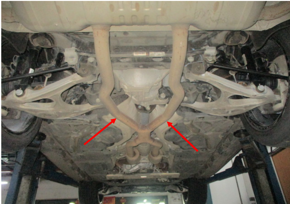
Photo 20 shows a general view of the Motor Car's exhaust system (arrowed). My examination of the Motor Car's exhaust system revealed no sign(s) or indication(s) of any cut or weld marks along its catalytic converters, exhaust pipes and on its rear muffler.
