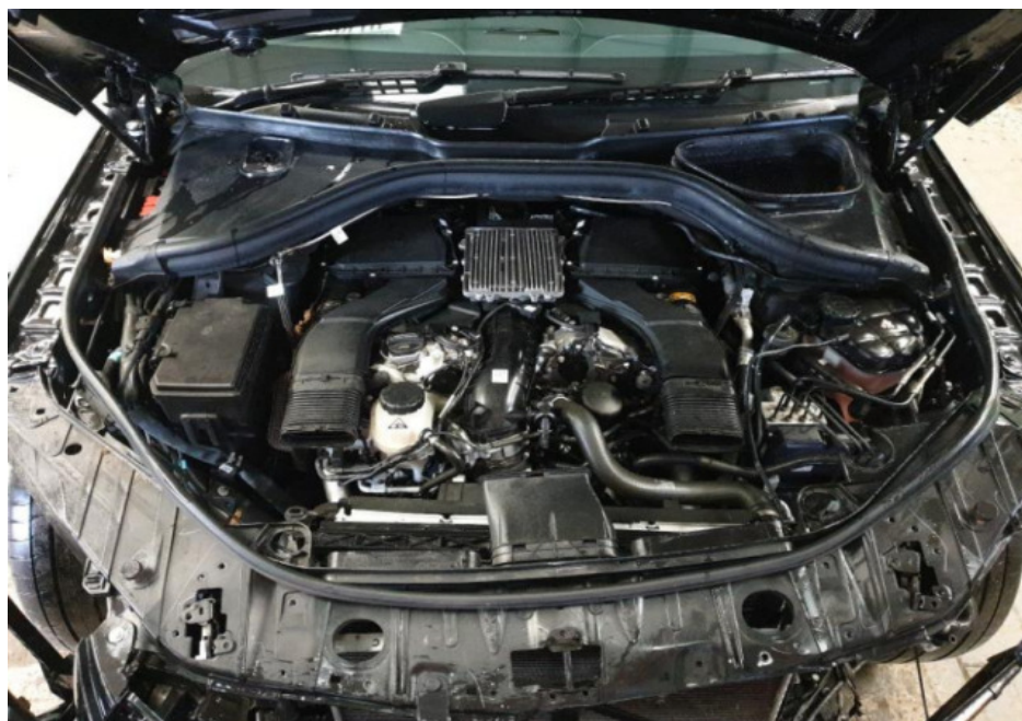
Photo 4 shows the engine compartment of the Motor Car (photograph provided to me). The front support panel and front support panel top cover were observed to be damaged however parts within the engine compartment were unaffected as seen from the photograph.
