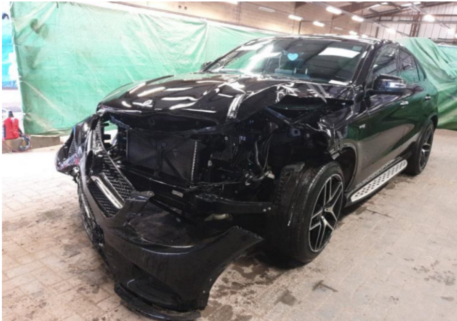
Photo 1 shows the front left body of the Motor Car (photograph provided to me). The Motor Car was observed to have sustained damage at its frontal portion. The front bumper, front bumper reinforcement, front left headlamp, front left fender, front left fender wheel arc garnish and front bonnet were amongst the parts that were observed to have been damaged.
