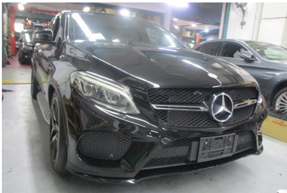
Photo 9 shows a general view of the front right body of the Motor Car at the time of my inspection. The Motor Car was observed to be in a relatively good general condition with no loose exterior fittings observed. The body parts at the frontal portion of the Motor Car were visually examined and it was observed that the repair/restoration works carried out to the damaged area of the Motor Car (refer to photograph 2 & 3 above) were reasonably adequate and in order.
