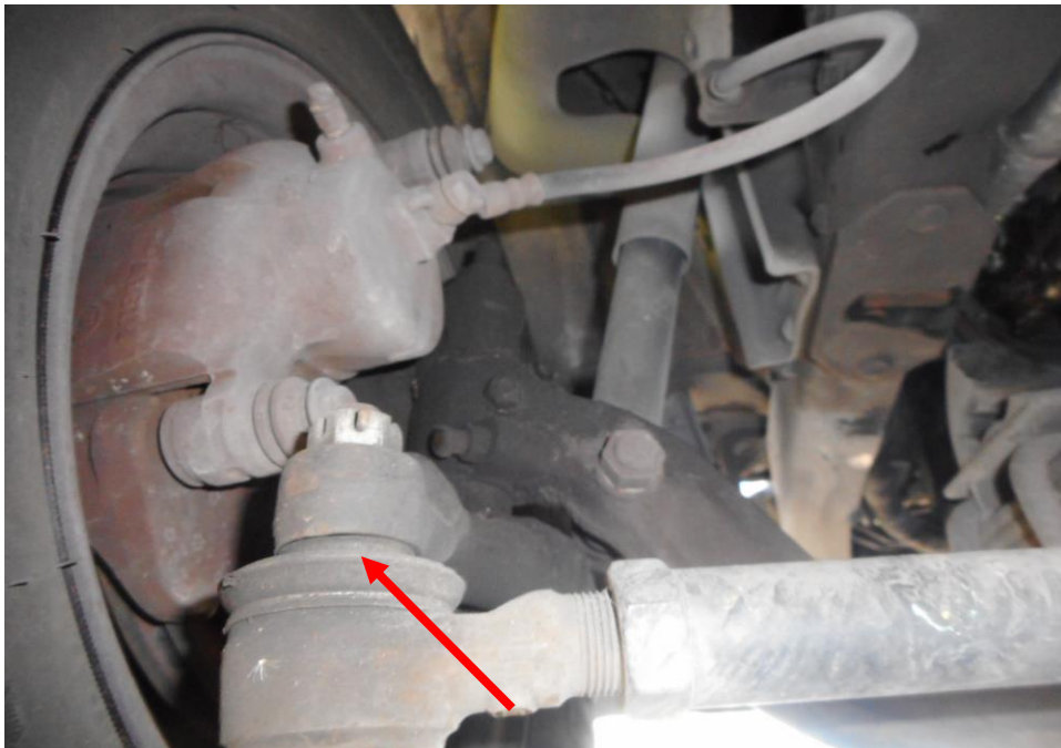
Photo 17 shows the various undercarriage components at the front left wheel of the Motor Lorry, in particular the steering tie rod end and ball joints (arrowed) were observed to be damaged.
