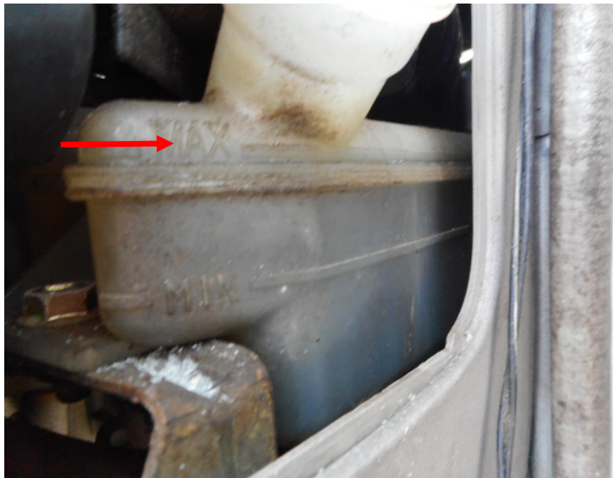
Photo 14 shows the brake fluid reservoir of the Motor Lorry at the time of our inspection. The brake fluid was observed to be of sufficient level and without any visible contamination (arrowed).
