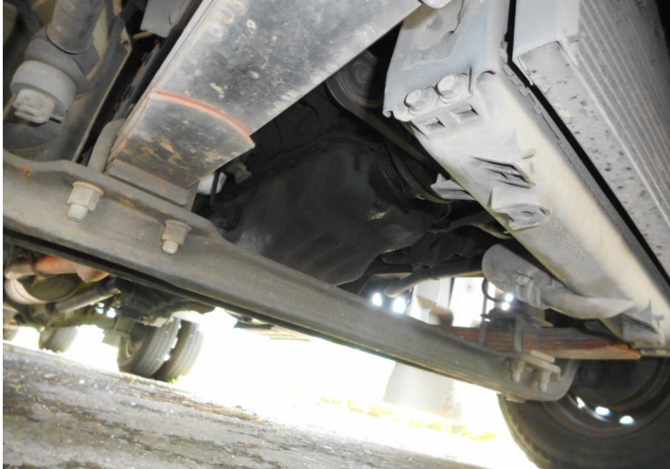
Photo 15 shows the undercarriage of the engine of the Motor Lorry at the time of our inspection. There was also sign(s) and indication(s) of old fluid stain within the engine undercarriage area.
