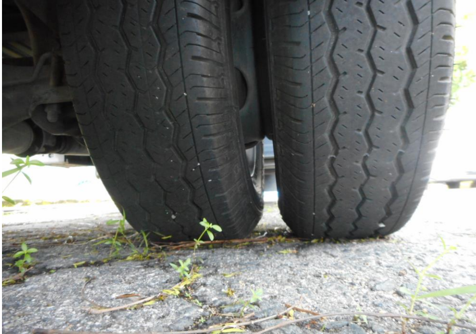
Photo 10 shows the condition of the rear right tyres of the Motor Lorry, which observed to be in serviceable condition with remaining tread depth of approximately 4.1mm. The tyres, which were wrapped around standard steel wheel rim, were also observed to be sufficiently inflated for vehicular operation.
