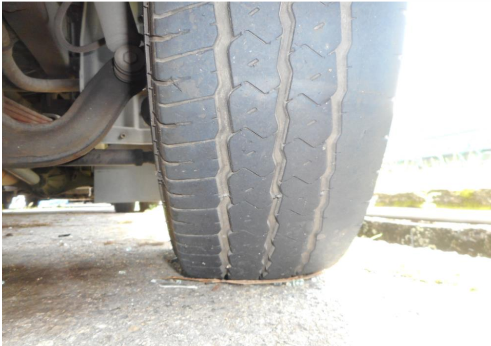
Photo 12 shows the condition of the front right tyre of the Motor Lorry, which was observed to be in serviceable condition with remaining tread depth of approximately 5.5mm. The tyre, which was wrapped around standard steel wheel rim, was also observed to be sufficiently inflated for vehicular operation.
