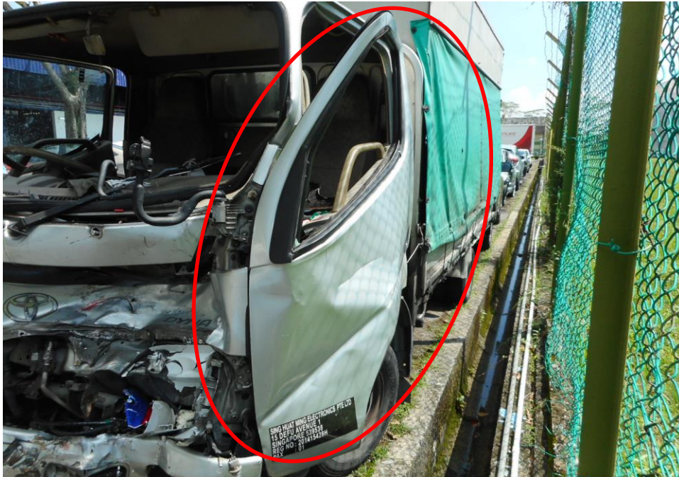
Photo 4 shows the close up view of the left door of the Motor Lorry at the time of our inspection. The Motor Lorry was observed to have sustained damages to its left door (circled) as a result of the accident.
