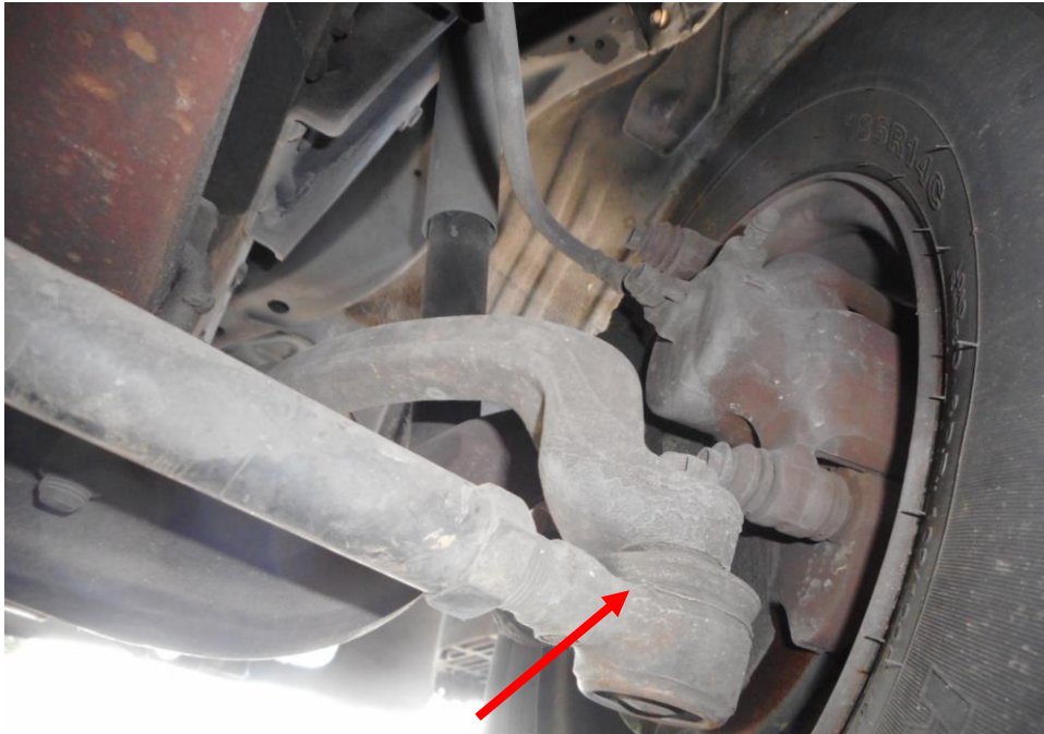
Photo 16 shows the various undercarriage components at the front right wheel of the Motor Lorry, in particular the steering tie rod end and ball joints (arrowed). The various undercarriage components of the Motor Lorry were all found to be intact without any visible damage. There was also no sign of fluid stain(s) observed on the various undercarriage components.
