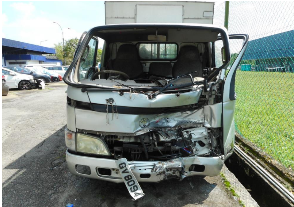
Photo 1 shows a general view of the front windscreen and body panel of the Motor Lorry at the time of our inspection. The Motor Lorry was observed sustained major damages to its frontal due to the accident.
