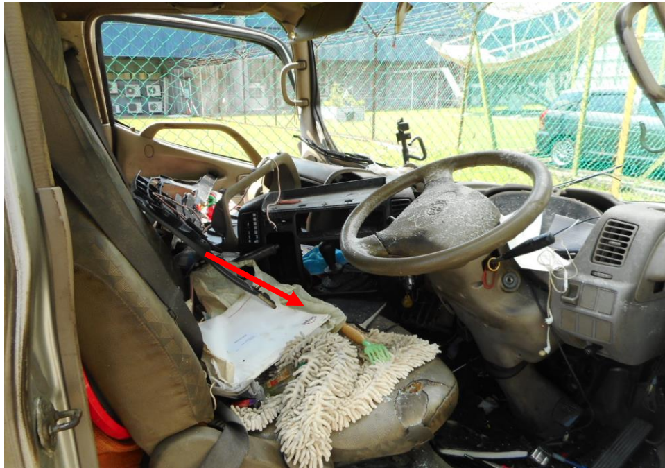
Photo 8 shows the close up view of the interior cabin of the Motor Lorry. It was observed to have sustained extensive induced damages to the dashboard as a result of the accident.
