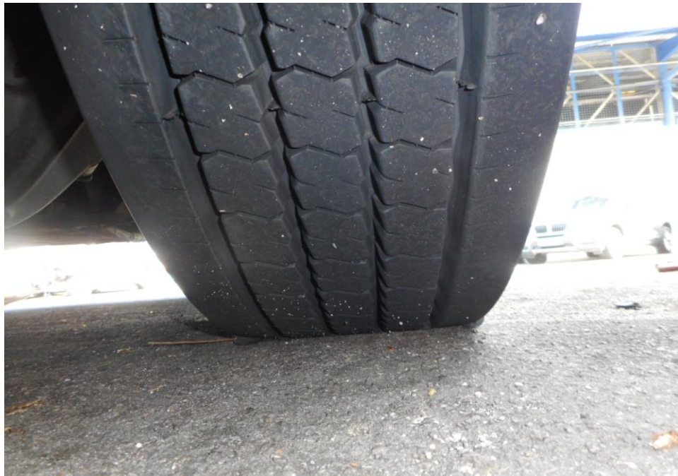
Photo 7 shows the condition of the front right tyre of the Motor Bus, which was observed to be in serviceable condition with remaining tread depth of approximately 12.2mm. The tyre, which was wrapped around standard steel wheel rim, was also observed to be sufficiently inflated for vehicular operation. There was no tear, cut or burst mark(s) on the outer and the inner sidewalls as well as across the tread of the 6 tyres that were fitted on the Motor Bus.
