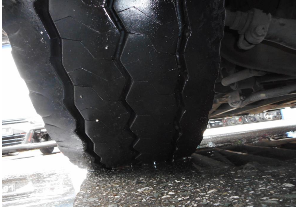
Photo 10 shows the condition of the front left tyres of the Motor Bus, which were observed to be in serviceable condition with remaining tread depth of approximately 13.8mm. There was also no tear, cut or burst mark(s) on the outer and the inner sidewalls as well as across the tread of the 6 tyres that were fitted on the Motor Bus.
