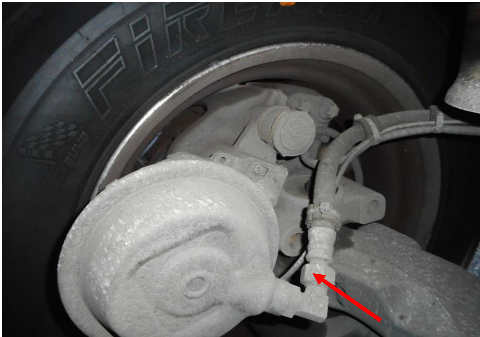
Photo 19 shows the brake pipe (arrowed) at the front left wheel of the Motor Bus. I did not observe any leakage of brake fluid at the time of my inspection of the Motor Bus. My static tests of the Motor Bus's braking system, along with my visual examination of the various mechanical components in the braking system had indicated that there was no internal leakage of pressure/vacuum. Hence the braking system of the Motor Bus was likely to be in serviceable condition at the material time of accident.
