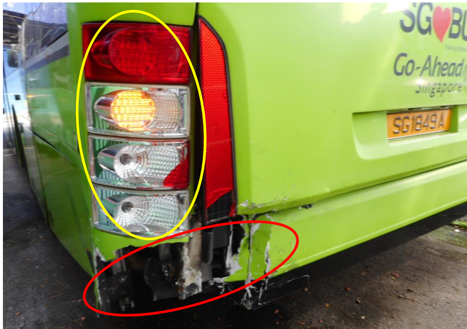
Photo 3 shows a close up view of the Motor Bus's rear body at the time of my inspection. It appeared to have sustained damage at its rear left portion. Its rear brake lamp (yellow circle) and rear body panel (red circle) were damage at the time of my inspection.
