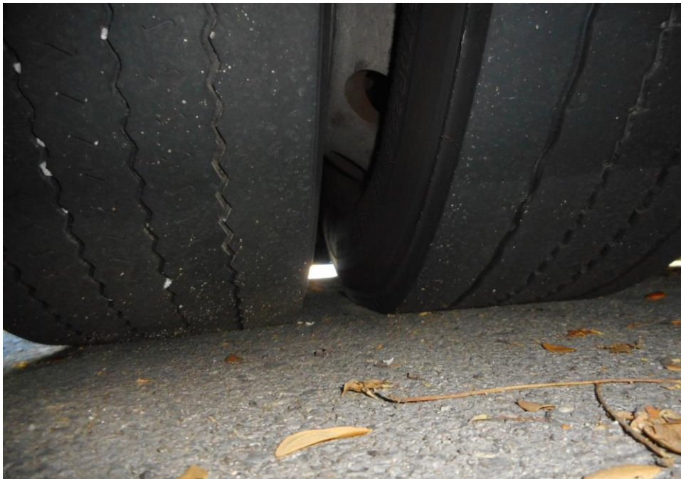
Photo 9 shows the condition of the rear left tyres of the Motor Bus, which was observed to be in serviceable condition with remaining tread depth of approximately 6.4mm. The tyres, which were wrapped around standard steel wheel rim, were also observed to be sufficiently inflated for vehicular operation. There was also no damage found on all 6 steel wheel rims of the Motor Bus.
