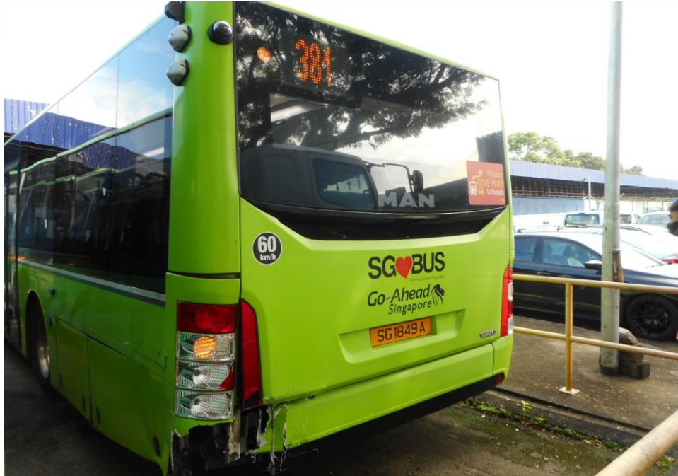
Photo 2 shows a general view of the Motor Bus's rear body at the time of my inspection. It appeared to have sustained damage at its rear left portion. Its rear brake lamp and rear body panel were damage at the time of my inspection.
