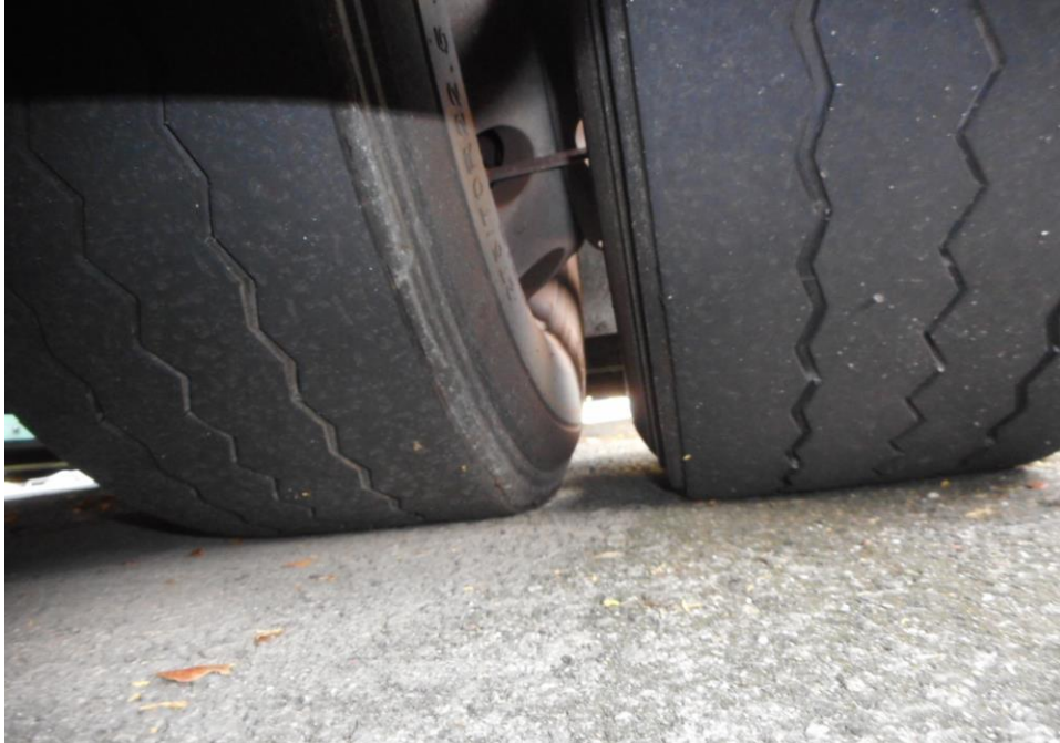
Photo 8 shows the condition of the rear right tyre of the Motor Bus, which was observed to be in serviceable condition with remaining tread depth of approximately 2.8mm. The tyre, which was wrapped around standard steel wheel rim, was also observed to be sufficiently inflated for vehicular operation.
