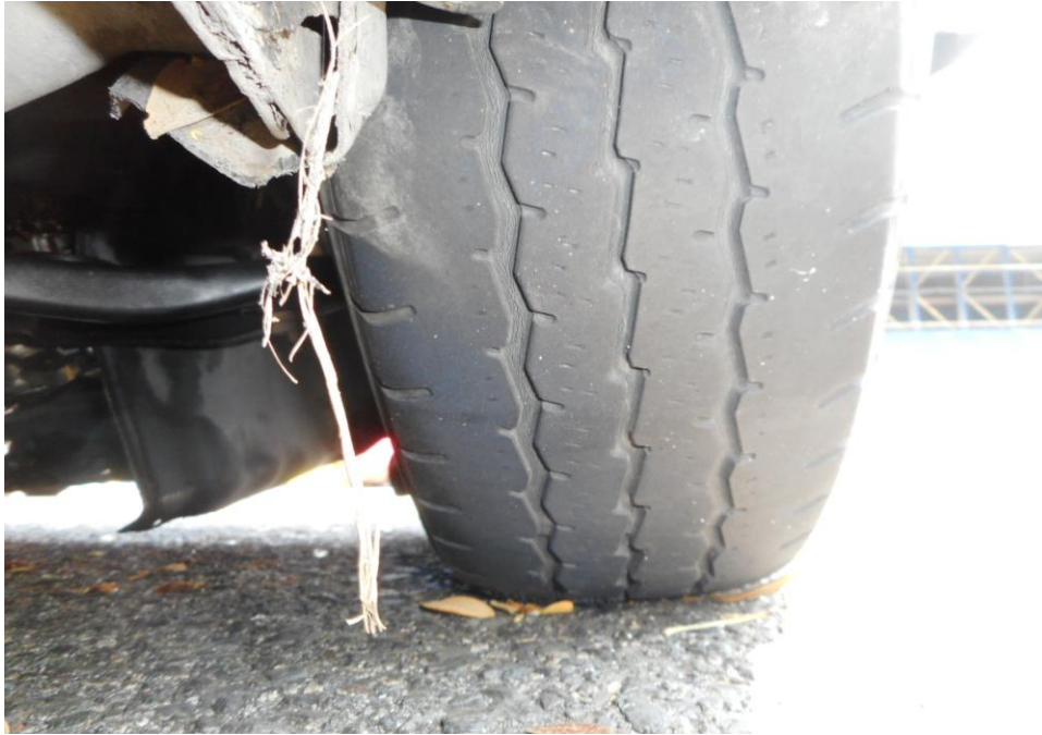
Photo 9 shows the condition of the front right tyre of the Motor Car, which was observed to be in serviceable condition with remaining tread depth of approximately 3.7mm. The tyre, which was wrapped around alloy wheel rim, was also observed to be sufficiently inflated for vehicular operation.
