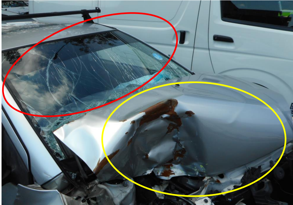
Photo 3 shows the close up view of the Motor Car's front body at the time of my inspection. The Motor car was observed to have sustained damage at its front portion. Its front windscreen (red circle) and front bonnet (red circle) was damaged as a result of the accident.
