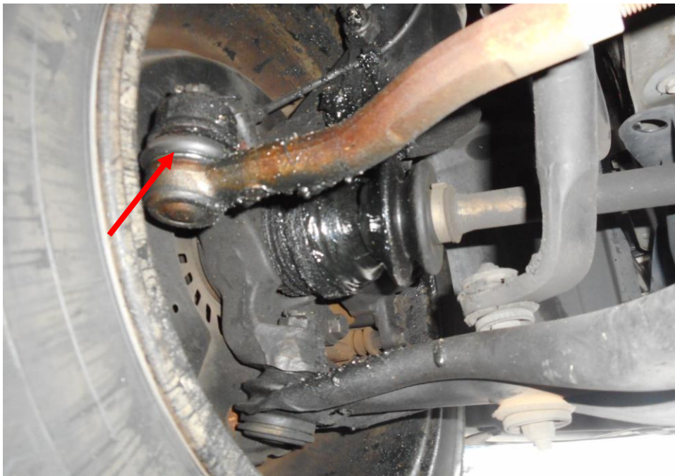
Photo 19 shows the various undercarriage components at the front left wheel of the Motor Car, in particular the steering tie rod end (arrowed). The various Undercarriage components of the Motor Car were all found to be intact without any visible damage. There was also no sign of fluid stain(s) observed on the various undercarriage components. However, observed was old grease stains around the surroundings.
