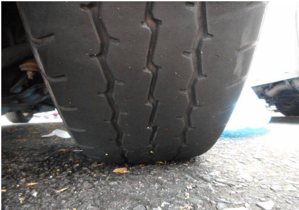
Photo 12 shows the condition of the front left tyre of the Motor Car, which was observed to be in serviceable condition with remaining tread depth of approximately 2.8mm. The tyre was also observed to be sufficiently inflated for vehicular operation with no tear, cut or burst mark(s).
