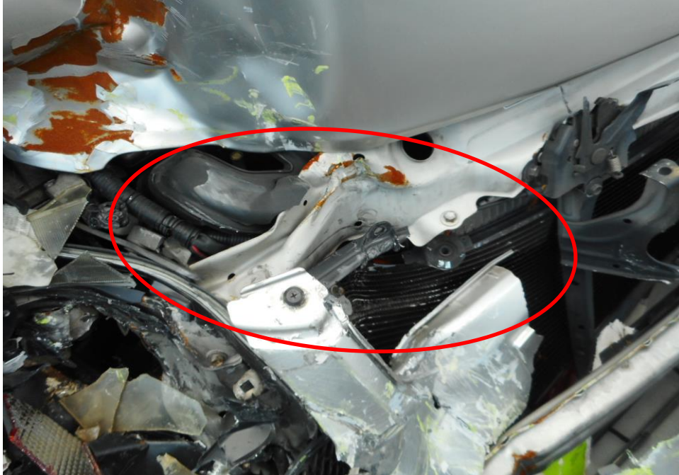
Photo 5 shows the close up view of the Motor Car's front body at the time of my inspection. The Motor car was observed to have sustained damage at its front portion. Its engine (circled) was damaged as a result of the accident.
