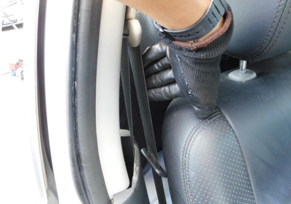
Photo 21 shows that the seat belt on the right seat was not worn at the material time of accident as the safety pre-tensioners was activated at the moment of impact and caused the seat belt to be locked into the last position.
