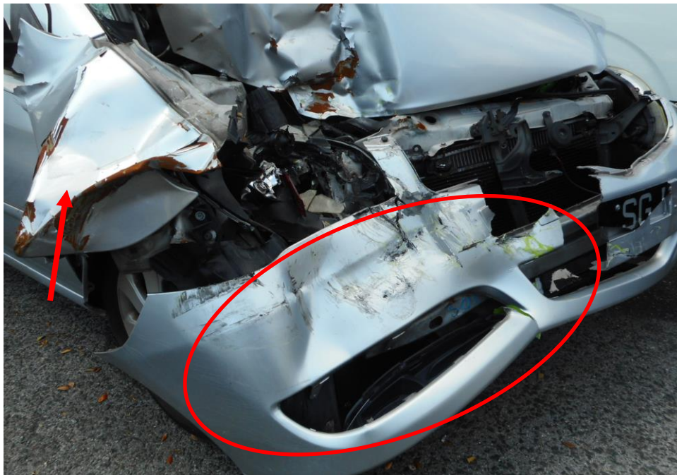
Photo 4 shows the close up view of the Motor Car's front body at the time of my inspection. The Motor car was observed to have sustained damage at its front portion. Its front bumper (circled) and front right fender (arrowed) was amongst the body parts and various components in the engine compartments were also damaged as a result of the accident.
