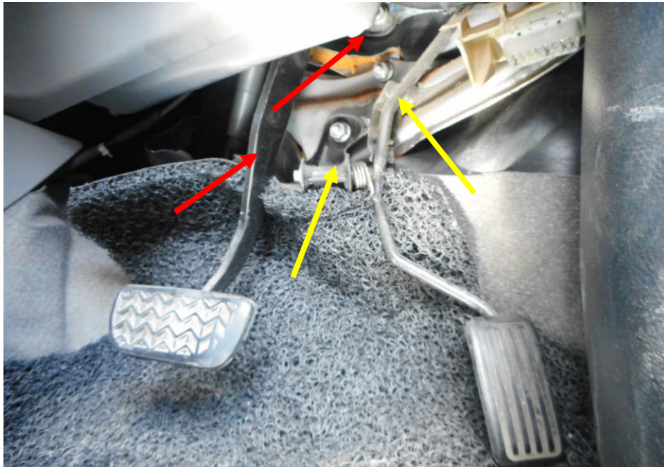
Photo 20 shows the close up view of the Motor Car's brake pedal and brake booster at the time of my inspection. Its brake pedal, brake pedal (red arrowed) and accelerator pedal (yellow arrow) was observed to be damaged as a result of the induced impact from the accident.
