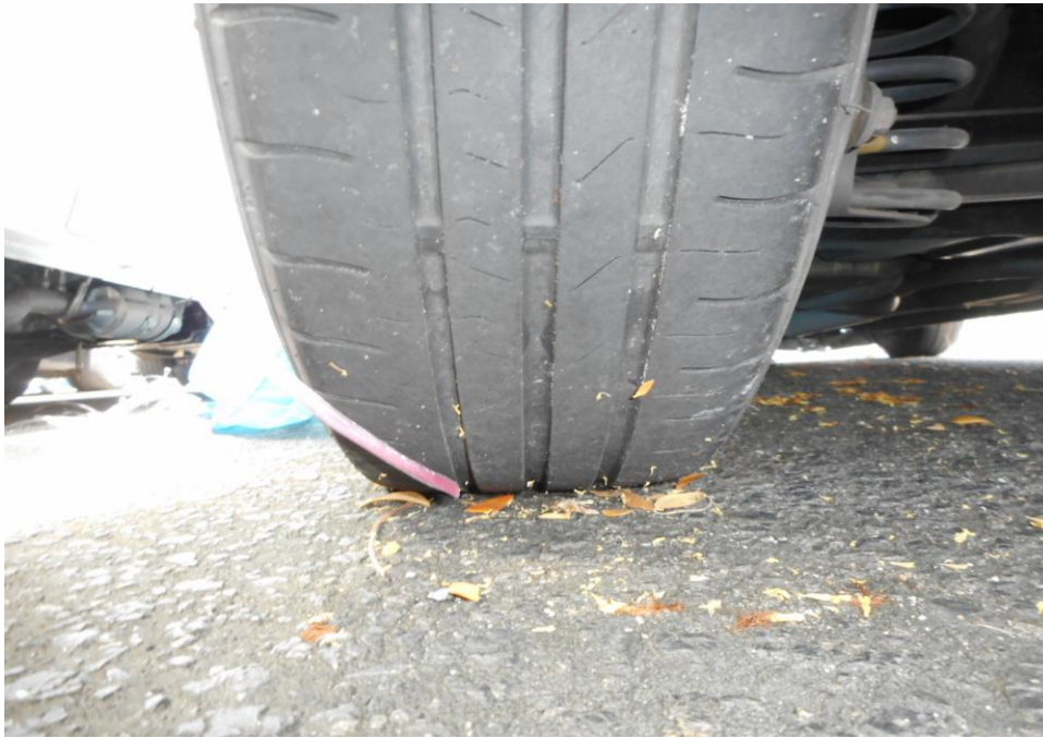
Photo 11 shows the condition of the rear left tyre of the Motor Car, which was observed to be in serviceable condition with remaining tread depth of approximately 3.8mm. The tyre was also observed to be sufficiently inflated for vehicular operation with no tear, cut or burst mark(s).
