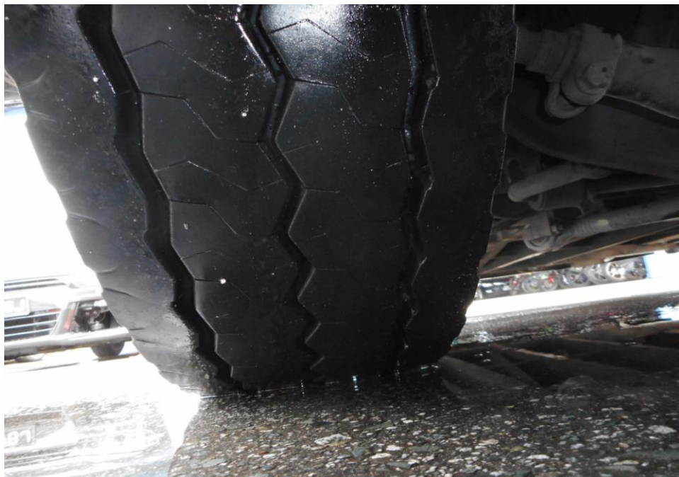
Photo 9 shows the condition of the front left tyres of the Motor Bus, which were observed to be in serviceable condition with remaining tread depth of approximately 13mm. There was also no tear, cut or burst mark(s) on the outer and the inner sidewalls as well as across the tread of the 6 tyres that were fitted on the Motor Bus.
