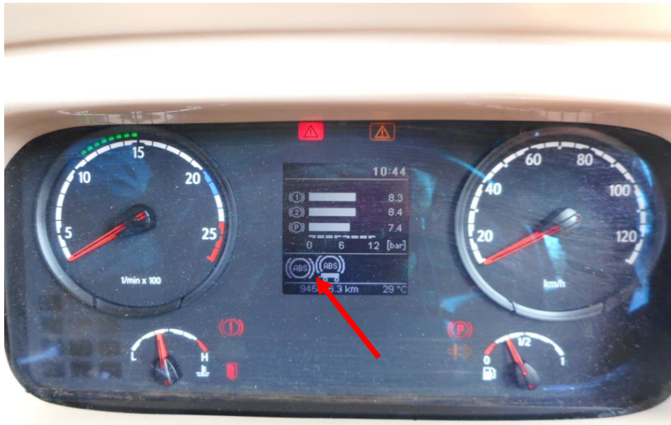
Photo 24 shows the warning light for Anti-Lock Brake System (ABS) appearing on the instrument panel of the Motor Bus during the self-test of its various electronic operating systems when its engine was cranked.
