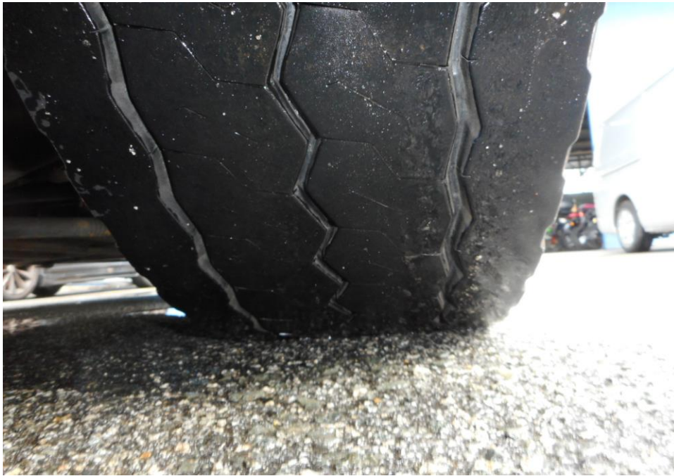
Photo 6 shows the condition of the front right tyre of the Motor Bus, which was observed to be in serviceable condition with remaining tread depth of approximately 9.9mm. The tyre, which was wrapped around standard steel wheel rim, was also observed to be sufficiently inflated for vehicular operation. There was no tear, cut or burst mark(s) on the outer and the inner sidewalls as well as across the tread of the 6 tyres that were fitted on the Motor Bus.
