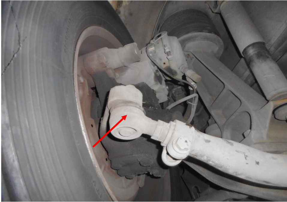
Photo 20 shows the various undercarriage components at the front left wheel of the Motor Bus, in particular the steering tie rod end (arrowed). The various undercarriage components of the Motor Bus were all found to be intact without any visible damage. There was also no sign of fluid stain(s) observed on the various undercarriage components.
