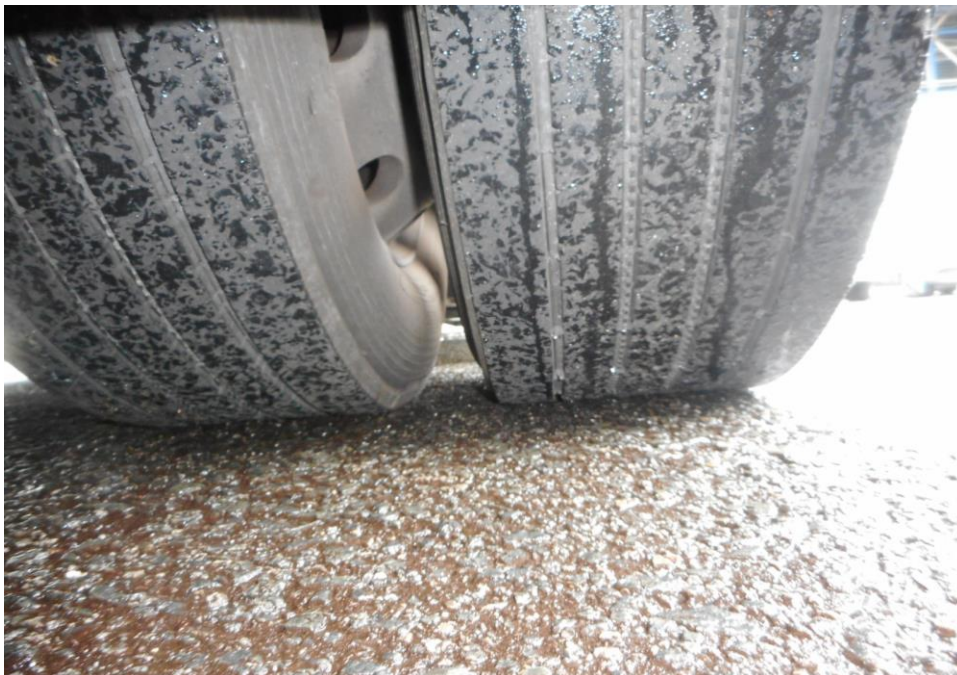
Photo 7 shows the condition of the rear right tyre of the Motor Bus, which was observed to be in serviceable condition with remaining tread depth of approximately 6.5mm. The tyre, which was wrapped around standard steel wheel rim, was also observed to be sufficiently inflated for vehicular operation.
