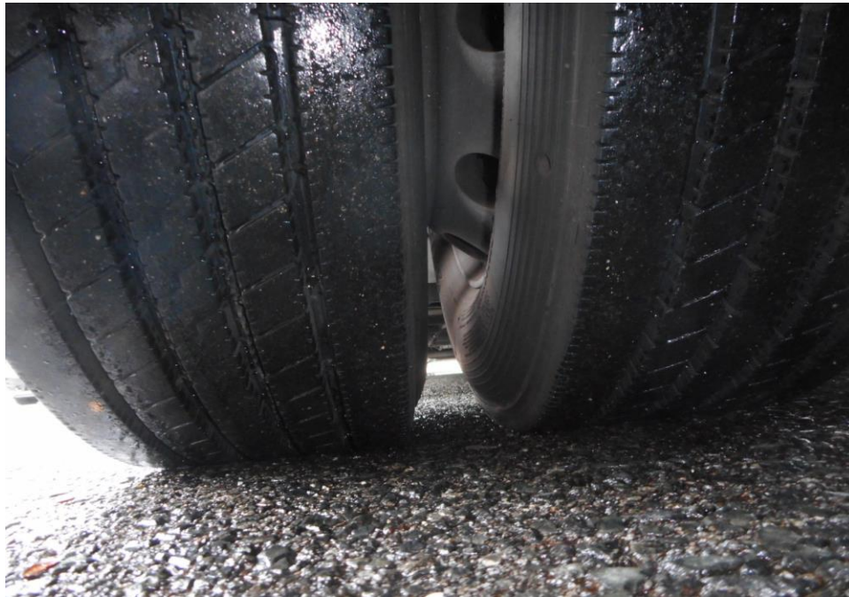
Photo 8 shows the condition of the rear left tyres of the Motor Bus, which was observed to be in serviceable condition with remaining tread depth of approximately 13.8mm. The tyres, which were wrapped around standard steel wheel rim, were also observed to be sufficiently inflated for vehicular operation. There was also no damage found on all 6 steel wheel rims of the Motor Bus.
