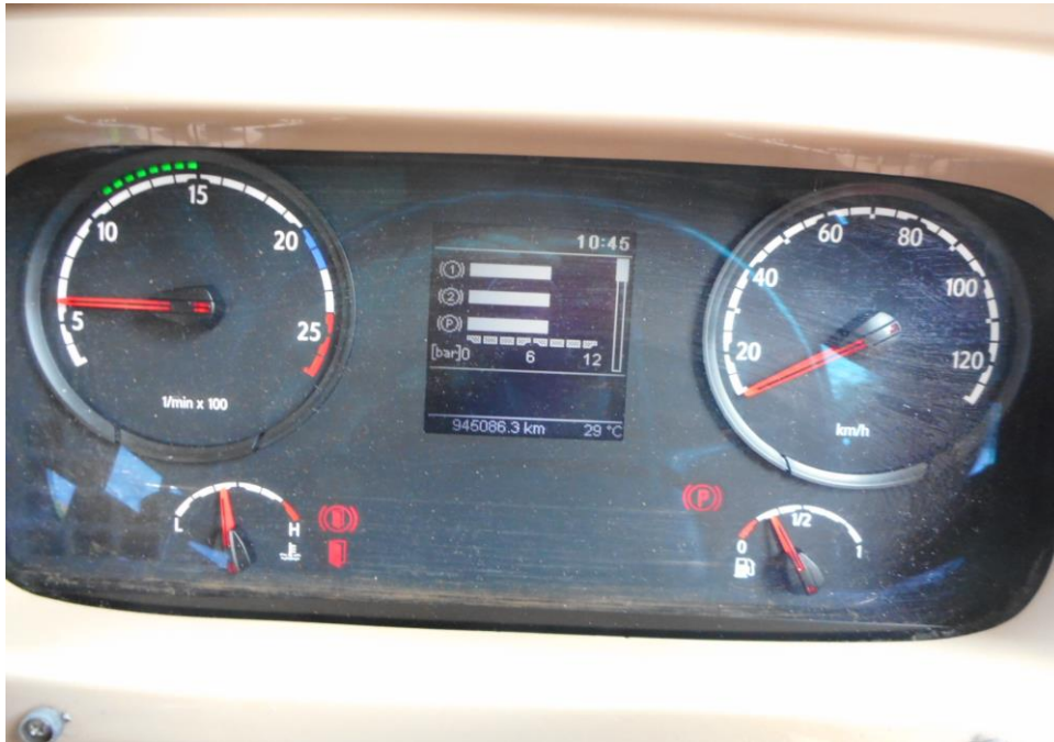
Photo 25 shows no warning lights illuminated on the instrument panel of the Motor Bus after the engine was cranked. This would suggest that there was no abnormality to the various electronic operating systems of the Motor Bus, like the ABS
