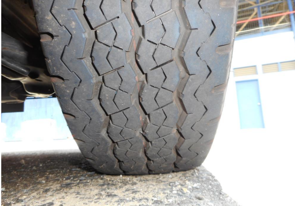
Photo 6 shows the condition of the front right tyre of the Motor Lorry, which was observed to be in serviceable condition with remaining tread depth of approximately 7.2mm. The tyre, which was wrapped around standard steel wheel rim, was also observed to be sufficiently inflated for vehicular operation. There was no tear, cut or burst mark(s) on the outer and the inner sidewalls as well as across the tread of the 4 tyres that were fitted on the Motor Lorry.
