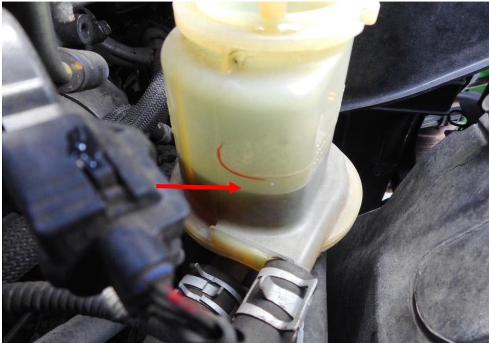
Photo 14 shows the power steering fluid reservoir of the Motor Lorry at the time of my inspection. The power steering fluid was observed to be of sufficient level (arrowed) and without any visible contamination.
