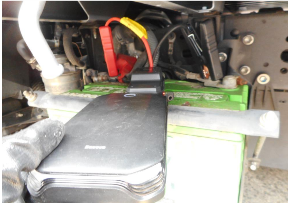
Photo 16 shows the jumpstarting process of the Motor Lorry's engine. The engine of the Motor Lorry was unable to be jumpstarted up despite multiple attempts in starting it.
