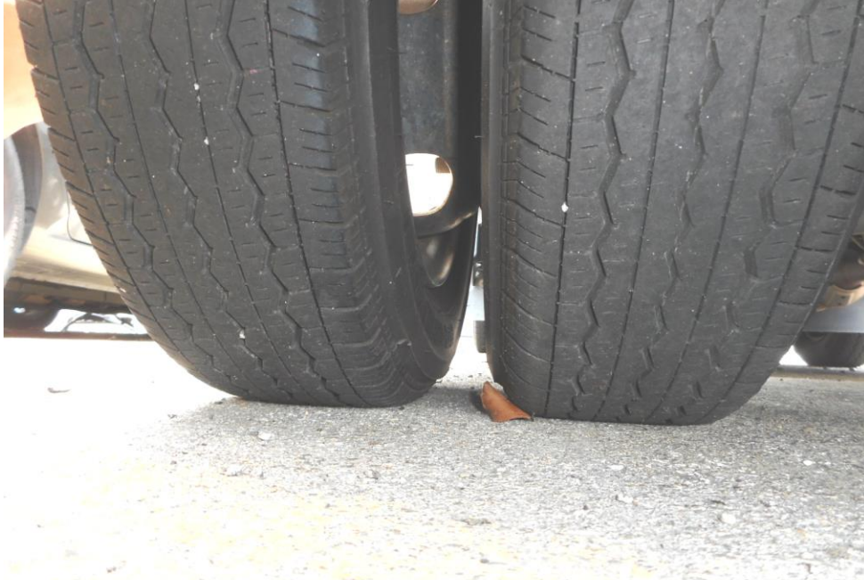
Photo 8 shows the condition of the rear left tyres of the Motor Lorry, which was observed to be in serviceable condition with remaining tread depth of approximately 3.3mm. The tyres, which were wrapped around standard steel wheel rim, were also observed to be sufficiently inflated for vehicular operation. There was also no damage found on all 4 steel wheel rims of the Motor Lorry.
