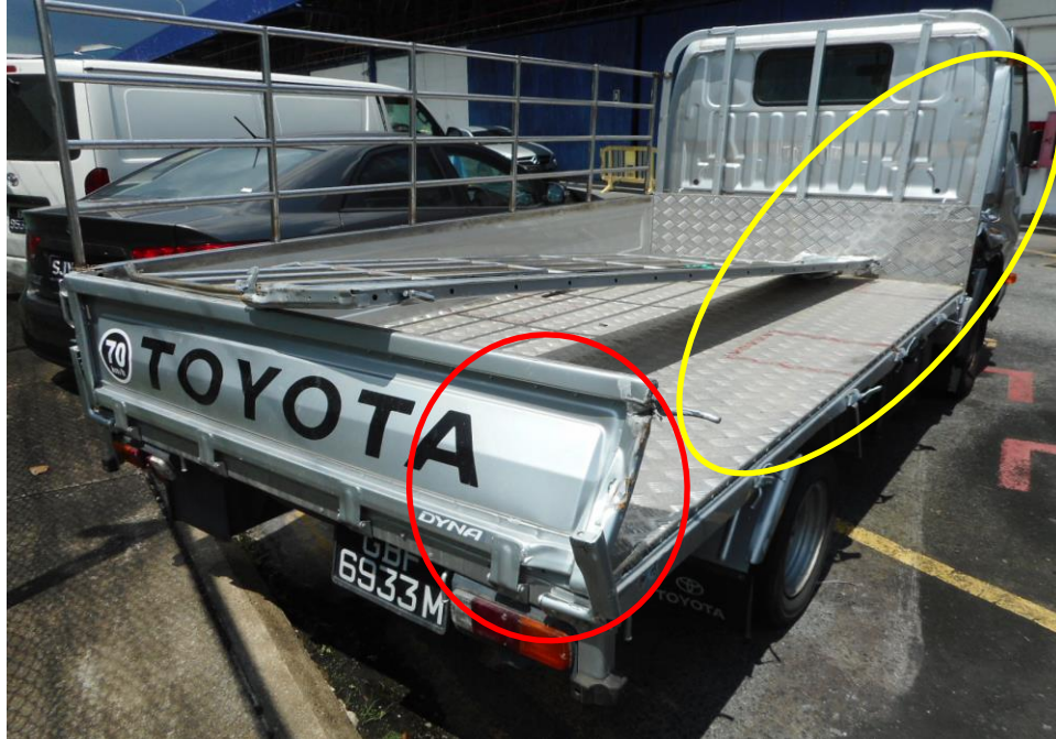
Photo 4 shows close up view of the Motor Lorry's right and rear portion at the time of my inspection. It appeared to have sustained damage at its left portion. Its rear body panel (red circle) and right body panel (yellow circle) were damaged at the time of my inspection as result of the accident.
