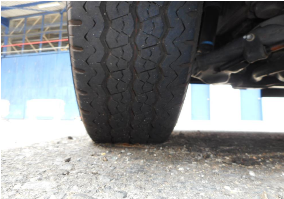
Photo 9 shows the condition of the rear right tyres of the Motor Lorry, which were observed to be in serviceable condition with remaining, tread depth of approximately 7.2mm. There was also no tear, cut or burst mark(s) on the outer and the inner sidewalls as well as across the tread of the 4 tyres that were fitted on the Motor Lorry.
