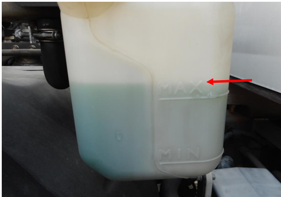
Photo 16 shows the engine coolant reservoir of the Motor Lorry at the time of my inspection. The engine coolant was observed to be of sufficient level (arrowed) and without any visible contamination.
