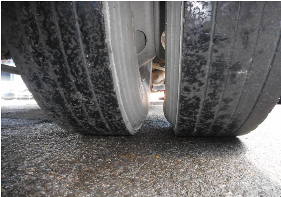
Photo 11 shows the condition of the rear right tyre of the Motor Lorry, which was observed to be in serviceable condition with remaining tread depth of approximately 2.7mm. The tyre, which was wrapped around standard steel wheel rim, it was observed to be sufficiently inflated for vehicular operation.
