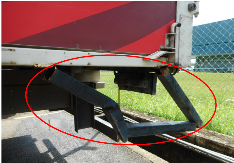
Photo 7 shows a close up view of the Motor Lorry's left portion at the time of my inspection. It appeared to have sustained damage at its left portion. Its left body panel (circled) was damage at the time of my inspection as a result of the accident.
