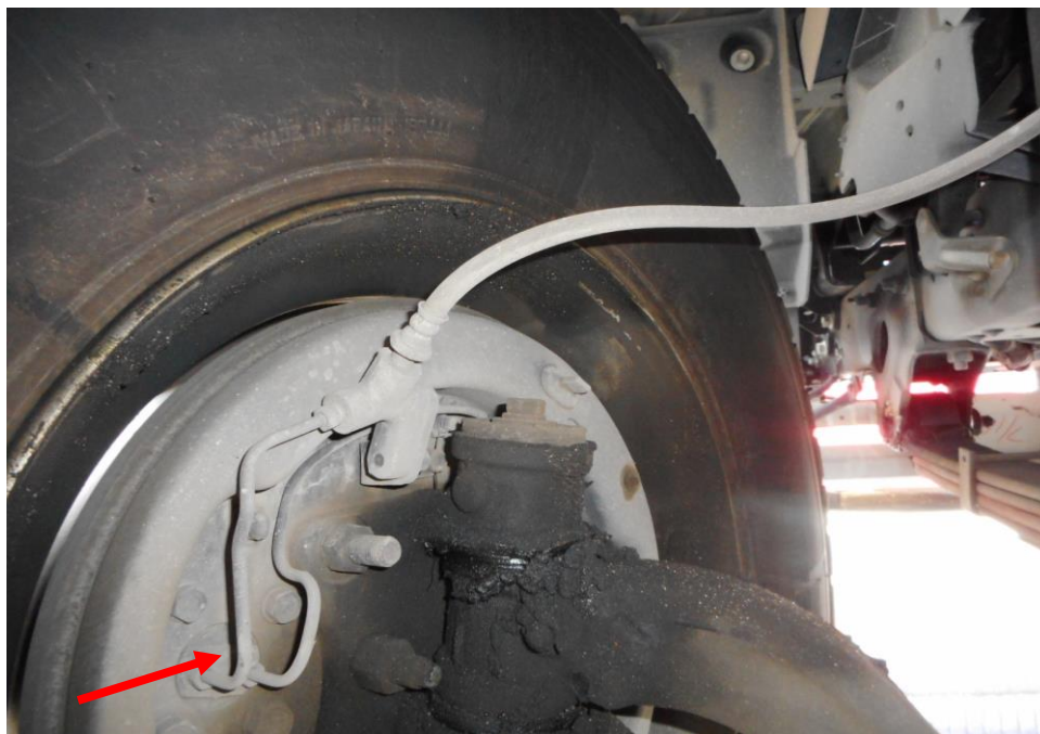
Photo 25 shows the brake hose/pipe (arrowed) at the front left wheel of the Motor Lorry. My static tests of the Motor Bus's braking system, along with my visual examination of the various mechanical components in the braking system had indicated that there was no internal leakage of pressure/vacuum. Hence the braking system of the Motor Bus was likely to be in serviceable condition at the material time of accident.
