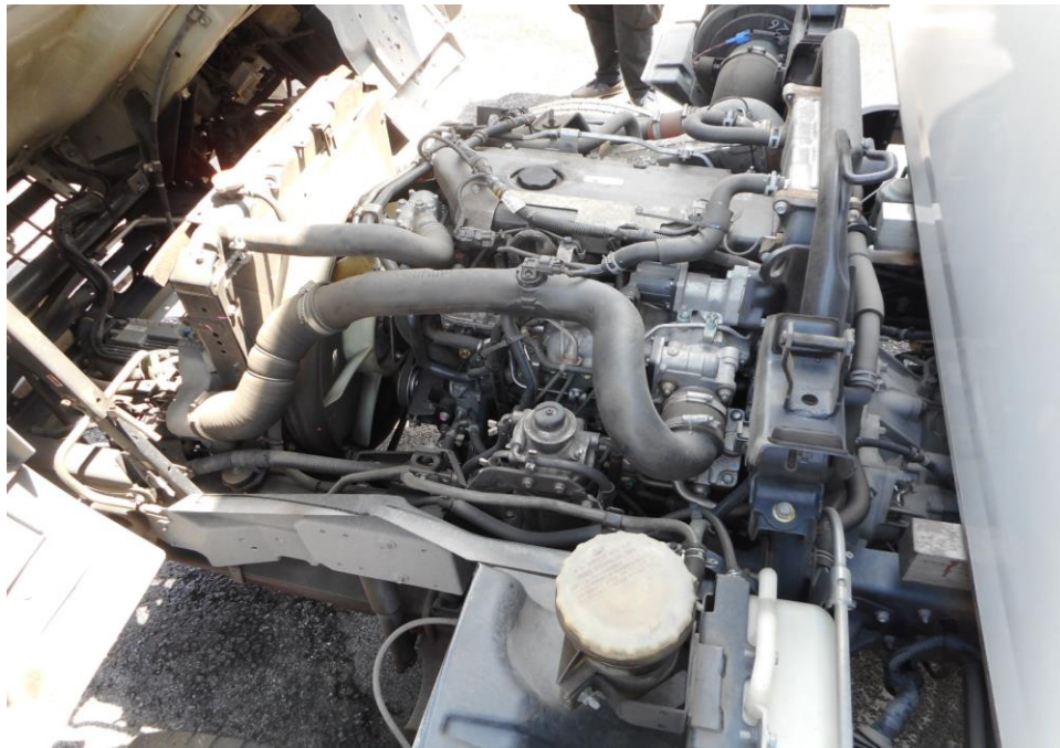
Photo 14 shows a general view of the Motor Lorry's engine compartment, which was accessed by lifting the front cabin of the Motor Lorry. The various parts and components inside the engine compartment were unaffected by the accident. There was also no sign(s) or indication(s) of fresh fluid leakage and/or fluid stain within the engine compartment
