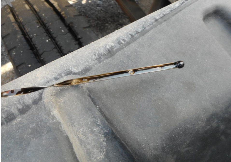
Photo 17 shows the engine oil dip stick of the Motor Lorry at the time of my inspection. The engine oil was observed to be of sufficient level and without any visible contamination.
