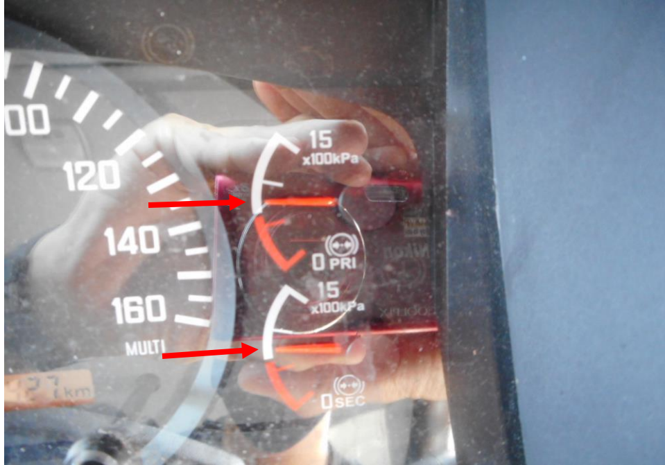
Photo 15 shows the air in the air brake cylinder of the Motor Bus at the time of my inspection. The air in the cylinder was observed to be of sufficient level & serviceable at the time of the accident.
