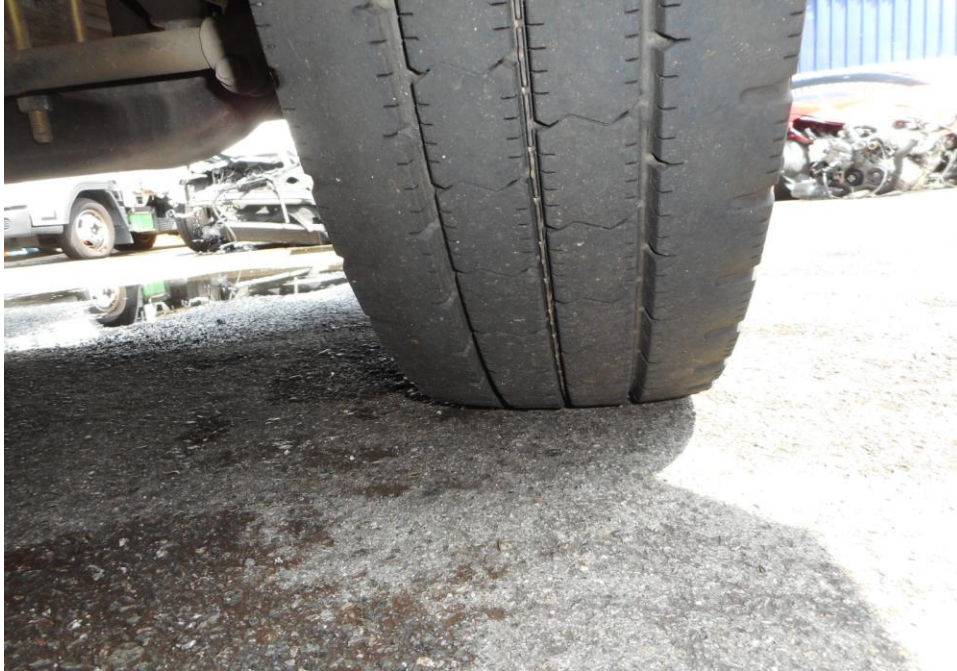
Photo 10 shows the condition of the front right tyre of the Motor Lorry, which was observed to be in serviceable condition with remaining tread depth of approximately 7.2mm. The tyre, which was wrapped around standard steel wheel rim, was also observed to be sufficiently inflated for vehicular operation. There was no tear, cut or burst mark(s) on the outer and the inner sidewalls as well as across the tread of the 6 tyres that were fitted on the Motor Lorry.
