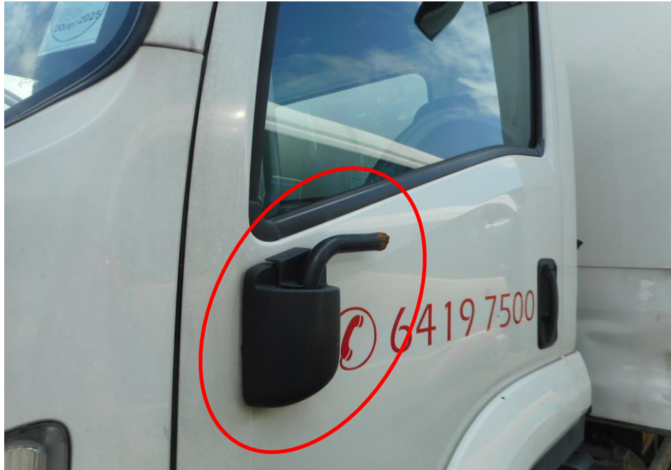
Photo 4 shows a close up view of the Motor Lorry's left portion at the time of my inspection. It appeared to have sustained damage at its left portion. Its left rear view mirror (red circle) was damage at the time of my inspection as a result of the accident.
