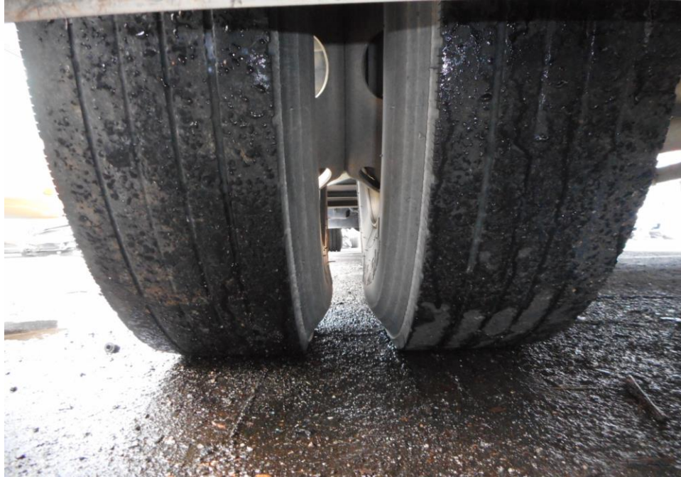
Photo 12 shows the condition of the rear left tyres of the Motor Lorry, which was observed to be in serviceable condition with remaining tread depth of approximately 1.7mm. The tyres, which were wrapped around standard steel wheel rim, were also observed to be sufficiently inflated for vehicular operation. There was also no damage found on all 6 steel wheel rims of the Motor Lorry.
