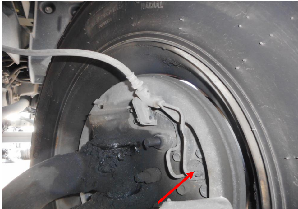
Photo 24 shows the brake hose/pipe (arrowed) at the front right wheel of the Motor Lorry. My static tests of the Motor Bus's braking system, along with my visual examination of the various mechanical components in the braking system had indicated that there was no internal leakage of pressure/vacuum. Hence the braking system of the Motor Bus was likely to be in serviceable condition at the material time of accident.
