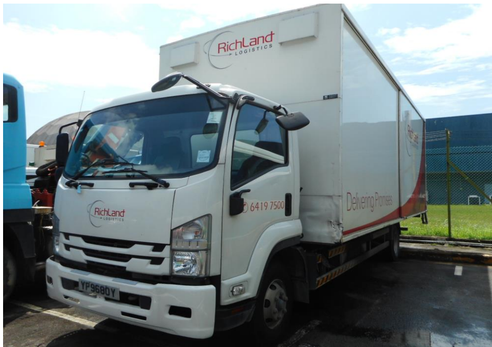
Photo 3 shows a general view of the Motor Lorry's left portion at the time of my inspection. It appeared to have sustained damage at its left portion. Its left rear view mirror and left body panels was damage at the time of my inspection.
