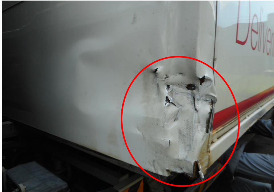
Photo 6 shows a close up view of the Motor Lorry's left portion at the time of my inspection. It appeared to have sustained damage at its left portion. Its left body panel (circled) was damage at the time of my inspection as a result of the accident.
