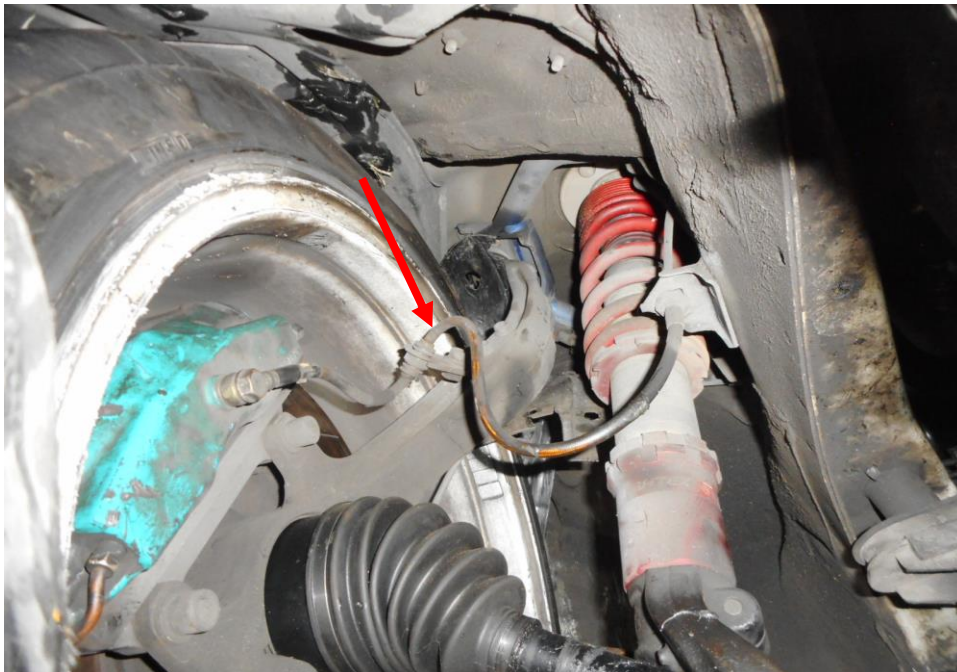
Photo 25 shows the brake hose/pipe (arrowed) at the front right wheel of the Motor Car. I did not observe any leakage of brake fluid at the time of my inspection of the Motor Car. Static tests of the Motor Car's braking system had indicated that there was no internal leakage of pressure/vacuum. The undercarriage components of the Motor Car were also all found to be intact and without any visible damage.
