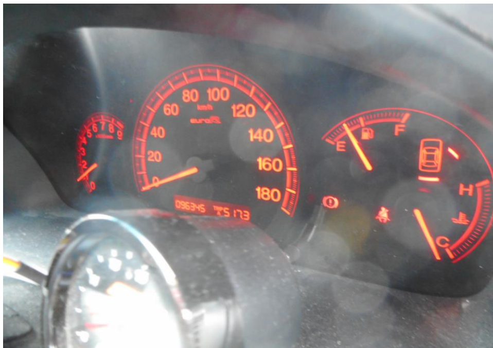
Photo 32 shows no warning lights illuminated on the instrument panel of the Motor Car after the engine was cranked. This would suggest that there was no abnormality to the electronic operating system of the Motor Car, like the ABS, EPS and etc.
