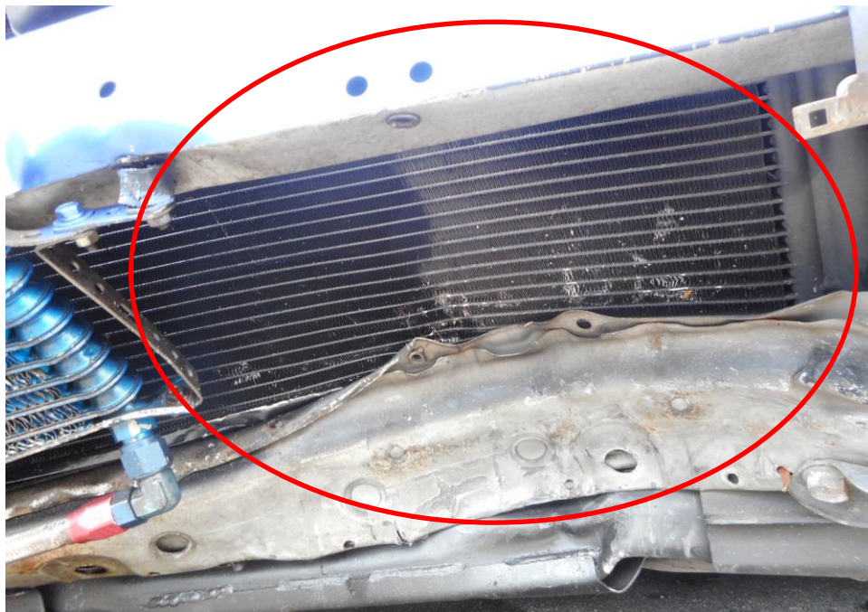
Photo 9 shows the close up view of the Motor Car's front engine at the time of my inspection. The Motor Car was observed to have sustained damage at its engine coolant radiator (circled) as a result of the accident.
