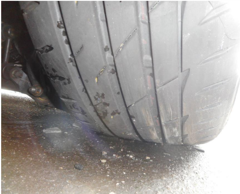
Photo 14 shows the condition of the front right tyre of the Motor Car, which was observed to be in serviceable condition with remaining tread depth of approximately 6.4mm. The tyre was sufficiently inflated for vehicular operation with no tear, cut or burst mark(s) on the outer and the inner sidewalls as well as across the tread. The 4 tyres of the Motor Car were wrapped around alloy wheel rims without any damage.
