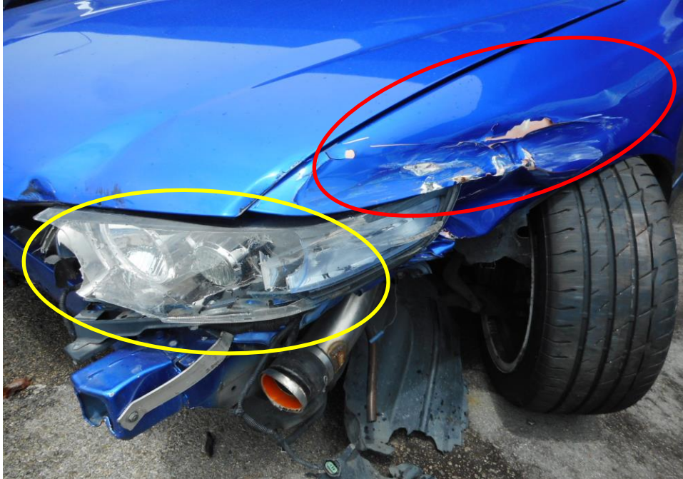
Photo 4 shows the close up view of the Motor Car's front body at the time of my inspection. The Motor Car was observed to have sustained damage at its front left fender (red circle) and front left headlamp (yellow circle) as a result of the accident.
