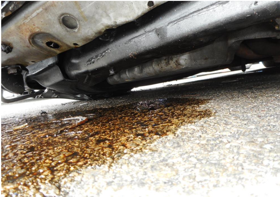
Photo 22 shows the undercarriage of the Motor Car, at the area where the engine housing and transmission housing are located. I did observed fluid leak) on the underside of the Motor Car, this leakage came from the damaged engine oil cooler as a result of the accident.
