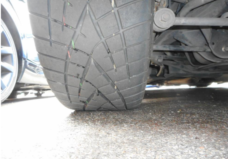
Photo 16 shows the condition of the rear left tyre of the Motor Car, which was observed to be in serviceable condition with remaining tread depth of approximately 4.9mm. The tyre, which was wrapped around alloy wheel rim, was also observed to be sufficiently inflated for vehicular operation. The 4 tyres of the Motor Car were wrapped around standard steel wheel rims.
