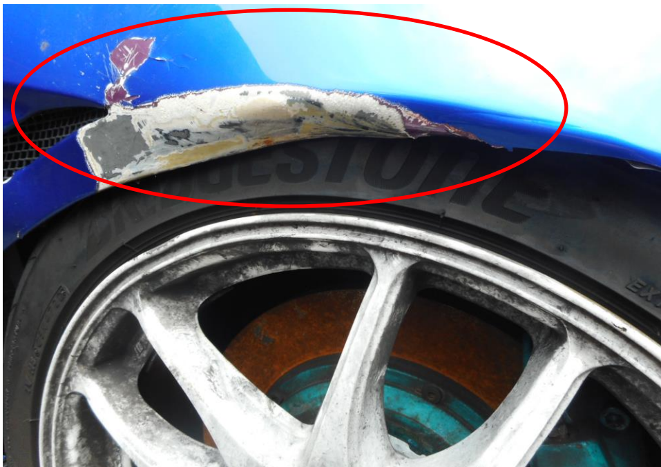
Photo 7 shows the close up view of the Motor Car's front body at the time of my inspection. The Motor Car was observed to have sustained damage at its front right fender (circled) as a result of the accident.
