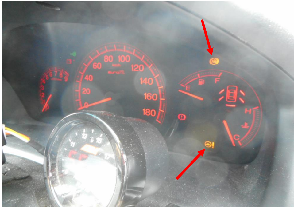
Photo 31 shows the warning light for Anti-Lock Brake System (ABS) and Electric Power Steering System (EPS) (arrowed) appearing on the instrument panel of the Motor Car during the self-test of its various electronic operating systems when its engine was cranked.
