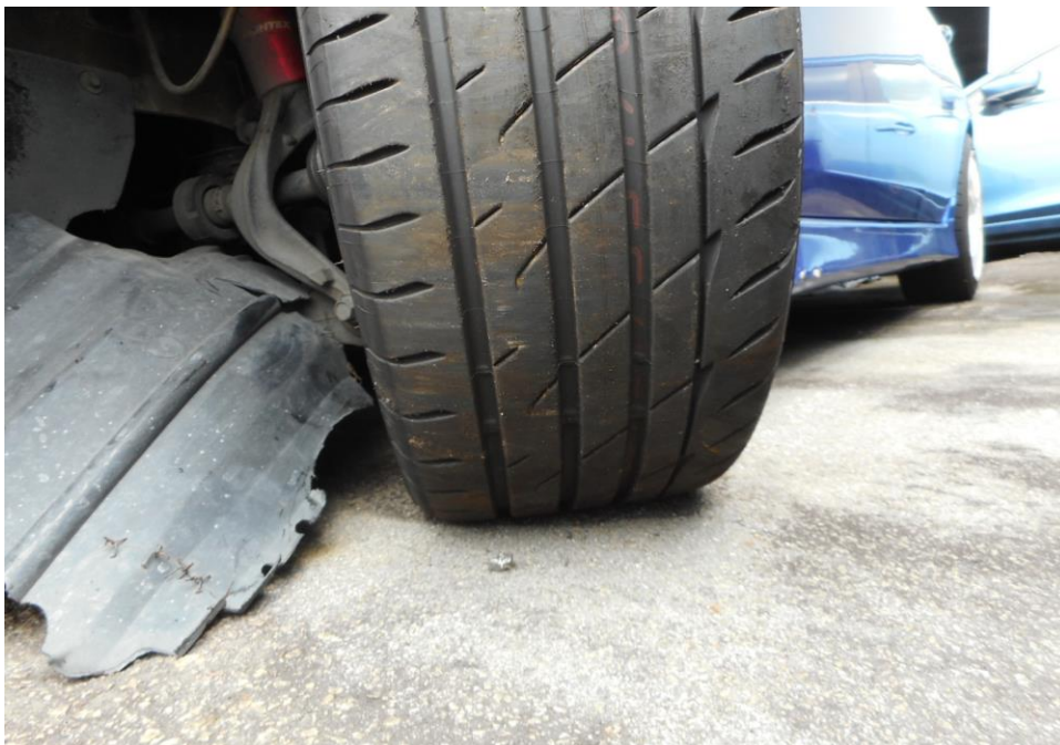
Photo 17 shows the condition of the front left tyre of the Motor Car, which was observed to be in serviceable condition with remaining tread depth of approximately 6.7mm. There was also no tear, cut or burst mark(s) on the outer and the inner sidewalls as well as across the tread of the Motor Car's 4 tyres.
