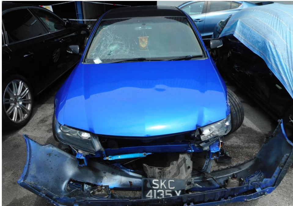
Photo 2 shows a general view of the Motor Car's front body at the time of my inspection. The front windscreen, front bumper, front left headlamp, front left and right fender was the body parts and various engine components that were damaged as a result of the accident.
