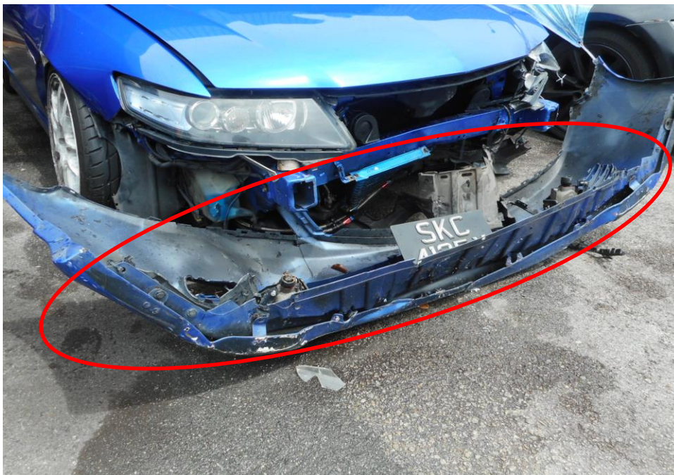
Photo 5 shows the close up view of the Motor Car's front body at the time of my inspection. The Motor Car was observed to have sustained damage at its front bumper (circled) as a result of the accident.
