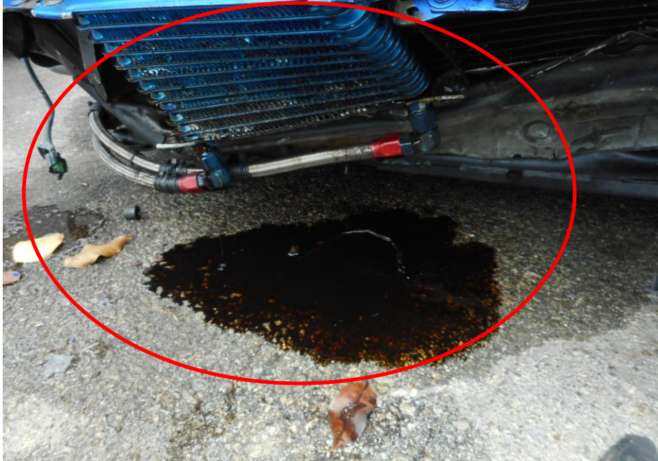
Photo 10 shows the close up view of the Motor Car's front engine at the time of my inspection. The Motor Car was observed to have sustained damage at its engine oil cooler (circled) and there was engine oil leakage as a result of the accident.
