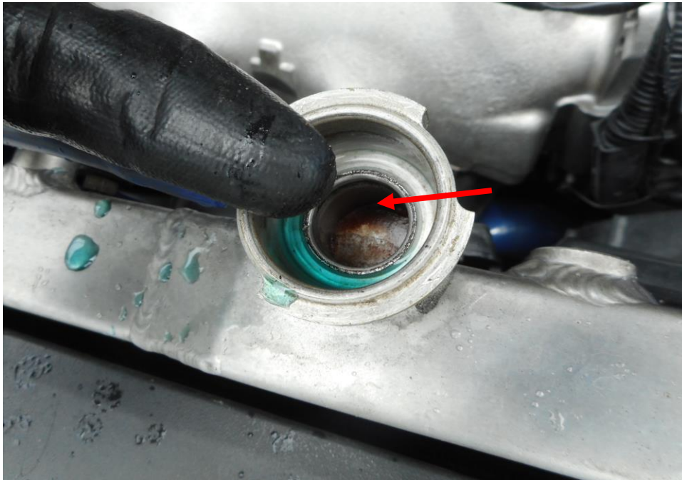
Photo 20 shows checks being carried out to the engine coolant of the Motor Car at the time of my inspection. The engine coolant was observed to be of insufficient level (arrowed) as there was a leakage from the damaged engine coolant radiator.
