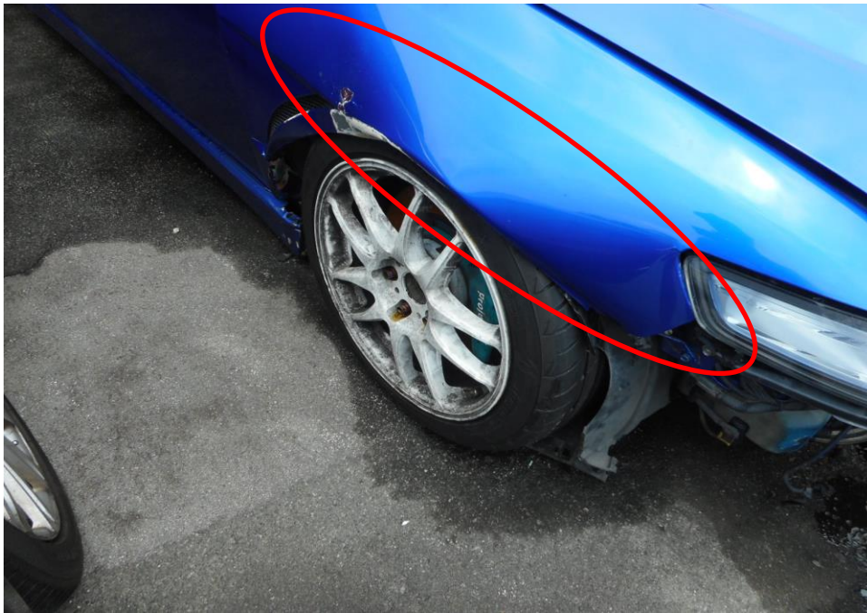
Photo 6 shows the close up view of the Motor Car's front body at the time of my inspection. The Motor Car was observed to have sustained damage at its front right fender (circled) as a result of the accident.
