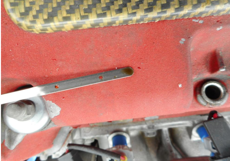
Photo 21 shows the engine oil dip stick of the Motor Car at the time of my inspection. The engine oil was observed to be of insufficient level as there was a leakage from the damaged engine oil cooler.
