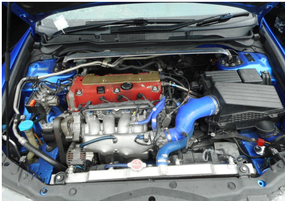
Photo 18 shows a general view of the Motor Car's engine compartment. The various parts and components inside the engine compartment were unaffected by the accident. There was also no sign(s) or indication(s) of fluid leakage and/or fluid stain within the engine compartment.
