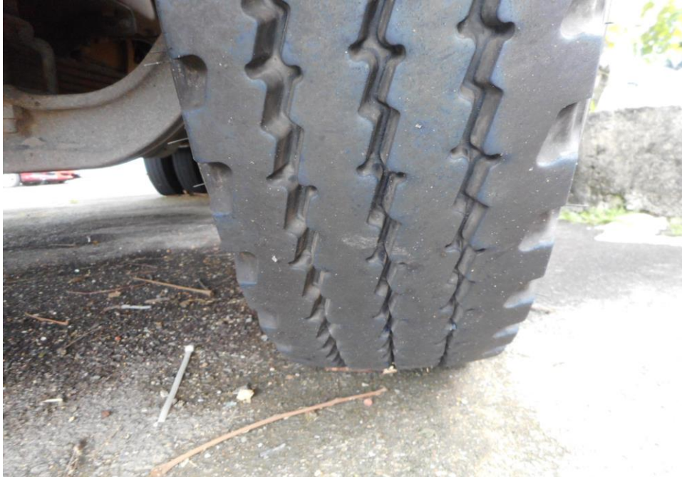
Photo 10 shows the condition of the rear right tyres of the Motor Lorry, which were observed to be in serviceable condition with remaining, tread depth of approximately 11.4mm. There was also no tear, cut or burst mark(s) on the outer and the inner sidewalls as well as across the tread of the 6 tyres that were fitted on the Motor Lorry.
