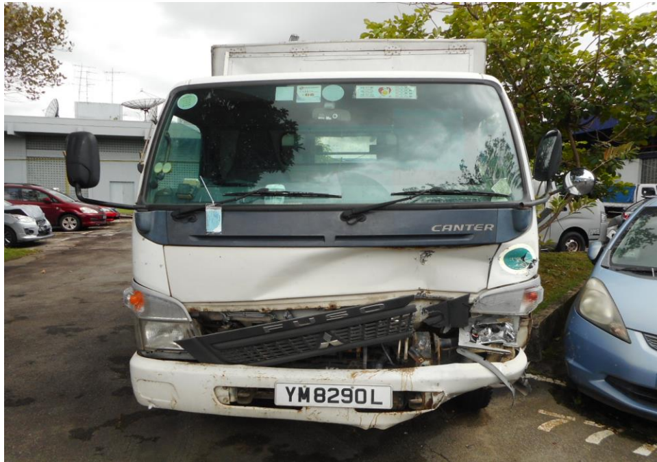
Photo 2 shows a general view of the Motor Lorry's frontal portion at the time of my inspection. It appeared to have sustained damage at its frontal portion. Its front body panel, front bumper and front left headlamp were damage at the time of my inspection as a result of the accident.
