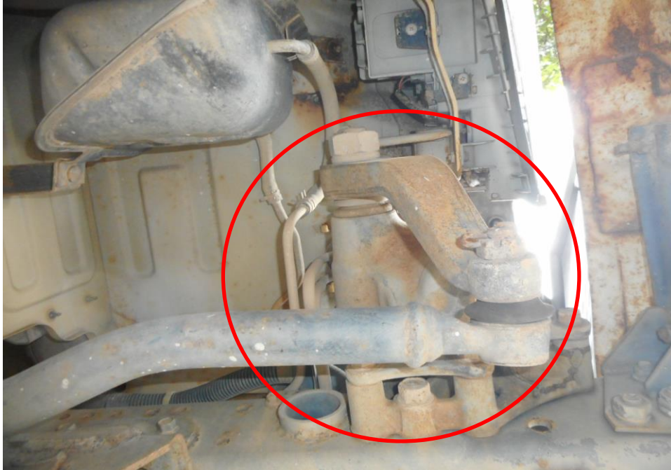
Photo 19 shows a general view of the steering box (circled) of the Motor Lorry at the time of my inspection. The steering box was observed to be unaffected by the accident.
