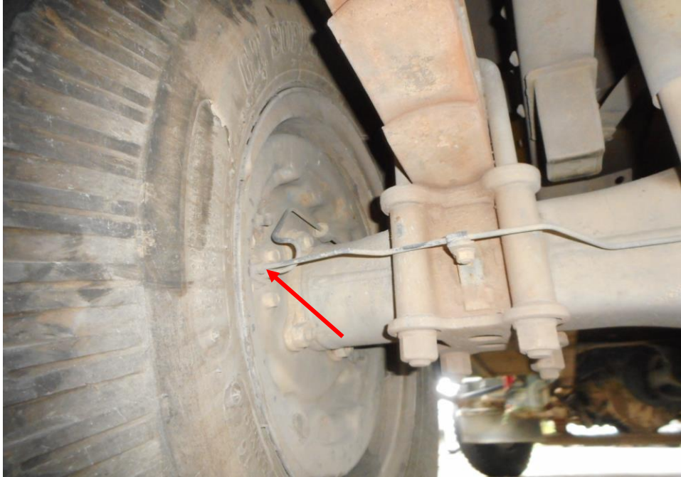
Photo 15 shows the brake pipe (arrowed) at the rear left wheel of the Motor Lorry. I did not observe any leakage of brake fluid at the time of my inspection of the Motor Lorry.
