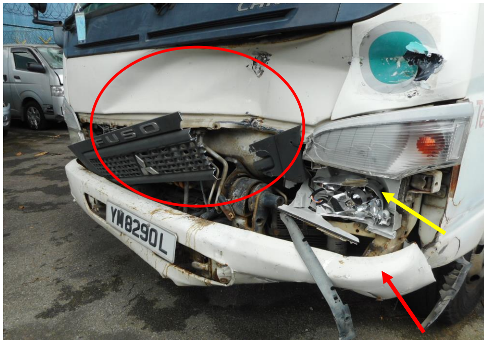
Photo 3 shows a close up view of the Motor Lorry's frontal portion at the time of my inspection. It appeared to have sustained damage at its frontal portion. Its front body panel (circled), front bumper (red arrow) and front left headlamp (yellow arrow) were damage at the time of my inspection.as a result of the accident.
