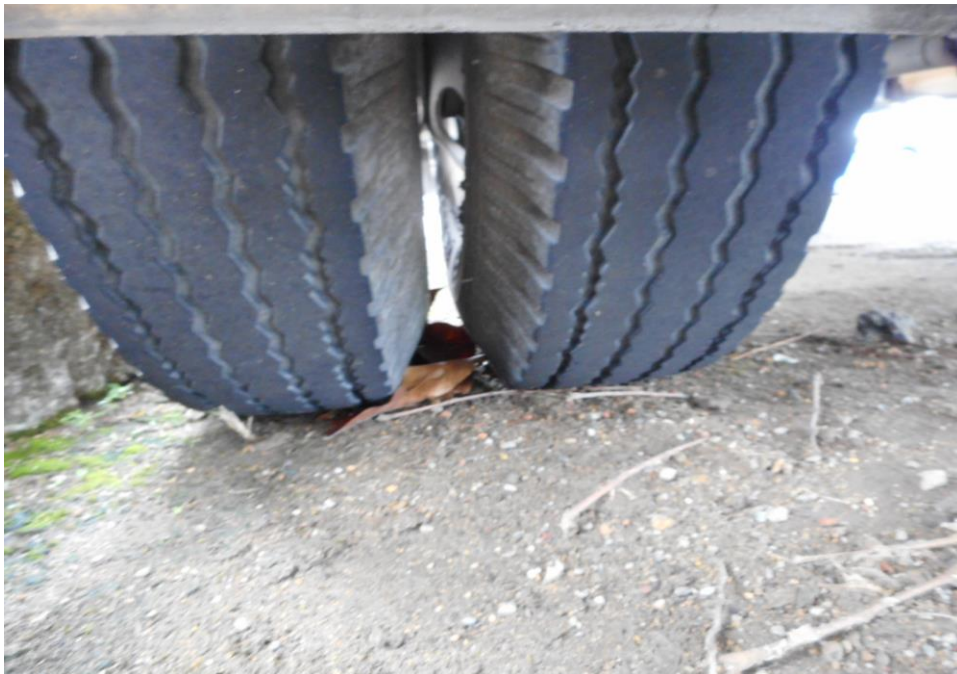
Photo 9 shows the condition of the rear left tyres of the Motor Lorry, which was observed to be in serviceable condition with remaining tread depth of approximately 4.8mm. The tyres, which were wrapped around standard steel wheel rim, were also observed to be sufficiently inflated for vehicular operation. There was also no damage found on all 6 steel wheel rims of the Motor Lorry.
