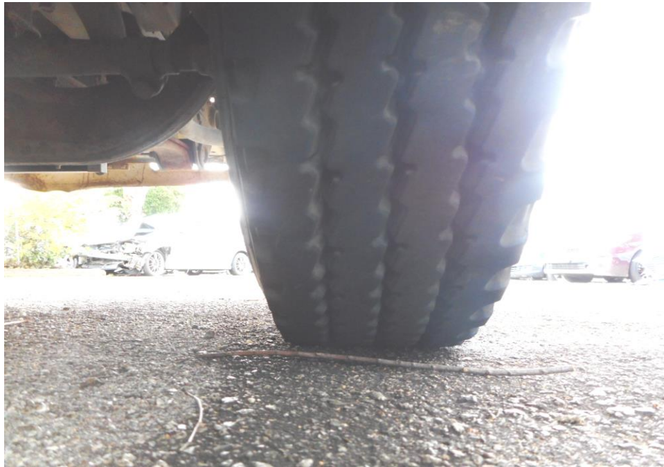
Photo 7 shows the condition of the front right tyre of the Motor Lorry, which was observed to be in serviceable condition with remaining tread depth of approximately 11.4mm. The tyre, which was wrapped around standard steel wheel rim, was also observed to be sufficiently inflated for vehicular operation. There was no tear, cut or burst mark(s) on the outer and the inner sidewalls as well as across the tread of the 6 tyres that were fitted on the Motor Lorry.
