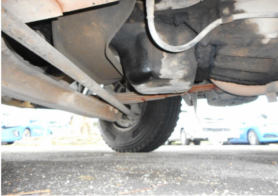
Photo 13 shows the undercarriage of the Motor Lorry, at the area where the engine housing and transmission housing are located. I did observed old engine fluid stain(s) on the underside of the Motor Lorry.
