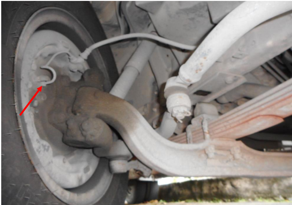
Photo 16 shows the brake hose/pipe (arrowed) at the front right wheel of the Motor Lorry. No leakage of brake fluid was observed. Visual examination of the various components of the braking system like the brake drum (circled), brake pedal etc had revealed all to be intact and without visible damage at the time of accident. There was also no sign of fluid stain(s) observed on the various undercarriage components.
