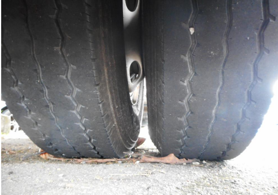
Photo 8 shows the condition of the rear right tyre of the Motor Lorry, which was observed to be in serviceable condition with remaining tread depth of approximately 3.3mm. The tyre, which was wrapped around standard steel wheel rim, it was observed to be sufficiently inflated for vehicular operation.
