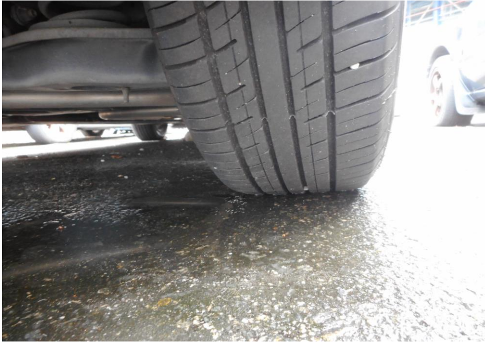
Photo 8 shows the condition of the rear right tyre of the Motor Car, which was observed to be in serviceable condition with remaining tread depth of approximately 5.8mm. The tyre was also observed to be sufficiently inflated for vehicular operation with no tear, cut or burst mark(s).
