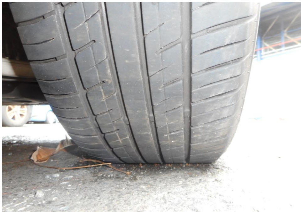
Photo 7 shows the condition of the front right tyre of the Motor Car, which was observed to be in serviceable condition with remaining tread depth of approximately 4.9mm. The tyre was sufficiently inflated for vehicular operation with no tear, cut or burst mark(s) on the outer and the inner sidewalls as well as across the tread. The 4 tyres of the Motor Car were wrapped around standard steel wheel rims without any damage.
