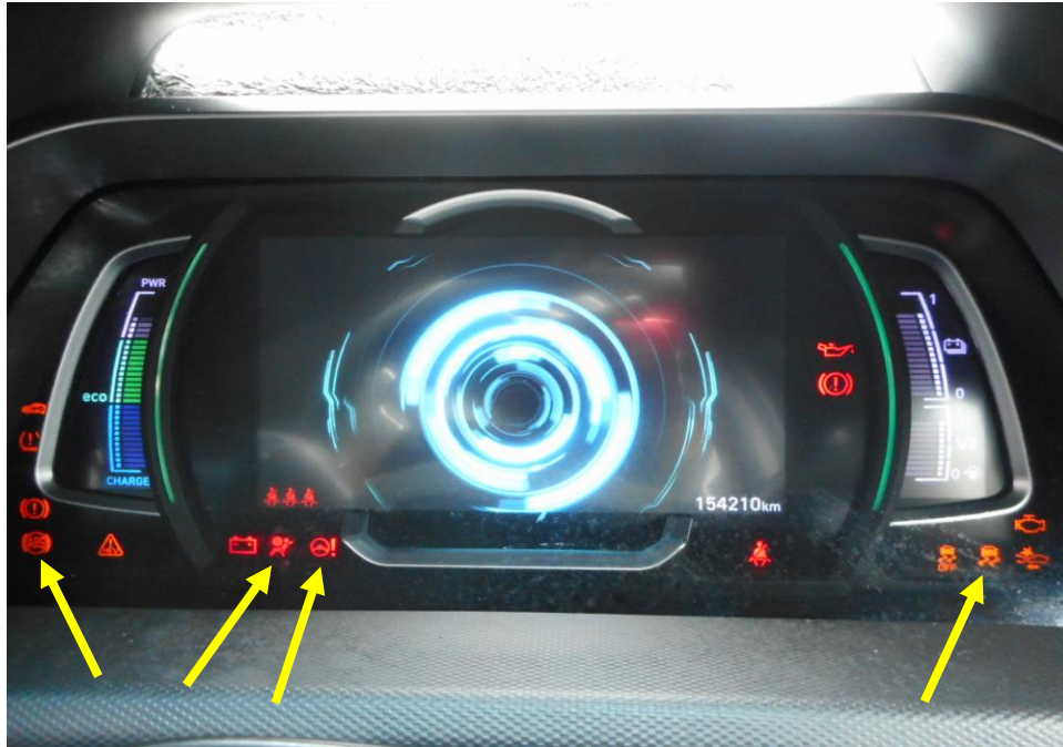
Photo 23 shows the warning light for Anti-Lock Brake System (ABS) and Power Steering System (EPS), Supplemental Restraint System (SRS) and Traction Control (TC) (arrowed) appearing on the instrument panel of the Motor Car during the self-test of its various electronic operating systems when its engine was cranked.
