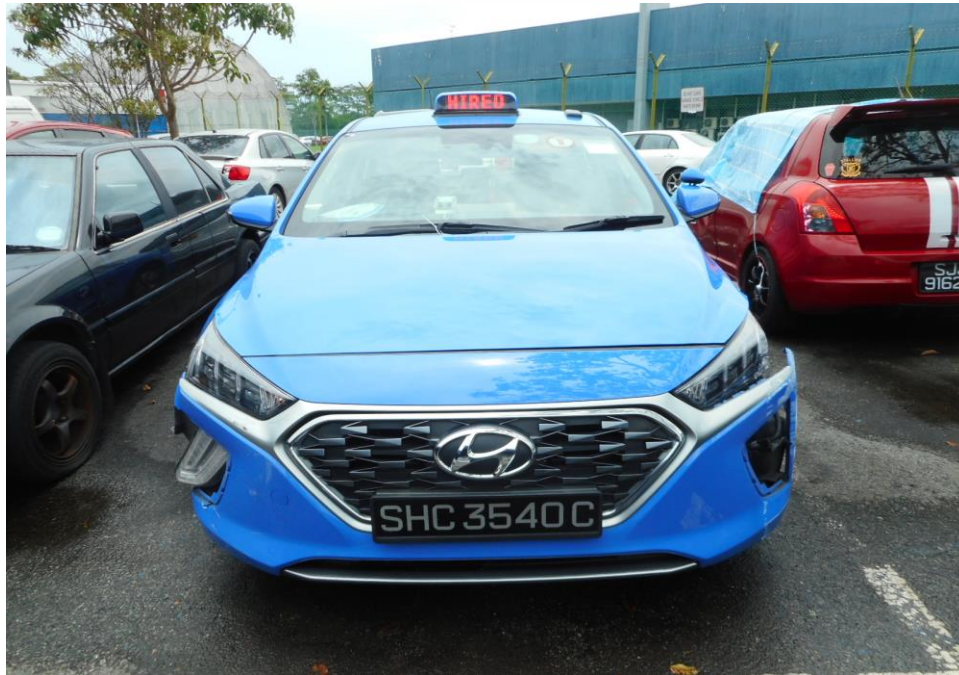
Photo 2 shows a general view of the Motor Car's front body at the time of my inspection. The front portion of the Motor Car was observed to have sustained damage. Its front left headlamp, front bumper and front left fender was the body parts that were damaged as a result of the accident.
