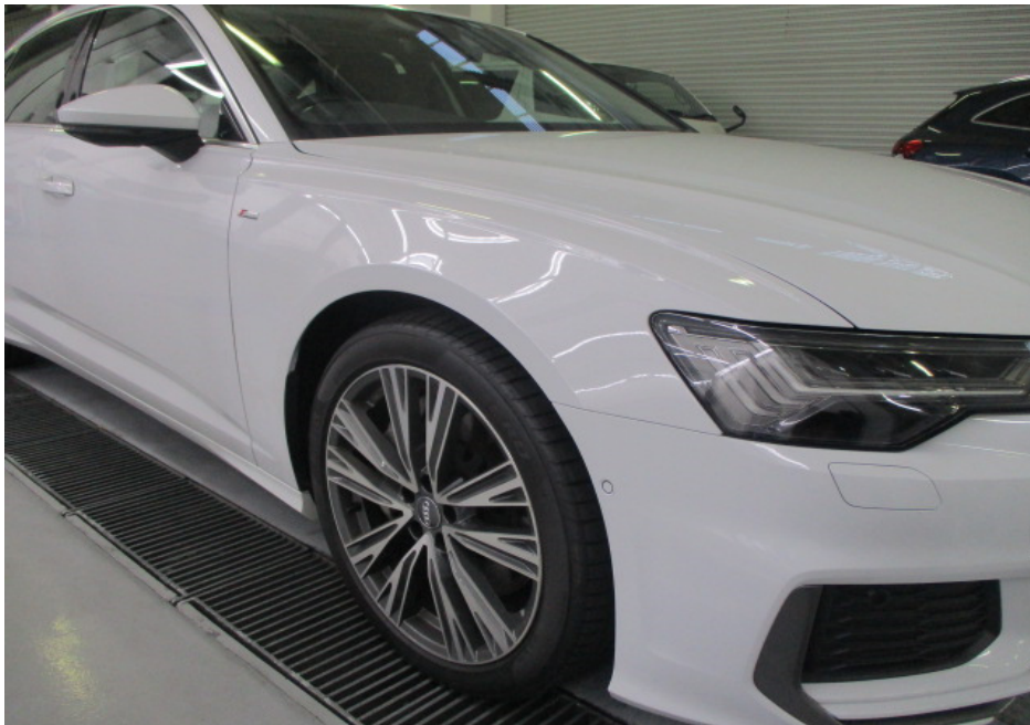
Photo 7 shows a closer view of the front bumper, front right headlamp, front right headlamp washer cover and front right fender of the Motor Car. The body parts at the front right portion of the Motor Car were visually examined and it was observed that the repair/restoration works carried out to the damaged area of the Motor Car (refer to photograph 1 above) were reasonably adequate and in order.
