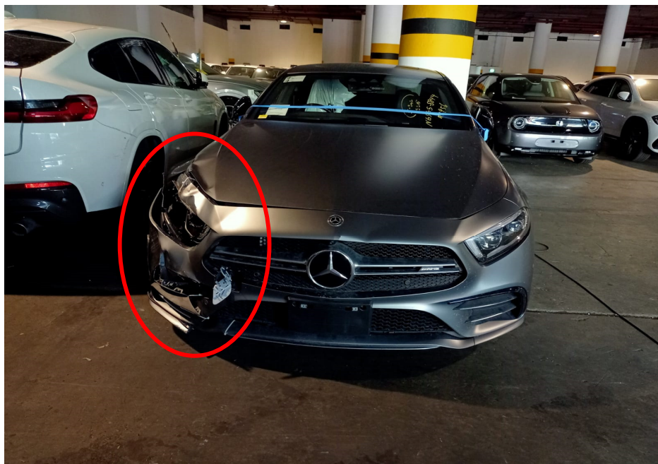
Photo 1 shows the frontal body of the Motor Car (photograph provided to me). The Motor Car was observed to have sustained damage at its front right portion (circled). The front bumper, front right headlamp and front bonnet were amongst the parts that were observed to have been damaged.
