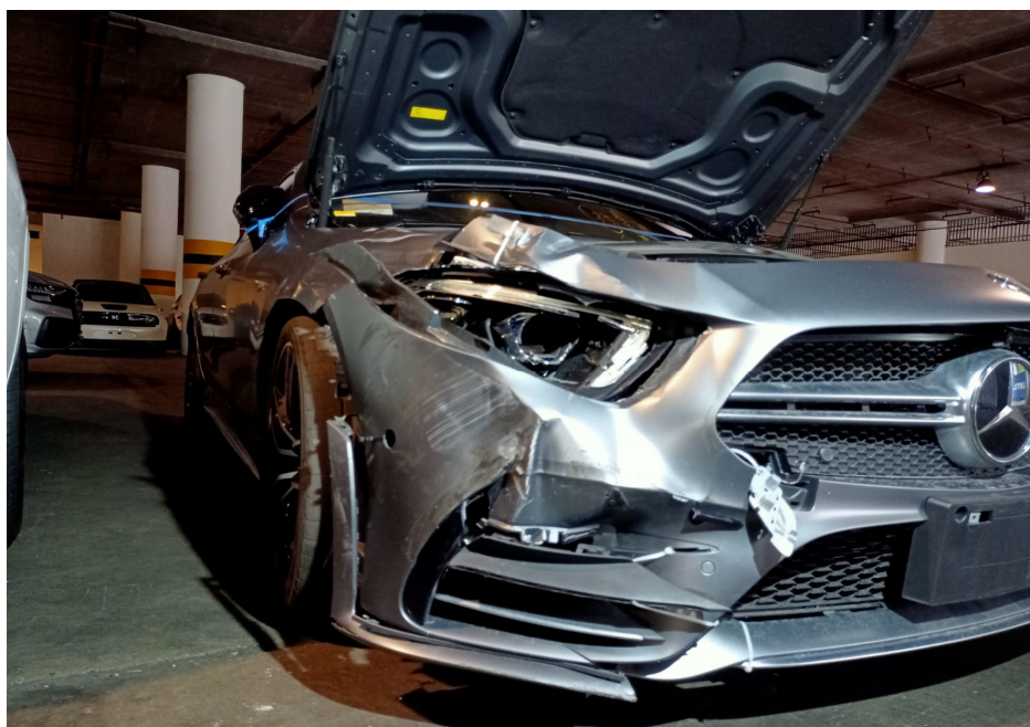
Photo 2 shows a closer view of the damage at the front right portion of the Motor Car (photograph provided to me). The front bumper, front bumper right lower grille, front bumper right lower grille garnish, front bumper right lower lip, radiator grille, front right headlamp and front right fender were amongst the parts that were observed to have been damaged.
