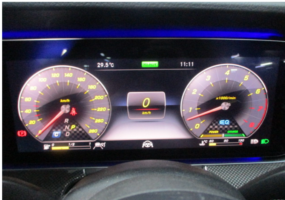
Photo 15 shows the respective warning lights no longer illuminated, indicating that there is no fault detected to the ABS, SRS, EPS and TCS systems of the Motor Car during the self-test. These electronic systems were hence in working condition at the time of my inspection.
