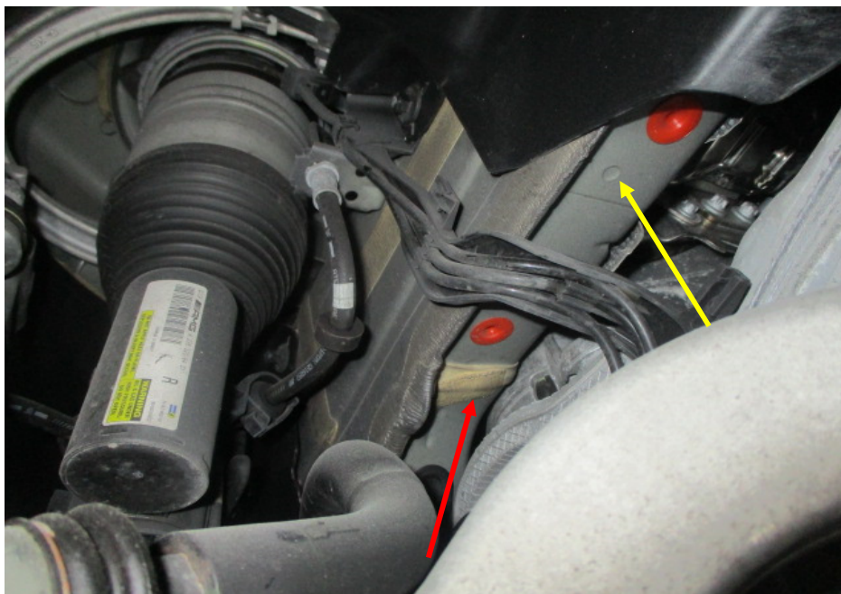
Photo 22 shows the chassis/structural body at the underside front right of the Motor Car. I did not find any weld marks other than original spot weld marks (yellow arrow) on the chassis/structural body of the Motor Car. The original factory sealant (red arrow) at the joints along the chassis/structural body was also untouched, indicating no work was done on the chassis/structural body of the Motor Car and that the chassis/structural body was originally fitted.
