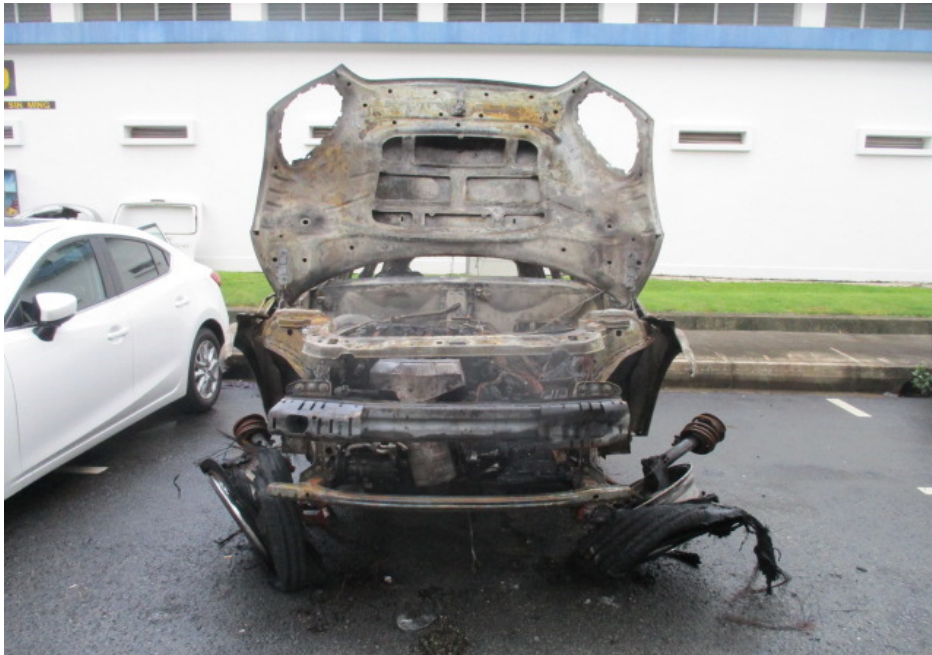
Photo 1 shows the general view of the frontal portion of the Insured Vehicle at the time of our inspection. The Insured Vehicle was observed to have sustained extensive fire damage all around. Its engine compartment and interior compartment were completely burnt. Rust had accumulated all over the Insured Vehicle as a result of exposure to environmental condition for a period of time.
