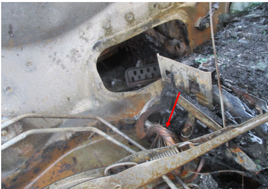
Photo 7 shows a close up view of the faint greenish residue found on the wirings around the rear portion of the engine compartment (arrowed). The presence of greenish residue indicates internal heating of copper wires, a sign of an electrical short circuit.
