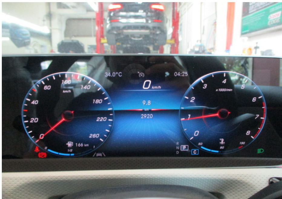
Photo 16 shows the respective warning lights no longer illuminated, indicating that there is no fault detected to the ABS, SRS, EPS TCS systems of the Motor Car during the self-test. These electronic systems were hence in working condition at the time of my inspection.
