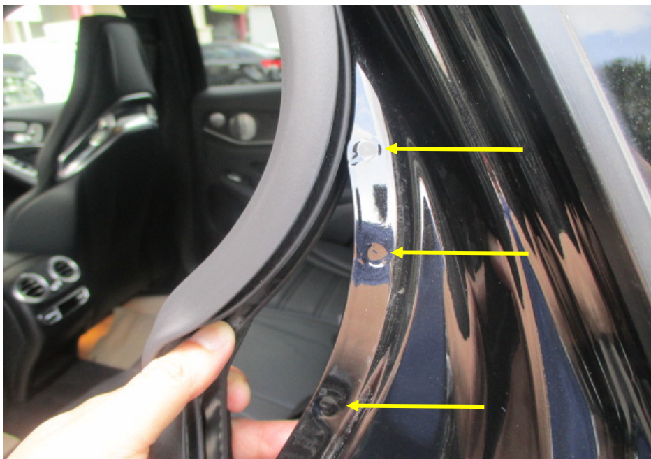
Photo 26 shows the left side "C" pillar of the Motor Car. I did not find any weld marks other than original spot weld marks (arrowed) on the left side "C" pillar of the Motor Car which, indicates that there was no re-welding works carried out. In general, I had found all the non-detachable body panels of the Motor Car to be originally fitted at the time of my inspection.
