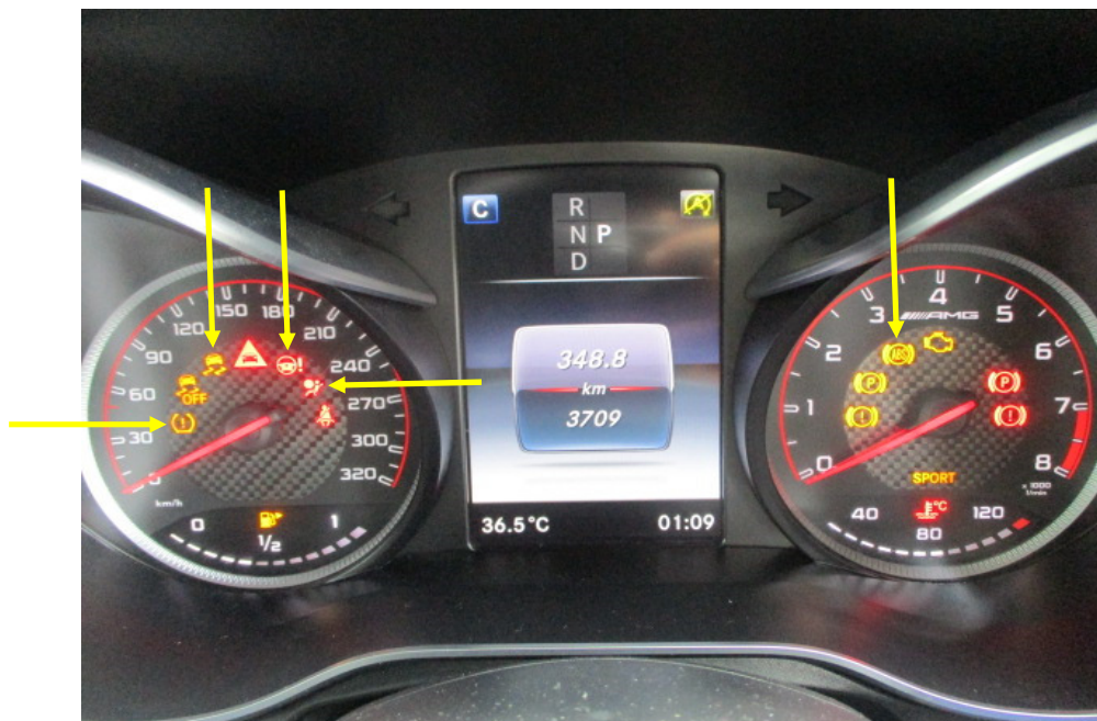
Photo 15 shows the warning lights for the various electronic safety features appearing on the instrument panel of the Motor Car during its self-test when the engine is cranked, in particular the ABS, SRS, EPS, TPM and TCS lights (arrowed).
