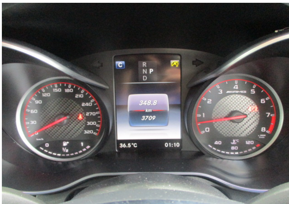
Photo 16 shows the respective warning lights no longer illuminated, indicating that there is no fault detected to the ABS, SRS, EPS, TPM and TCS systems of the Motor Car during the self-test. These electronic systems were hence in working condition at the time of my inspection.
