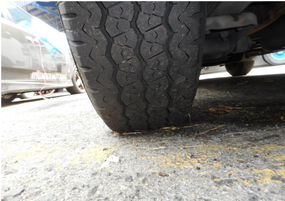
Photo 9 shows the condition of the rear left tyres of the Motor Van, which was observed to be in serviceable condition with remaining tread depth of approximately 5.4mm. The tyres, which were wrapped around standard steel wheel rim, were also observed to be sufficiently inflated for vehicular operation. There was also no damage found on all 4 steel wheel rims of the Motor Van.
