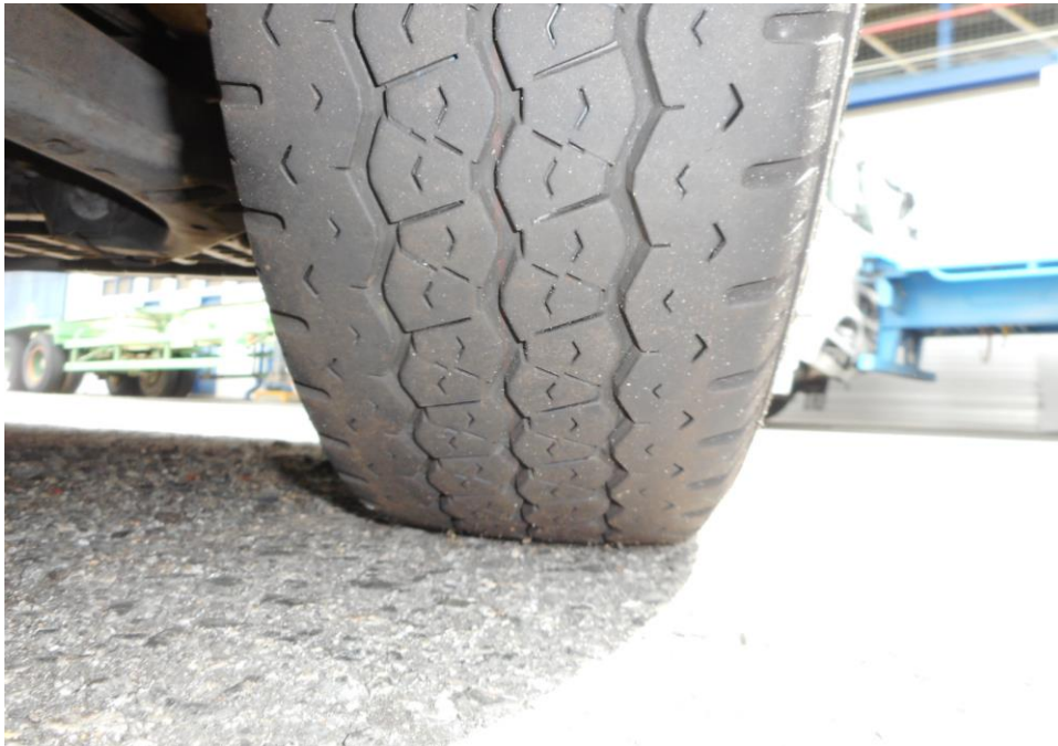
Photo 7 shows the condition of the front right tyre of the Motor Van, which was observed to be in serviceable condition with remaining tread depth of approximately 5.1mm. The tyre, which was wrapped around standard steel wheel rim, was also observed to be sufficiently inflated for vehicular operation. There was no tear, cut or burst mark(s) on the outer and the inner sidewalls as well as across the tread of the 4 tyres that were fitted on the Motor Van.
