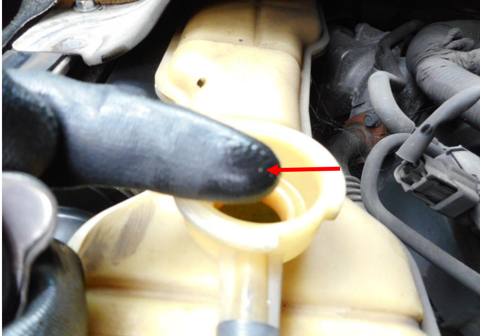
Photo 13 shows the engine coolant reservoir of the Motor Van at the time of my inspection. The engine coolant was observed to be of sufficient level (arrowed) and without any visible contamination.
