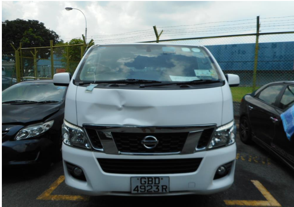
Photo 2 shows a general view of the Motor Van's frontal portion at the time of my inspection. It appeared to have sustained damage at its frontal portion. Its front body panel were damage at the time of my inspection.
