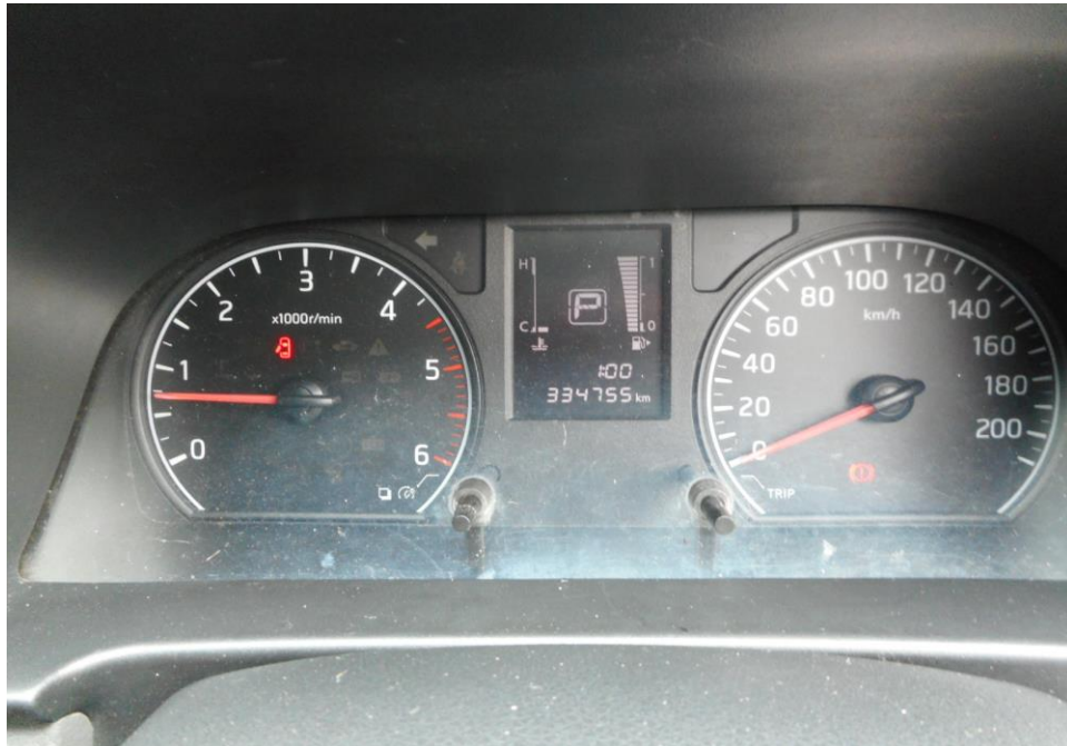
Photo 24 shows no warning lights illuminated on the instrument panel of the Motor Van after the engine was cranked. This would suggest that there was no abnormality to the electronic operating system of the Motor Van, like the ABS and SRS etc.
