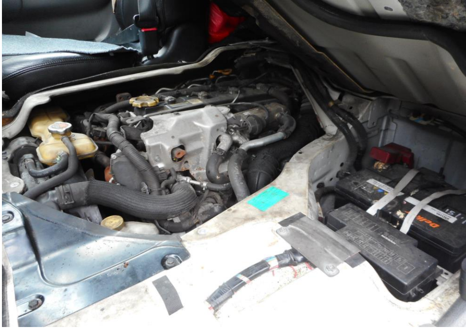
Photo 11 shows a general view of the Motor Van's engine compartment, which was accessed by lifting the front cabin of the Motor Van. The various parts and components inside the engine compartment were unaffected by the accident. There was also no sign(s) or indication(s) of fresh fluid leakage and/or fluid stain within the engine compartment
