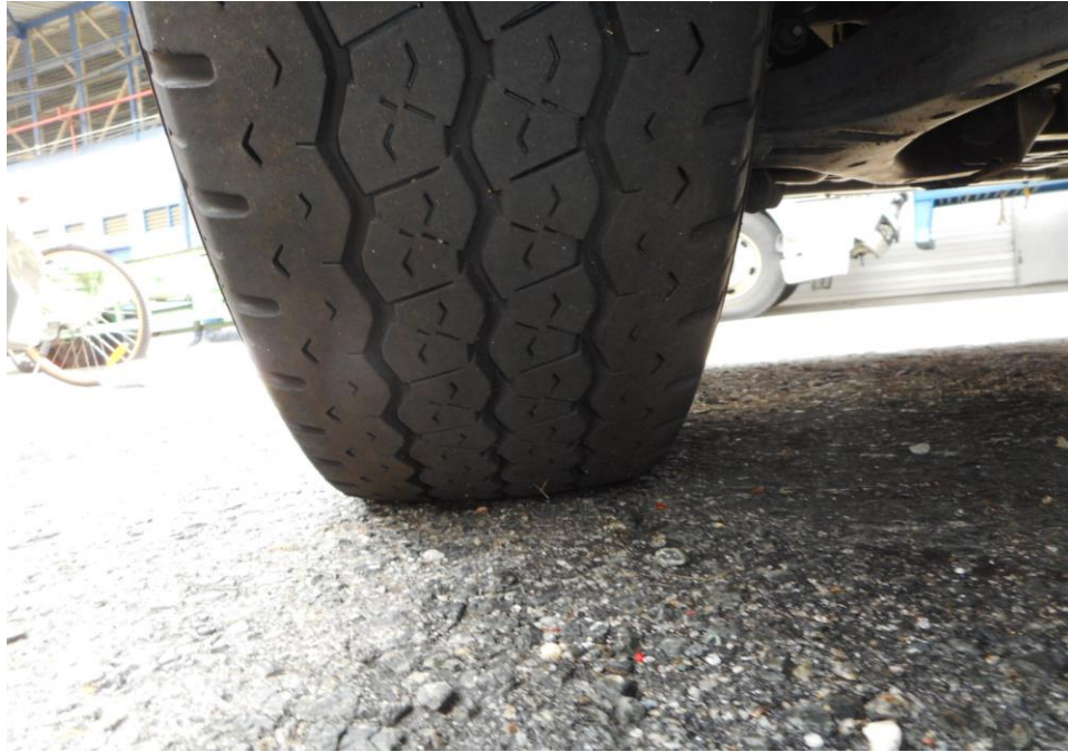
Photo 10 shows the condition of the rear right tyres of the Motor Van, which were observed to be in serviceable condition with remaining, tread depth of approximately 5.1mm. There was also no tear, cut or burst mark(s) on the outer and the inner sidewalls as well as across the tread of the 4 tyres that were fitted on the Motor Van.
