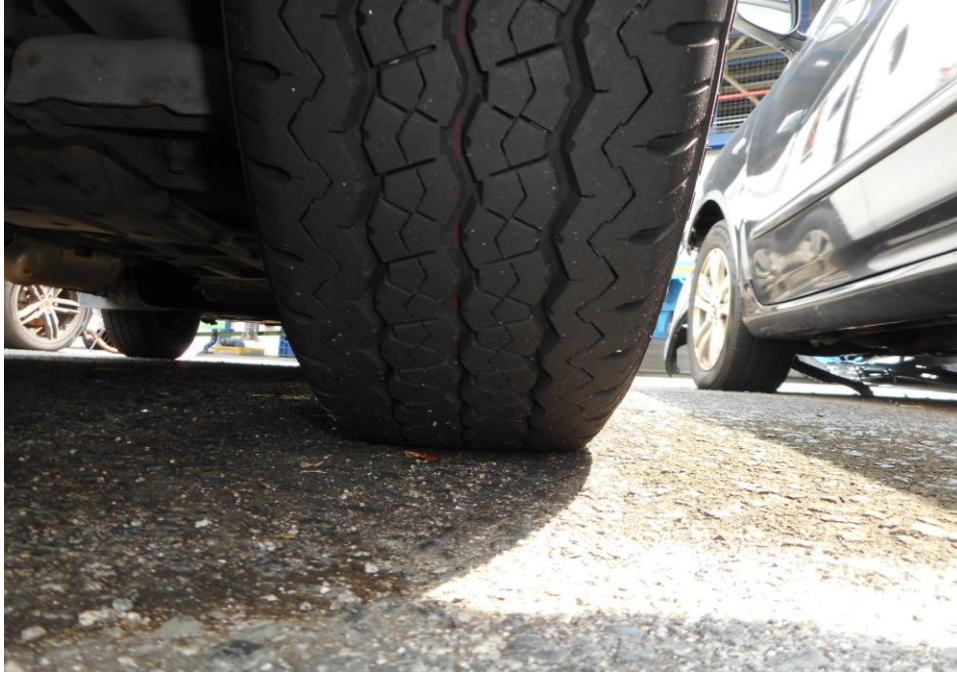
Photo 8 shows the condition of the rear right tyre of the Motor Van, which was observed to be in serviceable condition with remaining tread depth of approximately 7.3mm. The tyre, which was wrapped around standard steel wheel rim, it was observed to be sufficiently inflated for vehicular operation.
