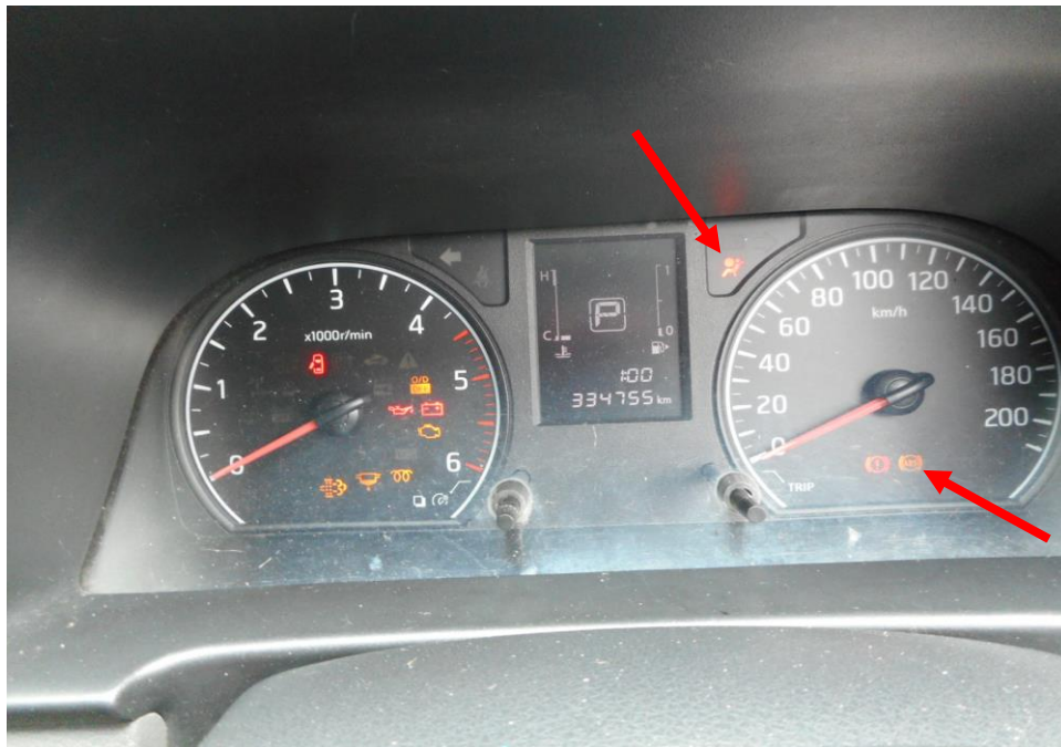
Photo 23 shows the warning light for Anti-Lock Brake System (ABS) and Supplemental Restraint System (SRS) (arrowed) appearing on the instrument panel of the Motor Van during the self-test of its various electronic operating systems when its engine was cranked.
