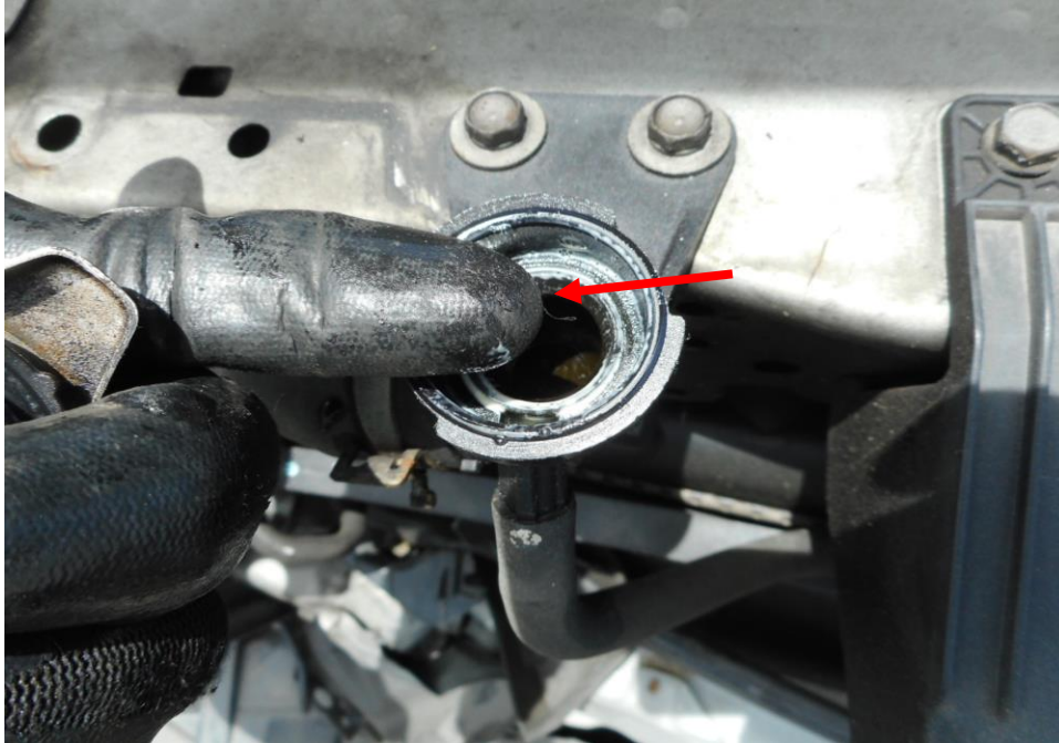
Photo 15 shows checks being carried out to the engine coolant of the Motor Car at the time of my inspection. The engine coolant was observed to be insufficient level (arrowed) as the result of the accident had damaged the engine radiator and caused the leakage of engine coolant.
