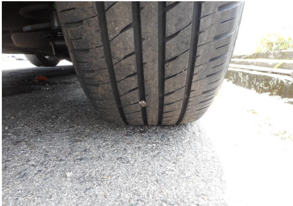
Photo 9 shows the condition of the rear right tyre of the Motor Car, which was observed to be in serviceable condition with remaining tread depth of approximately 5.3mm. The tyre was also observed to be sufficiently inflated for vehicular operation with no tear, cut or burst mark(s).
