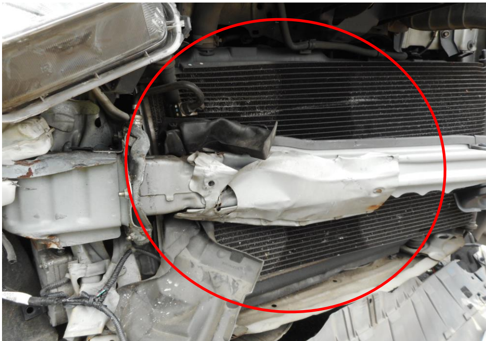
Photo 5 shows the close up view of the Motor Car's front body at the time of my inspection. The Motor car was observed to have sustained damage at its front portion. Its engine radiator (circled) was amongst the various components in the engine compartments were also damaged as a result of the accident.
