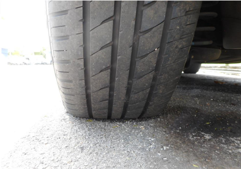
Photo 10 shows the condition of the rear left tyre of the Motor Car, which was observed to be in serviceable condition with remaining tread depth of approximately 5.3mm. The tyre was also observed to be sufficiently inflated for vehicular operation with no tear, cut or burst mark(s).
