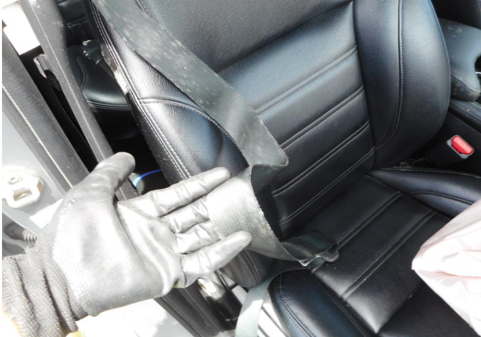
Photo 26 shows that the seat belt on the right seat was worn at the material time of accident as the safety pre-tensioners was activated at the moment of impact and caused the seat belt to be locked into the last position.
