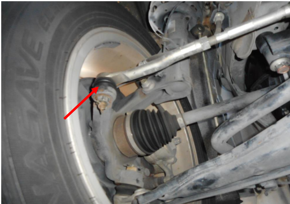
Photo 23 shows the various undercarriage components at the front left wheel of the Motor Car, in particular the steering tie rod end (arrowed). The various steering components were all found to be intact, suggesting that the steering system of the Motor Car was likely to be in serviceable condition at the material time of accident. There was also no sign of fluid stain(s) observed on the various undercarriage components.
