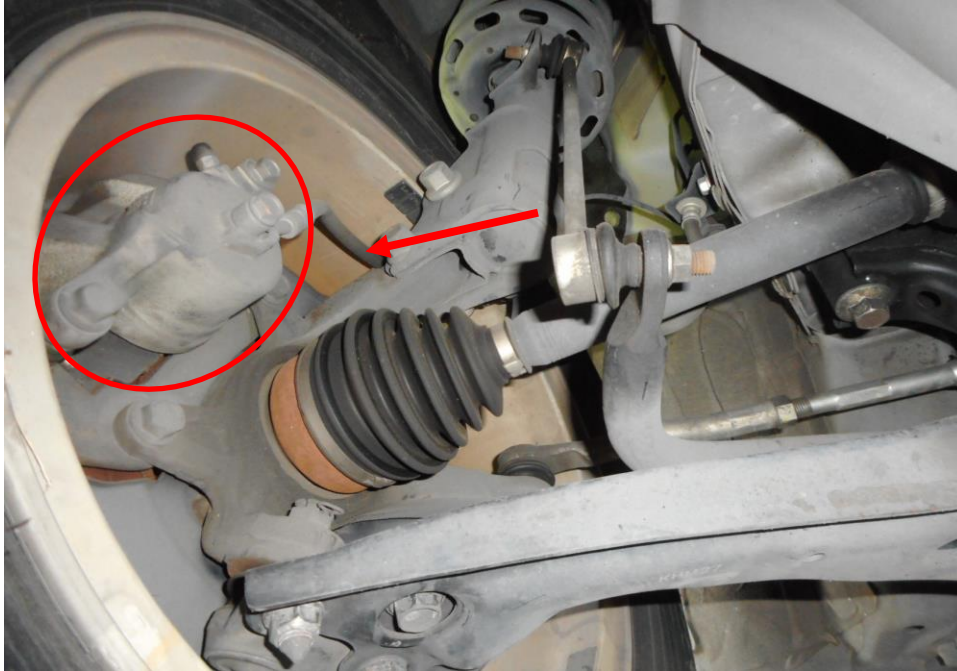
Photo 20 shows the brake hose/pipe (arrowed) at the front right wheel of the Motor Car. No leakage of brake fluid was observed. Visual examination of the various components of the braking system like the brake caliper (circled) brake pedal etc had revealed all to be intact and without visible damage at the time of accident. There was also no sign of fluid stain(s) observed on the various undercarriage components.
