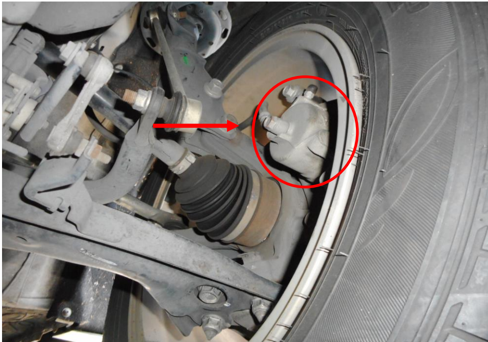
Photo 21 shows the brake hose/pipe (arrowed) at the front left wheel of the Motor Car. No leakage of brake fluid was observed. Visual examination of the various components of the braking system like the brake caliper (circled), brake pedal etc had revealed all to be intact and without visible damage at the time of accident. There was also no sign of fluid stain(s) observed on the various undercarriage components.
