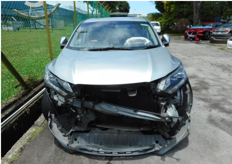
Photo 2 shows a general view of the Motor Car's front body at the time of my inspection. The Motor car was observed to have sustained damage at its front portion. Its front bonnet, front right headlamp, front bumper, front right fender was amongst the body parts and various components in the engine compartments were also damaged as a result of the accident.
