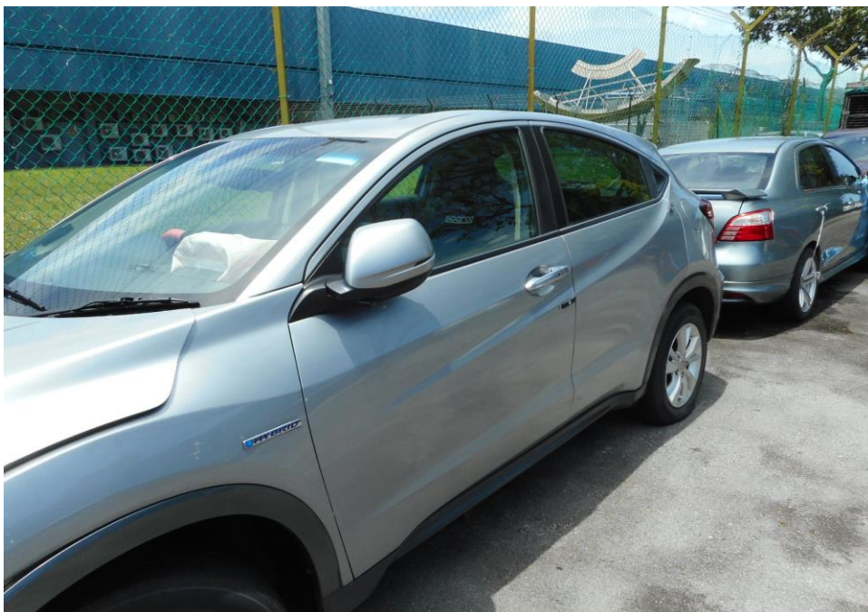
Photo 7 shows a general view of the Motor Car's left body at the time of my inspection. The left portion of the Motor Car was observed to have been undamaged by the accident.
