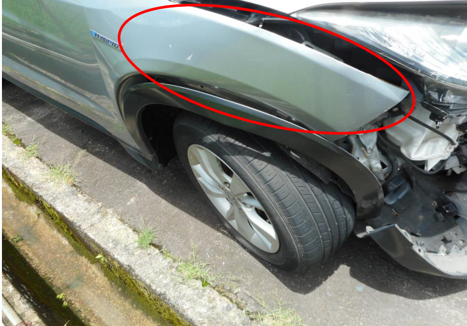
Photo 4 shows the general view of the Motor Car's front body at the time of my inspection. The Motor car was observed to have sustained damage at its front portion. Its front right fender (circled) was amongst the body parts and various components in the engine compartments were also damaged as a result of the accident.
