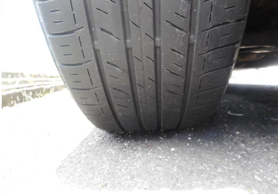
Photo 8 shows the condition of the front right tyre of the Motor Car, which was observed to be in serviceable condition with remaining tread depth of approximately 4.5mm. The tyre was also observed to be sufficiently inflated for vehicular operation with no tear, cut or burst mark(s).
