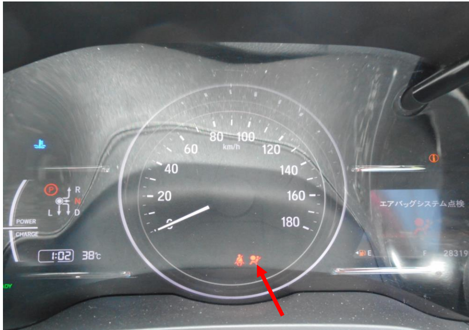
Photo 25 shows no warning lights illuminated on the instrument panel of the Motor Car after the engine was cranked. This would suggest that there was no abnormality to the electronic operating system of the Motor Car, like the ABS, EPS and TC etc. The Supplemental Restraint System (SRS) (arrowed) light remained on due to the deployment of the airbag as a result of the accident.
