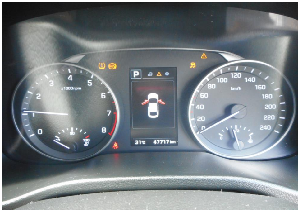
Photo 26 shows only the ABS and TC warning lights illuminated on the instrument panel of the Motor Car after the engine was cranked. This was caused by the damaged front left tyre and rim as a result of the accident.
