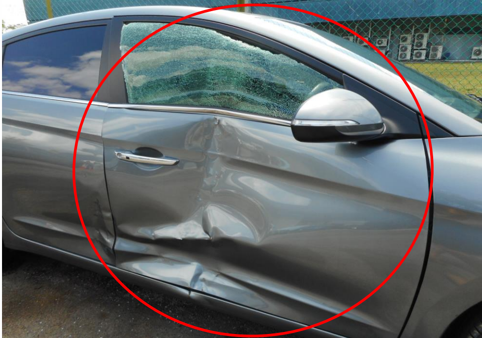
Photo 8 shows a close up view of the Motor Car's right body at the time of my inspection. The right portion of the Motor Car was observed to have sustained damage at its right door (circled) as a result of the accident.
