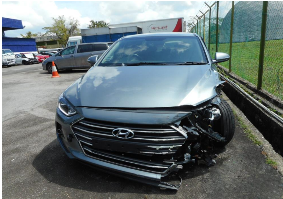
Photo 3 shows a general view of the Motor Car's front body at the time of my inspection. The front portion of the Motor Car was observed to have sustained damage. Its front bonnet, front bumper and front left headlamp was the body parts that were damaged as a result of the accident.
