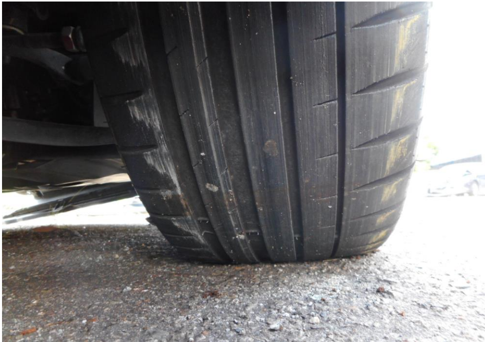
Photo 9 shows the condition of the front right tyre of the Motor Car, which was observed to be in serviceable condition with remaining tread depth of approximately 4.6mm.
