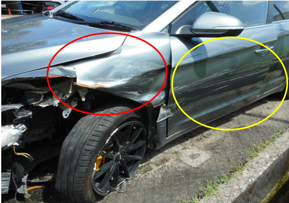
Photo 6 shows a close up view of the Motor Car's left body at the time of my inspection. The left portion of the Motor Car was observed to have sustained damage at its left fender (red circle) and left door (yellow circle) as a result of the accident.
