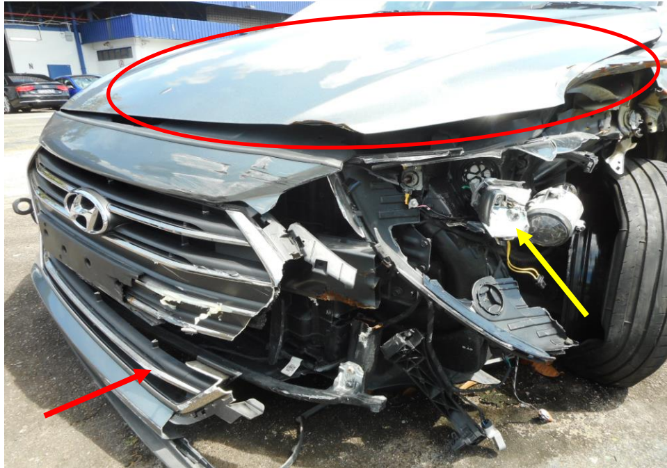
Photo 4 shows the close up view of the Motor Car's front body at the time of my inspection. The Motor Car was observed to have sustained damage at its front bonnet (red circle), front bumper (red arrow) and front left headlamp (yellow arrow) as a result of the accident.
