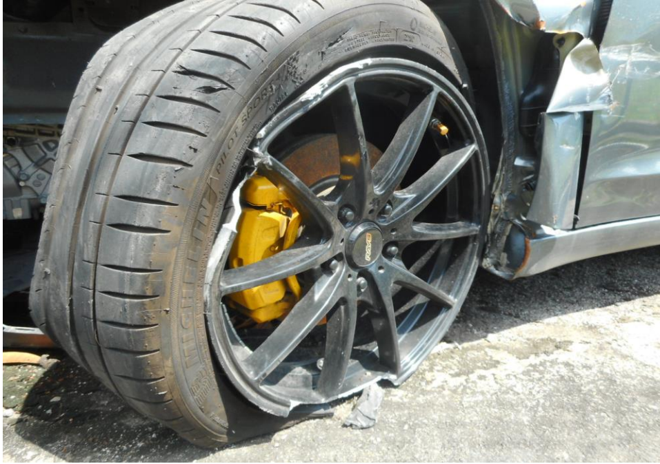
Photo 12 shows the condition of the front left tyre of the Motor Car, which was observed to be in unserviceable condition with remaining tread depth of approximately 4.6mm. The tyre was observed to have slipped of the damaged wheel rim and deflated as a result of the accident.
