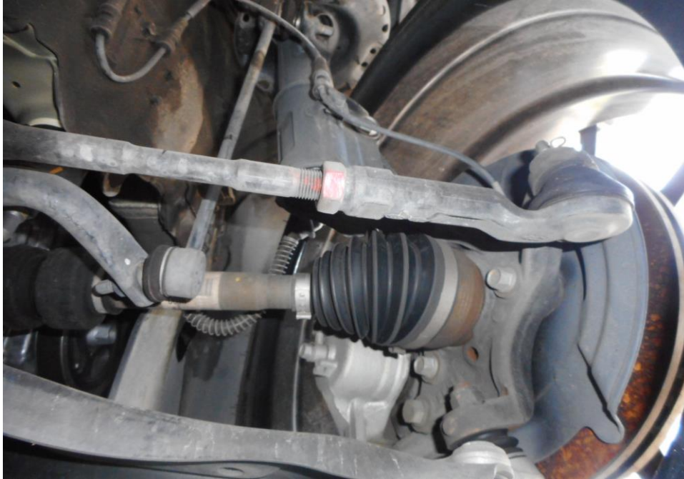
Photo 22 shows the various undercarriage components at the front right wheel of the Motor Car, which had included the steering tie rod (red arrowed) and the driveshaft (yellow arrowed). The various undercarriage components of the Motor Car were all found to be intact without any visible damage.
