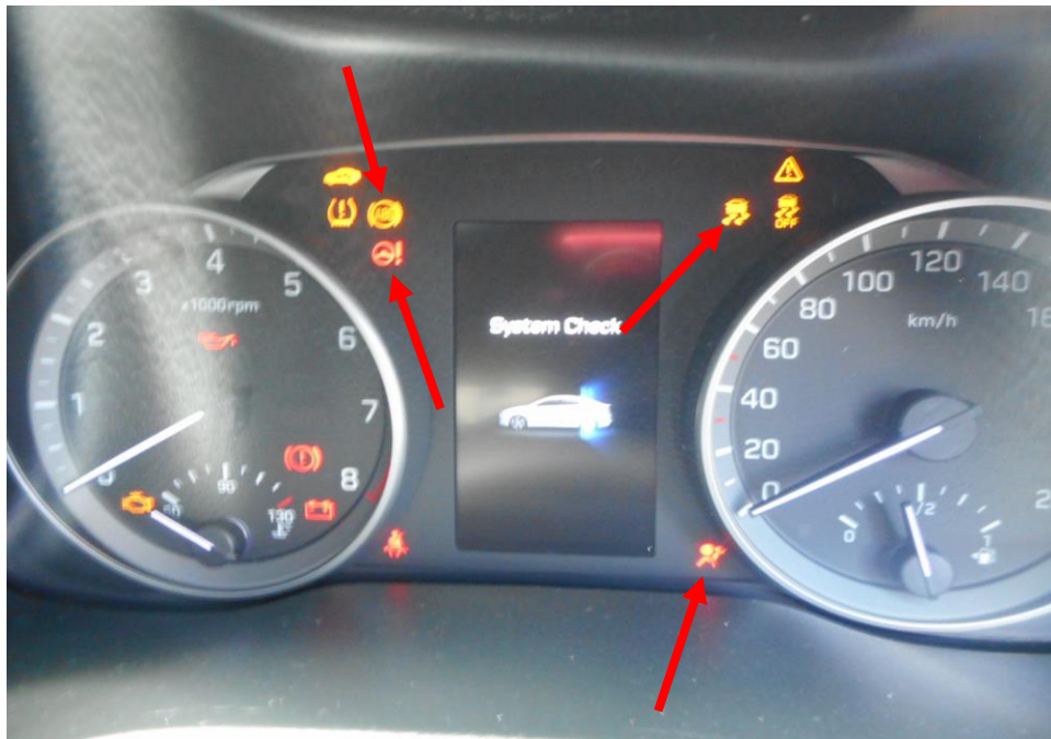
Photo 25 shows the warning light for Anti-Lock Brake System (ABS) and Power Steering System (EPS), Supplemental Restraint System (SRS) and Traction Control (TC) (arrowed) appearing on the instrument panel of the Motor Car during the self-test of its various electronic operating systems when its engine was cranked.
