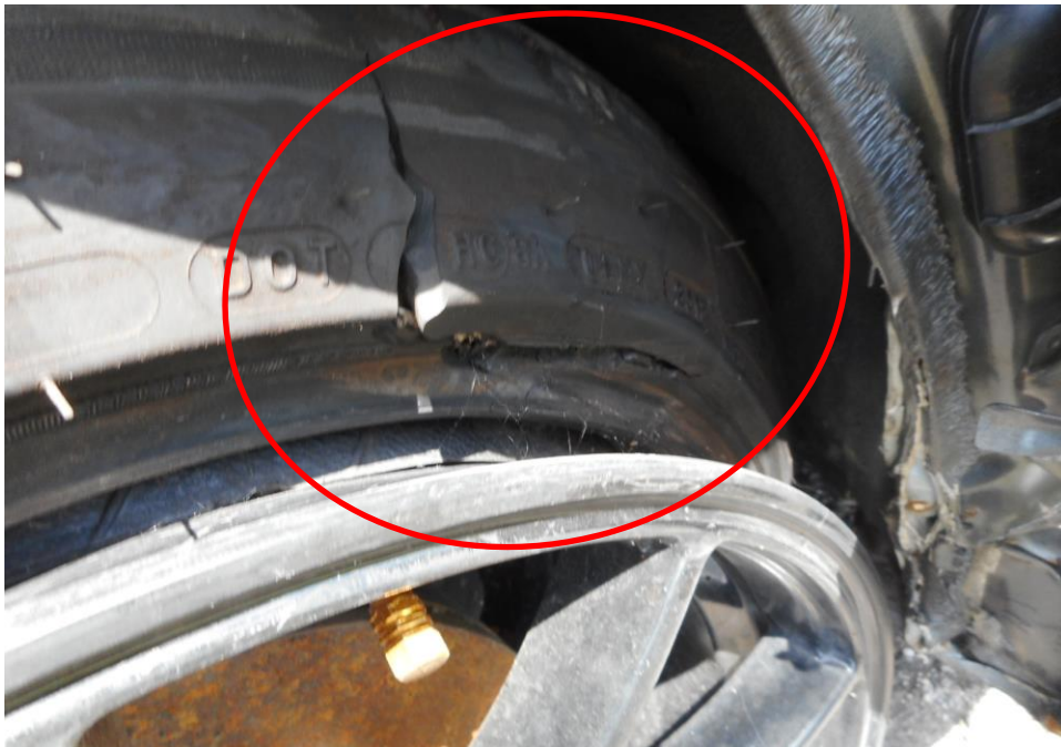
Photo 13 shows the close up condition of the front right tyre of the Motor Car, which was observed to be in unserviceable condition. The tyre was observed to be cut and slipped of the damaged wheel rim (circled) and deflated as a result of the accident.
