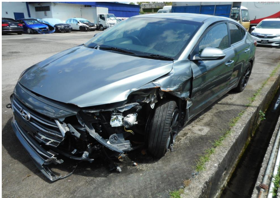
Photo 5 shows a general view of the Motor Car's left body at the time of my inspection. The left portion of the Motor Car was observed to have sustained damage at its left fender and left door as a result of the accident.
