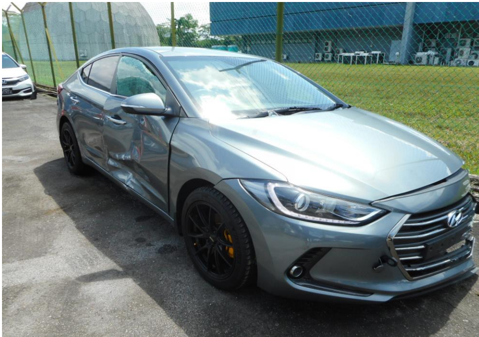
Photo 7 shows a general view of the Motor Car's right body at the time of my inspection. The right portion of the Motor Car was observed to have sustained damage at its right door as a result of the accident.
