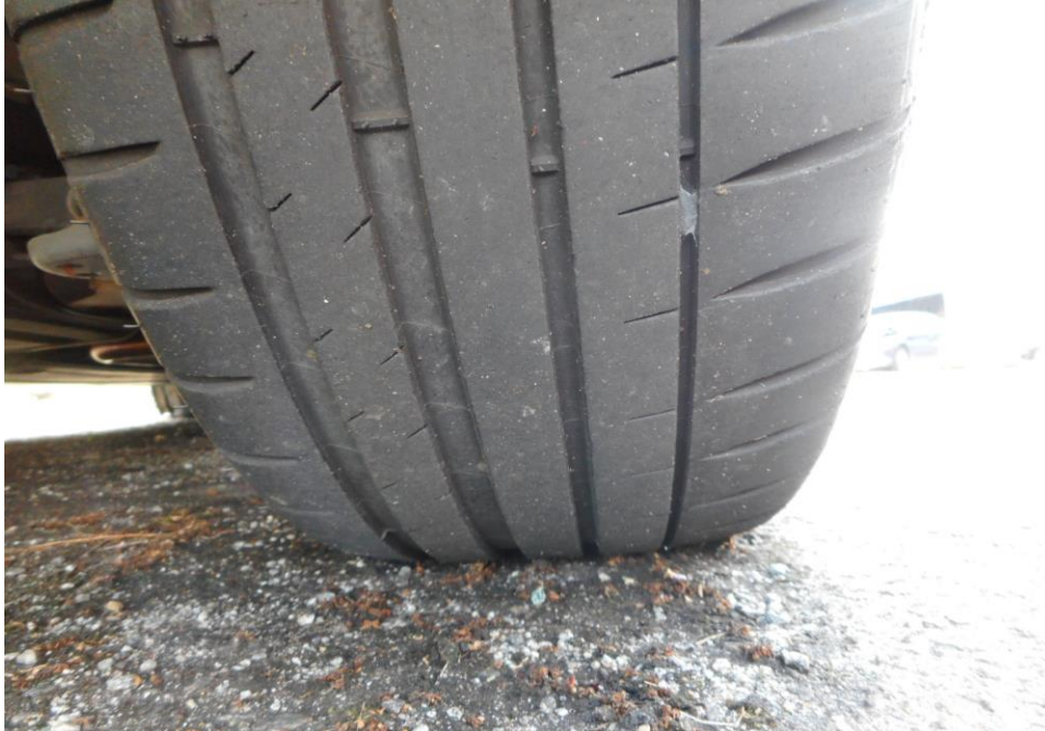
Photo 10 shows the condition of the rear right tyre of the Motor Car, which was observed to be in serviceable condition with remaining tread depth of approximately 4.9mm.
