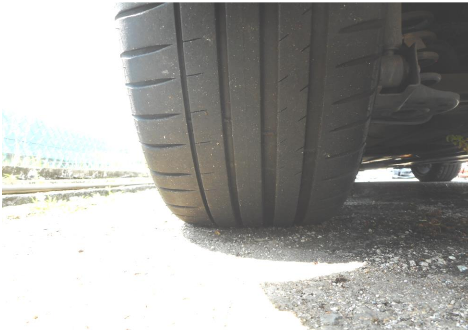
Photo 11 shows the condition of the rear left tyre of the Motor Car, which was observed to be in serviceable condition with remaining tread depth of approximately 4.9mm. The tyre, which was wrapped around steel wheel rim, was also observed to be sufficiently inflated for vehicular operation.
