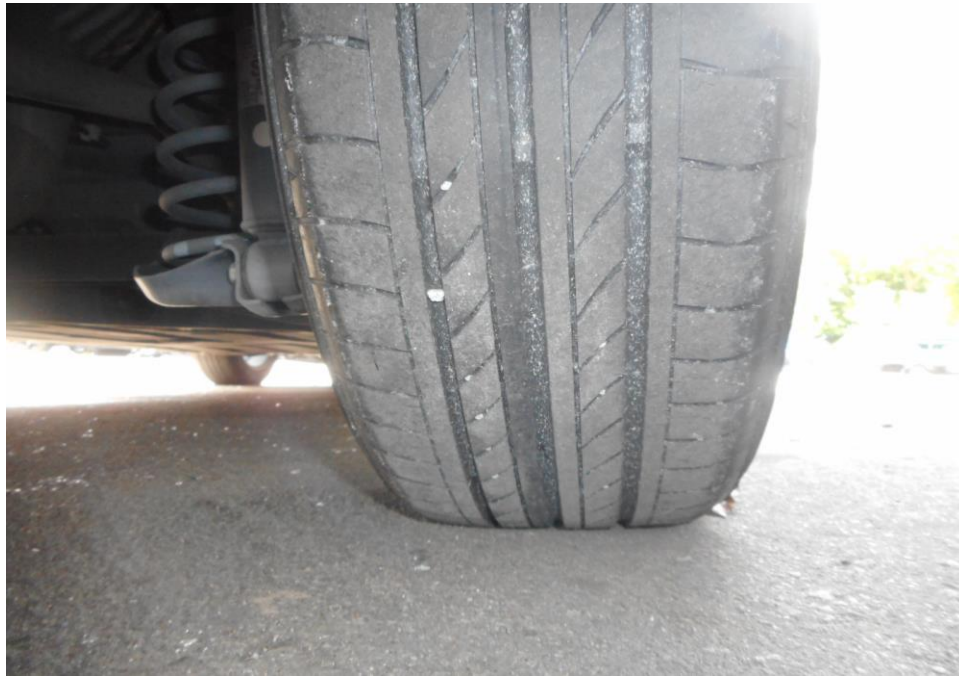
Photo 8 shows the condition of the rear right tyre of the Motor Car, which was observed to be in serviceable condition with remaining tread depth of approximately 3.8mm. The tyre was also observed to be sufficiently inflated for vehicular operation with no tear, cut or burst mark(s).
