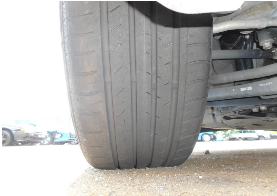
Photo 10 shows the condition of the front left tyre of the Motor Car, which was observed to be in serviceable condition with remaining tread depth of approximately 3.7mm. There was also no tear, cut or burst mark(s) on the outer and the inner sidewalls as well as across the tread of the Motor Car's 4 tyres.
