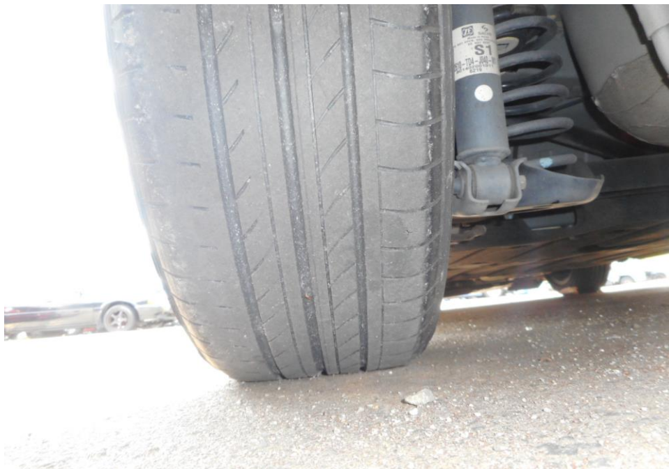
Photo 9 shows the condition of the rear left tyre of the Motor Car, which was observed to be in serviceable condition with remaining tread depth of approximately 3.4mm. The tyre, which was wrapped around steel wheel rim, was also observed to be sufficiently inflated for vehicular operation. The 4 tyres of the Motor Car were wrapped around standard steel wheel rims.
