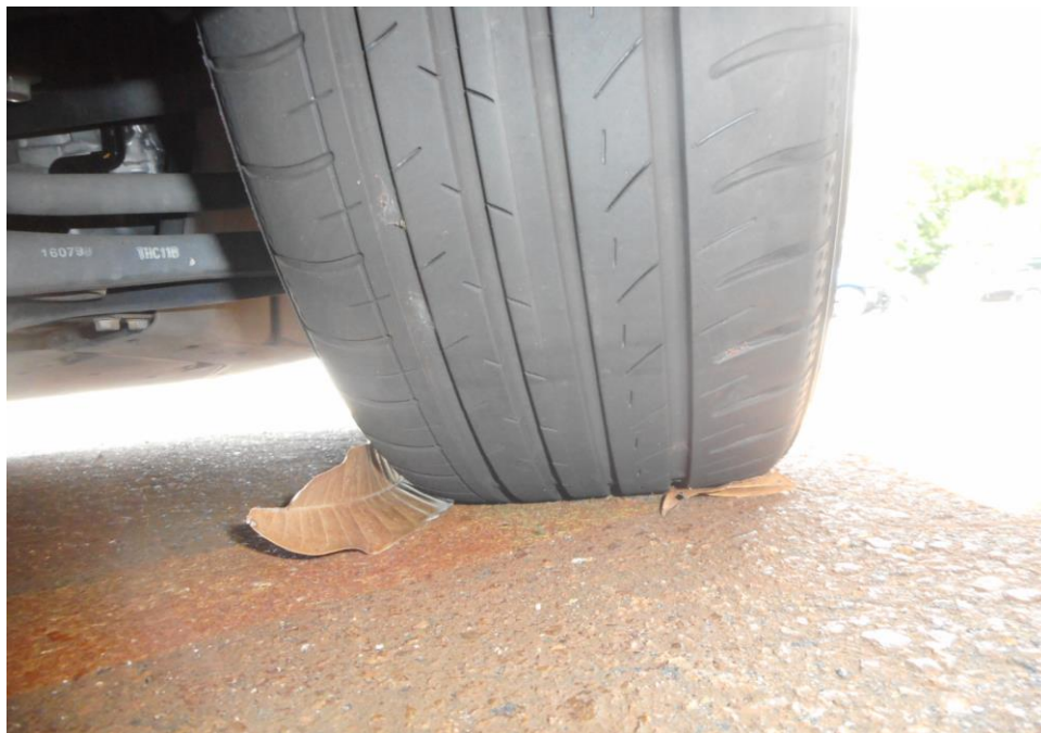
Photo 7 shows the condition of the front right tyre of the Motor Car, which was observed to be in serviceable condition with remaining tread depth of approximately 5.1mm. The tyre was sufficiently inflated for vehicular operation with no tear, cut or burst mark(s) on the outer and the inner sidewalls as well as across the tread. The 4 tyres of the Motor Car were wrapped around standard steel wheel rims without any damage.
