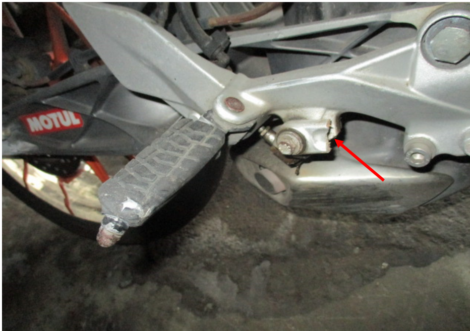
Photo 11 shows the broken rear brake pedal of the Motorcycle as a result of the accident (arrowed).
