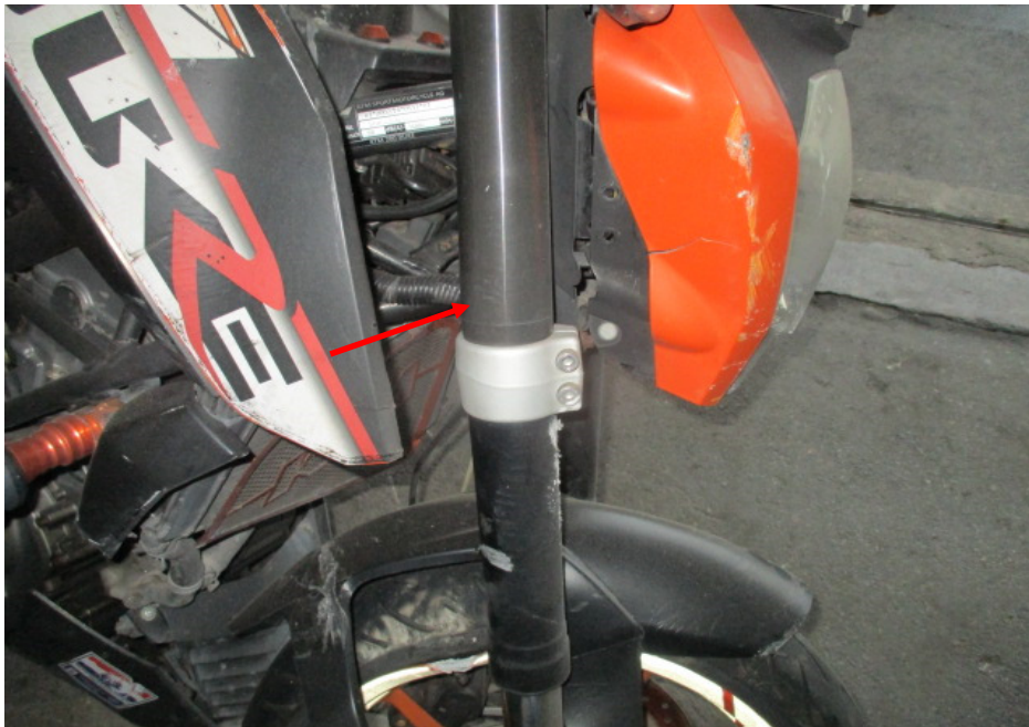
Photo 19 shows the front forks of the Motorcycle. The front right fork was observed to be bent inwards (arrowed) as a result of the accident. We were hence not able to conduct any tests on the steering system of the Motorcycle.
