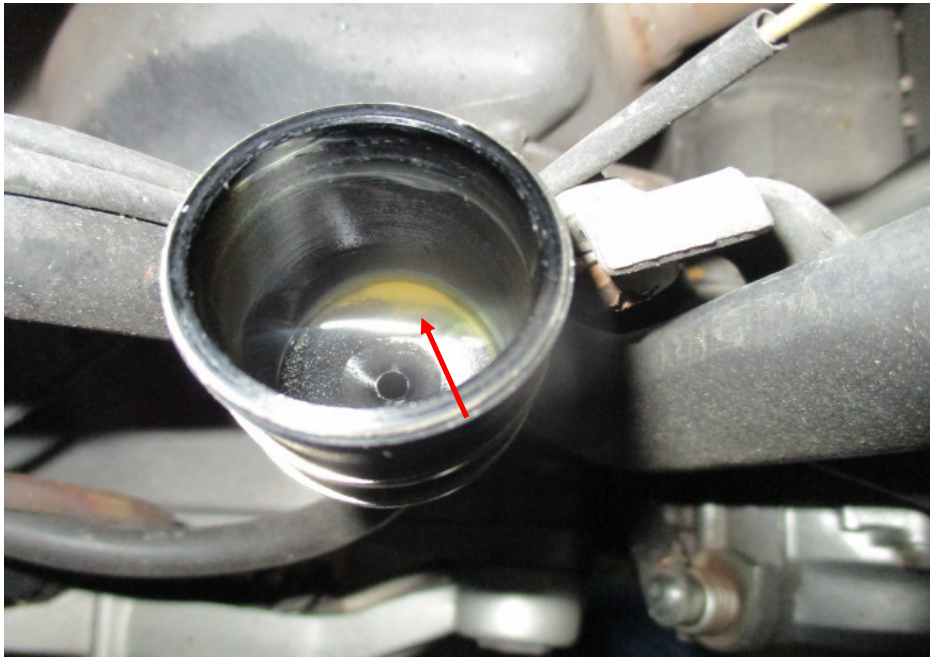
Photo 24 shows the brake fluid reservoir for the rear brake of the Motorcycle. The brake fluid was found to be of insufficient level for operating purposes (arrowed).
