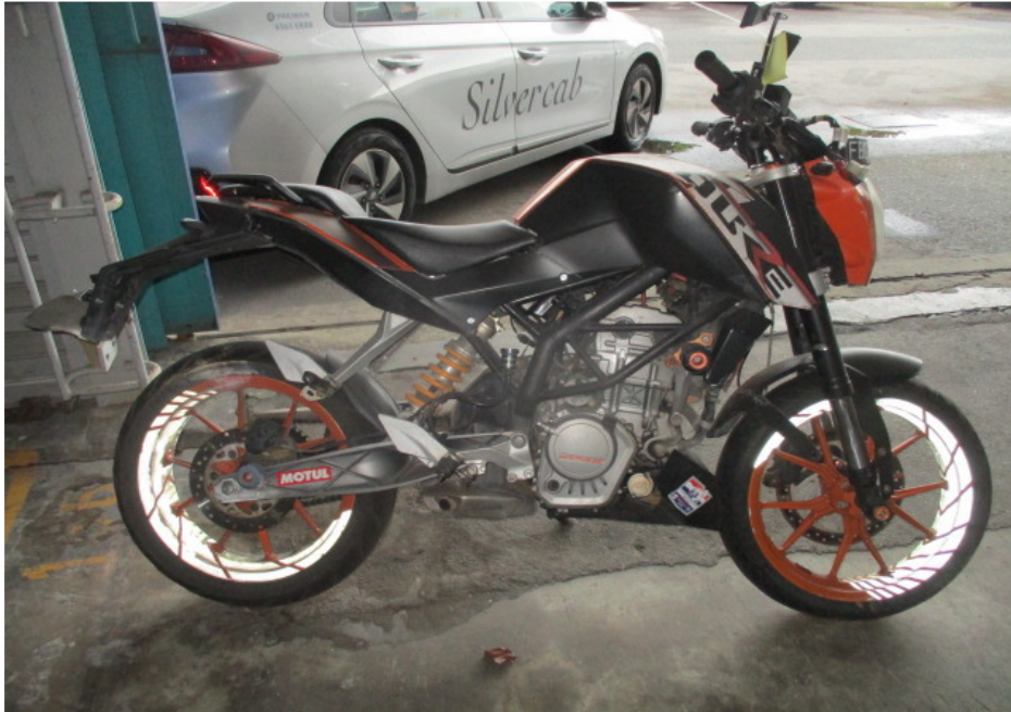
Photo 3 shows a general view of the right body of the Motorcycle at the time of our inspection. The Motorcycle had sustained damages all around. Body parts that were found to have been damaged include its headlight assembly, speedometer gauge, front fork assembly, front mudguard, left tank cover, side mirrors, front brake lever, clutch lever, handlebar ends, rear brake pedal, belly pan and right radiator cover, among others.
