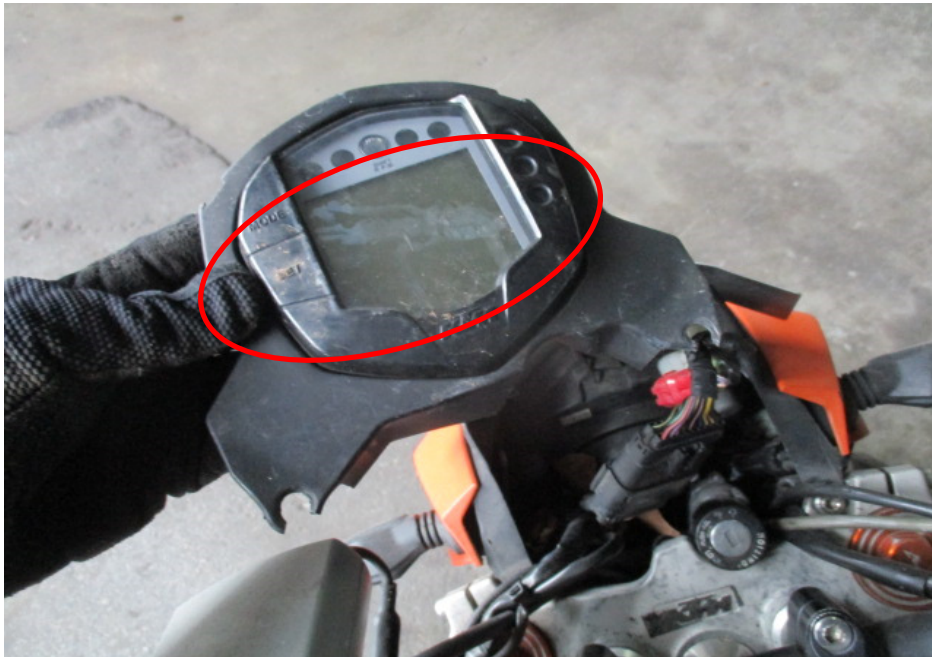
Photo 1 shows the mileage of the Motorcycle which could not be recorded at the time of our inspection due to the damaged speedometer gauge (circled).
