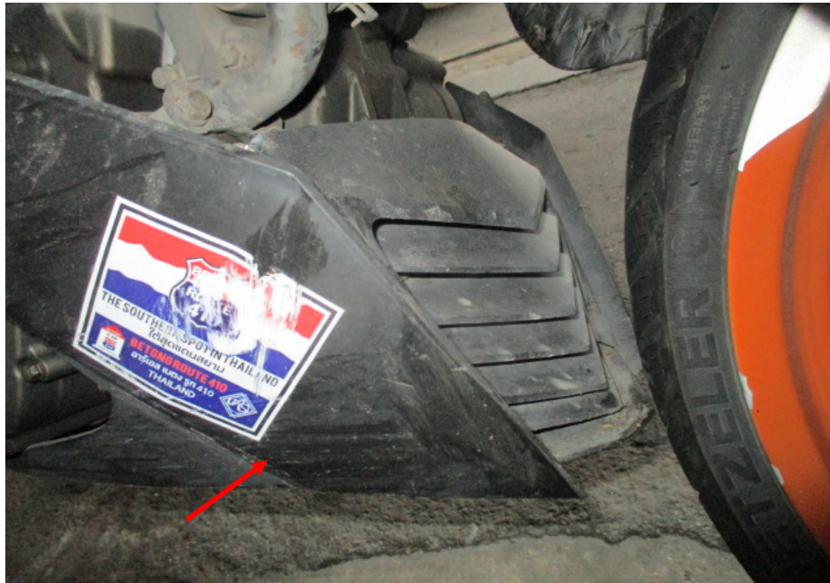
Photo 9 shows a closer view of the belly pan which was amongst the body parts at the front body of the Motorcycle that had sustained damages as a result of the accident (arrowed).
