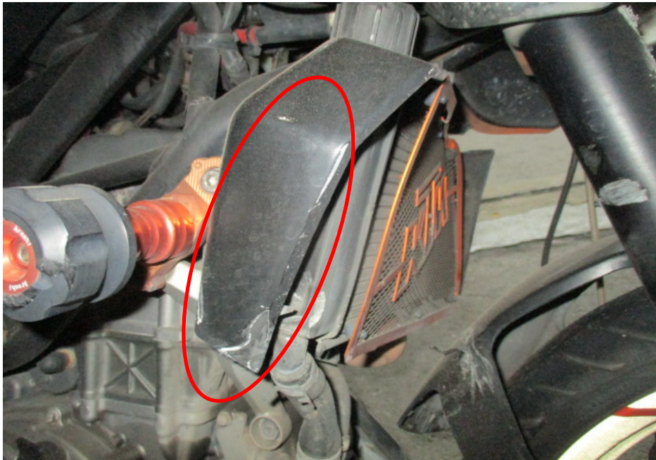
Photo 8 shows a closer view of the right radiator cover which was amongst the body parts at the rear body of the Motorcycle that had sustained damages as a result of the accident (circled).
