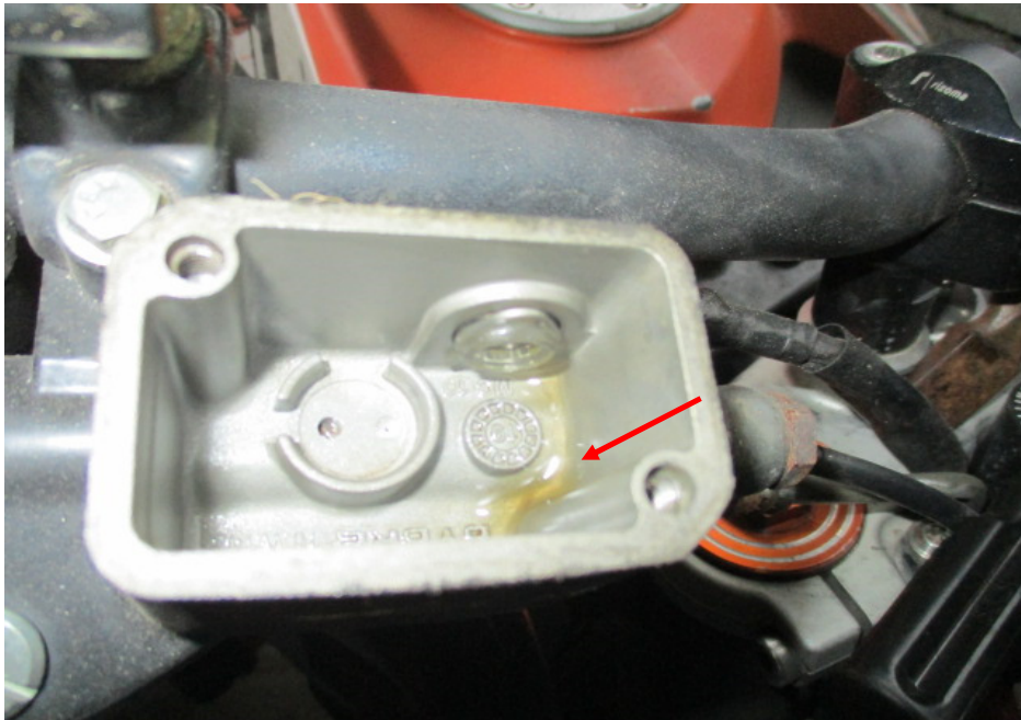
Photo 21 shows the brake fluid reservoir for the front brake of the Motorcycle. The brake fluid was found to be of insufficient level for operating purposes (arrowed).
