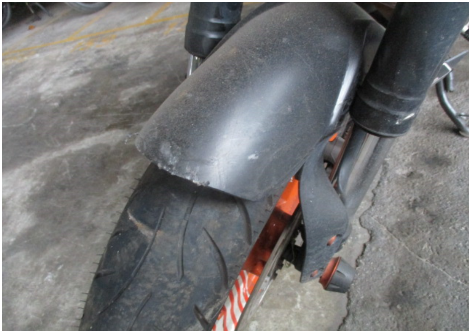
Photo 6 shows a closer view of the front mudguard, which was amongst the body parts of the Motorcycle that had sustained damage as a result of the accident.
