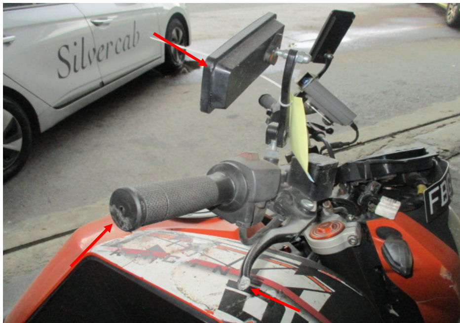
Photo 10 shows a closer view of the right side mirror and right handlebar end and front brake lever (arrowed), which were amongst the body parts of the Motorcycle that had sustained damage as a result of the accident.
