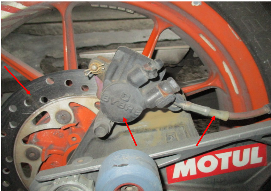
Photo 23 shows a close up view of the rear brake caliper, rear brake disc and rear brake hose (arrowed) of the Motorcycle, which are all part of the components in the hydraulic rear brake system of the Motorcycle. Our visual checks of these various components had revealed all to be intact with no visible damage. No leakage of brake fluid was also observed.
