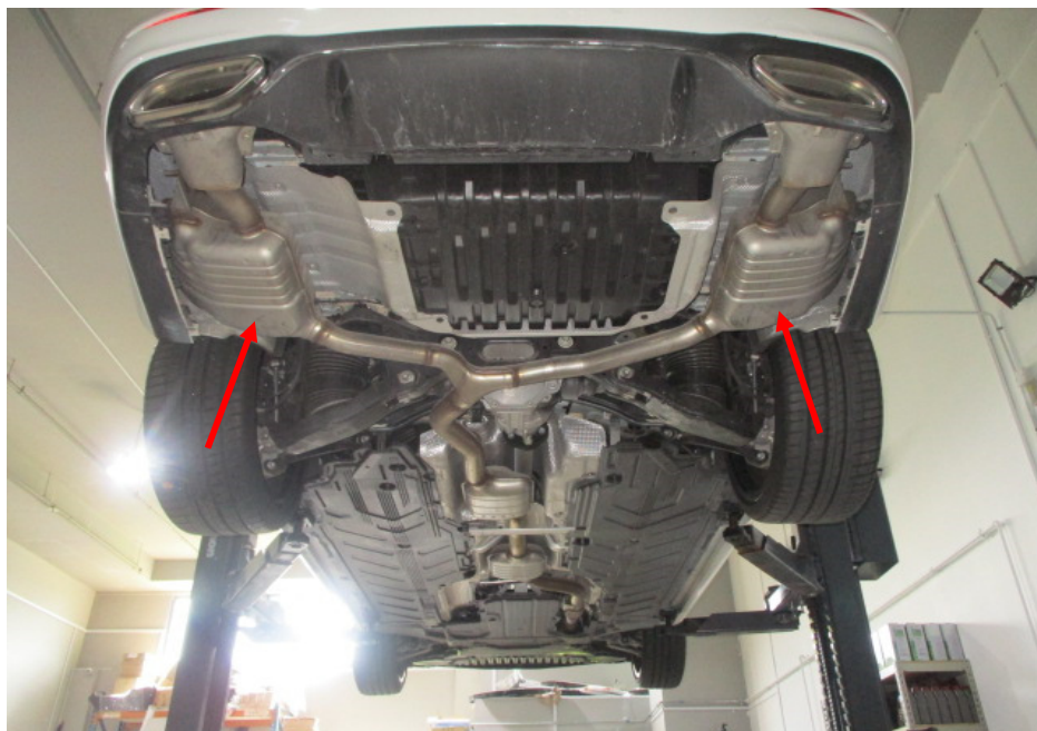
Photo 20 shows the Motor Car's rear exhaust mufflers (arrowed). My examination of the Motor Car's exhaust system revealed no sign(s) or indication(s) of any cut or weld marks along its exhaust pipes and on its catalytic converter.
