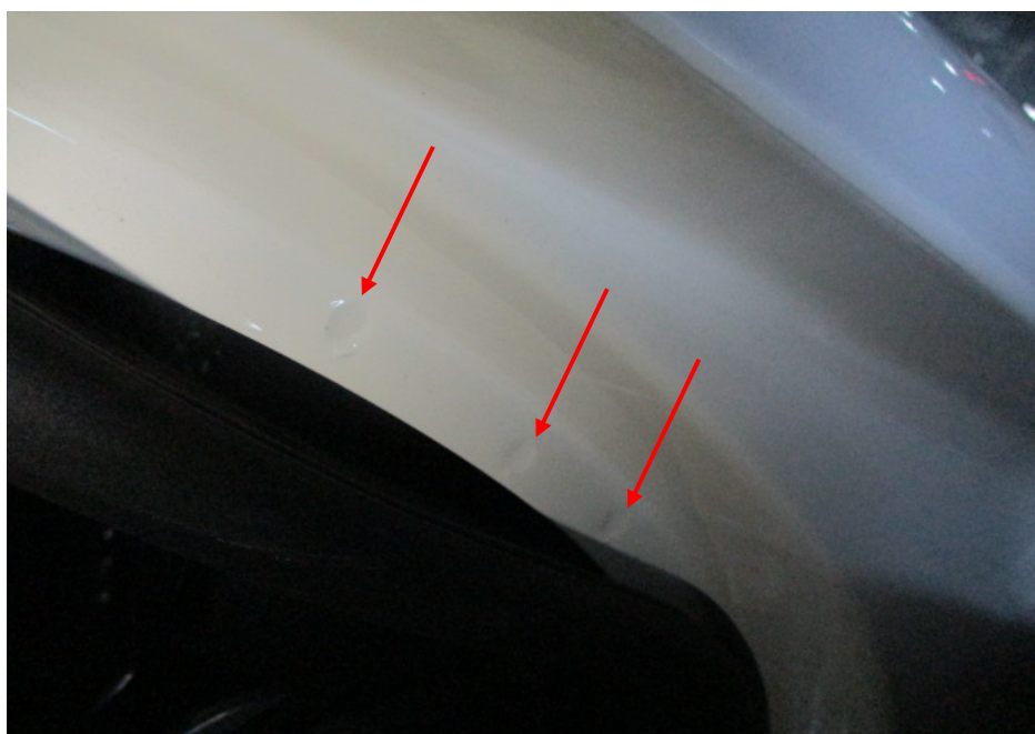
Photo 23 shows the right side "A" pillar of the Motor Car. I did not find any weld marks other than original spot weld marks (arrowed) on the right side "A" pillar of the Motor Car which, indicates that there was no re-welding works carried out. In general, I had found all the non-detachable body panels of the Motor Car to be originally fitted at the time of my inspection.
