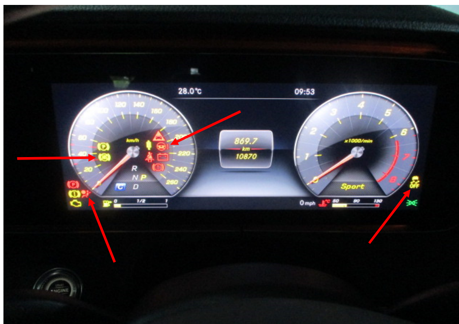
Photo 14 shows the warning lights for the various electronic safety features appearing on the instrument panel of the Motor Car during its self-test when the engine is cranked, in particular the ABS, SRS, EPS and TCS lights (arrowed).
