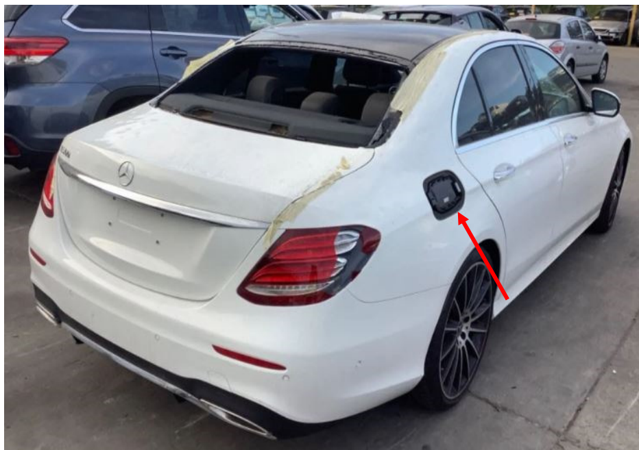
Photo 3 shows the rear right body of the Motor Car prior to any repairs being carried out (photograph provided to me). Relatively minor indentation damage was seen on the rear bootlid. The rear right taillamp was also observed to be broken. The fuel filler cover (arrowed) was observed to be either dislodged, removed or damaged.
