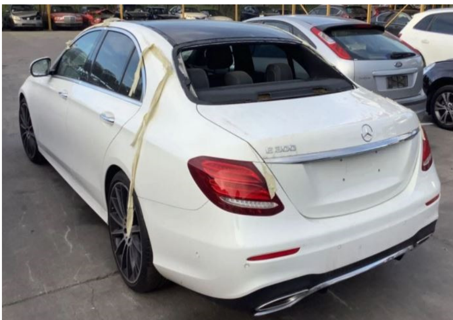
Photo 4 shows the rear left body of the Motor Car prior to any repairs being carried out (photograph provided to me). The Motor Car was observed to have sustained damages of indentation nature to multiple exterior body parts like its rear bootlid amongst others. The rear windscreen was also observed to be broken.
