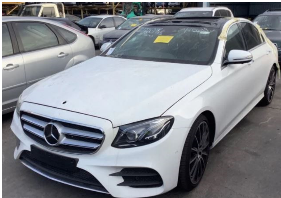
Photo 1 shows the front left body of the Motor Car prior to any repairs being carried out (photograph provided to me). The Motor Car was observed to have sustained damages of indentation nature to multiple exterior body parts like its front bonnet. The panoramic sunroof was also observed to be damaged.
