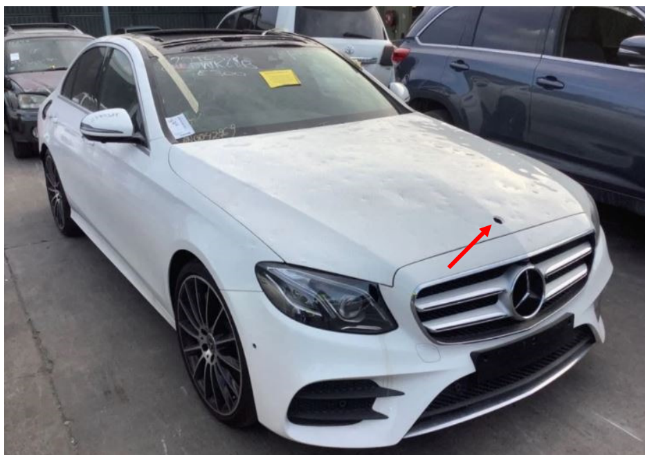
Photo 2 shows the front right body of the Motor Car prior to any repairs being carried out (photograph provided to me). The Motor Car was observed to have sustained damages of indentation nature to multiple exterior body parts like its front bonnet. As seen from the photograph, there were multiple relatively minor indentations on the front bonnet. The front bonnet emblem (arrowed) was observed to be either dislodged, removed or damaged.
