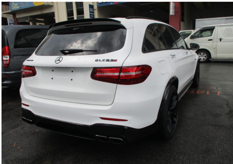
Photo 9 shows a general view of the rear right body of the Motor Car at the time of my inspection. The damaged parts at the rear right portion of the Motor Car, in particular the rear right wheel rim and rear right fender wheel arc garnish were visually examined, and it was observed that the repair/restoration works carried out to the damaged area of the Motor Car (refer to photograph 2 above) were reasonably adequate and in order.
