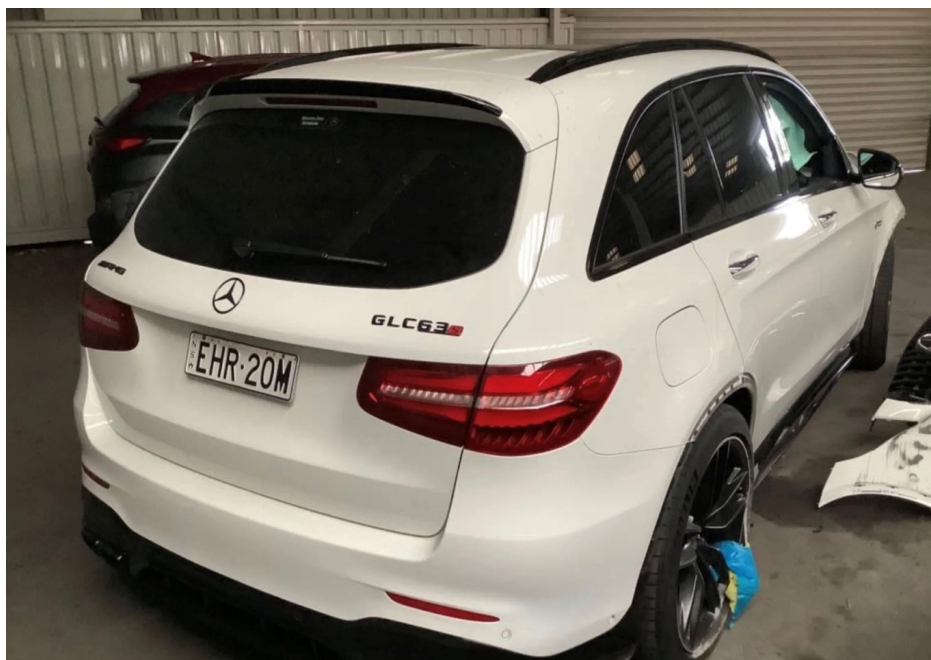
Photo 2 shows the rear right body of the Motor Car (photograph provided to me). Damage was seen to the rear right wheel rim. The rear right fender wheel arc garnish was observed to be either dislodged, removed or damaged.
