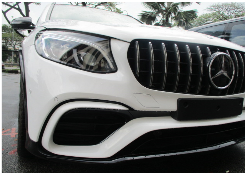
Photo 6 shows a closer view of the Motor Car's front bumper, front bumper right lower grille, front bumper lower lip and front right headlamp. The body parts at the front right portion of the Motor Car were visually examined and it was observed that the repair/restoration works carried out to the damaged area of the Motor Car (refer to photograph 1 above) were reasonably adequate and in order.
