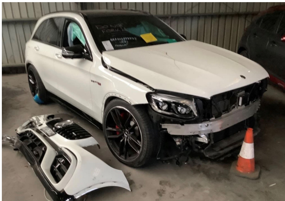
Photo 1 shows the front right body of the Motor Car (photograph provided to me). The Motor Car was observed to have sustained damage at its front right portion. Body parts damaged include the front bumper, front bumper right lower grille, front bumper centre lower grille, front bumper lower lip, front bumper reinforcement, front right headlamp, front bonnet, front right fender, front right fender inner shield and front right fender wheel arc garnish amongst others.
