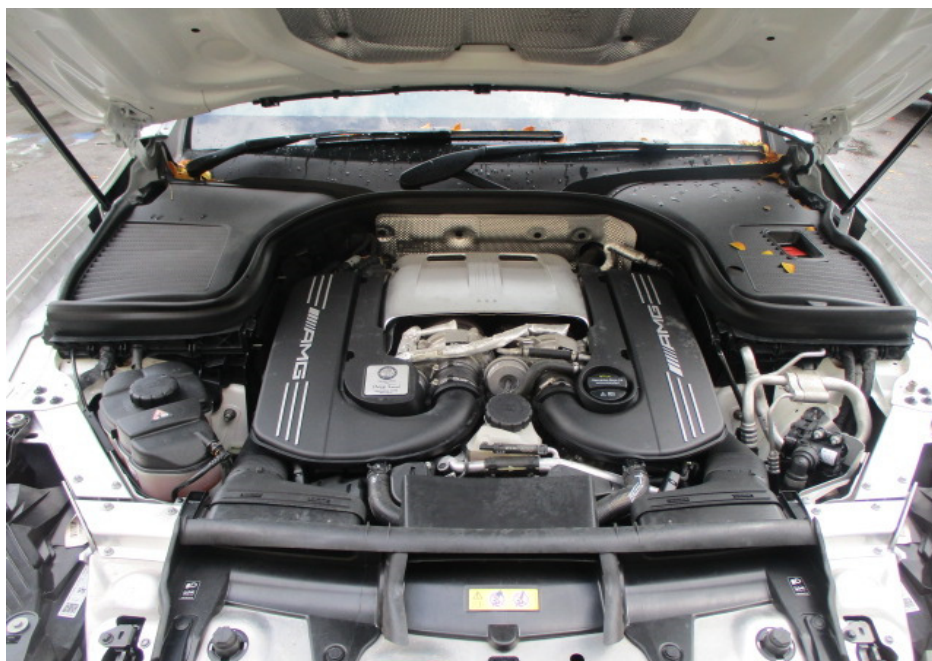
Photo 11 shows a general view of the engine compartment of the Motor Car at the time of my inspection. The various parts and components inside the engine compartment were all observed to be intact and properly fitted. There was also no sign(s) or indication(s) of fluid leak and/or fluid stain found inside the engine compartment.
