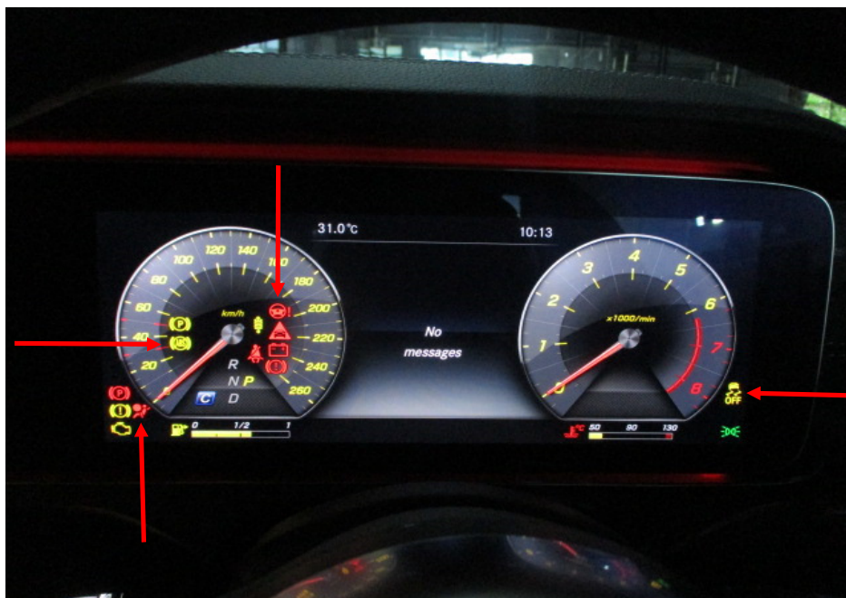
Photo 15 shows the warning lights for the various electronic safety features appearing on the instrument panel of the Motor Car during its self-test when the engine is cranked, in particular the ABS, SRS, EPS and TCS lights (arrowed).
