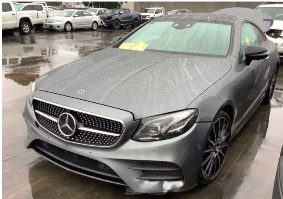
Photo 3 shows the front left body of the Motor Car prior to any repairs being carried out (photograph provided to me). The front bumper was observed to be dented at its left lower portion. The orientation of the front left wheel appears to be more towards the right as compared to the front right wheel (refer to photograph 4 below), suggesting possible damage to the front undercarriage of the Motor Car.
