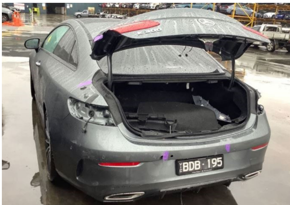
Photo 2 shows the rear left body of the Motor Car prior to any repairs being carried out (photograph provided to me). The Motor Car was observed to have sustained damages at its rear portion. The rear bumper, rear end panel and various inner trims within the rear boot compartment were observed to be damaged. The rear left taillamp was either dislodged, removed or damaged.
