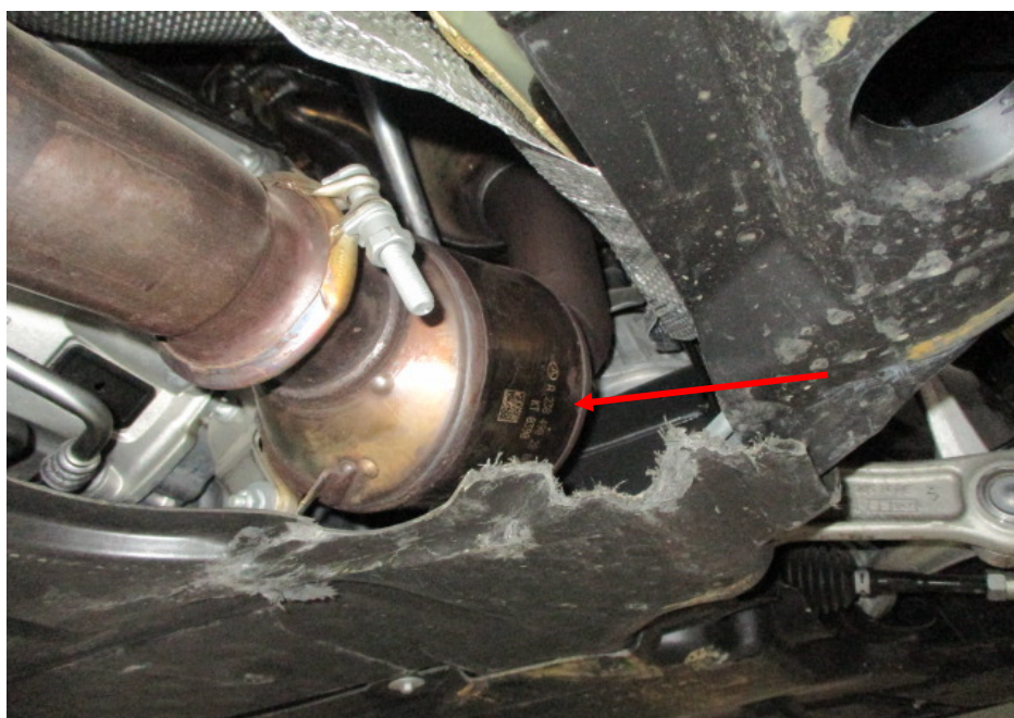
Photo 21 shows the Motor Car's catalytic converter (arrowed). My examination of the Motor Car's exhaust system revealed no sign(s) or indication(s) of any cut or weld marks along its exhaust pipes and on its rear mufflers.
