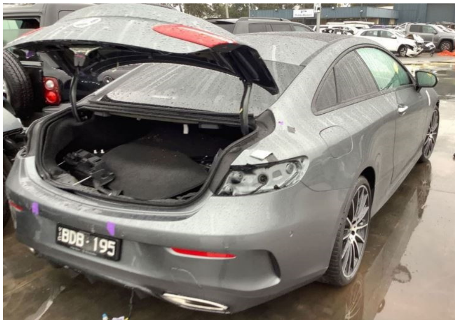
Photo 1 shows the rear right body of the Motor Car prior to any repairs being carried out (photograph provided to me). The Motor Car was observed to have sustained damages at its rear portion. The rear bootlid weatherstrip and various inner trims within the rear boot compartment were observed to be damaged. The rear right taillamp was either dislodged, removed or damaged.
