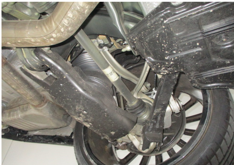
Photo 18 shows a general view of the control arms and linkages at the rear left wheel of the Motor Car. I did not observe any fluid leak and/or fluid stain on the underside of the Motor Car. All the Motor Car's undercarriage components were observed to be intact and secured in an appropriate manner.
