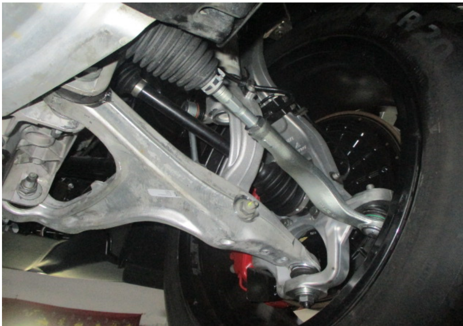
Photo 19 shows the various undercarriage components at the front right wheel of the Motor Car. The mechanical components, control arms and linkages were all found to be intact and secured in an appropriate manner.
