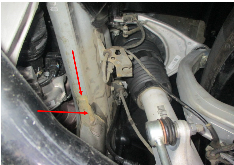
Photo 24 shows the chassis/structural body at the underside front left of the Motor Car. The original factory sealant (arrowed) at the joints along the chassis/structural body was observed to be untouched. In general, I had found no work was carried out on the chassis/structural body of the Motor Car. The chassis/structural body of the Motor Ca was originally fitted.
