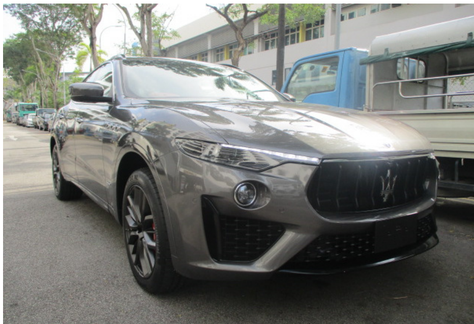
Photo 7 shows a general view of the front right body of the Motor Car at the time of my inspection. The Motor Car was observed to be in a relatively good general condition with no loose exterior fittings observed. The body parts at the front right portion of the Motor Car were visually examined and it was observed that the repair/restoration works carried out to the damaged area of the Motor Car (refer to photograph 1 above) were reasonably adequate and in order.
