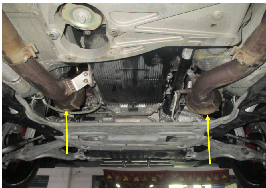
Photo 21 shows the Motor Car's catalytic converters (arrowed). My examination of the Motor Car's exhaust system revealed no sign(s) or indication(s) of any cut or weld marks along its exhaust pipes and on its rear mufflers.
