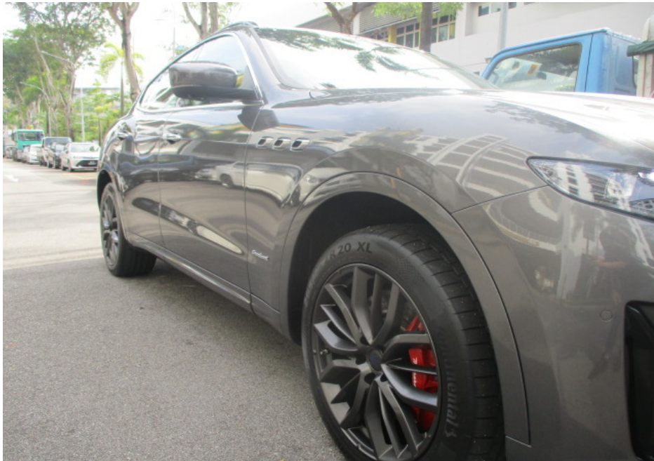
Photo 8 shows a closer view of the front bumper, front right headlamp, front right fender wheel arc garnish and front right wheel of the Motor Car at the time of my inspection. The body parts at the front right portion of the Motor Car were visually examined and it was observed that the repair/restoration works carried out to the damaged area of the Motor Car (refer to photograph 1 above) were reasonably adequate and in order.
