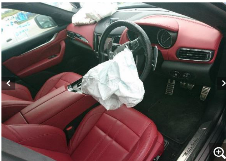
Photo 6 shows a general view of the interior compartment of the Motor Car (photograph provided to me). The driver's airbag and front left passenger airbag were activated as seen from the photograph that was provided.
