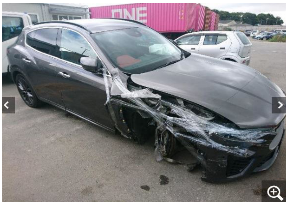
Photo 1 shows the front right body of the Motor Car (photograph provided to me). The Motor Car was observed to have sustained damage at its front right portion. The front bumper, front bumper right lower grille, front right headlamp, front right fender, front right fender inner panel, front right fender inner shield, front right fender wheel arc garnish, front right wheel rim and front bonnet were amongst the body parts that were observed to have been damaged. The front right undercarriage parts were also observed to be damaged.
