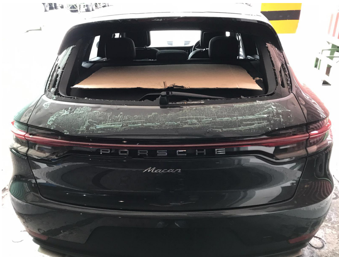
Photo 3 shows the rear body of the Motor Car prior to any repairs being carried out (photograph provided to me). The Motor Car was observed to have sustained damage of indentation nature to multiple exterior body parts like its rear tailgate. As seen from the photographs provided, the indentations were relatively minor. The rear windscreen glass was also observed to be broken.
