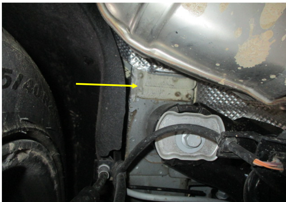
Photo 22 shows the chassis/structural body at the underside rear left of the Motor Car. I did not find any weld marks other than original spot weld marks on the chassis/structural body of the Motor Car. The original factory sealant (arrowed) at the joints along the chassis/structural body was also untouched. In general, I had found no work was carried out on the chassis/structural body of the Motor Car. The chassis/structural body of the Motor Car was originally fitted.
