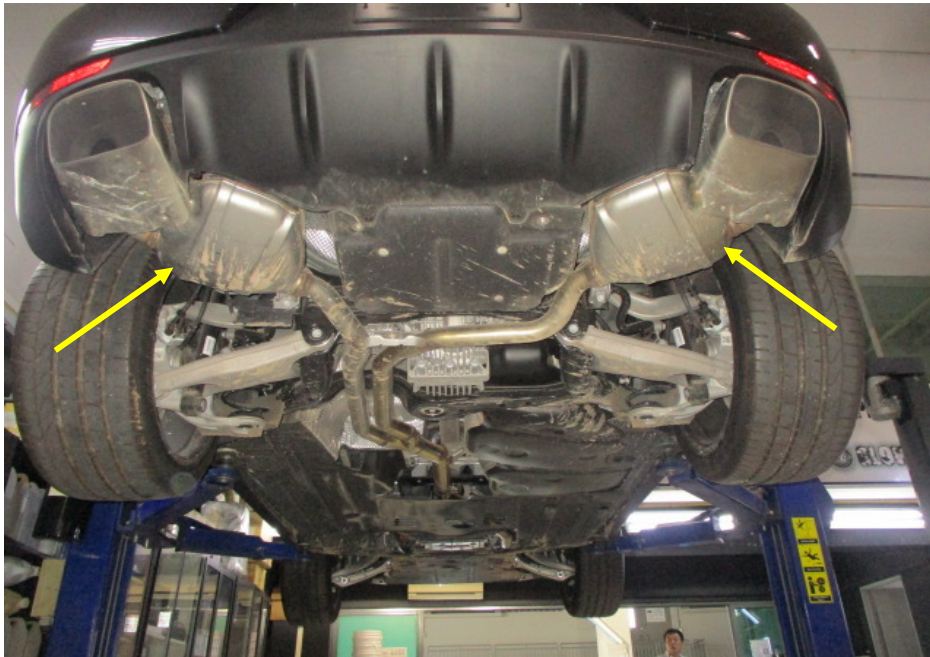
Photo 20 shows the Motor Car's rear mufflers (arrowed). My examination of the Motor Car's exhaust system revealed no sign(s) or indication(s) of any cut or weld marks along its exhaust pipes and on its catalytic converter.
