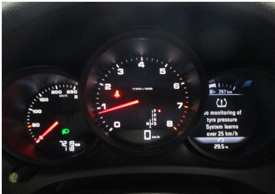
Photo 15 shows the respective warning lights no longer illuminated, indicating that there is no fault detected to the ABS, SRS, TPM and TCS systems of the Motor Car during the self-test. These electronic systems were hence in working condition at the time of my inspection.
