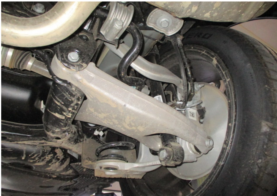
Photo 17 shows a general view of the control arms and linkages at the rear right wheel of the Motor Car. I did not observe any fluid leak and/or fluid stain on the underside of the Motor Car. All the Motor Car's undercarriage components were observed to be intact and secured in an appropriate manner.
