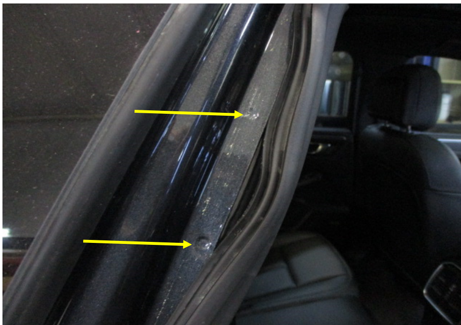
Photo 24 shows the right side “C” pillar of the Motor Car. I did not find any weld marks other than original spot weld marks (arrowed) on the right side “C” pillar of the Motor Car, which indicates that there was no re-welding works carried out. In general, I had found all the non-detachable body panels of the Motor Car to be originally fitted at the time of my inspection.
