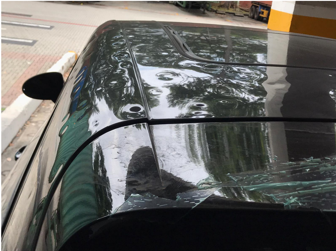
Photo 4 shows the roof panel of the Motor Car prior to any repairs being carried out (photograph provided to me). Relatively minor indentation damage was seen on the roof panel. The sunroof, as seen from the photograph, was unaffected.
