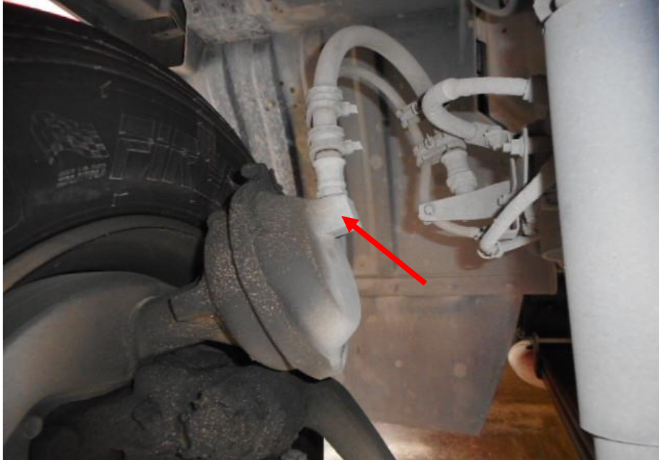
Photo 14 shows the brake air cylinder and air pipes (arrowed) at the front left wheel of the Lorry. My visual inspection of the mechanical components of the Lorry's braking system appear to suggest that its braking system was in serviceable condition at the material time of accident.
