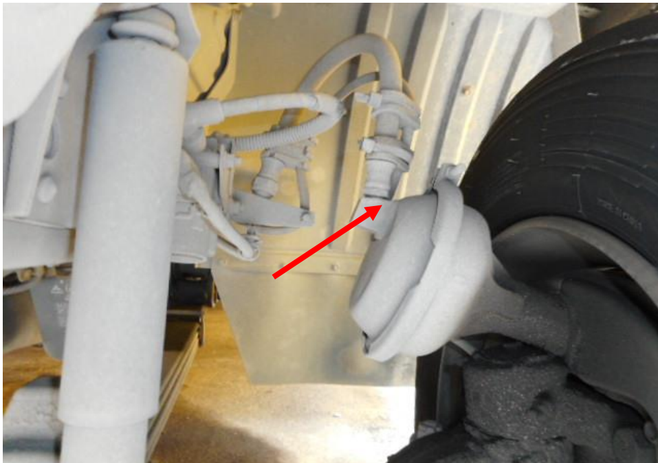
Photo 15 shows the brake air cylinder and air pipes (arrowed) at the front right wheel of the Lorry. My visual inspection of the mechanical components of the Lorry's braking system appear to suggest that its braking system was in serviceable condition at the material time of accident.
