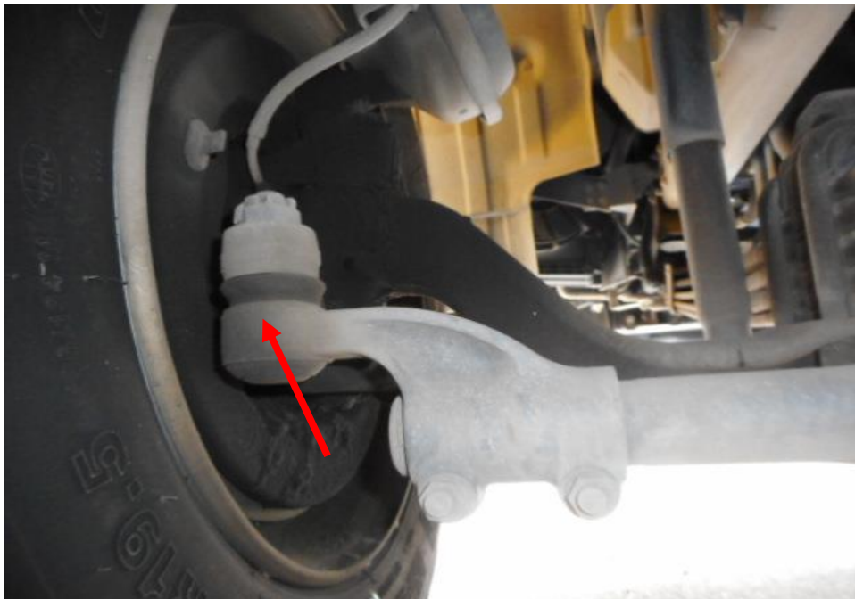
Photo 12 shows the undercarriage components at the front left wheel of the Lorry. The various undercarriage components of the Lorry were all observed to be intact and without any visible damage. This had included the steering rack and steering ball joints (arrowed) of the Lorry, which were observed to be securely attached to the front left wheel and front right wheel.
