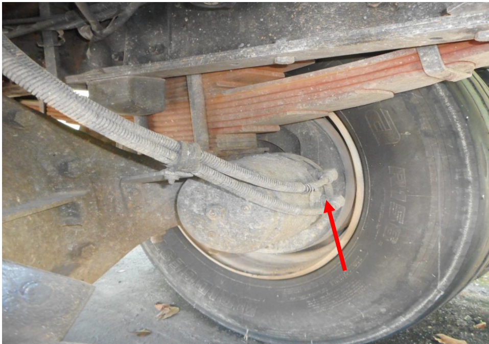
Photo 17 shows the brake air cylinder and air pipes (arrowed) at the front right wheel of the Lorry. My visual inspection of the mechanical components of the Lorry's braking system appear to suggest that its braking system was in serviceable condition at the material time of accident.
