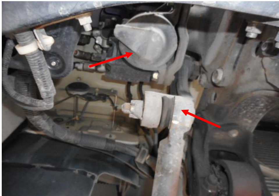
Photo 10 shows the front underside of the Lorry. I was not able to conduct any test(s) on the steering system of the Lorry as the engine of the Lorry could not be started. My visual checks on the various mechanical components of the steering system like the steering box, steering shaft and steering linkages (arrowed) amongst others revealed all to be intact and in good condition.
