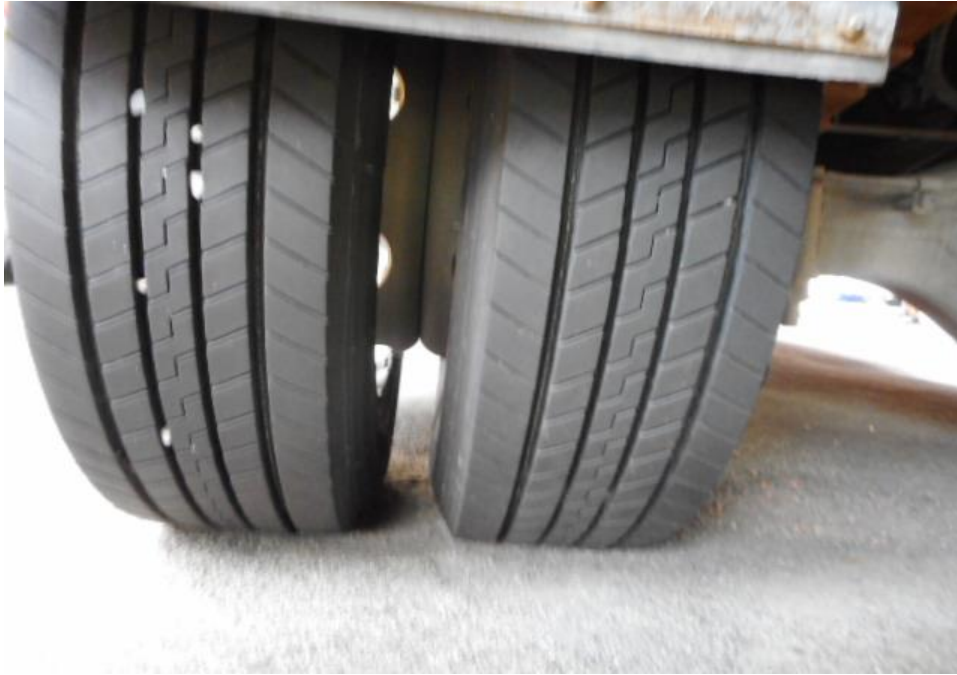
Photo 8 the condition of the rear left tyres of the Lorry, which was observed to be in serviceable condition with remaining, tread depth of approximately 9.1mm. The tyres, which were wrapped around standard steel wheel rim, were also observed to be sufficiently inflated for vehicular operation. There was also no damage found on all 6 steel wheel rims of the Lorry.
