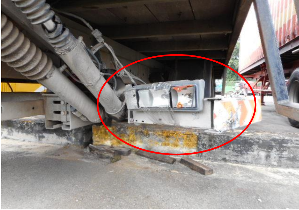
Photo 2 shows a close up view of the rear body of the Lorry at the time of my inspection. The Lorry was observed to have sustained damage at its rear right brake lamp (circled) as a result of the accident.
