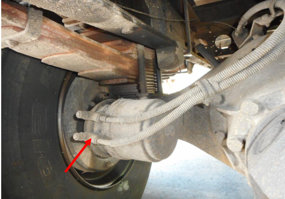
Photo 16 shows the brake air cylinder and air pipes (arrowed) at the rear left wheel of the Lorry. My visual inspection of the mechanical components of the Lorry's braking system appear to suggest that its braking system was in serviceable condition at the material time of accident.
