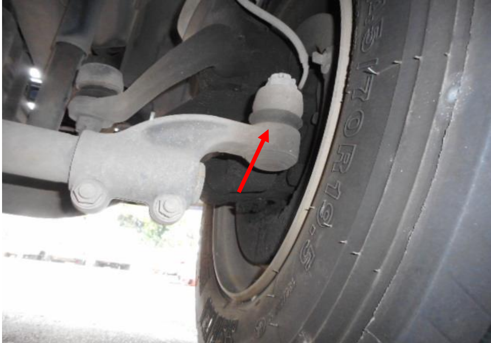
Photo 11 shows the undercarriage components at the front right wheel of the Lorry. The various undercarriage components of the Lorry were all observed to be intact and without any visible damage. This had included the steering rack and steering ball joints (arrowed) of the Lorry. Visual examinations of the mechanical components of the steering system appear to indicate that the Lorry's steering system was in serviceable condition.
