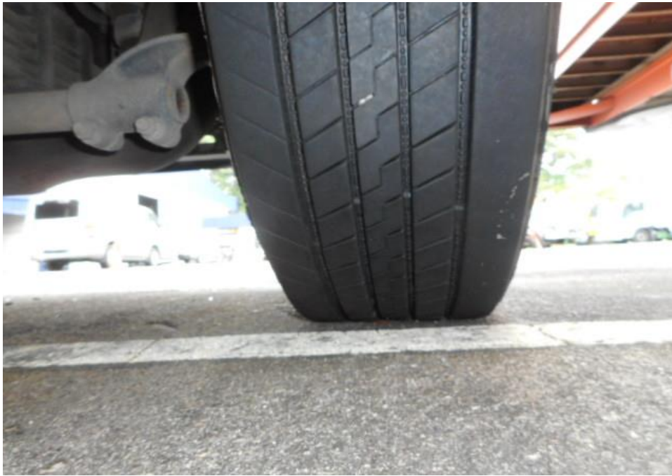
Photo 6 shows the condition of the front right tyre of the Lorry, which was observed to be in serviceable condition with remaining tread depth of approximately 9.4mm. The tyre, which was wrapped around standard steel wheel rim, was also observed to be sufficiently inflated for vehicular operation. There was no tear, cut or burst mark(s) on the outer and the inner sidewalls as well as across the tread of the 6 tyres that were fitted on the Lorry.
