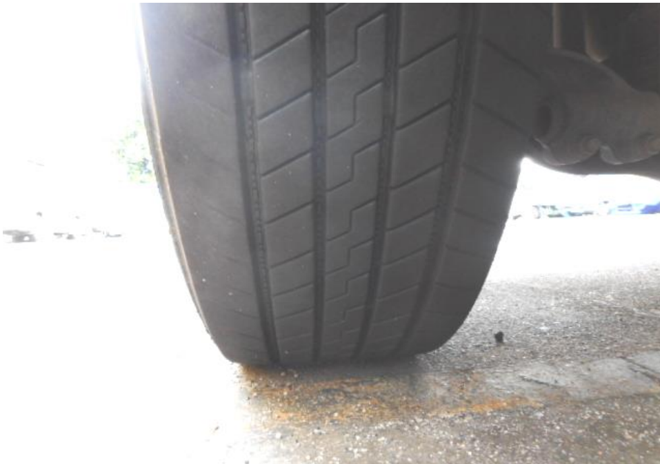
Photo 9 shows the condition of the front left tyre of the Lorry, which were observed to be in serviceable condition with remaining, tread depth of approximately 10.4mm. There was also no tear, cut or burst mark(s) on the outer and the inner sidewalls as well as across the tread of the 6 tyres that were fitted on the Lorry.
