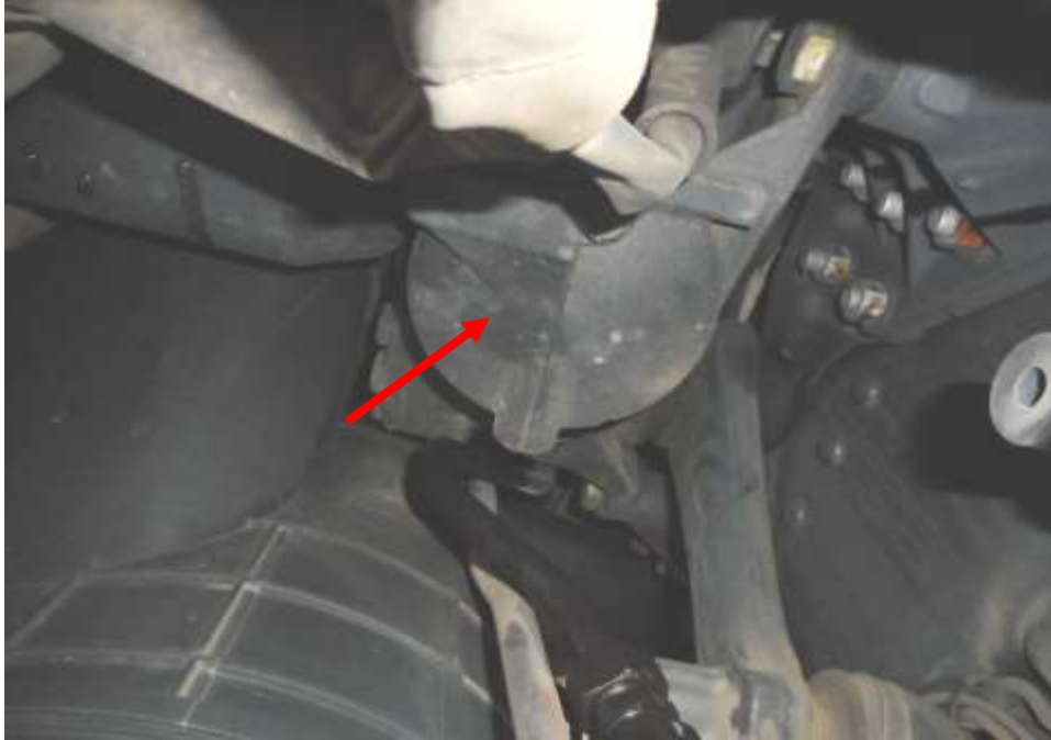
Photo 18 shows the steering box component (arrowed) at the undercarriage of the Trailer was found to be intact without any visible damage. There was also no sign of fluid stain(s) observed on the various undercarriage components.
