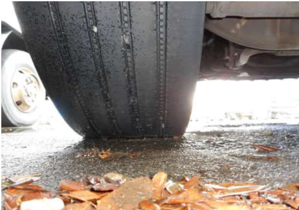
Photo 11 shows the condition of the rear right tyres of the Trailer, which were observed to be in serviceable condition with remaining, tread depth of approximately 6mm. There was also no tear, cut or burst mark(s) on the outer and the inner sidewalls as well as across the tread of the 6 tyres that were fitted on the Trailer.
