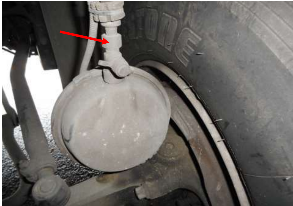
Photo 24 shows the brake hose/pipe (arrowed) at the front right wheel of the Trailer. My static tests of the Motor Bus's braking system, along with my visual examination of the various mechanical components in the braking system had indicated that there was no internal leakage of pressure/vacuum. Hence the braking system of the Motor Bus was likely to be in serviceable condition at the material time of accident.
