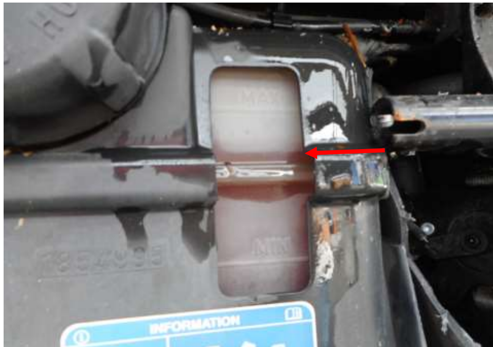
Photo 14 shows the engine coolant reservoir of the Trailer at the time of my inspection. The engine coolant was observed to be of sufficient level (arrowed) and without any visible contamination.
