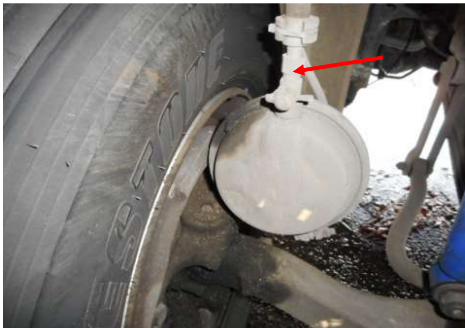
Photo 25 shows the brake hose/pipe (arrowed) at the front left wheel of the Trailer. My static tests of the Motor Bus's braking system, along with my visual examination of the various mechanical components in the braking system had indicated that there was no internal leakage of pressure/vacuum. Hence the braking system of the Motor Bus was likely to be in serviceable condition at the material time of accident.
