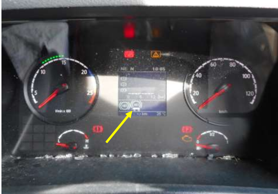
Photo 27 shows the warning light for Anti-Lock Brake System (ABS) (arrowed) appearing on the instrument panel of the Trailer during the self-test of its various electronic operating systems when its engine was cranked.
