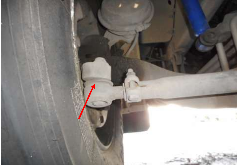
Photo 20 shows the various undercarriage components at the front left wheel of the Trailer, in particular the steering tie rod end (arrowed). The various undercarriage components of the Trailer were all found to be intact without any visible damage. There was also no sign of fluid stain(s) observed on the various undercarriage components.
