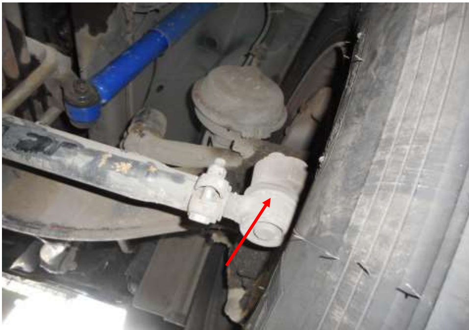
Photo 19 shows the various undercarriage components at the front right wheel of the Trailer, in particular the steering tie rod end (arrowed). The various steering components were all found to be intact, suggesting that the steering system of the Trailer was likely to be in serviceable condition at the material time of accident. There was also no sign of fluid stain(s) observed on the various undercarriage components.
