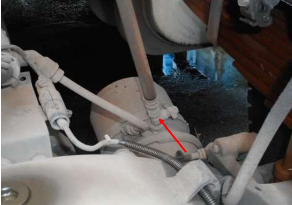
Photo 22 shows the brake pipe (arrowed) at the rear right wheel of the Trailer. I did not observe any leakage of brake fluid at the time of my inspection of the Trailer. My static tests of the Trailer's braking system, along with my visual examination of the various mechanical components in the braking system, had indicated that there was no internal leakage of pressure/vacuum. Hence the braking system of the Trailer was likely to be in serviceable condition at the material time of accident.
