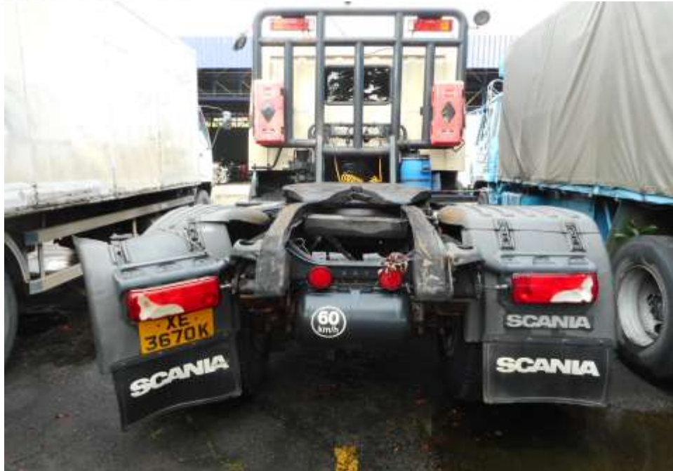
Photo 4 shows a general view of the Trailer's rear portion at the time of my inspection. It appeared to have sustained damage at its rear portion. Its rear mud guard was damage at the time of my inspection as a result of the accident.
