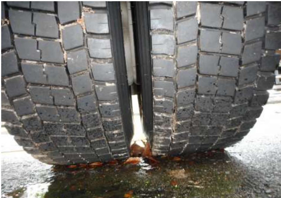
Photo 9 shows the condition of the rear right tyre of the Trailer, which was observed to be in serviceable condition with remaining tread depth of approximately 13.5mm. The tyre, which was wrapped around standard steel wheel rim, it was observed to be sufficiently inflated for vehicular operation.
