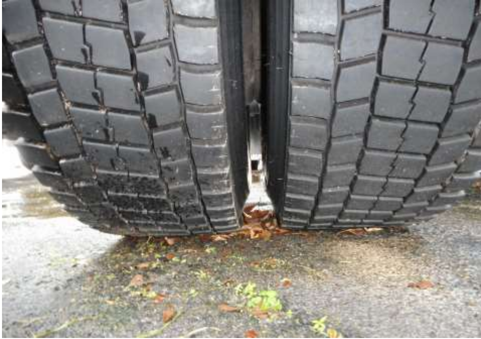
Photo 10 shows the condition of the rear left tyres of the Trailer, which was observed to be in serviceable condition with remaining tread depth of approximately 11.6mm. The tyres, which were wrapped around standard steel wheel rim, were also observed to be sufficiently inflated for vehicular operation. There was also no damage found on all 6 steel wheel rims of the Trailer.
