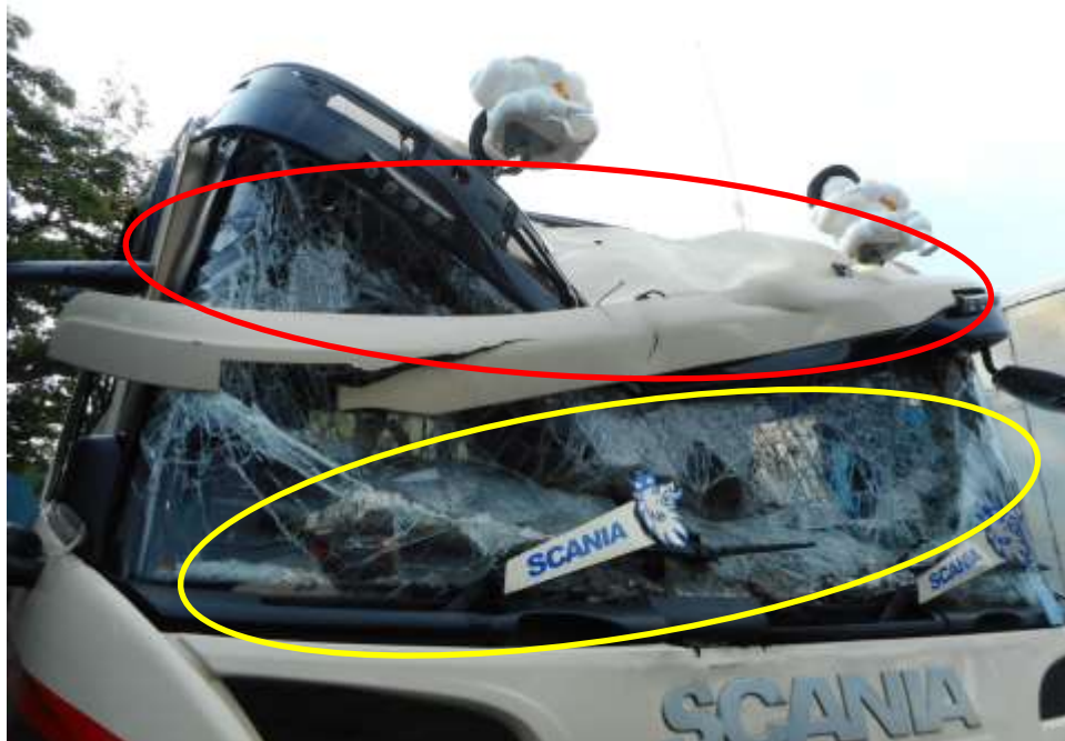
Photo 3 shows a close up view of the Trailer's front portion at the time of my inspection. It appeared to have sustained damage at its front portion. Its front windscreen (yellow circle) and front cabin panel (red circle) was damage at the time of my inspection as a result of the accident.
