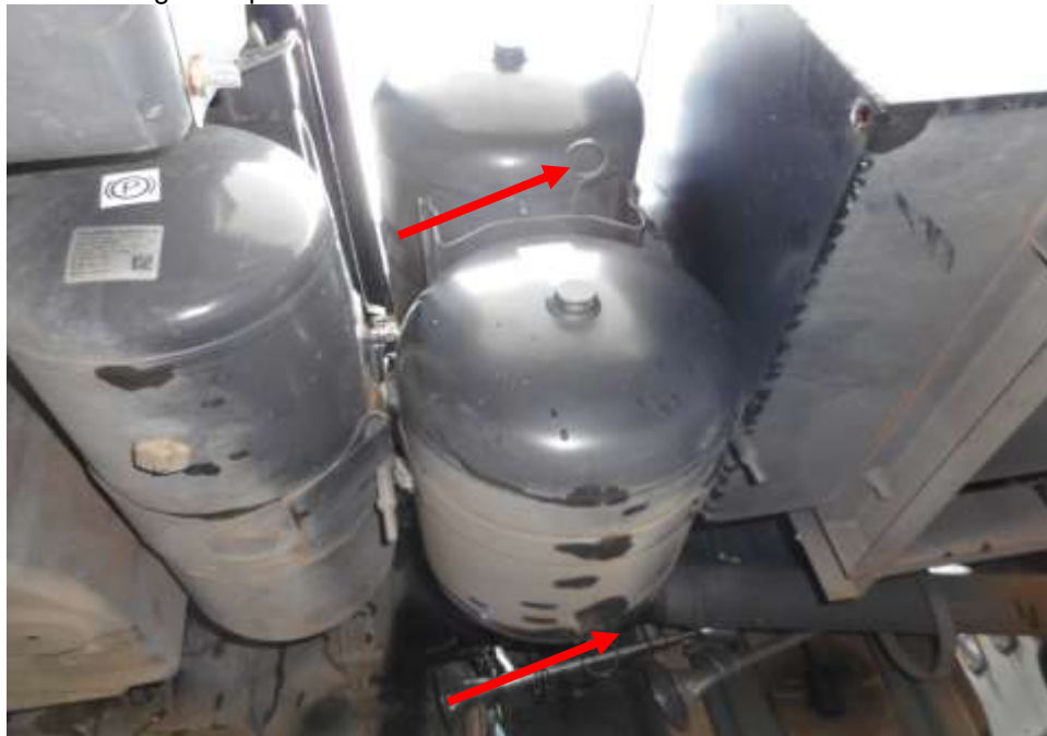
Photo 21 shows the air brake cylinders (arrowed) at the undercarriage of the Trailer. I did not observe any leakage of air brake fluid at the time of my inspection of the Trailer. My static tests of the Trailer's braking system, along with my visual examination of the various mechanical components in the braking system had indicated that there was no internal leakage of pressure/vacuum. Hence the braking system of the v was likely to be in serviceable condition at the material time of accident.
