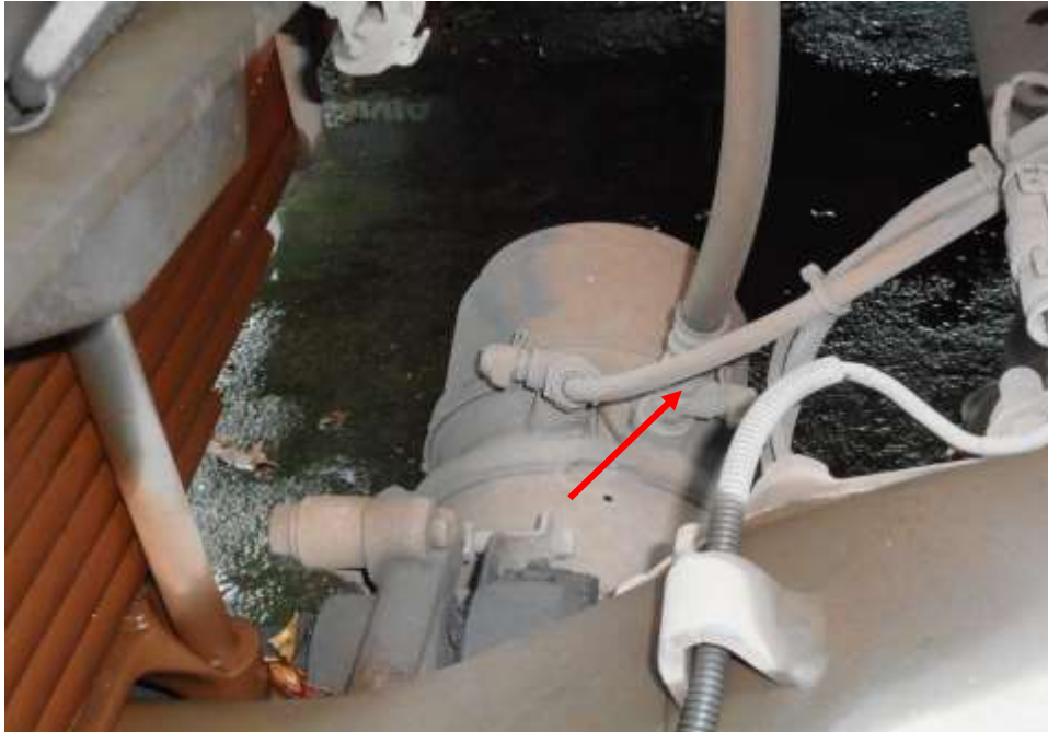
Photo 23 shows the brake pipe (arrowed) at the rear left wheel of the Trailer. I did not observe any leakage of brake fluid at the time of my inspection of the Trailer. My static tests of the Trailer's braking system, along with my visual examination of the various mechanical components in the braking system had indicated that there was no internal leakage of pressure/vacuum. Hence the braking system of the Trailer was likely to be in serviceable condition at the material time of accident.
