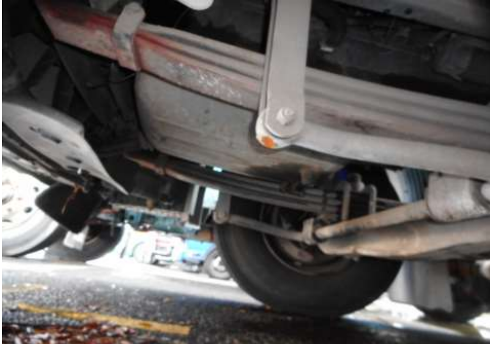
Photo 17 shows the undercarriage of the Trailer, at the area where the engine housing and transmission housing are located. I did not find any sign(s) or indication(s) of fluid leak and/or fluid stain(s) on the underside of the Trailer.
