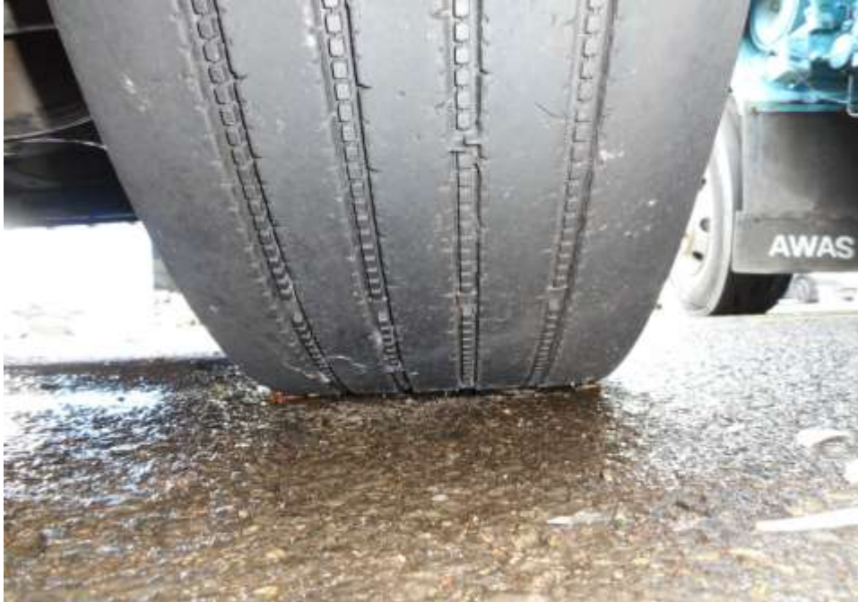
Photo 8 shows the condition of the front right tyre of the Trailer, which was observed to be in serviceable condition with remaining tread depth of approximately 5.6mm. The tyre, which was wrapped around standard steel wheel rim, was also observed to be sufficiently inflated for vehicular operation. There was no tear, cut or burst mark(s) on the outer and the inner sidewalls as well as across the tread of the 6 tyres that were fitted on the Trailer.
