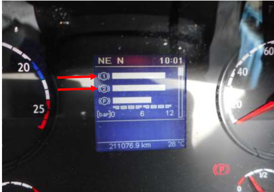
Photo 13 shows the air in the air brake cylinder of the Motor Bus at the time of my inspection. The air in the cylinder was observed to be of sufficient level & serviceable at the time of the accident.
