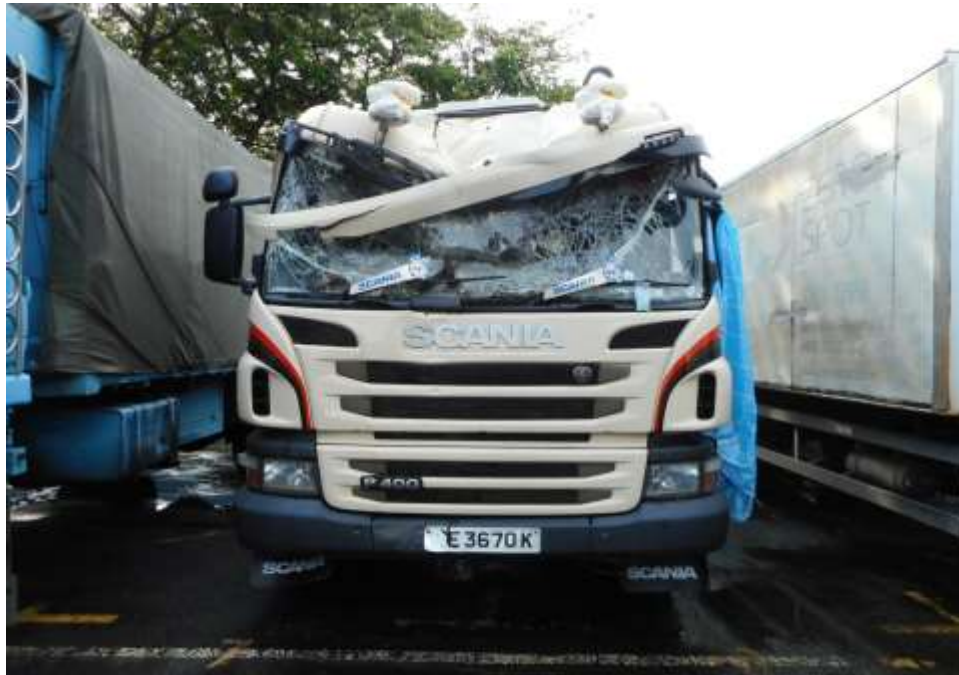
Photo 2 shows a general view of the Trailer's frontal portion at the time of my inspection. It appeared to have sustained damage at its front and rear portion. Its front windscreen, front cabin panel and rear left mud guard were damage at the time of my inspection.
