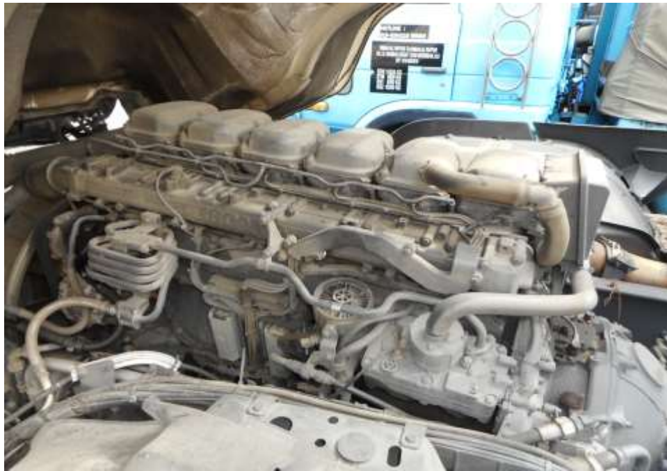
Photo 12 shows a general view of the Trailer's engine compartment, which was accessed by lifting the front cabin of the Trailer. The various parts and components inside the engine compartment were unaffected by the accident. There was also no sign(s) or indication(s) of fresh fluid leakage and/or fluid stain within the engine compartment
