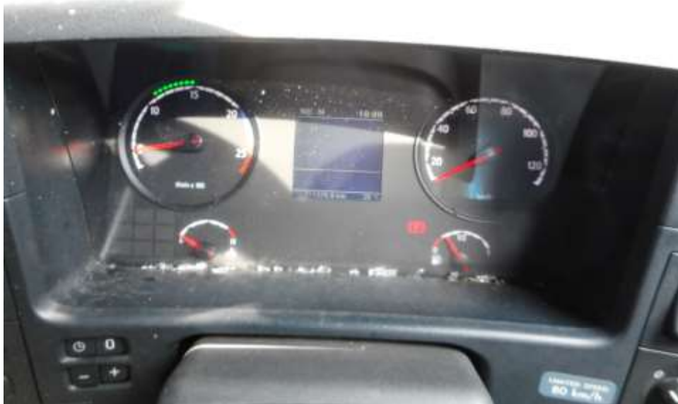
Photo 28 shows no warning lights illuminated on the instrument panel of the Trailer after the engine was cranked. This would suggest that there was no abnormality to the various electronic operating systems of the Trailer, like the ABS.
