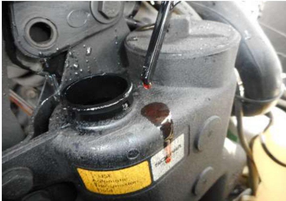
Photo 16 shows the power steering fluid reservoir of the Trailer at the time of my inspection. The power steering fluid was observed to be of sufficient level and without any visible contamination.
