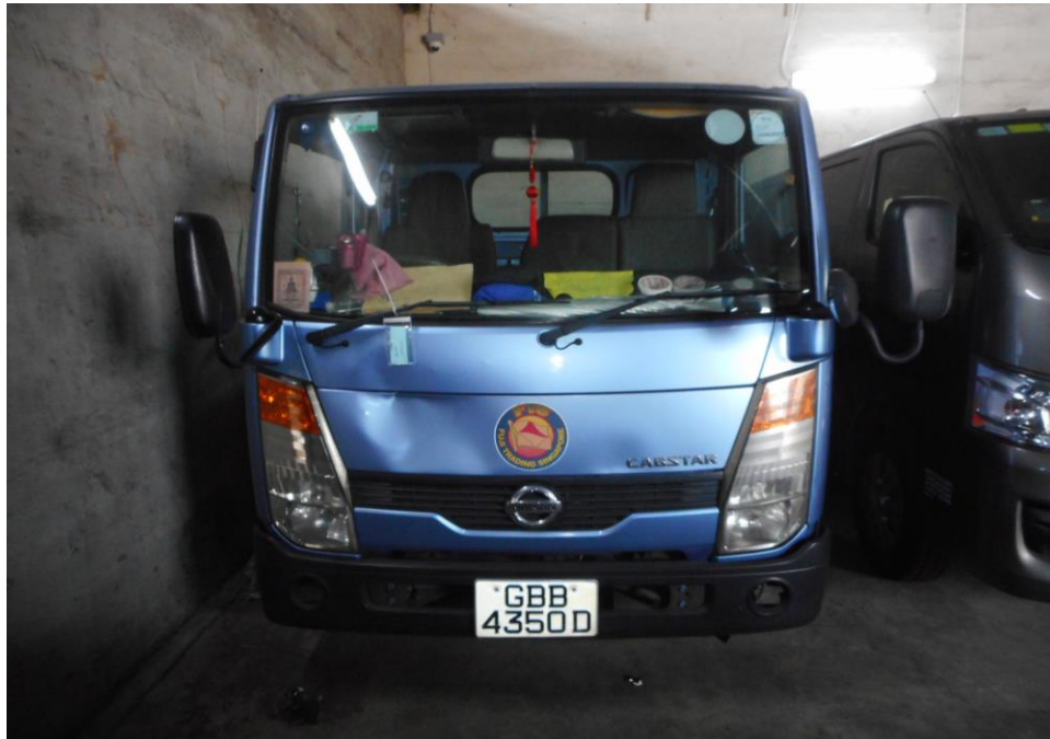
Photo 2 shows a general view of the Motor Lorry's frontal portion at the time of my inspection. It appeared to have sustained damage at its frontal portion. Its front body panel and front windscreen were damage at the time of my inspection.
