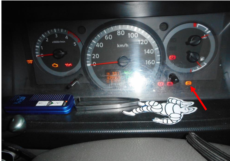
Photo 23 shows the warning light for Anti-Lock Brake System (ABS) (arrowed) appearing on the instrument panel of the Motor Lorry during the self-test of its various electronic operating systems when its engine was cranked.
