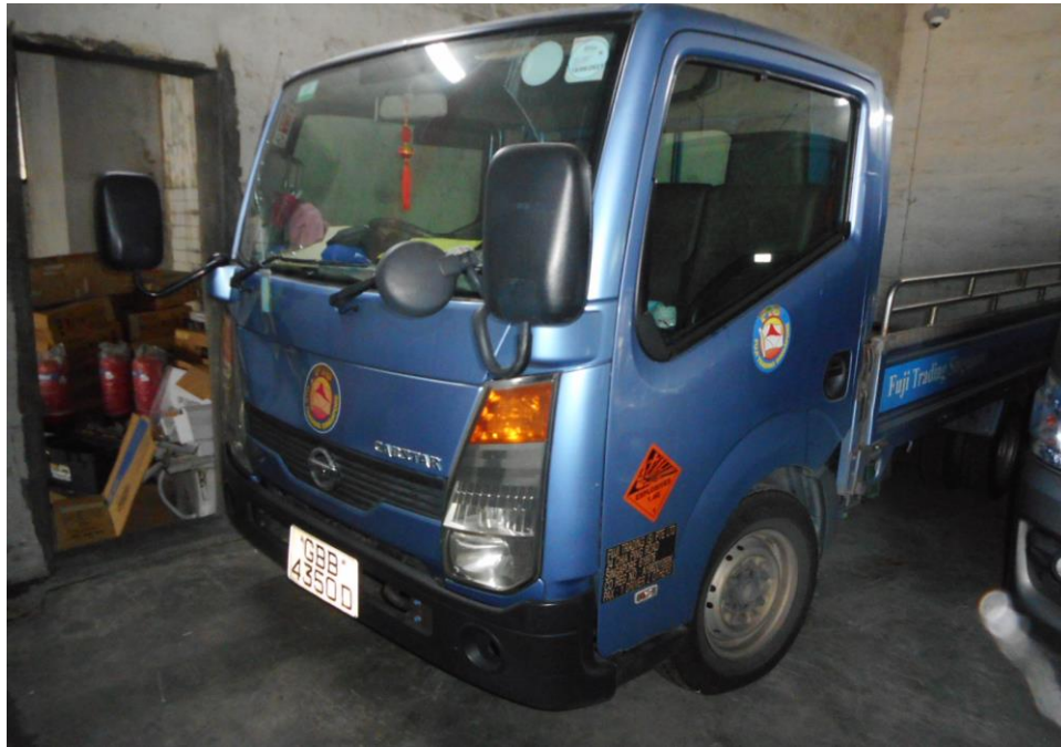
Photo 22 shows the front left wheel of the Motor Lorry turned to its right. During my steering system test, I did not experience any abnormal free play and/or resistance when I had turned the steering wheel towards full left and full right. This would suggest that the steering system of the Motor Lorry was likely to be in serviceable condition at the material time of accident.
