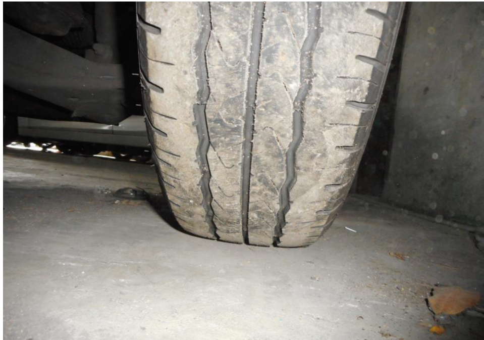
Photo 7 shows the condition of the front right tyre of the Motor Lorry, which was observed to be in serviceable condition with remaining tread depth of approximately 5.2mm. The tyre, which was wrapped around standard steel wheel rim, was also observed to be sufficiently inflated for vehicular operation. There was no tear, cut or burst mark(s) on the outer and the inner sidewalls as well as across the tread of the 4 tyres that were fitted on the Motor Lorry.
