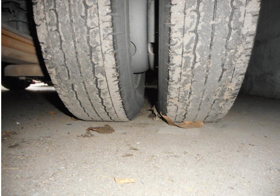
Photo 8 shows the condition of the rear right tyre of the Motor Lorry, which was observed to be in serviceable condition with remaining tread depth of approximately 2mm. The tyre, which was wrapped around standard steel wheel rim, it was observed to be sufficiently inflated for vehicular operation.
