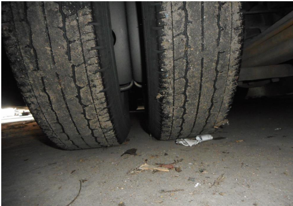
Photo 9 shows the condition of the rear left tyres of the Motor Lorry, which was observed to be in serviceable condition with remaining tread depth of approximately 1.6mm. The tyres, which were wrapped around standard steel wheel rim, were also observed to be sufficiently inflated for vehicular operation. There was also no damage found on all 4 steel wheel rims of the Motor Lorry.
