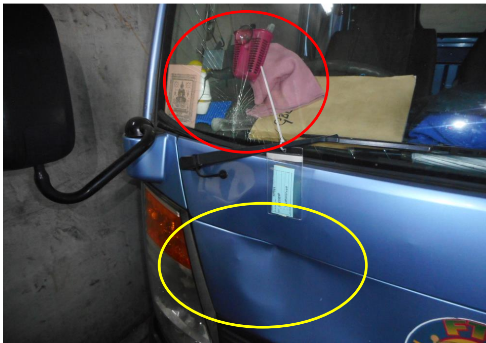
Photo 3 shows a close up view of the Motor Lorry's frontal portion at the time of my inspection. It appeared to have sustained damage at its frontal portion. Its front body panel (yellow circle) and front windscreen (red circle) was damage at the time of my inspection as a result of the accident.
