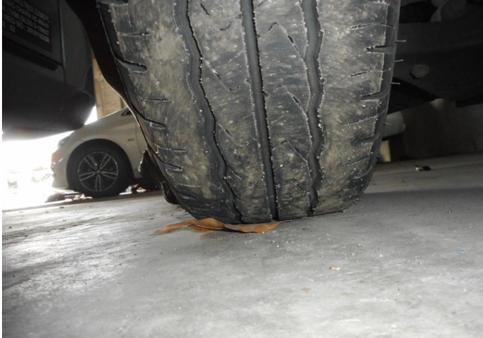
Photo 10 shows the condition of the rear right tyres of the Motor Lorry, which were observed to be in serviceable condition with remaining, tread depth of approximately 5.5mm. There was also no tear, cut or burst mark(s) on the outer and the inner sidewalls as well as across the tread of the 4 tyres that were fitted on the Motor Lorry.
