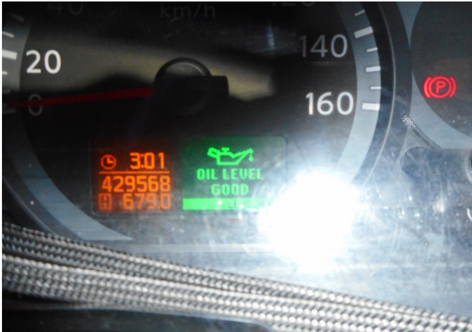
Photo 14 shows the engine oil display panel of the Motor Lorry at the time of my inspection. The engine oil was observed to be of sufficient level and without any contamination.
