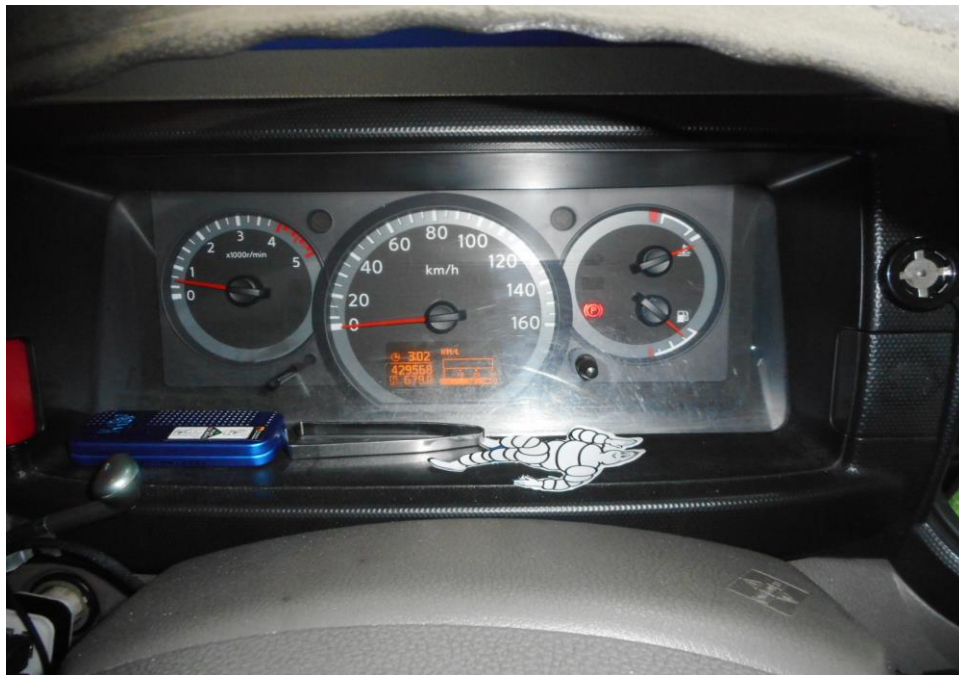
Photo 24 shows no warning lights illuminated on the instrument panel of the Motor Lorry after the engine was cranked. This would suggest that there was no abnormality to the electronic operating system of the Motor Lorry, like the ABS, etc.
