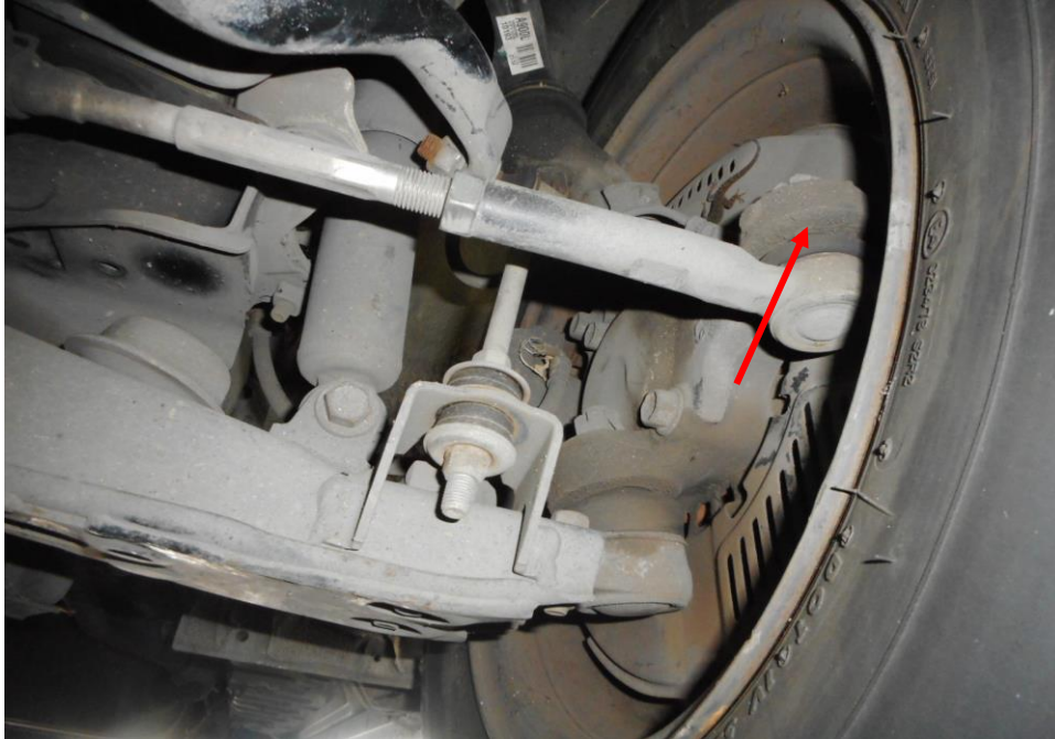
Photo 20 shows the various undercarriage components at the front left wheel of the Mini Bus, in particular the steering tie rod end (arrowed). The various undercarriage components of the Mini Bus were all found to be intact without any visible damage. There was also no sign of fluid stain(s) observed on the various undercarriage components.
