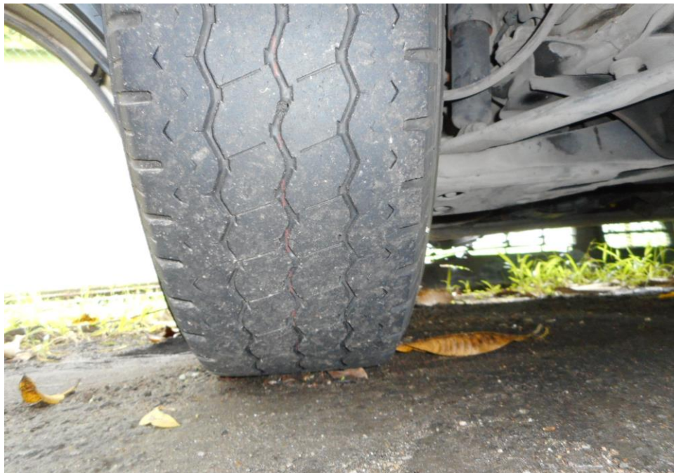
Photo 11 shows the condition of the rear right tyres of the Mini Bus, which were observed to be in serviceable condition with remaining, tread depth of approximately 2.7mm. There was also no tear, cut or burst mark(s) on the outer and the inner sidewalls as well as across the tread of the 4 tyres that were fitted on the Mini Bus.
