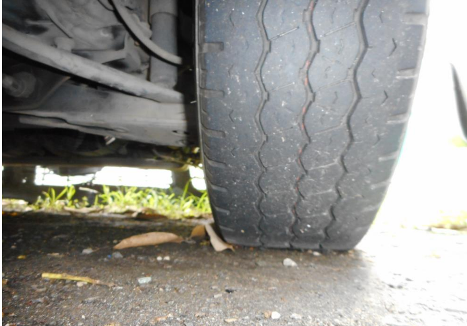
Photo 8 shows the condition of the front right tyre of the Mini Bus, which was observed to be in serviceable condition with remaining tread depth of approximately 3mm. The tyre, which was wrapped around standard steel wheel rim, was also observed to be sufficiently inflated for vehicular operation. There was no tear, cut or burst mark(s) on the outer and the inner sidewalls as well as across the tread of the 4 tyres that were fitted on the Mini Bus.
