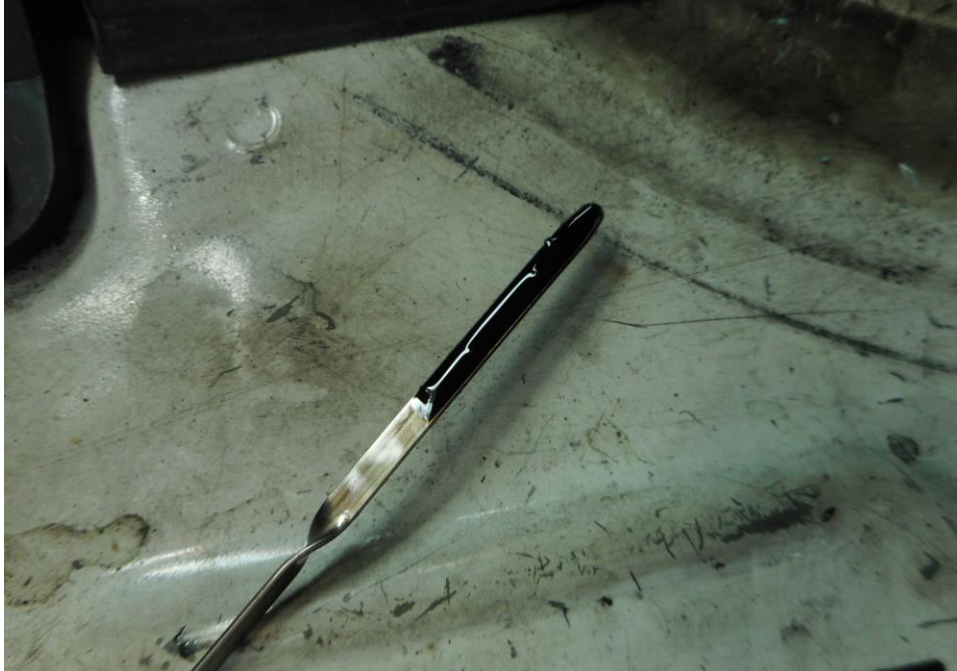
Photo 15 shows the engine oil dip stick of the Mini Bus at the time of my inspection. The engine oil was observed to be of sufficient level and without any visible contamination.
