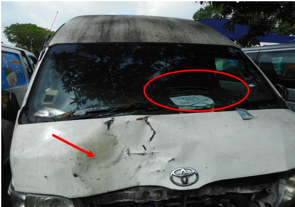
Photo 3 shows a general view of the Mini Bus's frontal portion at the time of my inspection. The Mini Bus front portion was observed to have sustained damage at its front windscreen (circled) and front body panel (arrowed) at the time of my inspection as result of the accident.
