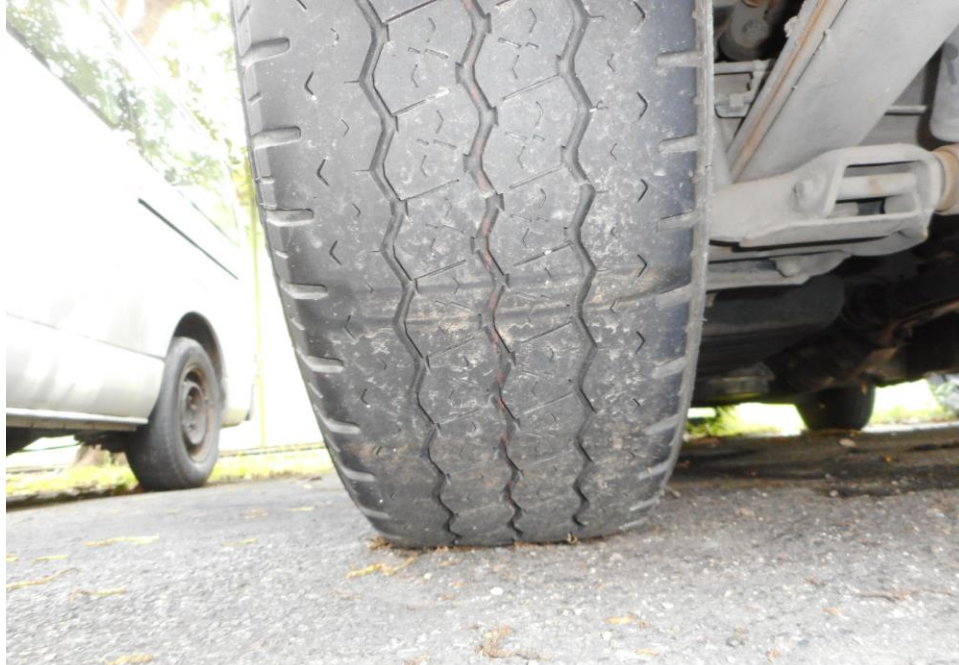
Photo 10 shows the condition of the rear left tyres of the Mini Bus, which was observed to be in serviceable condition with remaining tread depth of approximately 3.6mm. The tyres, which were wrapped around standard steel wheel rim, were also observed to be sufficiently inflated for vehicular operation. There was also no damage found on all 4 steel wheel rims of the Mini Bus.
