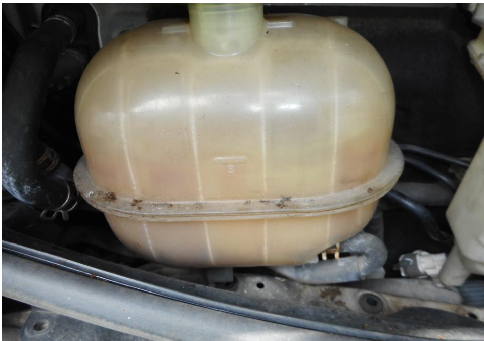
Photo 14 shows the engine coolant reservoir of the Mini Bus at the time of my inspection. The engine coolant was observed to be insufficient level as the damaged sustained from the accident had caused a leakage of engine coolant from the radiator.
