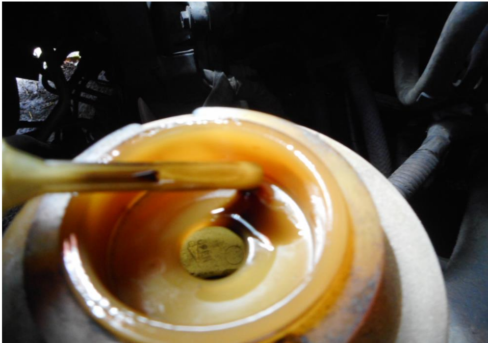
Photo 16 shows the power steering fluid reservoir of the Mini Bus at the time of my inspection. The power steering fluid was observed to be of sufficient level and without any visible contamination.
