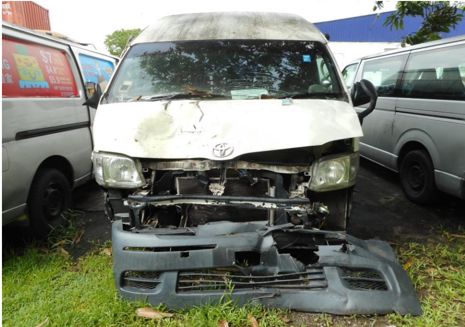
Photo 2 shows a general view of the Mini Bus's frontal portion at the time of my inspection. The Mini Bus front portion was observed to have sustained damage at its front windscreen, front body panel, front bumper and engine components were damage at the time of my inspection as result of the accident.
