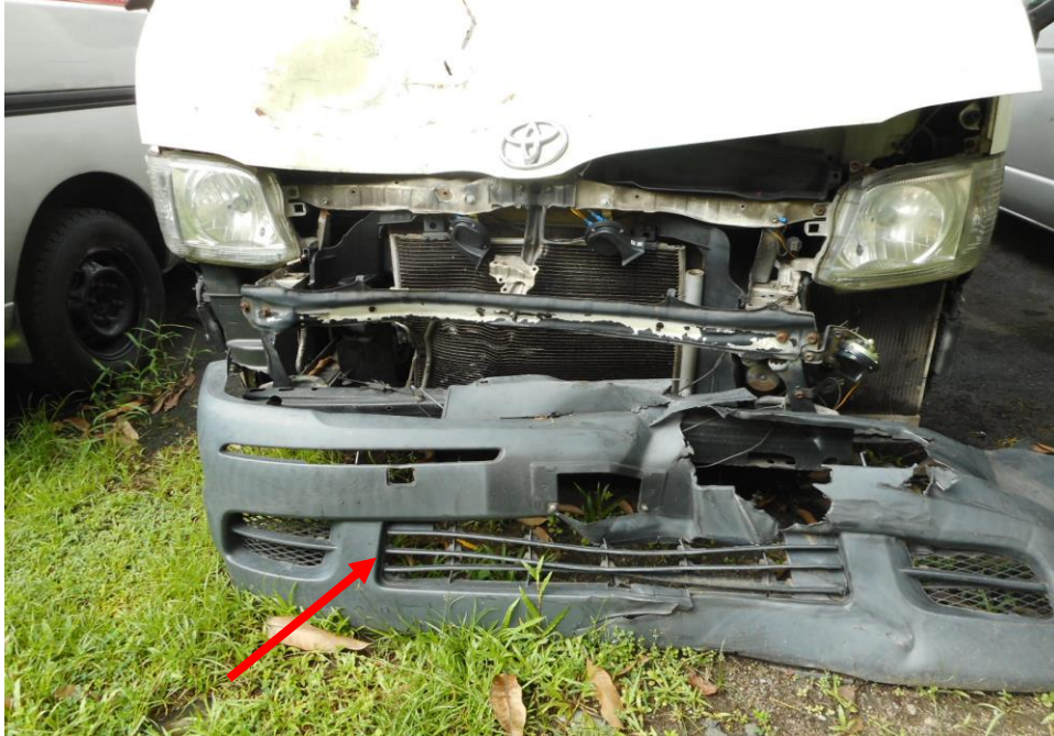
Photo 4 shows a general view of the Mini Bus's frontal portion at the time of my inspection. The Mini Bus front portion was observed to have sustained damage at its front bumper (arrowed) at the time of my inspection as result of the accident.
