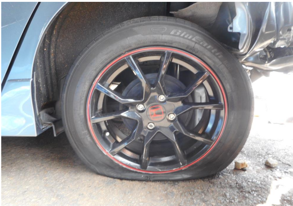
Photo 11 shows the condition of the rear left tyre of the Motor Car, which was observed to be cut and deflated as a result of the accident, with remaining tread depth of approximately 4.2mm.
