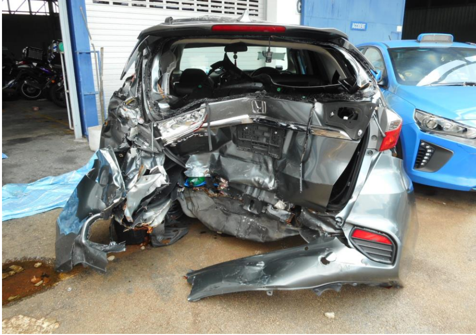
Photo 4 shows a general view of the Motor Car's rear body at the time of my inspection. The rear portion of the Motor Car was observed to have sustained damage. Its rear windscreen, rear boot and rear bumper was the body parts that were damaged as a result of the accident.
