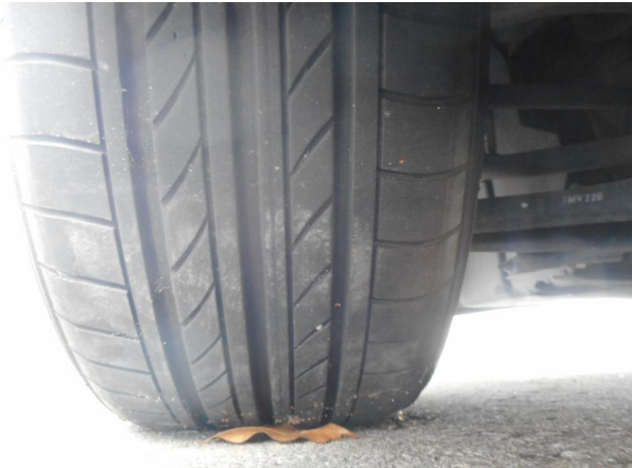
Photo 13 shows the condition of the front left tyre of the Motor Car, which was observed to be in serviceable condition with remaining tread depth of approximately 3.2mm. There was also no tear, cut or burst mark(s) on the outer and the inner sidewalls as well as across the tread of the Motor Car's 3 tyres.
