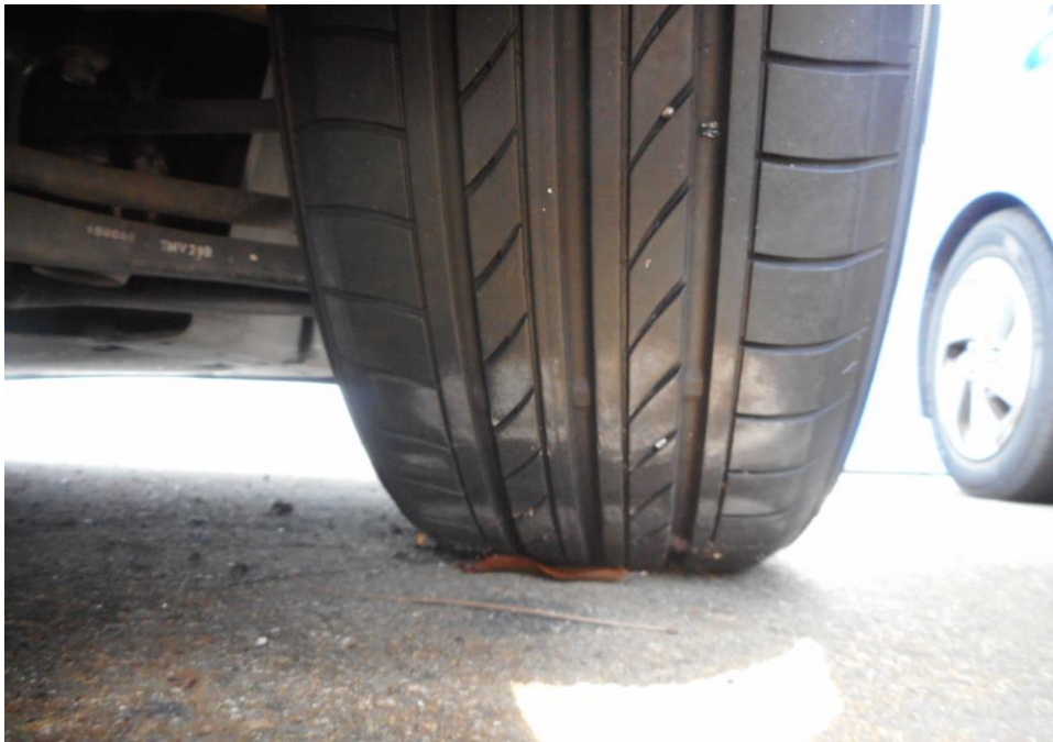
Photo 9 shows the condition of the front right tyre of the Motor Car, which was observed to be in serviceable condition with remaining tread depth of approximately 4.7mm. The tyre was sufficiently inflated for vehicular operation with no tear, cut or burst mark(s) on the outer and the inner sidewalls as well as across the tread. The 3 tyres of the Motor Car were wrapped around standard alloy wheel rims without any damage.
