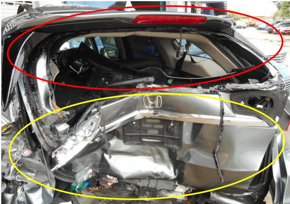
Photo 5 shows a close up view of the Motor Car's rear body at the time of my inspection. The rear portion of the Motor Car was observed to have sustained damage. Its rear windscreen (red circle) and rear boot (yellow circle) was the body parts that were damaged as a result of the accident.
