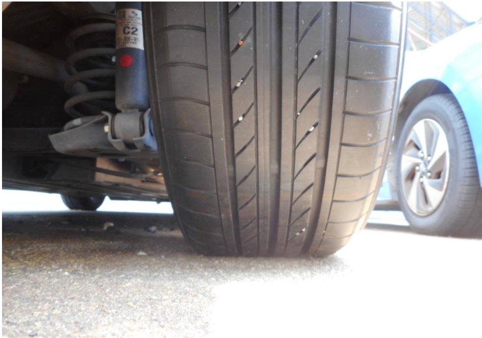
Photo 10 shows the condition of the rear right tyre of the Motor Car, which was observed to be in serviceable condition with remaining tread depth of approximately 3.9mm. The tyre was also observed to be sufficiently inflated for vehicular operation with no tear, cut or burst mark(s).
