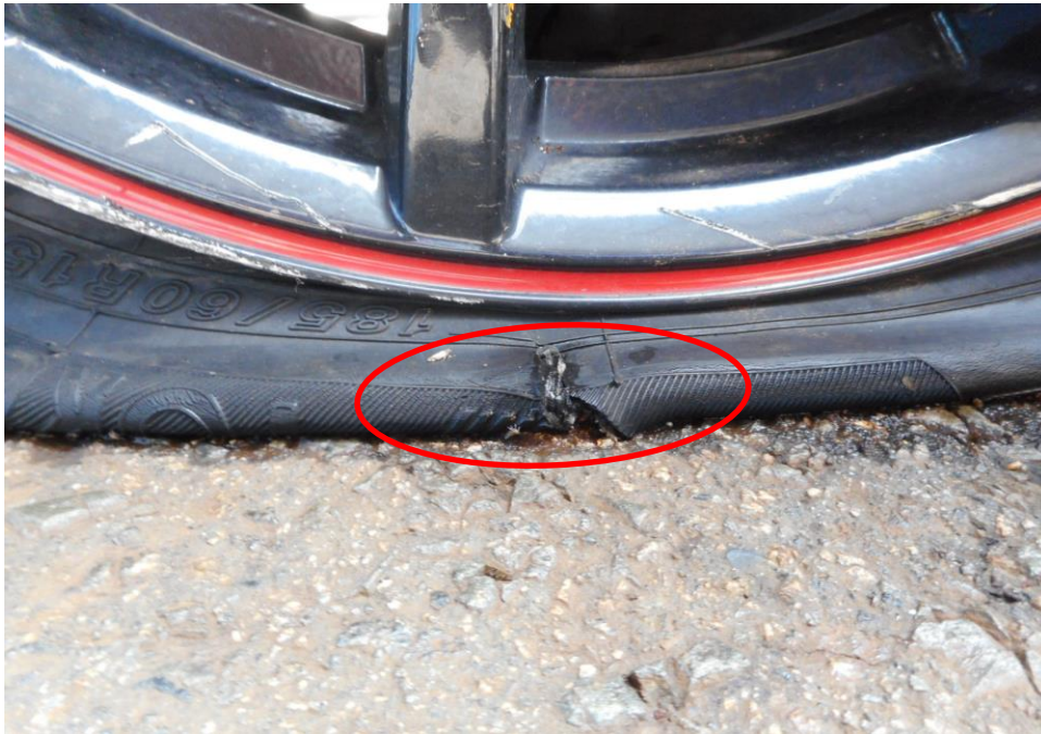
Photo 12 shows the close up condition of the rear left tyre of the Motor Car, which was observed to be cut and deflated (circled) as a result of the accident.
