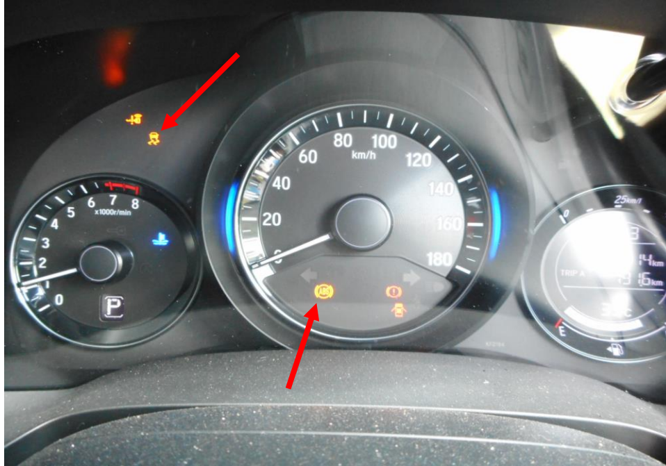
Photo 27 shows only the ABS and TC warning lights remained illuminated on the instrument panel of the Motor Car after the engine was cranked. This was likely due to the damaged rear left tyre as a result of the accident.
