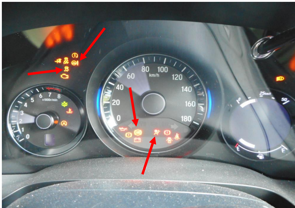
Photo 26 shows the warning light for Anti-Lock Brake System (ABS) and Power Steering System (EPS) and Supplemental Restraint System (SRS) (arrowed) appearing on the instrument panel of the Motor Car during the self-test of its various electronic operating systems when its engine was cranked.
